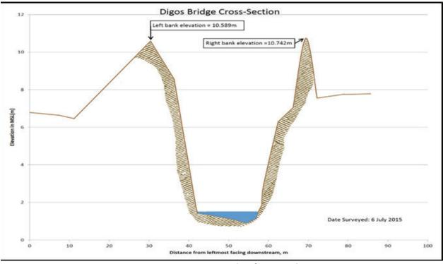
Figure 46. Cross-Section Plot of Digos Bridge
