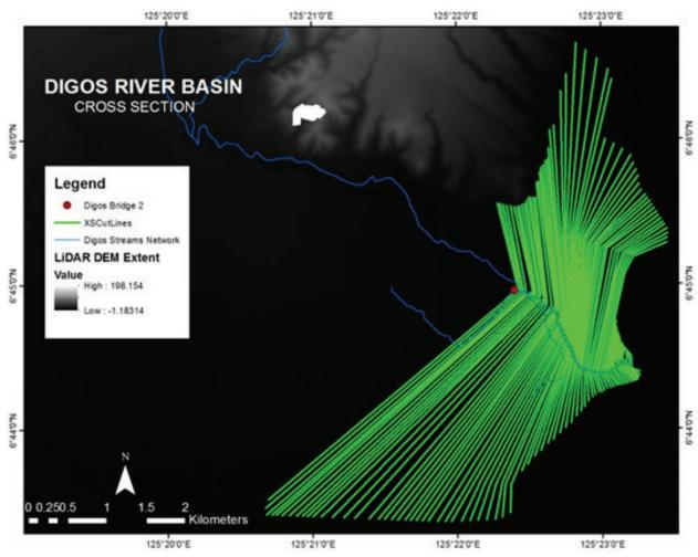
Figure 56. River cross-section of Digos River generated through Arcmap HEC GeoRAS tool
