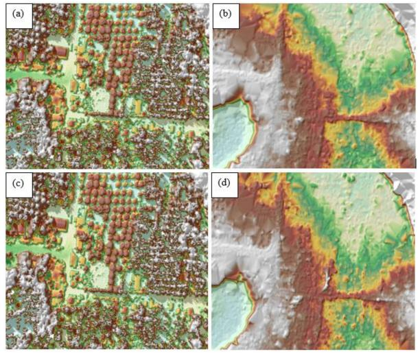
Figure 17. The production of last return DSM (a) and DTM (b), first return DSM (c) and secondary DTM (d) in some portion of Digos Floodplain
