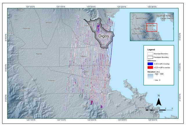
Figure 13. Elevation difference map between flight lines for Digos Floodplain.
