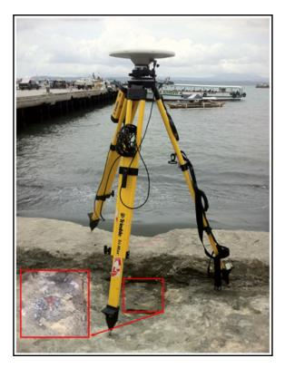
Figure 28. GNSS base receiver setup, Trimble® SPS 852 at DVS-1 at the east side of Pier, in Brgy. Leon Garcia Sr., Davao City, Davao Del Sur
