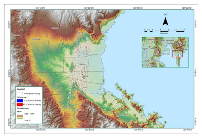
Figure A.8.14. Elevation difference between flight lines
