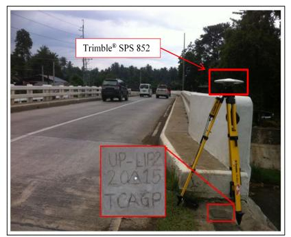
Figure 33. GNSS base receiver setup, Trimble® SPS 852 at UP-LIP2, on the right approach of Lipadas Bridge along National Highway in Brgy. Lizada, Toril District, Davao Del Sur
