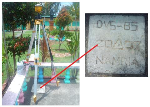
Figure 3. GPS set-up over DVS-85 located inside Mariano Sarona Elementary School, inside the fence of the flagpole (a) and NAMRIA reference point DVS-85 (b) as recovered by the field team.
