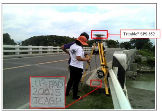
Figure 34. GNSS base receiver setup, Trimble® SPS 882 at UP-PAD, Padada Bridge, Brgy. Guihing, Municipality of Hagonoy, Davao del Sur
