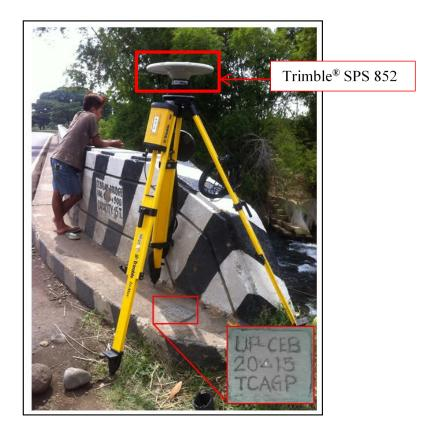
Figure 31. GNSS base receiver setup, Trimble® SPS 852 at UP-CEB on the right approach of Cebulan Bridge in Brgy Darong, Municipality of Santa Cruz, Davao Del Sur
