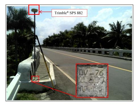
Figure 29. GNSS base receiver setup, Trimble® SPS 882 at DV-76 at the Gov. Miranda Bridge Approach, Brgy. Guadalupe, Municipality of Carmen, Davao Del Norte
