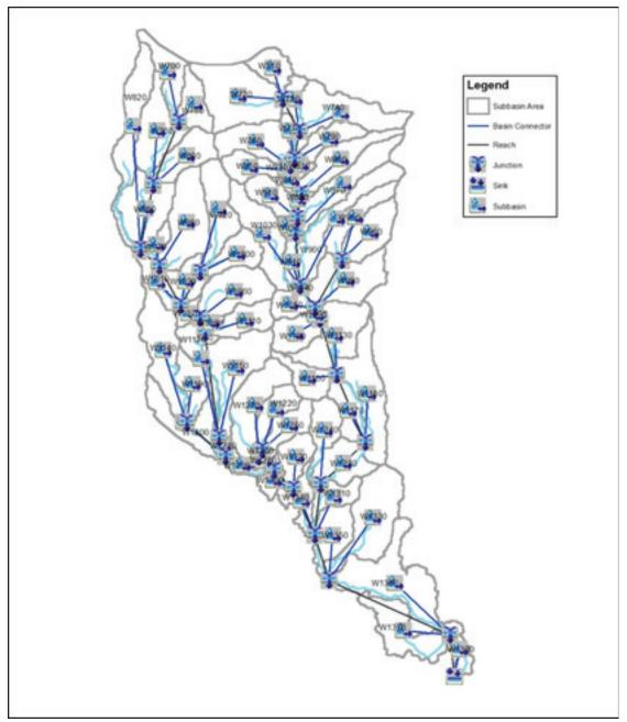
Figure 55. The Digos river basin model generated using  $\operatorname{HEC}\operatorname{-HMS}$
