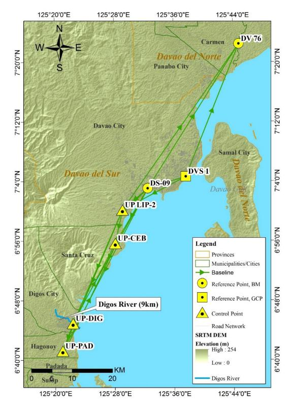
Figure 27. Overall GNSS Survey loop of Digos River Basin
