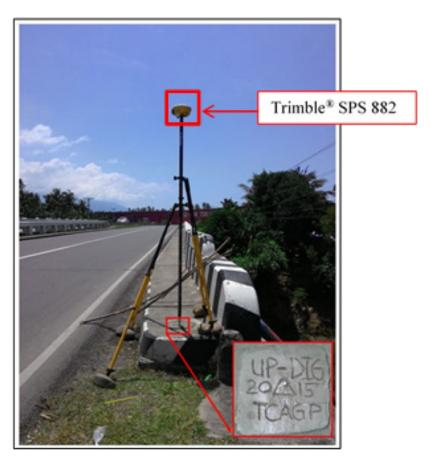
Figure 32. GNSS base receiver setup, Trimble® SPS 882 at UP-DIG, right approach of Digos Bridge in Brgy. Aplaya, Digos City, Davao Del Sur
