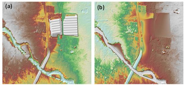
Figure 18. Portions in the DTM of Digos Floodplain – a building before (a) and after (b) manual editing
