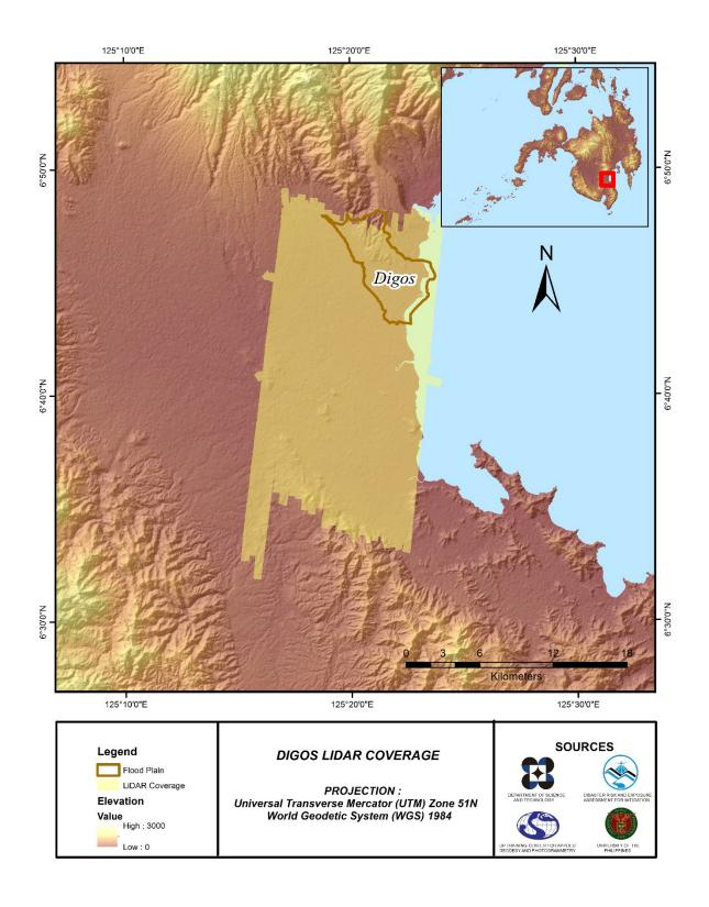
Figure 5. Actual LiDAR survey coverage for Digos floodplain
