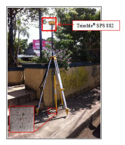
Figure 30. GNSS base receiver setup, Trimble® SPS 882 at DS-09 located at stair of Nograles Park along Mac Arthur Highway, in Brgy. Talomo, Davao City, Davao Del Sur
