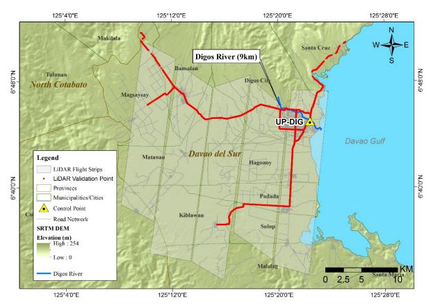
Figure 41. LiDAR Ground validation survey along Digos River Basin
