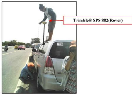
Figure 40. Validation points acquisition survey setup
