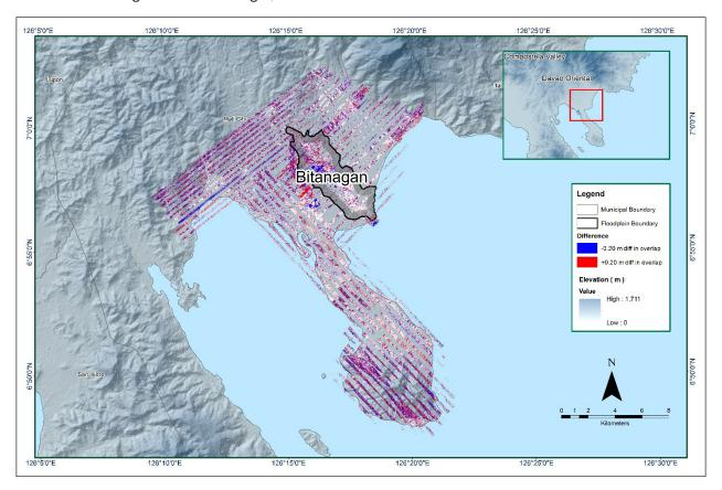
Figure 15. Elevation difference map between flight lines for Bitanagan Floodplain.
