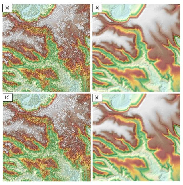
Figure 19. The production of last return DSM (a) and DTM (b), first return DSM (c) and secondary DTM (d) in some portion of Bitanagan Floodplain.
