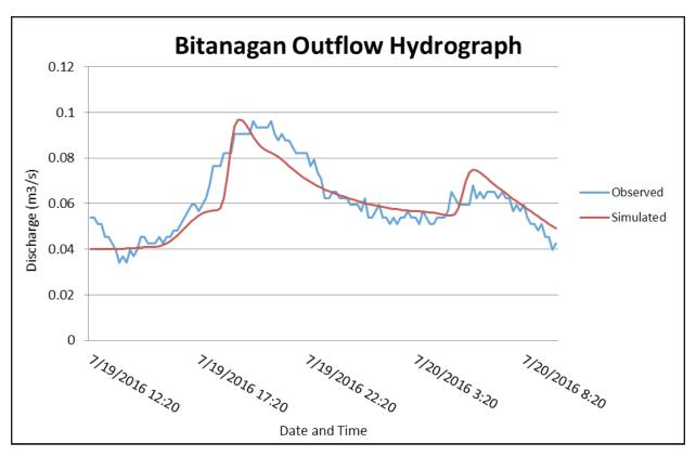
Figure 62. Outflow Hydrograph of Bitanagan produced by the HEC-HMS model compared with observed outflow Enumerated in Table 29 are the adjusted ranges of values of the parameters used in calibrating the model.
