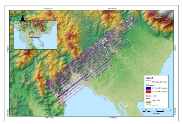
Elevation difference between flight lines
