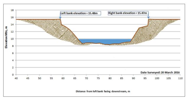
Figure 50. Cross-Section Plot of Bitanagan Bridge
