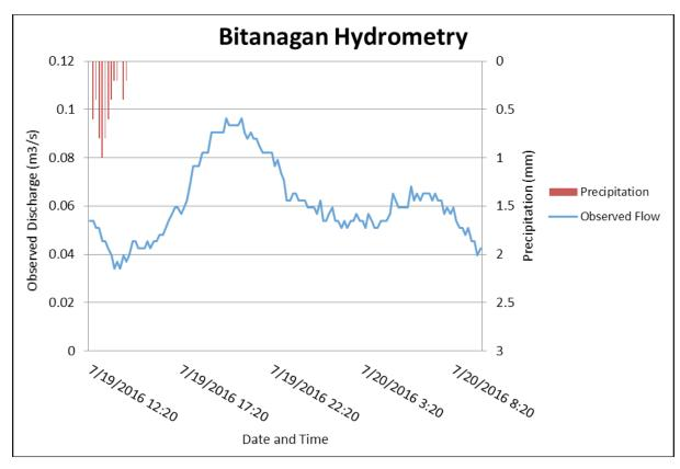
Figure 52. Rainfall and outflow data at Bitanagan Bridge used for modeling
