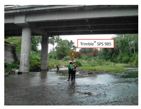
Figure 37. Gathering of random cross-section points along the downstream side of Bitanagan River
