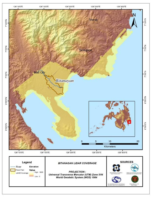
Figure 7. Actual LiDAR survey coverage for Bitanagan Floodplain.
