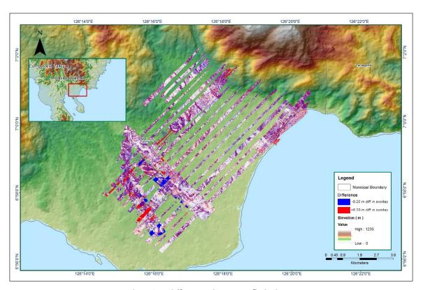
Elevation difference between flight lines
