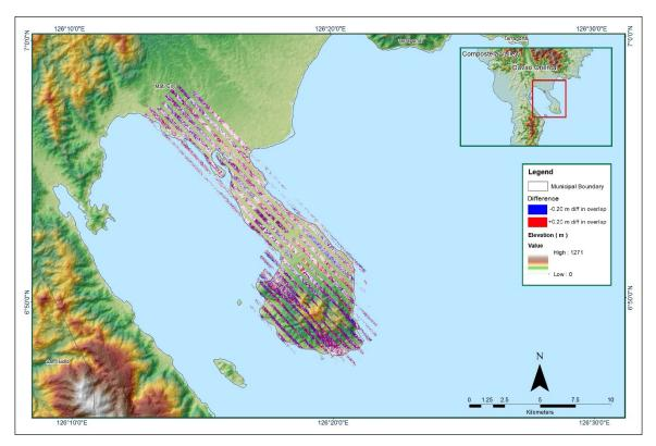
Elevation difference between flight lines
