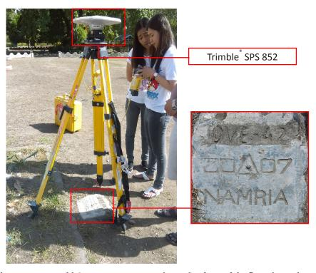
Figure 30. GNSS base set up, Trimble\* SPS 852, at DVE-42, located in front of the flagpole inside Don Enrique Lopez Elementary School in Brgy. Don Enrique Lopez, Mati City, Davao Oriental
