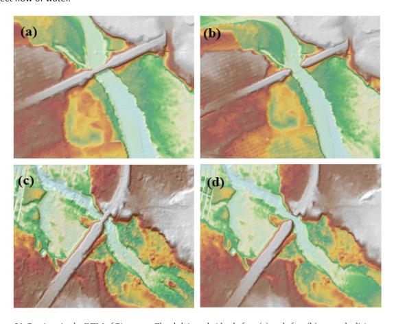
Figure 20. Portions in the DTM of Bitanagan Floodplain– a bridge before (a) and after (b) manual editing; a paddy field before (c) and after (d) data retrieval.
