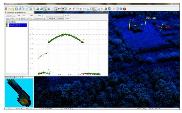
Figure 16. Quality checking for a Bitanagan flight 7318GC using the Profile Tool of QT Modeler.
