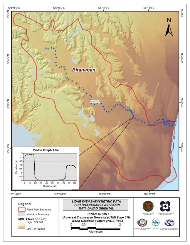
Figure 25. Map of Bitanagan Floodplain with bathymetric survey points shown in blue.
