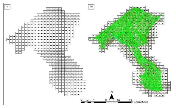
Figure 17. Tiles for Bitanagan Floodplain (a) and classification results (b) in TerraScan.
