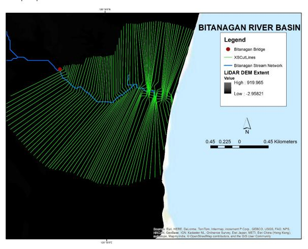
$Figure\ 60.\ River\ cross-section\ of\ Bitanagan\ River\ generated\ through\ Arcmap\ HEC\ GeoRAS\ tool$
