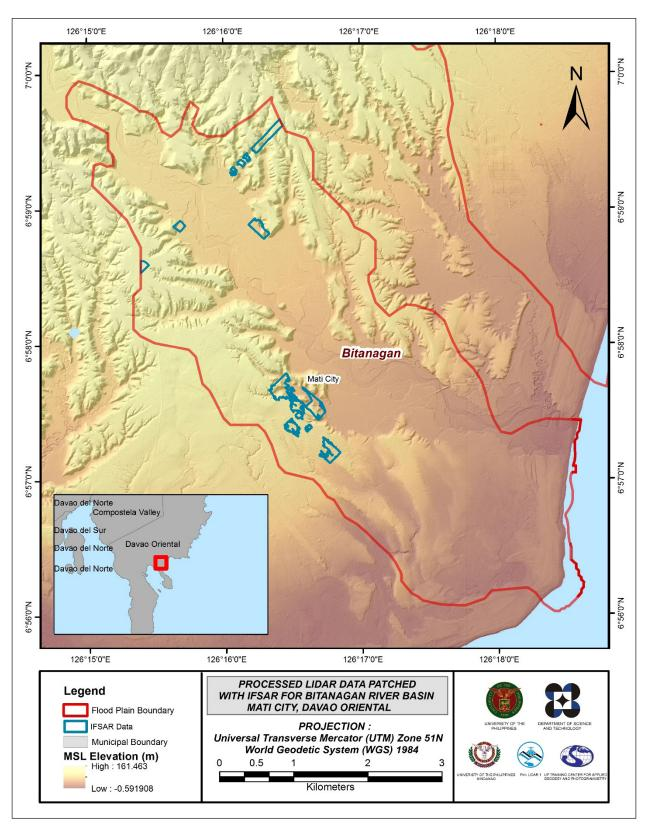
Figure 21. Map of Processed LiDAR Data for Bitanagan Floodplain.
