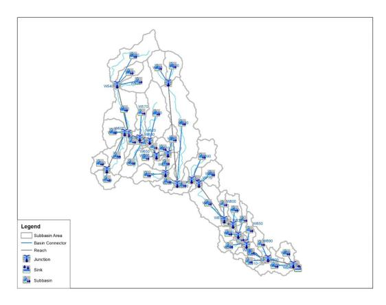
Figure 59. The Bitanagan river basin model generated using HEC-HMS.
