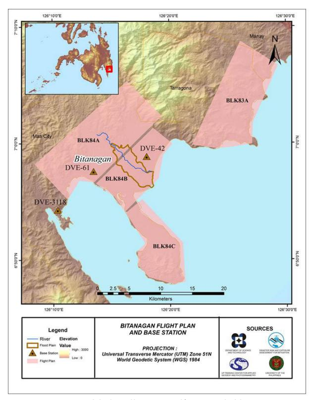
Figure 2. Flight plans and base stations used for Bitanagan Floodplain.
