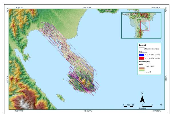
Elevation difference between flight lines
