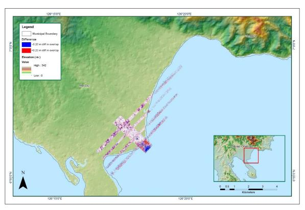
Elevation difference between flight lines
