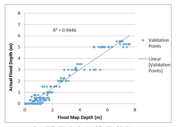
Figure 75. Flood Map Depth vs Actual Flood Depth for Bitanagan
