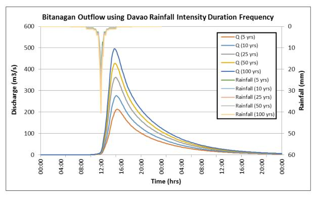
Figure 63. Outflow hydrograph at Bitanagan Station generated using the Davao RIDF simulated in HEC-HMS.
