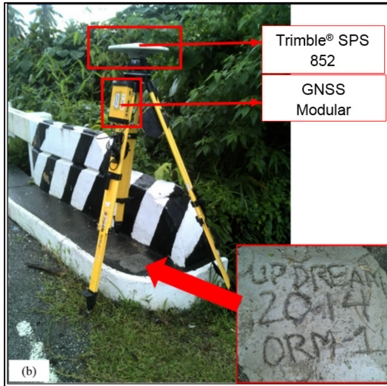
Figure 34. GPS setup of Trimble® SPS 852 at ORM-1, located on Subaan Bridge, Brgy. Subaan, Municipality of Socorro, Oriental Mindoro
