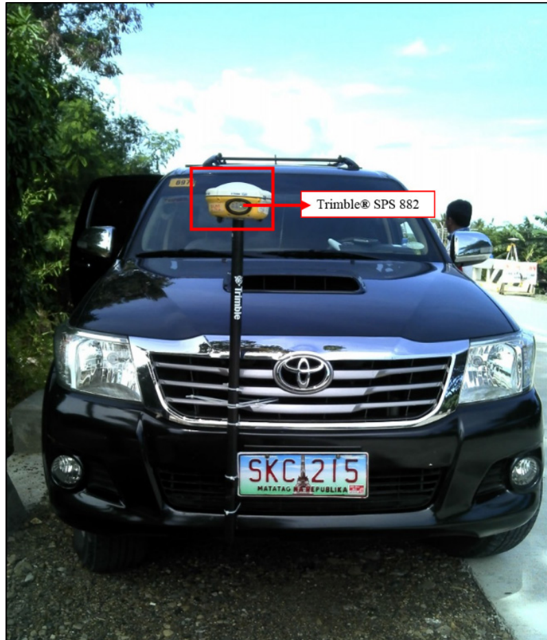
Figure 42. Trimble SPS®882 set-up for validation points acquisition survey for Sumagui River
