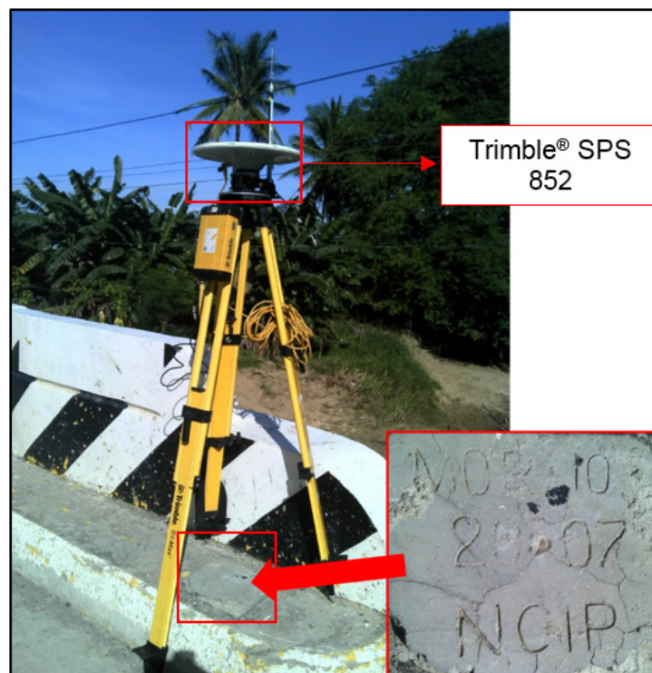
Figure 33. GPS setup of Trimble® SPS 852 at MOR-10, located in the approach of the Cawacat Bridge, in Brgy. Campasaan, Municipality of Bulalacao, Oriental Mindoro
