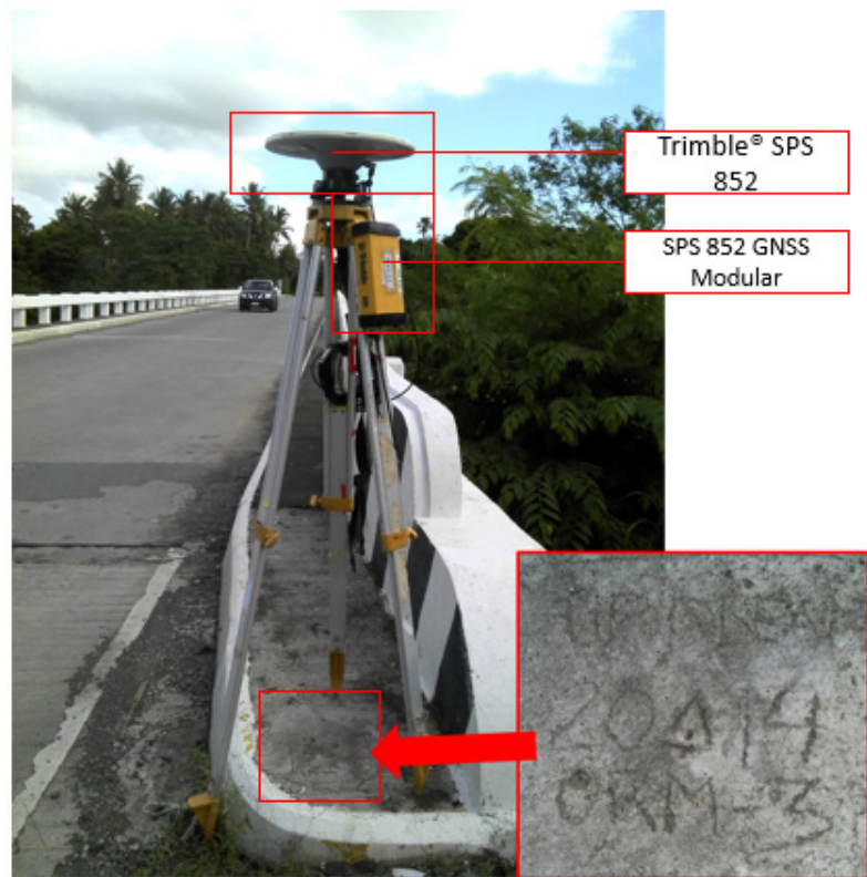
Figure 35. Trimble® SPS 985 setup at ORM-3 located at the approach of Balete Bridge, Brgy. Balete, Municipality of Gloria, Oriental Mindoro
