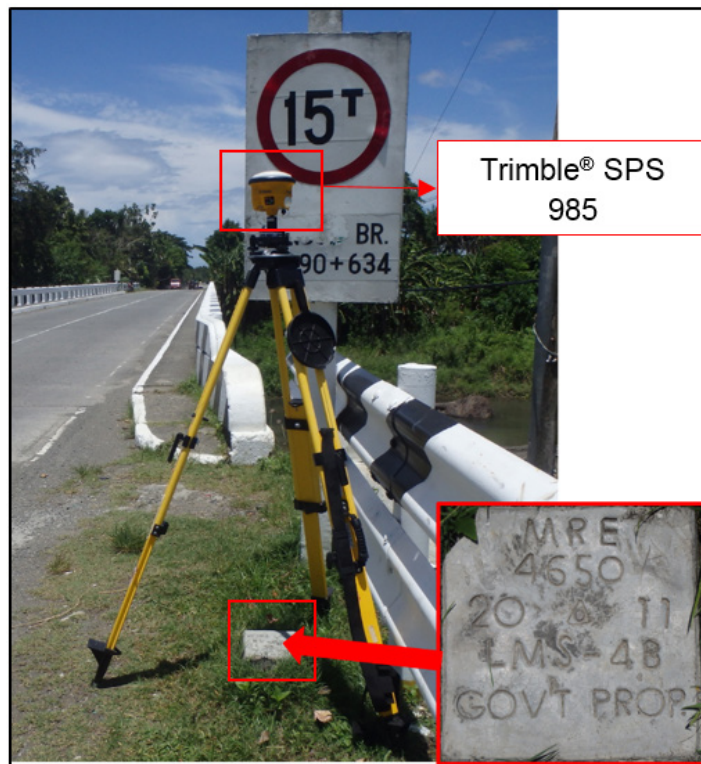
Figure 30. The GPS setup of Trimble® SPS 985 at MRE-4650, an LMS control point located at the approach of Bansud Bridge, in Brgy. Pagasa, Municipality of Bansud, Oriental Mindoro
