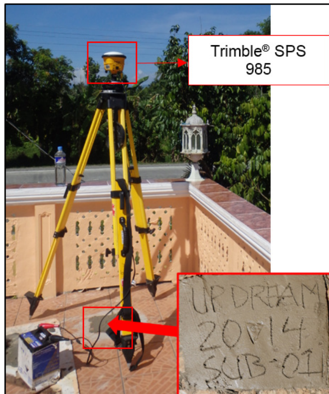
Figure 37. GPS setup of Trimble® SPS 985 at SUB-1, an established control point located at Maramot Residence in Brgy. Subaan, Municipality of Socorro, Oriental Mindoro
