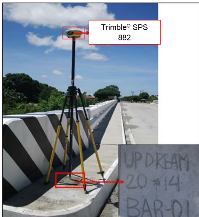
Figure 31. GPS setup of Trimble® SPS 882 at BAR-1, an established control point located in Baroc Bridge, Brgy. San Isidro, Mansalay, Oriental Mindoro
