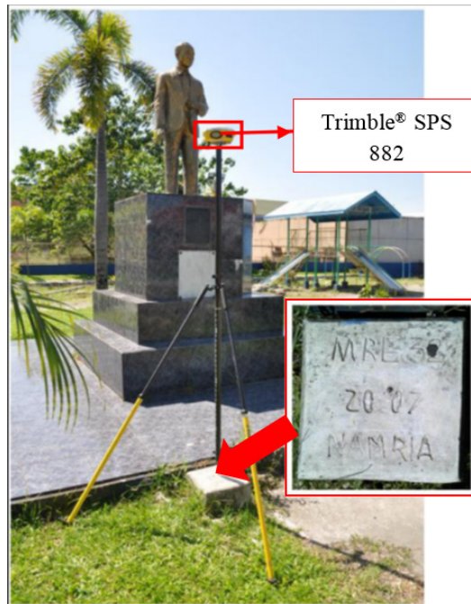
Figure 29. GPS setup of Trimble® SPS 882 at MRE-32, located at the Municipal Park of Victoria, in Brgy. Poblacion 1, Oriental Mindoro
