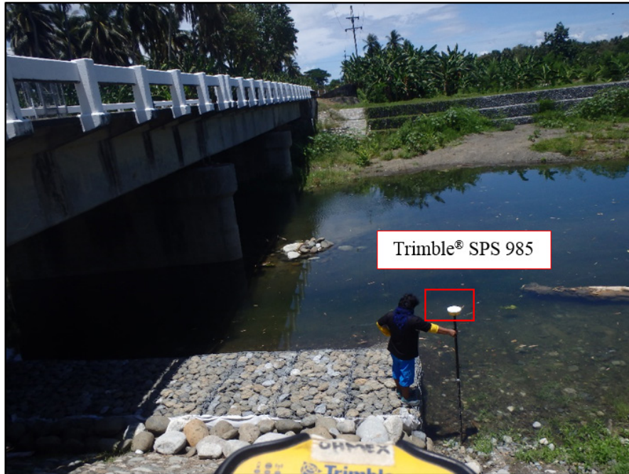
Figure 38. Cross-section and bridge as-built survey for Sumagui Bridge, Brgy Sumagui, Oriental Mindoro
