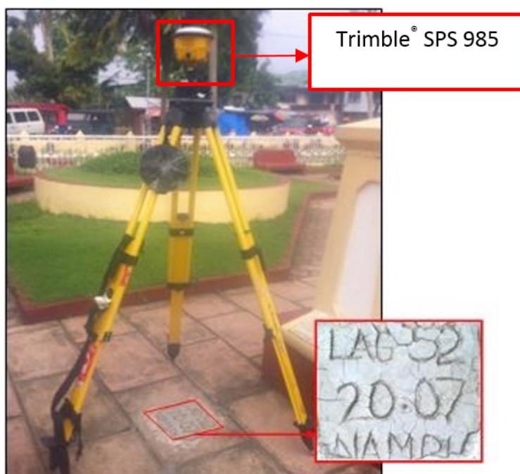
Figure 29. GNSS receiver set-up, Trimble® SPS 985 at LAG-52 in the Municipality of Magdalena, Laguna
