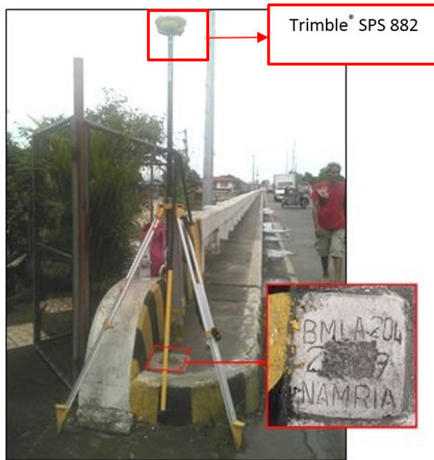
Figure 30. GNSS receiver set-up, Trimble® SPS 882 at LA-204 in the Municipality of Lumban, Laguna
