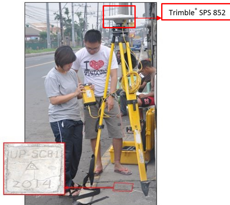
Figure 32. GNSS base receiver set-up, Trimble® SPS 852 at UP-SCB-1, San Cristobal Bridge in Calamba City, Laguna
