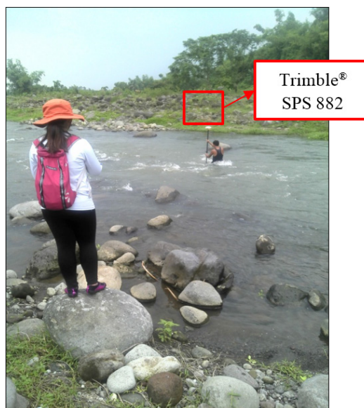
Figure 36. Manual Bathymetric survey in Sta. Cruz River
