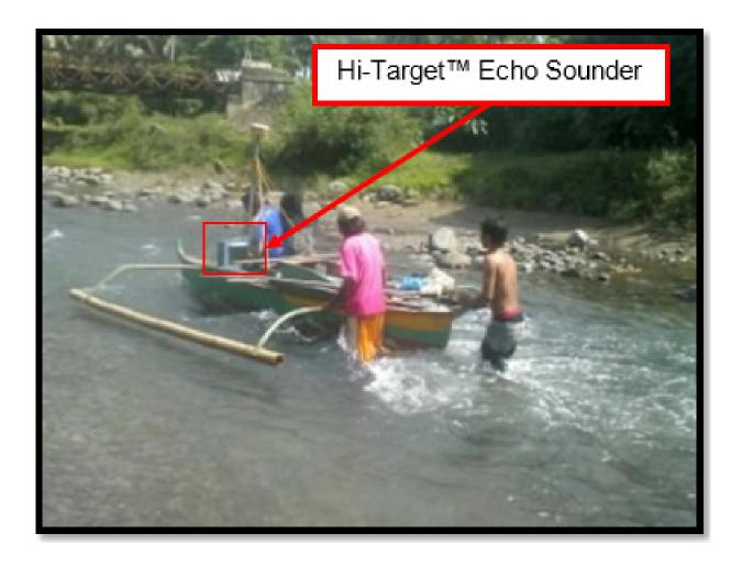
Figure 41. Bathymetric survey of ABSD at Ransang River using Hi-Target™ Echo Sounder (downstream)
