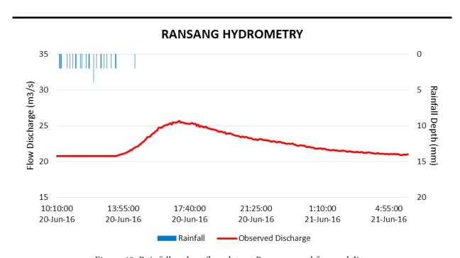
Figure 49. Rainfall and outflow data at Ransang used for modeling
