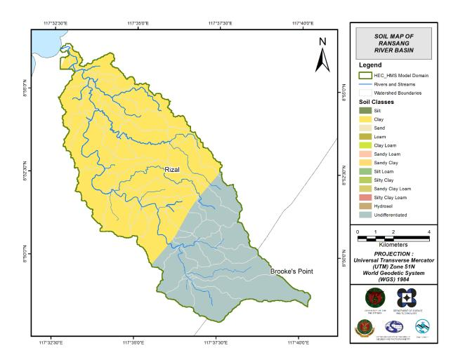
Figure 52. Soil map of Ransang River Basin used for the estimation of the CN parameter. (Source: DA)
