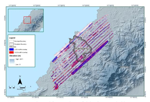
Figure 12. Elevation difference map between flight lines for Ransang Floodplain.
