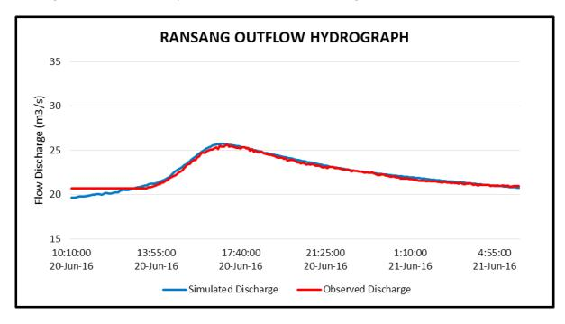
Figure 59. Outflow Hydrograph of Ransang produced by the HEC-HMS model compared with observed outflow.
