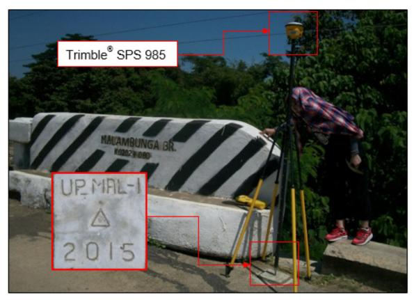
Figure 30. GNSS receiver set up, Trimble SPS 985, at UP\_MAL-1, Malambunga Bridge in Brgy. Punta Baja, Rizal, Province of Palawan
