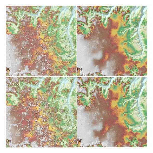
Figure 16. The production of last return DSM (a) and DTM (b), first return DSM (c) and secondary DTM (d) in some portion of Ransang Floodplain.
