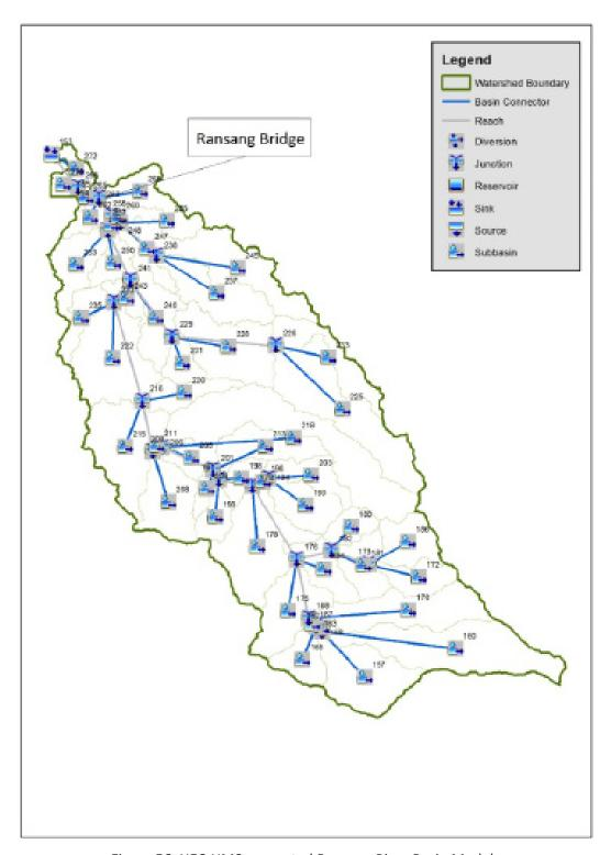
Figure 56. HEC-HMS generated Ransang River Basin Model.
