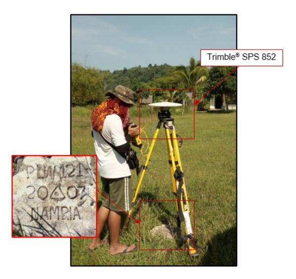
Figure 27. GNSS base set up, Trimble SPS 852, at PLW-121, located along the edge of a basketball court inside Cabkungan Elementary School in Brgy. Ransang, Rizal, Province of Palawan
