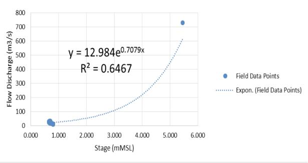
Figure 48. Rating Curve at Ransang Bridge, Rizal, Palawan
