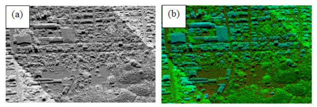
Figure 15. Point cloud before (a) and after (b) classification.
