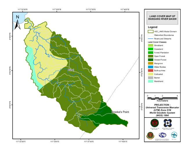
Figure 53. Land cover map of Ransang River Basin used for the estimation of the CN and watershed lag parameters of the rainfall-runoff model. (Source: NAMRIA)
