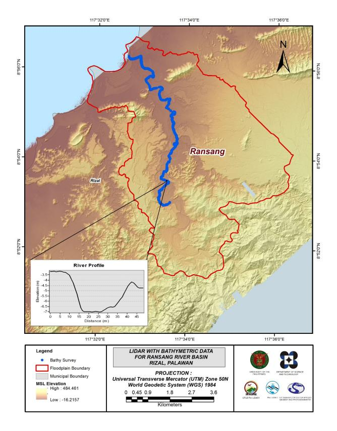
Figure 24. Map of Ransang Floodplain with bathymetric survey points shown in blue.
