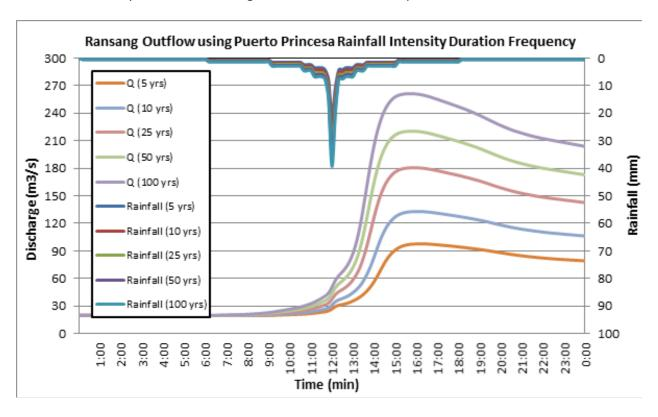
Figure 60. Outflow hydrograph at Ransang Station generated using Puerto Princesa RIDF simulated in HEC-HMS
