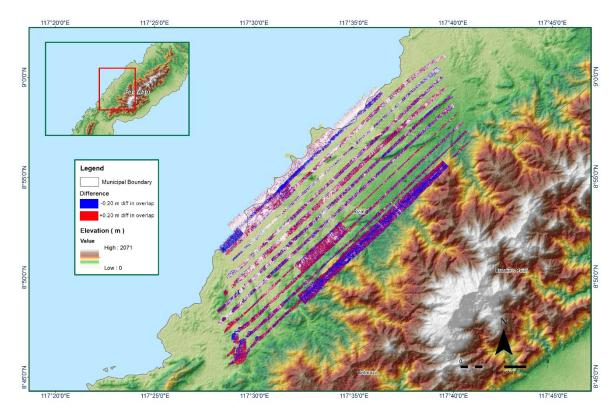
Figure A-8.7. Elevation difference between flight lines
