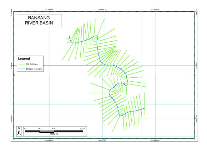
Figure 57. River cross-section of Ransang River generated through Arcmap HEC GeoRAS tool
