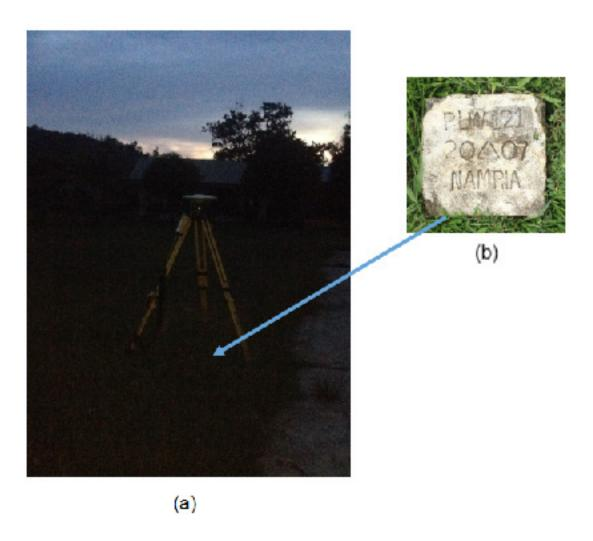
Figure 3. GPS set-up over PLW-121 as recovered within the vicinity of Cabkungan Elementary School in Brgy. Campong Ulay, Rizal, Palawan (a) and NAMRIA reference point PLW-121 (b) as recovered by the field team.
