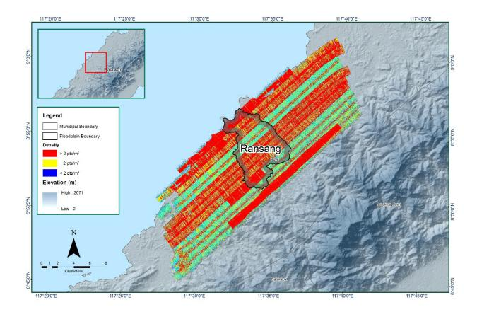
Figure 11. Pulse density map of merged LiDAR data for Ransang Floodplain.
