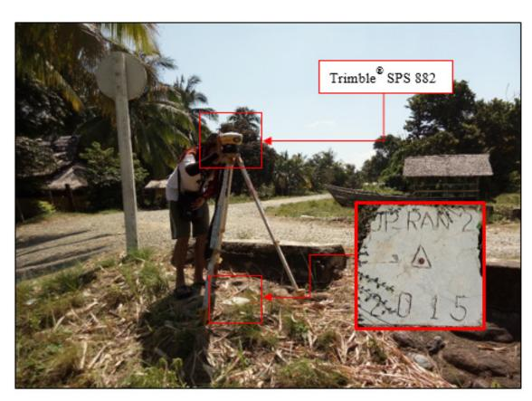
Figure 31. GNSS receiver set up, Trimble SPS 882, at UP\_RAN-2 beside the riprap near Ransang Bridge in Brgy. Ransang, Rizal, Province of Palawan
