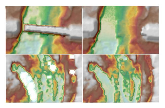
Figure 19. Portions in the DTM of Ransang Floodplain – a bridge before (a) and after (b) manual editing; and a data gap before (c) and after (d) filling.
