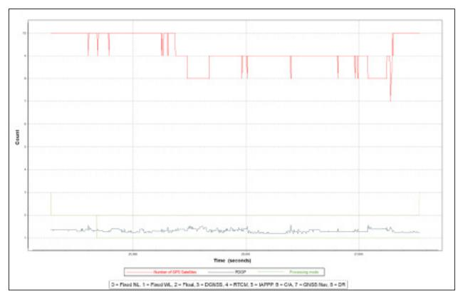
Figure 11. Solution Status Parameters of Pola Flight 3060P.
