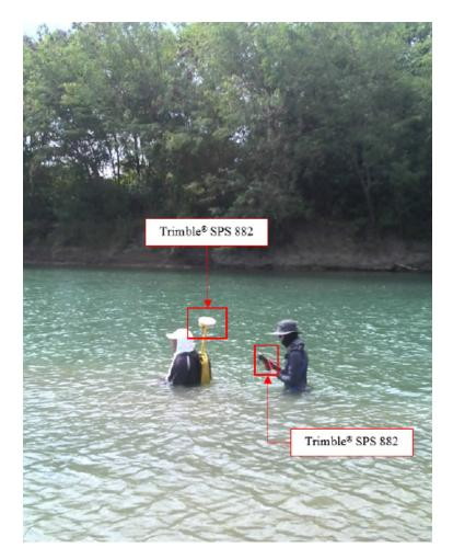
Figure 47. Manual Bathymetry set-up and execution for Pola River survey.
