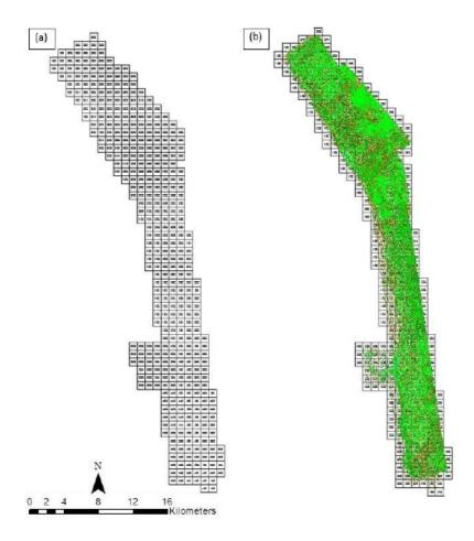
Figure 18. Tiles for Pola Floodplain (a) and classification results (b) in TerraScan.
