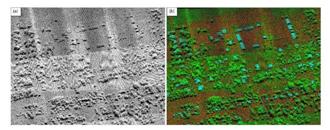
Figure 19. Point cloud before (a) and after (b) classification.
