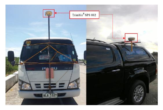
Figure 45. Validation points acquisition survey set-up
