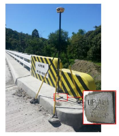
Figure 39. GNSS receiver set-up, Trimble® SPS 882, at UP-ALI, Alipid Bridge approach in Brgy. Sto. Niño, Municipality of Sablayan, Occidental Mindoro
