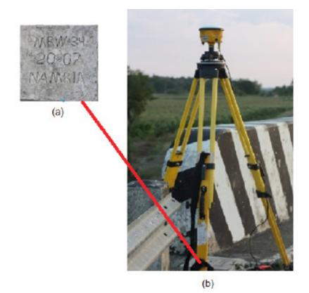
Figure 5. 5GPS set-up over MRW-34 as recovered in Balibago Bridge in Brgy. Armado, municipality of Abrade Ilog, Occidental Mindoro (a) and NAMRIA reference point MRW-34 (b) as recovered by the field team
