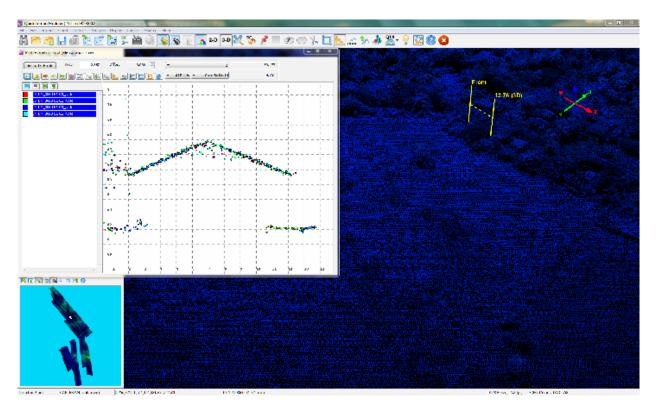
Figure 17. Quality checking for Pola flight 1166A using the Profile Tool of QT Modeler.
