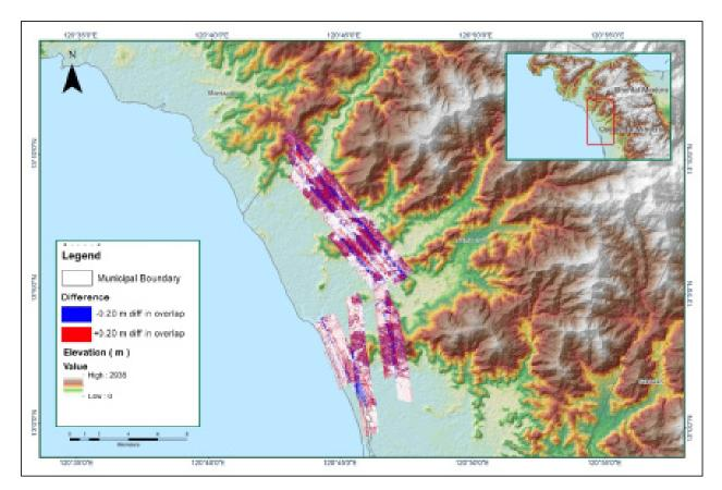
Figure A-8.28. Elevation difference between flight lines
