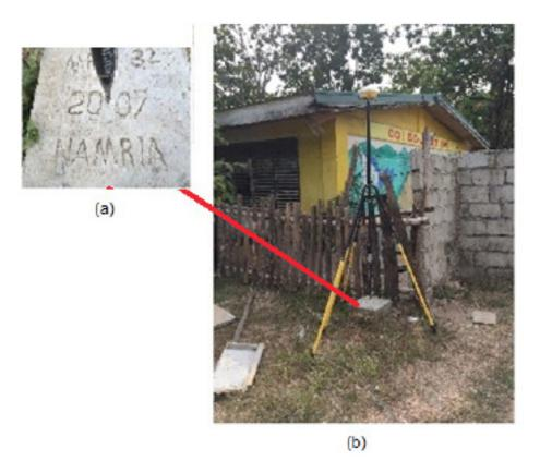
Figure 4. GPS set-up over MRW-32 as recovered in the corner of a day care center in Brgy. Fatima, municipality of Mamburao, Occidental Mindoro (a) and NAMRIA reference point MRW-32 (b) as recovered by the field
