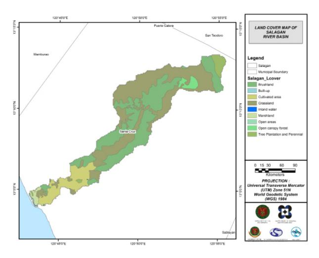
Figure 53. The land cover map of the Pola River Basin used for the estimation of the CN and watershed lag parameters of the rainfall-runoff model. (Source of data: Digital soil map of the Philippines published by the Bureau of Soil and Water Management – Department of Agriculture)
