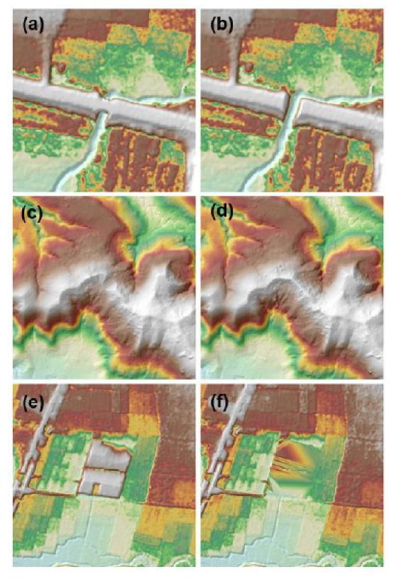
Figure 23. Portions in the DTM of Pola Floodplain – a bridge before (a) and after (b) manual editing; a mountain before (c) and after (d) data retrieval; and a building before (e) and after (f) manual editing
