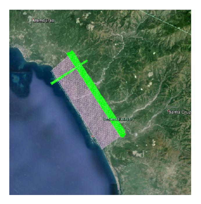
FLIGHT NO. 1124A BLK29O AREA: MISSION NAME: 3BLK29OS51A PARAMETERS: Alt: 600 Scan Freq: 40 kHz Scan Angle: 18 deg
