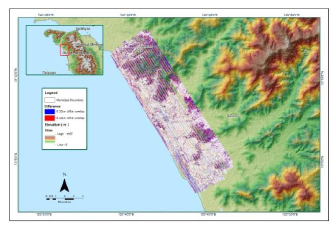
Figure A-8.7. Elevation difference between flight lines
