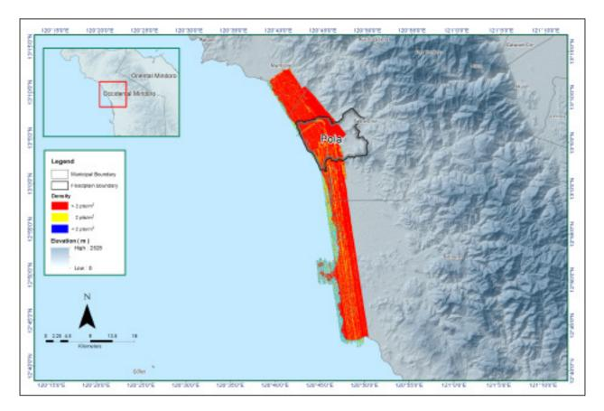
Figure 15. Density map of merged LiDAR data for Pola Floodplain.
