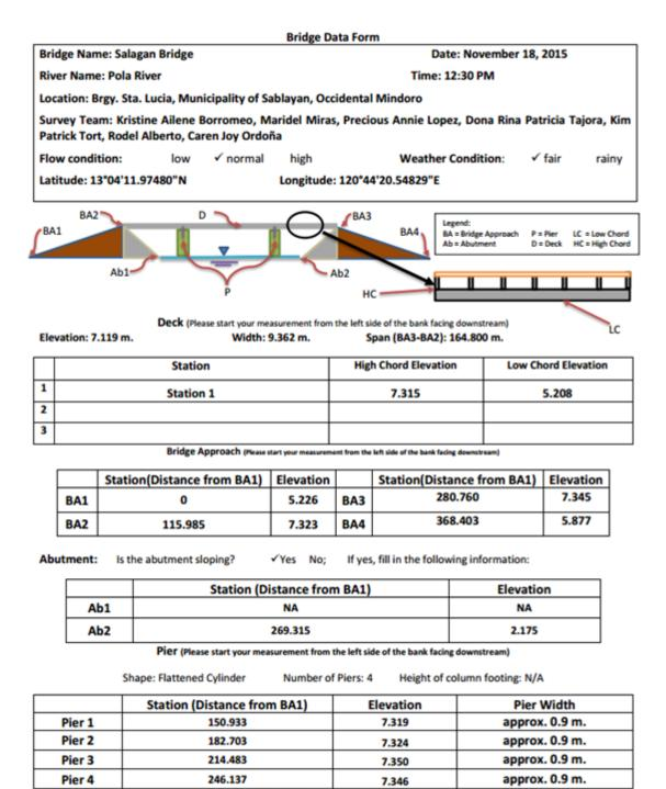
NOTE: Use the center of the pier as reference to its station
