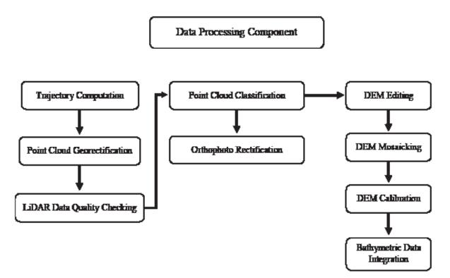
Figure 9. Schematic Diagram for Data Pre-Processing Component
