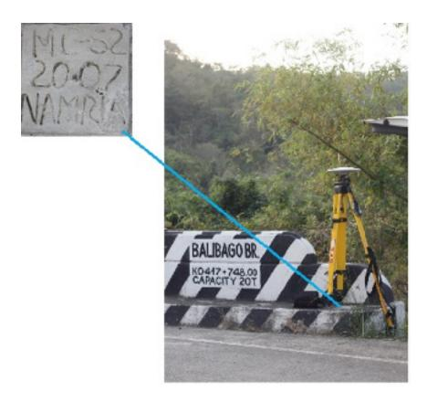
Figure 7. GPS set-up over MC-52as recovered in Balibago Bridge in Brgy. Armado, municipality of Abra de Ilog, Occidental Mindoro (a) and NAMRIA bench mark MC-52 (b) as recovered by the field team
