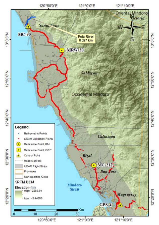
Figure 46. Validation Point Acquisition Survey for the Pola River Survey Area
