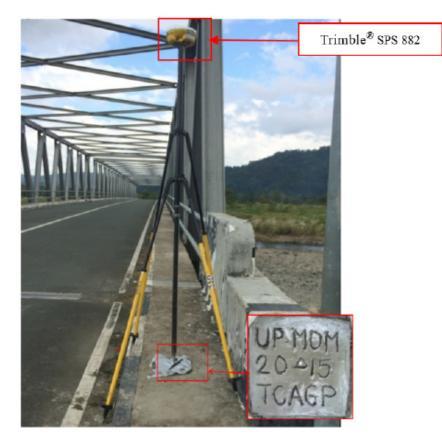
Figure 38. GNSS receiver set-up, Trimble® SPS 882, at UP-MOM, Mompong Bridge approached in Brgy. Lumang Bato, Municipality of Sablayan, Occidental Mindoro
