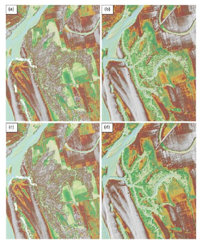
Figure 20. The production of last return DSM (a) and DTM (b), first return DSM (c) and secondary DTM (d) in some portion of Pola Floodplain.
