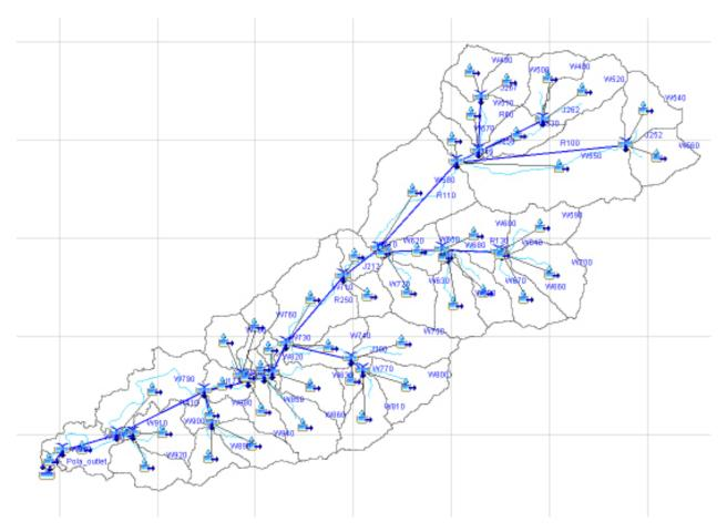
Figure 56. The Pola river basin model generated using HEC-HMS
