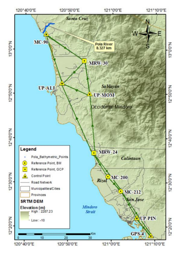
Figure 30. GNSS Network of Occidental Mindoro Field Survey
