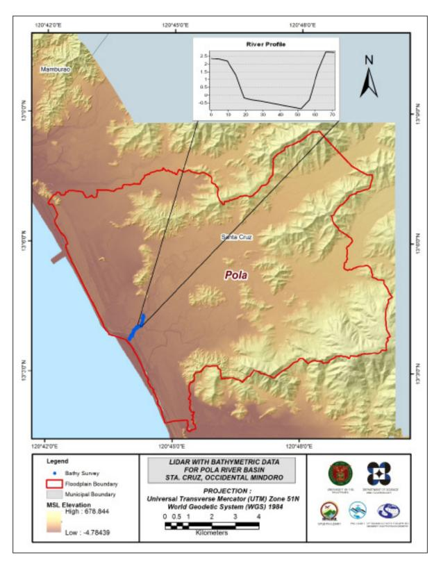
Figure 28. Map of Pola Floodplain with bathymetric survey points shown in blue.
