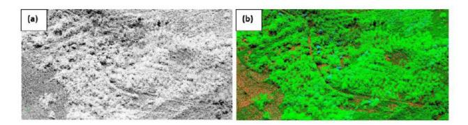
Figure 18. Point cloud before (a) and after (b) classification.
