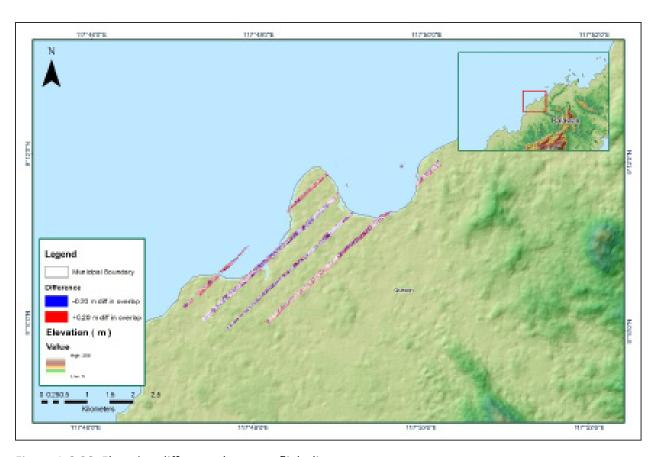
Figure A-8.28. Elevation difference between flight lines
