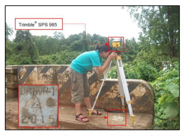
Figure 30. GNSS receiver set up, Trimble® SPS 985, at UP\_IWA-1, located at the approach of Iwahig Bridge in Brgy. Maasin, Quezon, Province of Palawan
