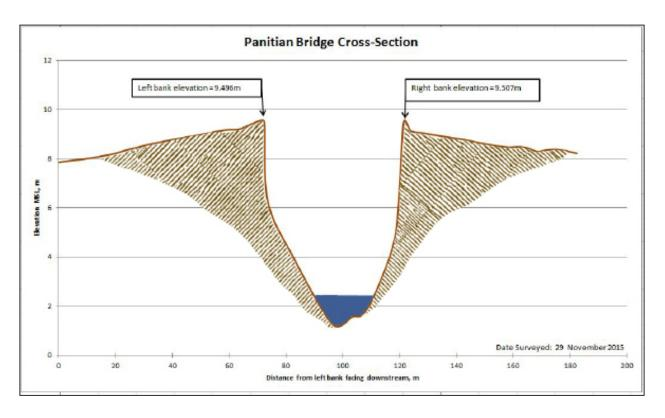
Figure 49. Cross-Section Plot of Panitian Bridge
