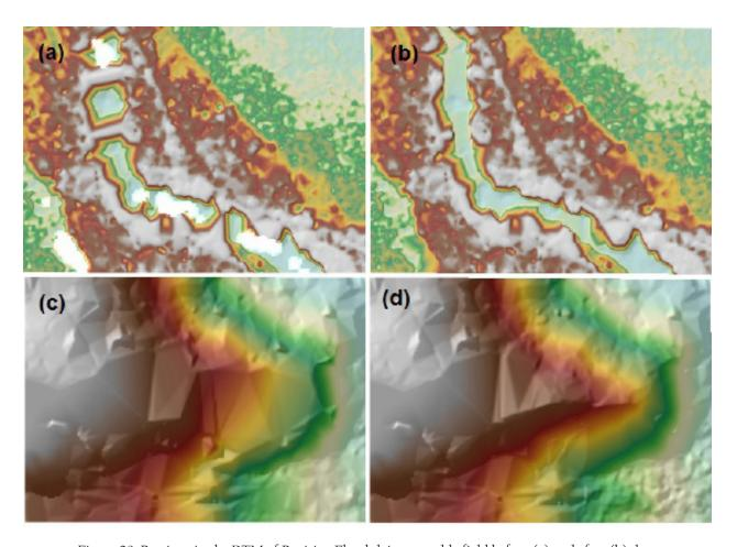
Figure 20. Portions in the DTM of Panitian Floodplain – a paddy field before (a) and after (b) data retrieval; a bridge before (c) and after manual editing (d).
