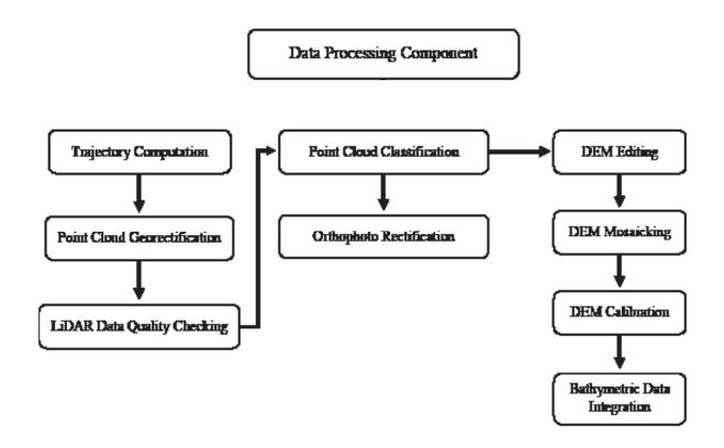
Figure 8. Schematic Diagram for Data Pre-Processing Component
