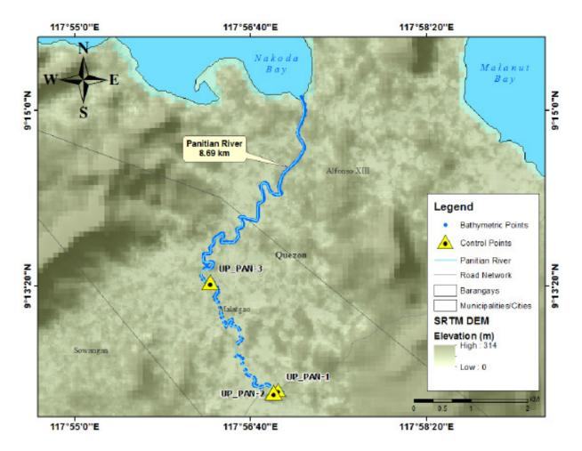
Figure 45. Bathymetric survey of Panitian River
