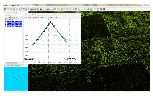
Figure 16. Quality checking for Panitian flight 3165P using the Profile Tool of QT Modeler.
