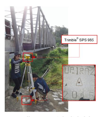
Figure 32. GNSS receiver set up, Trimble® SPS 985, at UP\_IRA-2, located on the side of Iraan Bridge in Brgy. Iraan, Rizal, Province of Palawan
