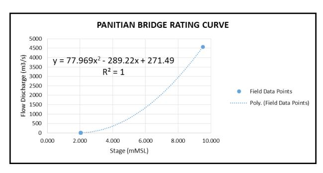
Figure 50. Rating curve at Panitian Bridge, Quezon, Palawan
