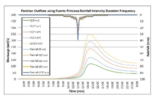
Figure 62. Outflow hydrograph at Panitian Station generated using Puerto Princesa RIDF simulated in HEC-HMS
