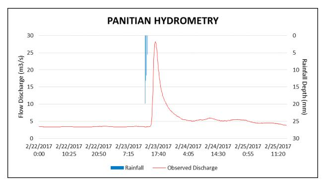
Figure 51. Rainfall and outflow data at Panitian River Basin used for modeling
