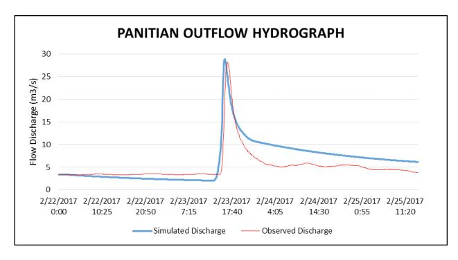
Figure 61. Outflow Hydrograph of Panitian produced by the HEC-HMS model compared with observed outflow.
