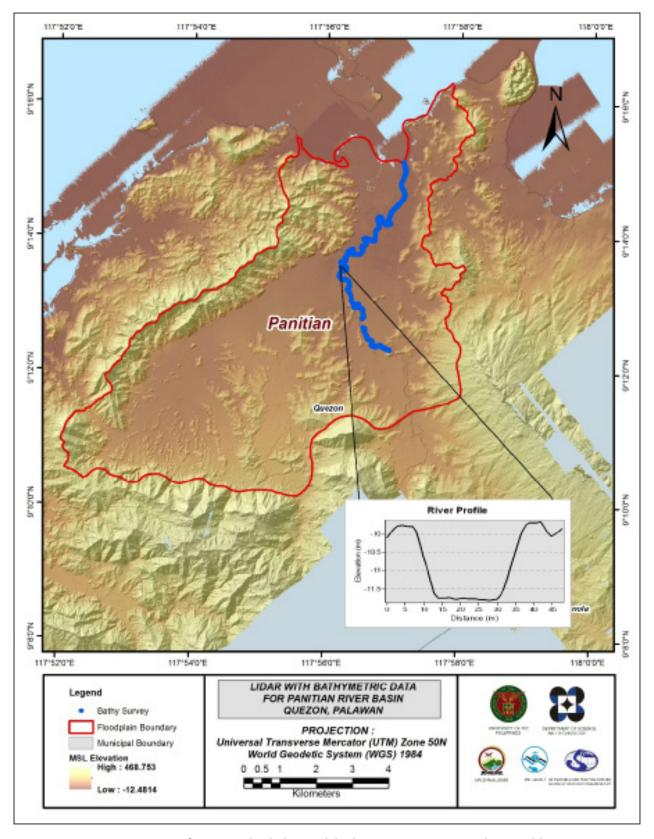
Figure 25. Map of Panitian Flood Plain with bathymetric survey points shown in blue.
