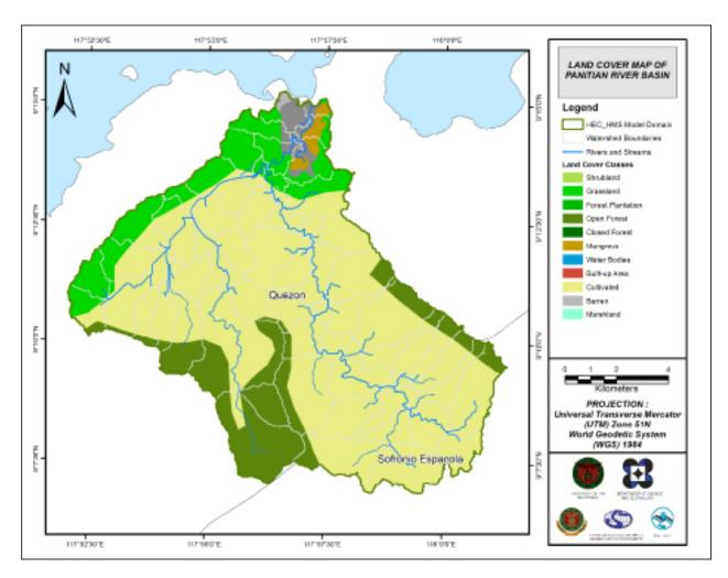
Figure 55. Land cover map of Panitian River Basin used for the estimation of the CN and watershed lag parameters of the rainfall-runoff model. (Source: NAMRIA)
