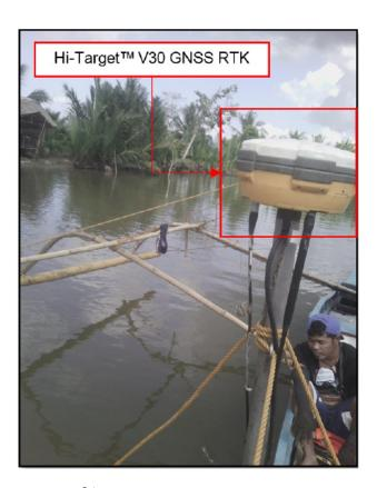
Figure 41. Bathymetric survey of ABSD at Panitian River using a Hi-Target™ GNSS Rover Receiver
