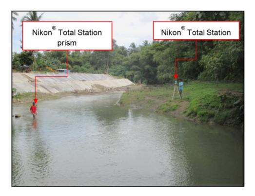
Figure 43. Manual bathymetric survey of ABSD at Panitian River using Nikon® Total Station
