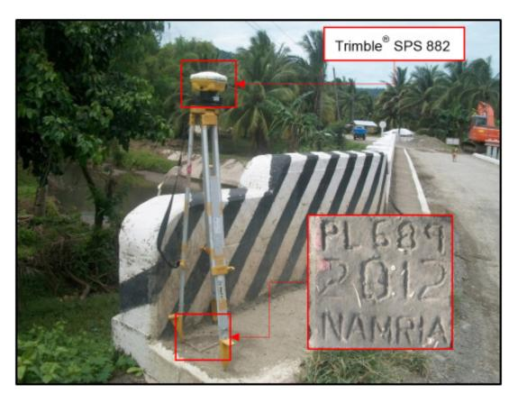
Figure 29. GNSS receiver set up, Trimble® SPS 882, at PL-689, located at the approach of Malatgao Bridge in Brgy. Sowangan, Quezon, Province of Palawan
