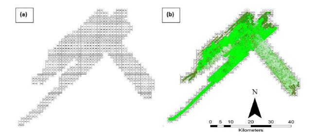
Figure 17. Tiles for Panitian Floodplain (a) and classification results (b) in TerraScan.
