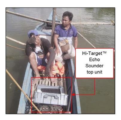
Figure 42. Bathymetric survey of ABSD at Panitian River using a Hi-Target™ Echo Sounder
