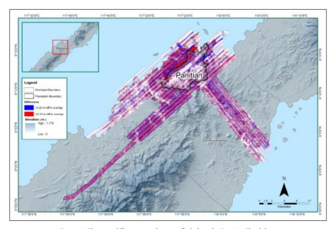
Figure 15. Elevation difference map between flight lines for Panitian Floodplain.
