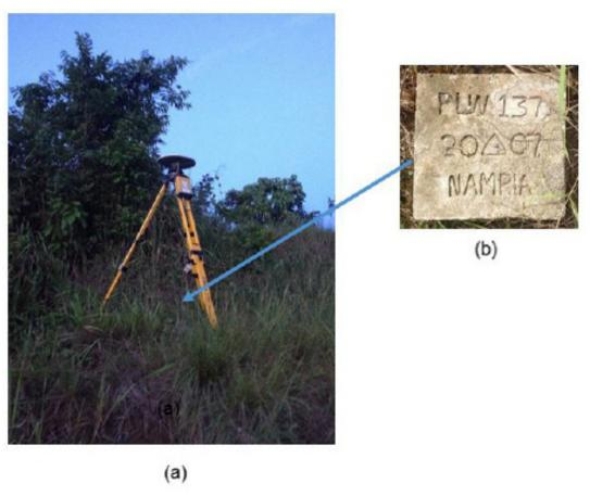
Figure 3. GPS set-up over PLW-137 as recovered at the top of the ridge along national highway in Brgy. Ipilan, Quezon, Palawan (a) and NAMRIA reference point PLW-137 (b) as recovered by the field team.
