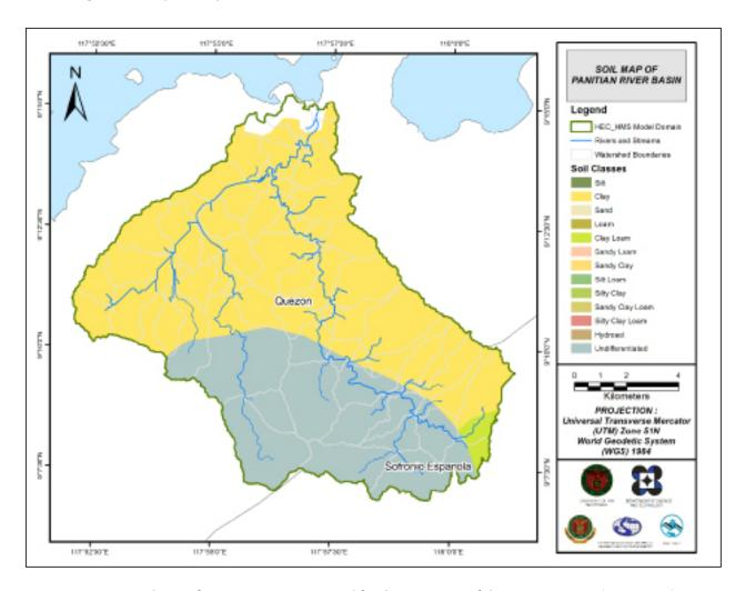
Figure 54. Soil map of Panitian River Basin used for the estimation of the CN parameter. (Source: DA)
