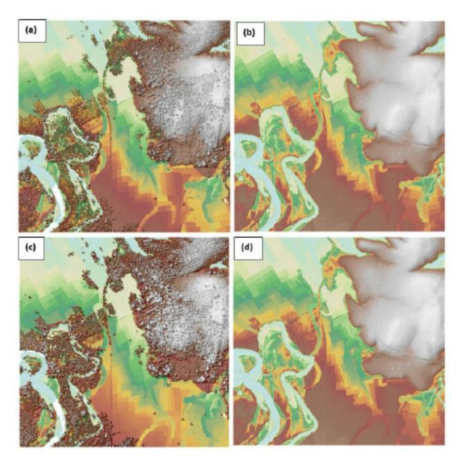
Figure 19. The production of last return DSM (a) and DTM (b), first return DSM (c) and secondary DTM (d) in some portion of Panitian Floodplain.
