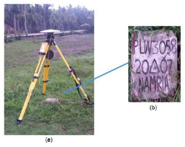
Figure 6. GPS set-up over PLW-3058 on the ground inside Caranasan Elementary School, Española, Palawan (a) and NAMRIA reference point PLW-3058 (b) as recovered by the field team.
