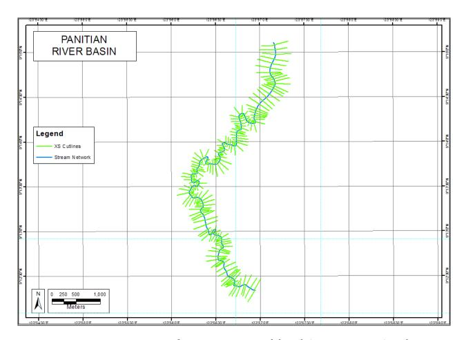
Figure 59. River cross-section of Panitian River generated through Arcmap HEC GeoRAS tool
