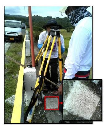
Figure 35. GNSS base receiver setup, Trimble\* SPS 852 at ATQ-20 in Brgy. Zaragoza, Municipality of Bugasong, Antique
