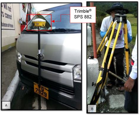
Figure 42. Setup of Trimble\* SPS 882 attached to a vehicle (A) and Setting up of GNSS base station at ATQ-20 (B)
