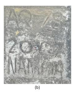
Figure 9. GPS set-up over AQ-78 as recovered in Barangay Ipayo, Patnongon, Province of Antique (a) NAMRIA reference point AQ-78 (b) as recovered by the field team.
