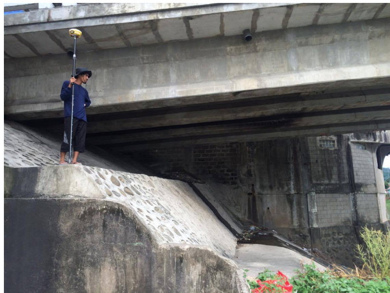
Figure 33. Cross-section survey at the Balanac Bridge
