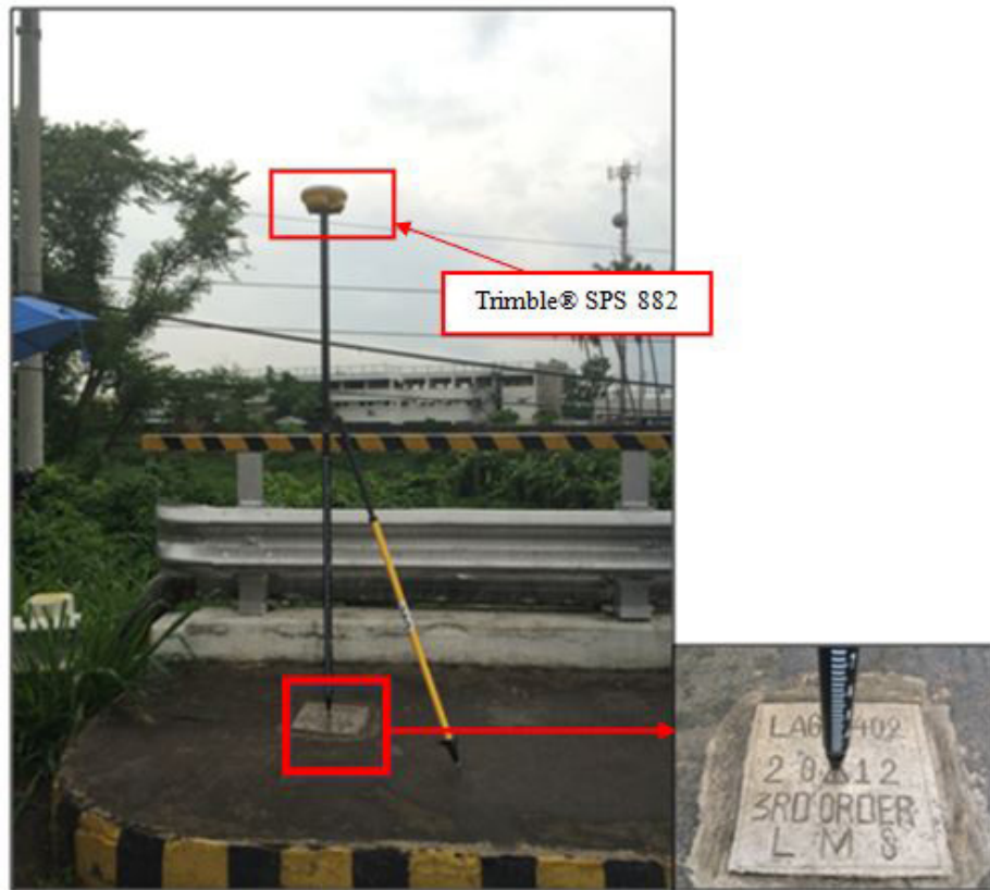
Figure 30. Trimble® SPS 882 GPS set-up at LAG 402 on the Pagsawitan Bridge, Pagsawitan, Laguna
