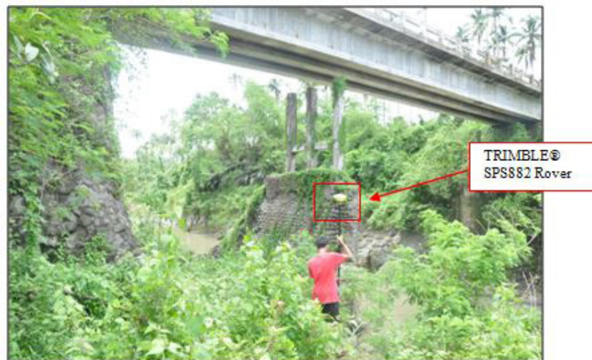
Figure 32. Cross-section survey at the Majayjay Bridge in Barangay Burlungan, Magdalena
