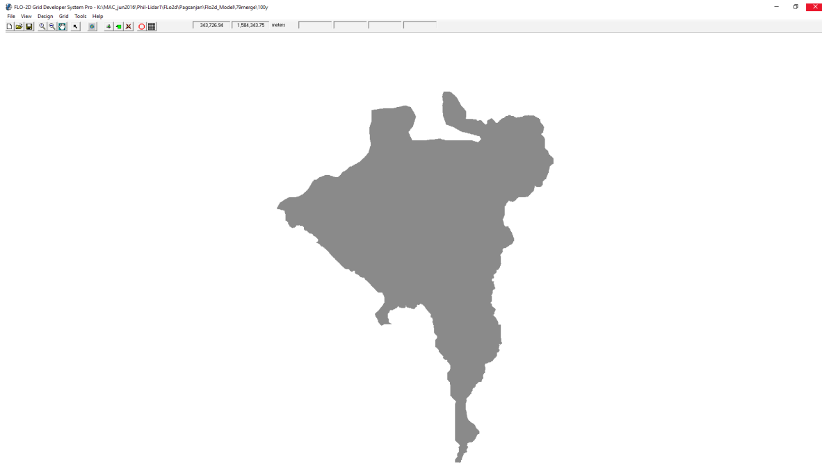
Figure 59. Screenshot of a sub-catchment with the computational area to be modeled in FLO-2D GDS Pro
