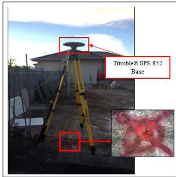
Figure 29. GNSS base receiver set-up, Trimble® SPS 852 at RB-1, located at the rooftop of Asia Blooms Hotel, Barangay Patimbao, Sta. Cruz, Laguna
