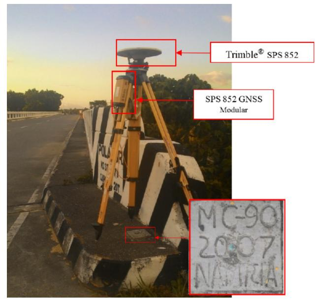
Figure 35. GNSS receiver, Trimble® SPS 852, at MC-90, used as marker, located at the Pola Bridge approach in Brgy. Barahan, Municipality of Santa Cruz, Occidental Mindoro
