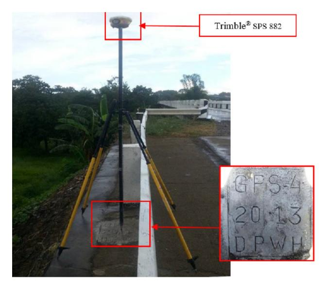
Figure 36. GNSS receiver, Trimble® SPS 882, at GPS-4 on right side of the road abutment after Caguray Bridge going to Bulalacao in Brgy. Poblacion, Municipality of Magsaysay, Occidental Mindoro
