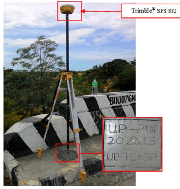
Figure 37. GNSS base receiver set-up, Trimble® SPS 882, at UP-PIN Pinamanaan Bridge approach in Brgy. Mapaya, Municipality of San Jose, Occidental Mindoro
