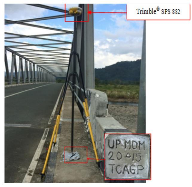
Figure 38. GNSS receiver set-up, Trimble® SPS 882, at UP-MOM, Mompong Bridge approached in Brgy. Lumang Bato, Municipality of Sablayan, Occidental Mindoro
