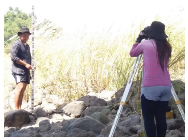
Figure 40. Bridge cross-section with water level elevation acquisition at Mompong Bridge, Brgy. Sta. Lucia, Municipality of Sablayan
