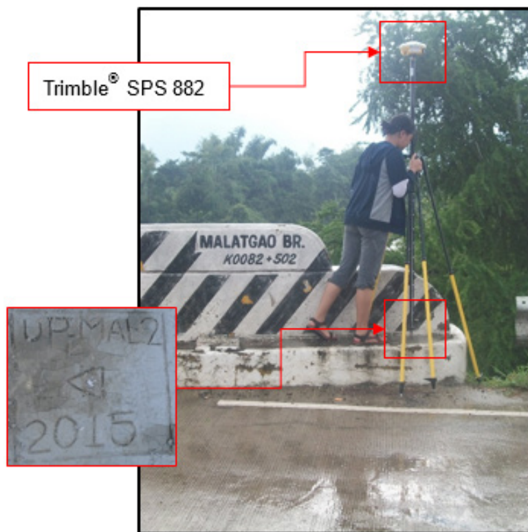
Figure 32. GNSS receiver set up, Trimble® SPS 882, at UP_MAL-2, located at the approach of Malatgao Bridge in Brgy. Tinagong Dagat, Narra, Province of Palawan
