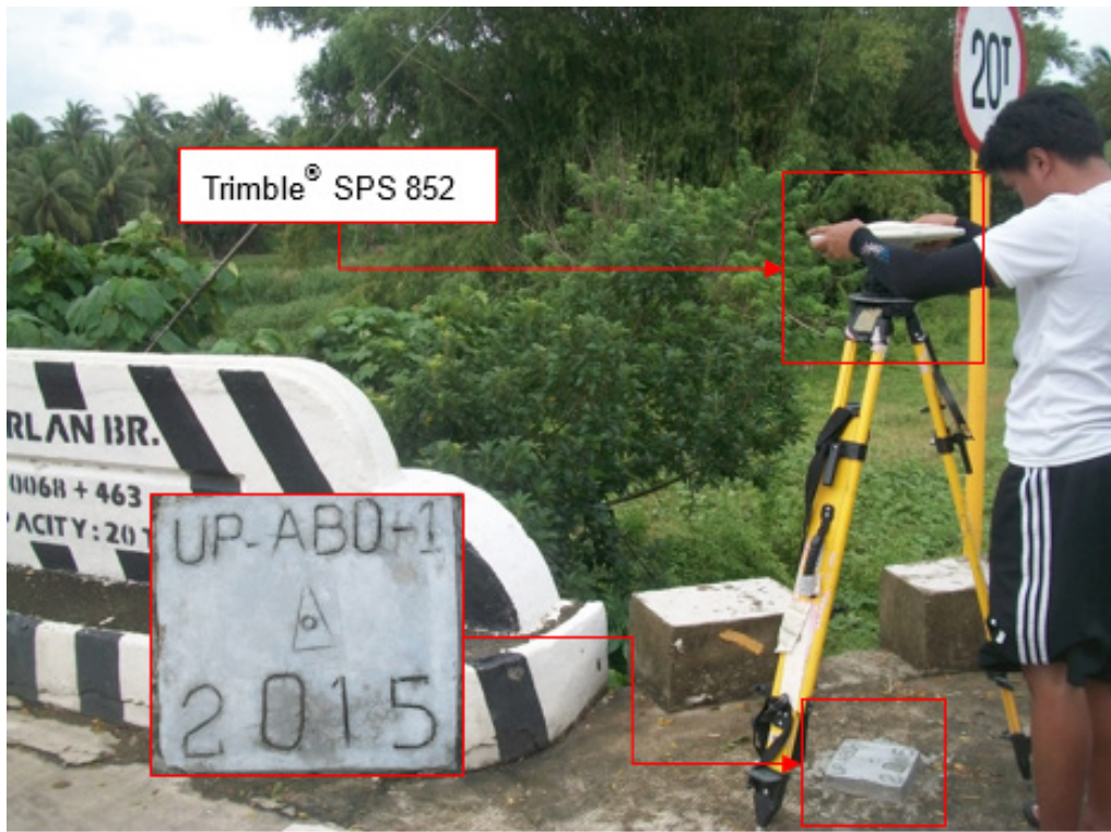
Figure 34. GNSS receiver set-up, Trimble® SPS 852, at UP_ABO-1, an established control point, beside the approach of Aborlan Bridge in Brgy. Gogognan, Aborlan, Palawan
