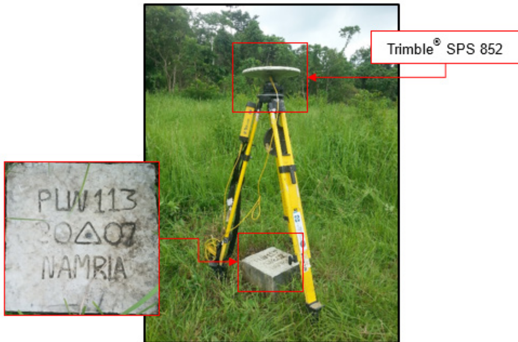
Figure 30. GNSS base set up, Trimble® SPS 852, at PLW-113, located southwest of Aborlan Water System in Brgy. Dumagueña, Narra, Province of Palawan
