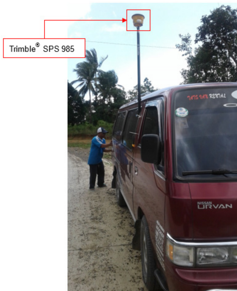
Figure 42. Validation points acquisition survey set-up for Iwahig Penal River
