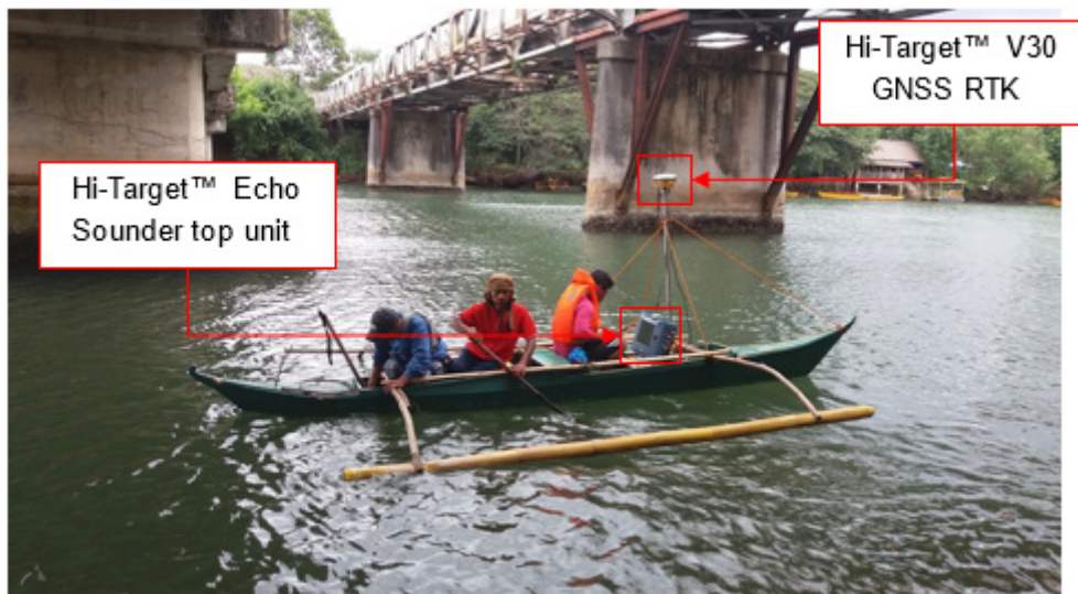
Figure 44. Bathymetric survey of ABSD at Iwahig Penal River using Hi-Target™ Echo Sounder
