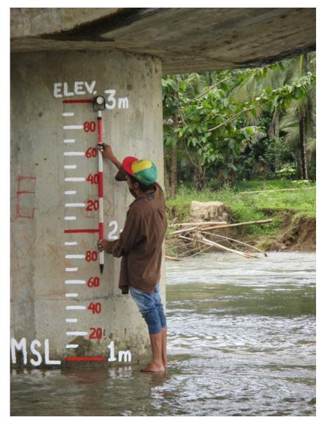
Figure 40. Water-level markings on Iraan Bridge
