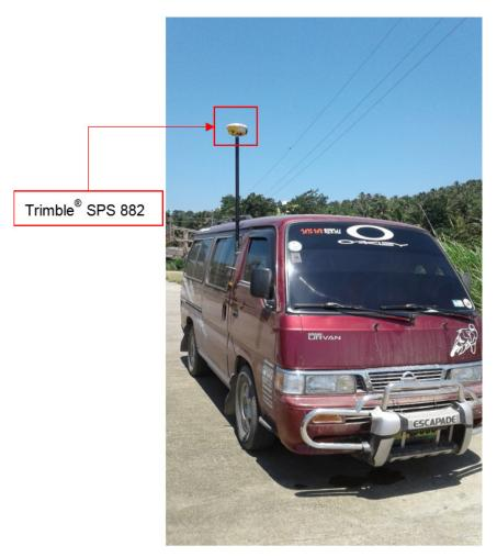
Figure 41. Validation points acquisition survey set up along Iraan River
