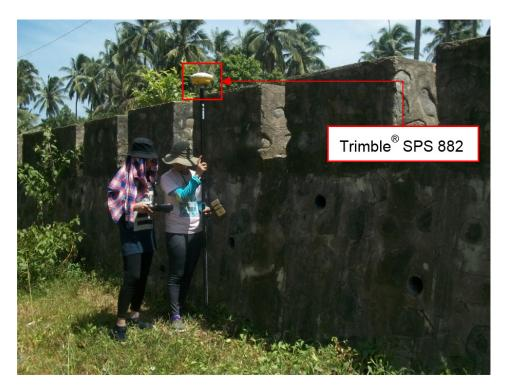
Figure 36. Gathering of random cross-section points along the approach of Iraan Bridge
