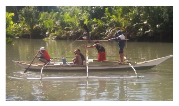
Figure 44. Manual Bathymetric survey using a Trimble® SPS 985 in GNSS PPK survey technique in Caramay River
