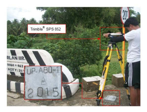
Figure 34. GNSS receiver set-up, Trimble® SPS 852, at UP\_ABO-1, an established control point, beside the approach of Aborlan Bridge in Brgy. Gogognan, Aborlan, Palawan
