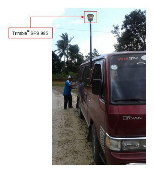
Figure 42. Validation Points Acquisition Set-up for Inagauan River
