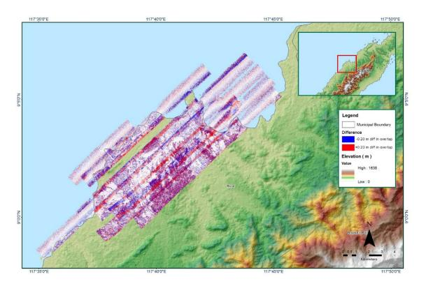
Figure A-8.14 Elevation difference between flight lines
