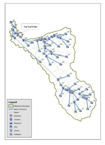
Figure 56 The Ilog-Ilog river basin model generated using HEC-HMS.
