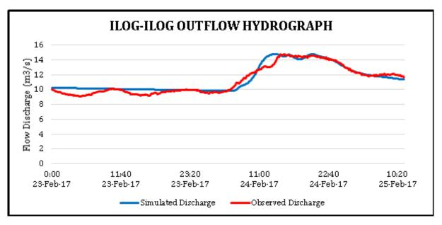
Figure 59 Outflow Hydrograph of Ilog-Ilog produced by the HEC-HMS model compared with observed outflow.
