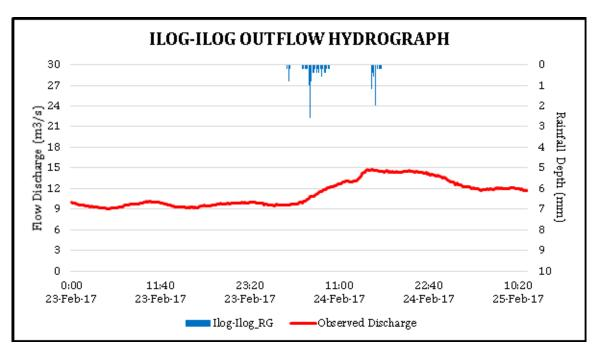
Figure 49. Rainfall and outflow data at Ilog-Ilog used for modeling.
