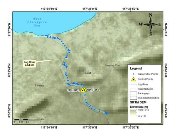
Figure 43. Bathymetric survey of Ilog-Ilog River.
