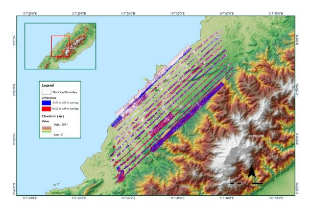
Figure A-8.21 Elevation difference between flight lines
