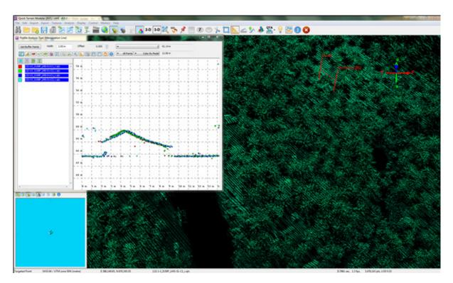
Figure 13 Quality checking for an Ilog-Ilog flight 3159P using the Profile Tool of QT Modeler.
