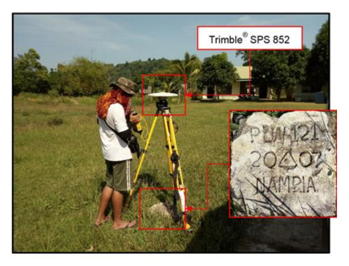
Figure 27. GNSS base set-up, Trimble® SPS 852, at PLW-121, located along the basketball court inside Cabcungan Elementary School in Brgy. Ransang, Rizal, Province of Palawan.
