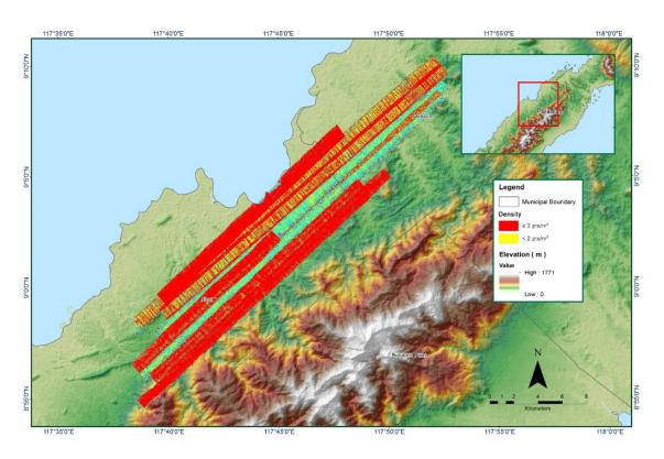
Figure A-8.6 Density map of merged LiDAR data
