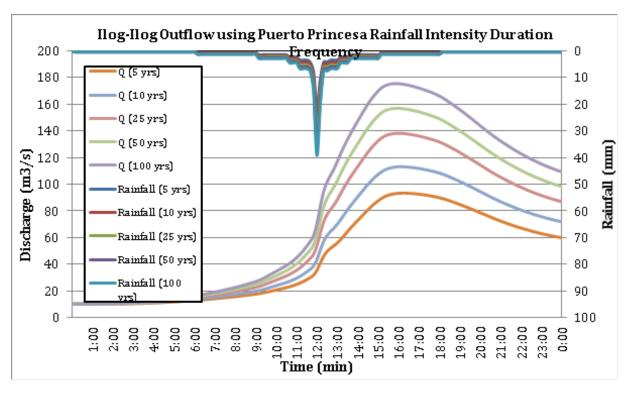
Figure 60 Outflow hydrograph at Ilog-Ilog Station generated using Puerto Princesa RIDF simulated in HEC-HMS.
