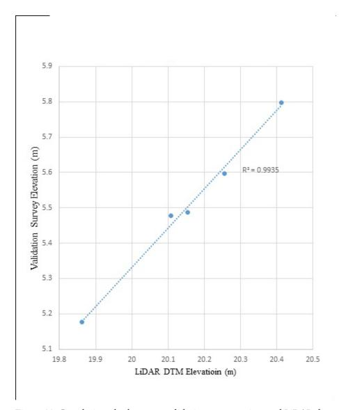
Figure 23. Correlation plot between validation survey points and LiDAR data.
