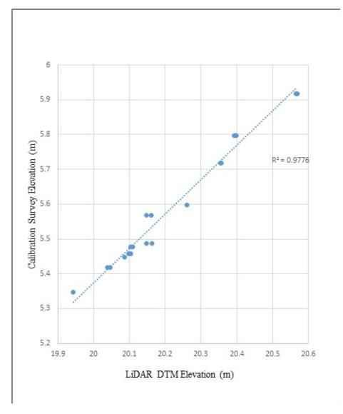
Figure 22 Correlation plot between calibration survey points and LiDAR data.
