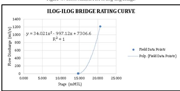
Figure 48 Rating Curve at Ilog-Ilog Bridge, Rizal, Palawan.
