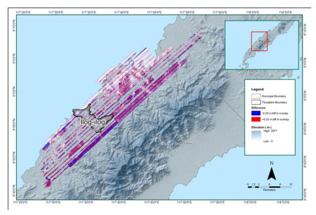
Figure 12 Elevation difference map between flight lines for Ilog-Ilog Floodplain.
