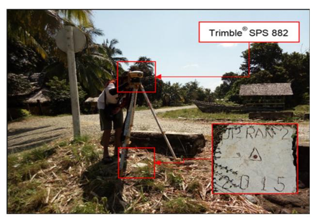
Figure 29. GNSS receiver set-up, Trimble® SPS 882, at UP\_ILO-1, located at the side of the railings near Ilog-Ilog Bridge in Brgy. Campong Ulay, Rizal, Province of Palawan.
