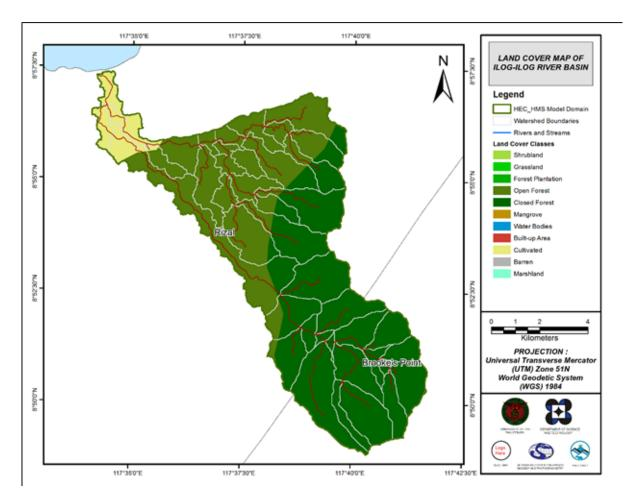
Figure 53 The land cover map of the Ilog-Ilog River Basin used for the estimation of the CN and watershed lag parameters of the rainfall-runoff model. (Source of data: Digital soil map of the Philippines published by the Bureau of Soil and Water Management – Department of Agriculture).
