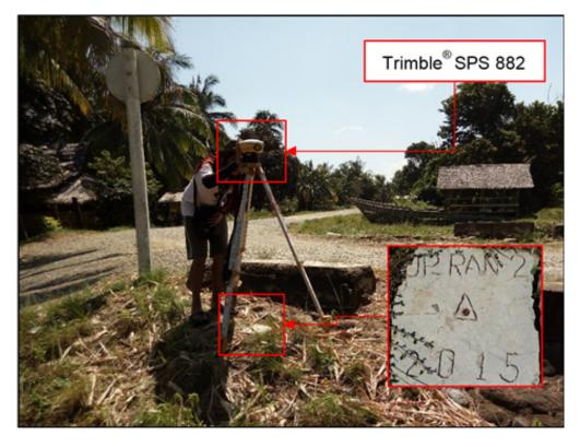
Figure 30. GNSS receiver set-up, Trimble® SPS 882, at UP\_RAN-2, located on a riprap near Ransang Bridge in Brgy. Ransang, Rizal, Province of Palawan.
