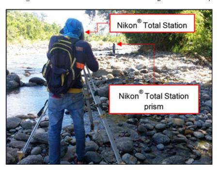
Figure 41. Manual bathymetric survey of ABSD along Ilog-Ilog River using a Nikon® Total Station.
