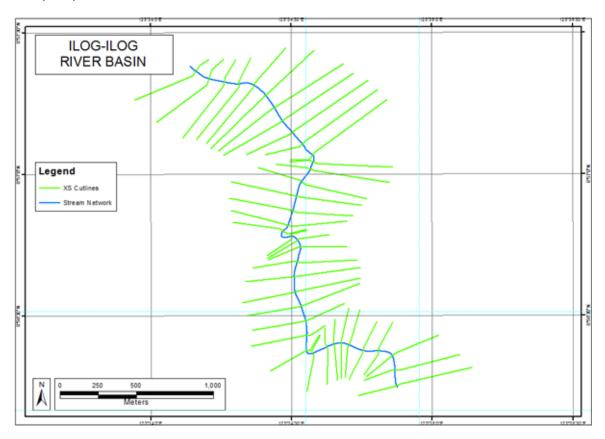
Figure 57 River cross-section of Ilog-Ilog River generated through Arcmap HEC GeoRAS tool.
