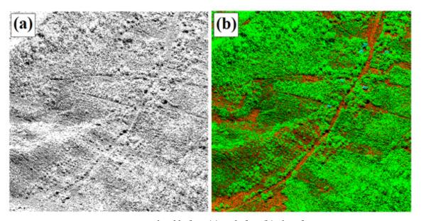
Figure 15 Point cloud before (a) and after (b) classification.
