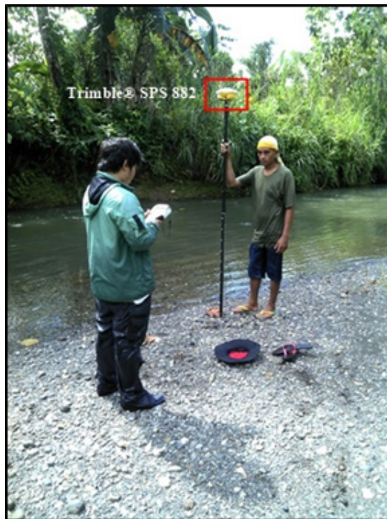
Figure 40. Cross-section and bridge as-built survey for Subaan Bridge, Brgy Subaan, Oriental Mindoro
