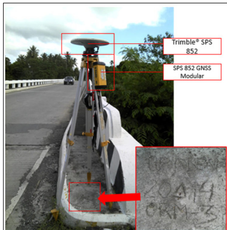
Figure 37. Trimble® SPS 985 setup at ORM-3 located at the approach of Balete Bridge, Brgy. Balete, Municipality of Gloria, Oriental Mindoro
