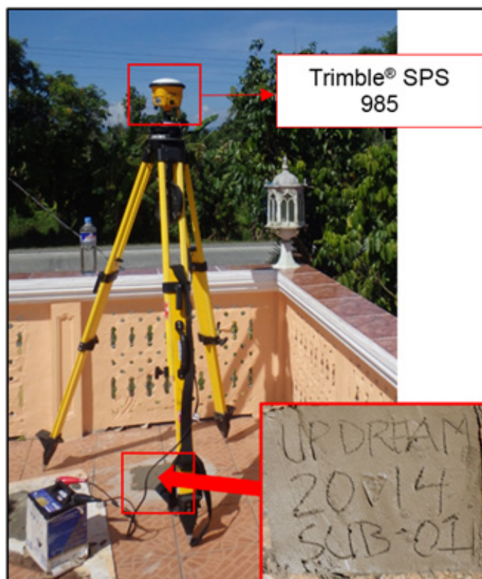
Figure 39. GPS setup of Trimble® SPS 985 at SUB-1, an established control point located at Maramot Residence in Brgy. Subaan, Municipality of Socorro, Oriental Mindoro
