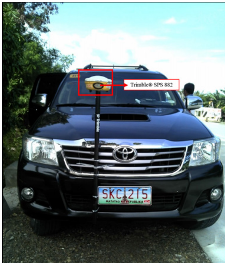
Figure 45. Trimble® SPS 882 setup for validation points acquisition survey for Butas River Basin
