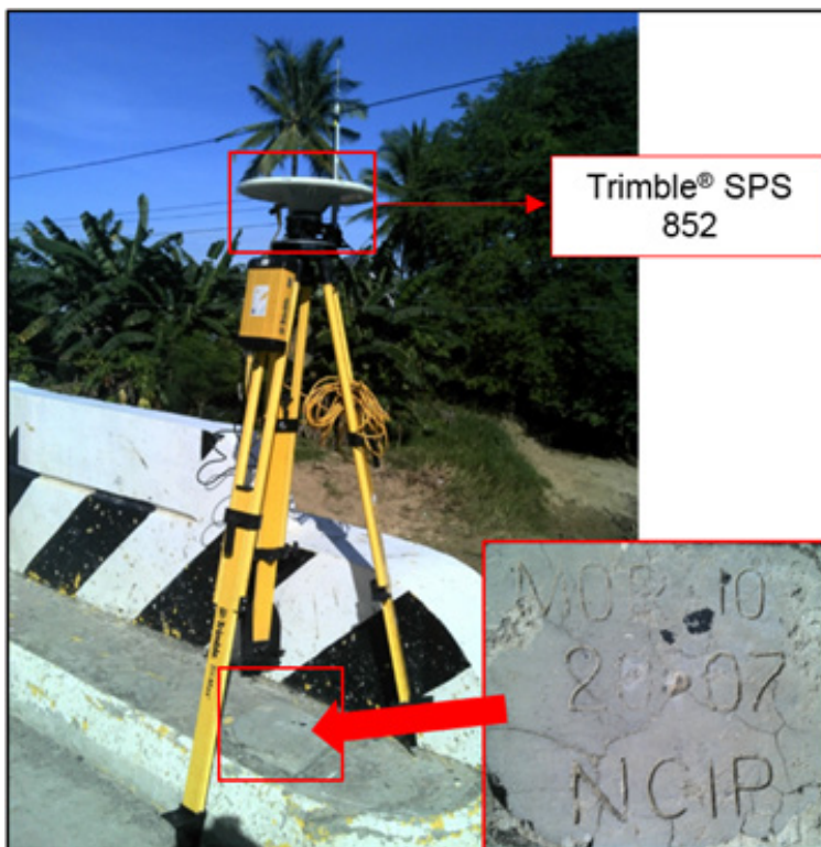
Figure 35. GPS setup of Trimble® SPS 852 at MOR-10, located in the approach of the Cawacat Bridge, in Brgy. Campasaan, Municipality of Bulalacao, Oriental Mindoro
