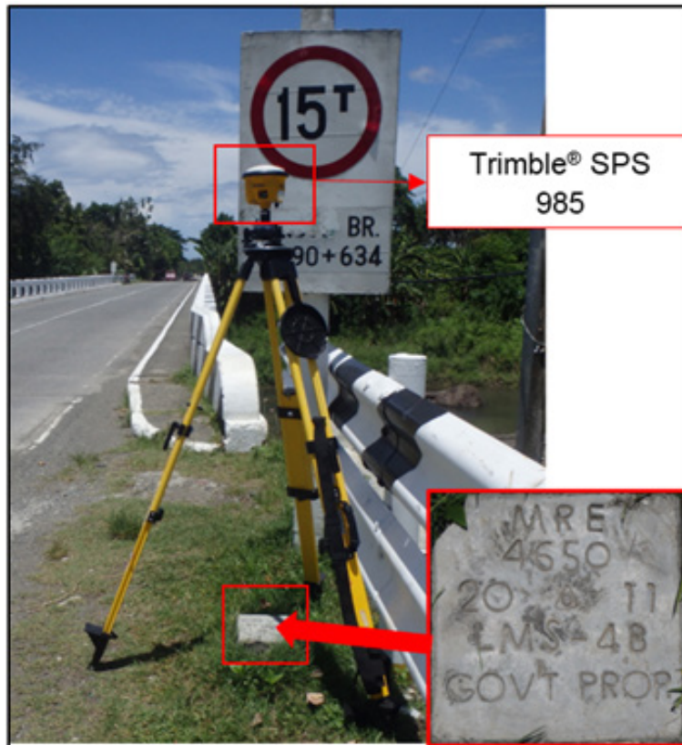
Figure 32. The GPS setup of Trimble® SPS 985 at MRE-4650, an LMS control point located at the approach of Bansud Bridge, in Brgy. Pagasa, Municipality of Bansud, Oriental Mindoro
