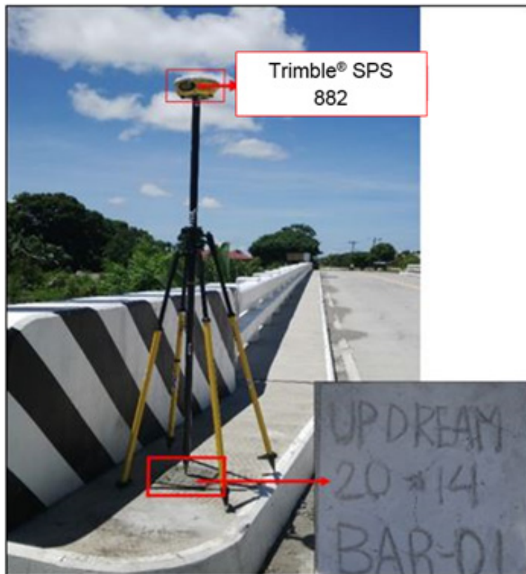
Figure 33. GPS setup of Trimble® SPS 882 at BAR-1, an established control point located in Baroc Bridge, Brgy. San Isidro, Mansalay, Oriental Mindoro
