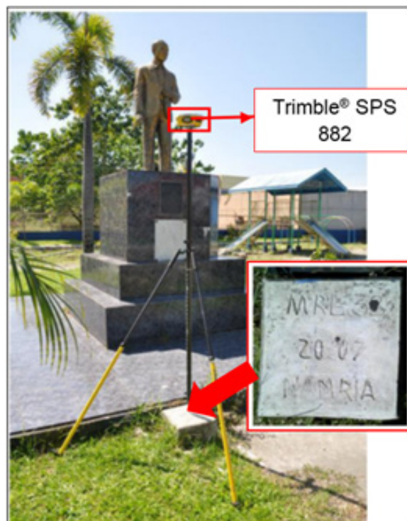
Figure 31. GPS setup of Trimble® SPS 882 at MRE-32, located at the Municipal Park of Victoria, in Brgy. Poblacion 1, Oriental Mindoro
