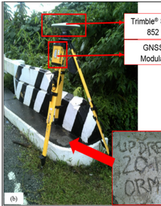
Figure 36. GPS setup of Trimble® SPS 852 at ORM-1, located on Subaan Bridge, Brgy. Subaan, Municipality of Socorro, Oriental Mindoro
