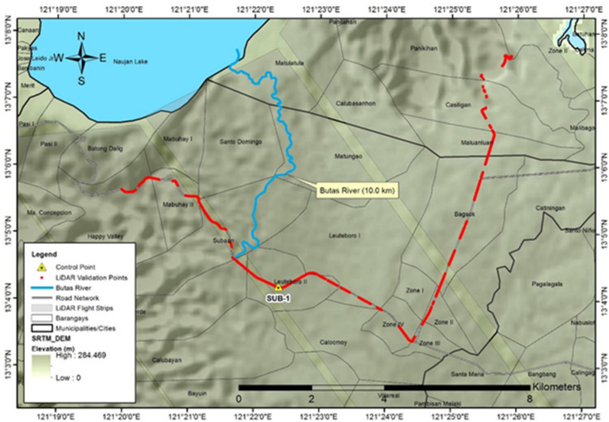
Figure 46. Validation points acquisition survey along Butas River Basin
