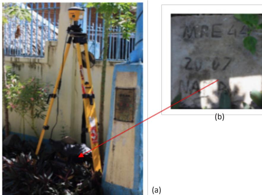
Figure 4. GPS set-up over MRE-44 as recovered just outside the compound of the barangay hall of Happy Valley, municipality of Roxas, Oriental Mindoro (a) and NAMRIA reference point MRE-44 (b) as recovered by the field team.
