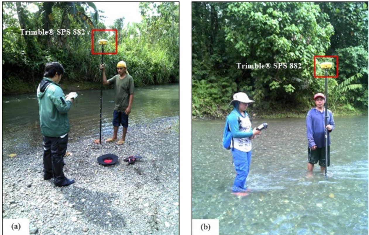
Figure 47. Bathymetric survey in Butas River: (a) upstream and (b) downstream
