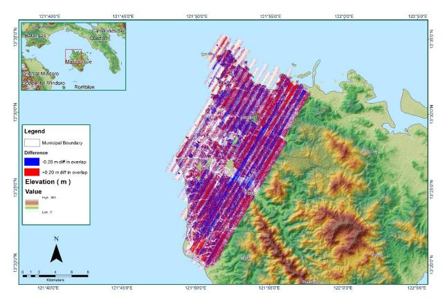
Figure A-8.7 Elevation difference between flight lines
