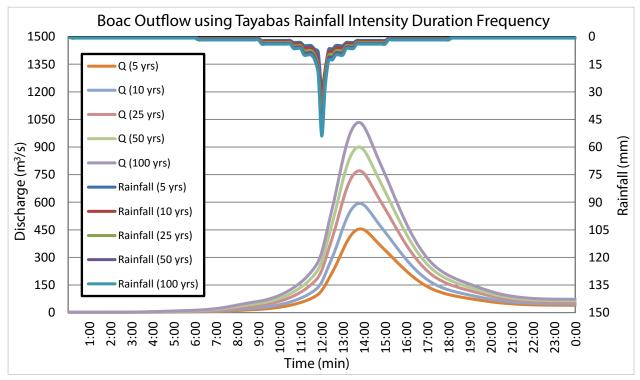
Figure 56. Outflow hydrograph at the Boac Station generated using the Tayabas RIDF, simulated in HEC-HMS
