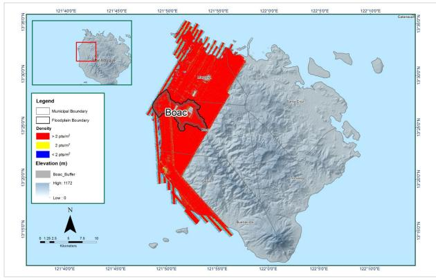
Figure 11. Pulse density map of merged LiDAR data for Boac Floodplain.
