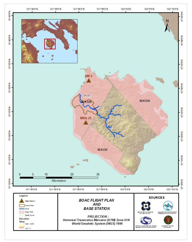
Figure 2. Flight plans and base stations used to cover the Boac floodplain survey
