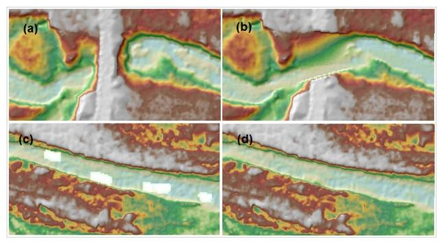
Figure 19. Portions in the DTM of the Boac Floodplain – a bridge (a) before and (b) after manual editing; and a data gap (c) before and (d) after data retrieval
