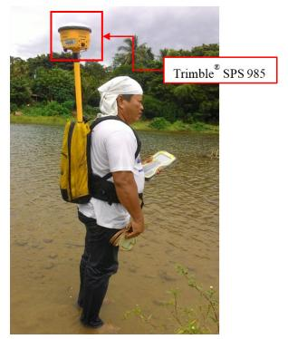
Figure 39. Bathymetric survey using Trimble® SPS 985 in GNSS PPK survey technique in the Boac River
