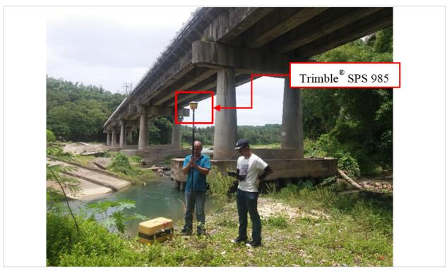
Figure 31. Bridge as-built survey, using PPK Technique
