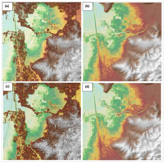
Figure 16. The production of last return DSM (a) and DTM (b), first return DSM (c) and secondary DTM (d) in some portion of Boac Floodplain.
