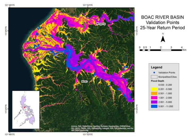
Figure 70. Validation points for a 25-year flood depth map of the Boac Floodplain
