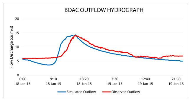
Figure 55. Outflow Hydrograph of Boac produced by the HEC-HMS model compared with observed outflow
