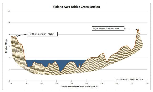
Figure 43. Cross-section plot of the Biglang Awa Bridge
