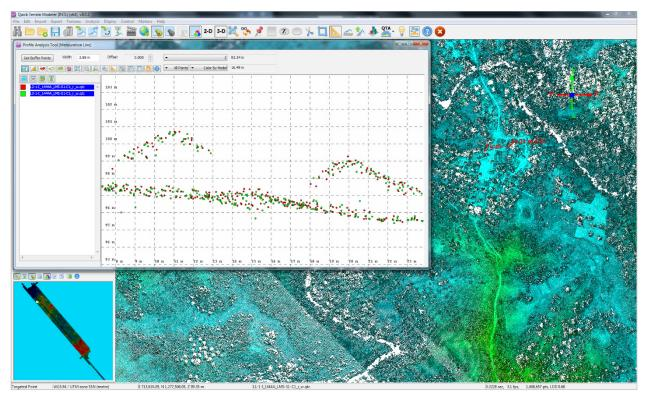
Figure 13. Quality checking for a Boac flight 7401GC using the Profile Tool of QT Modeler.
