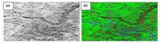
Figure 15. Point cloud before (a) and after (b) classification.
