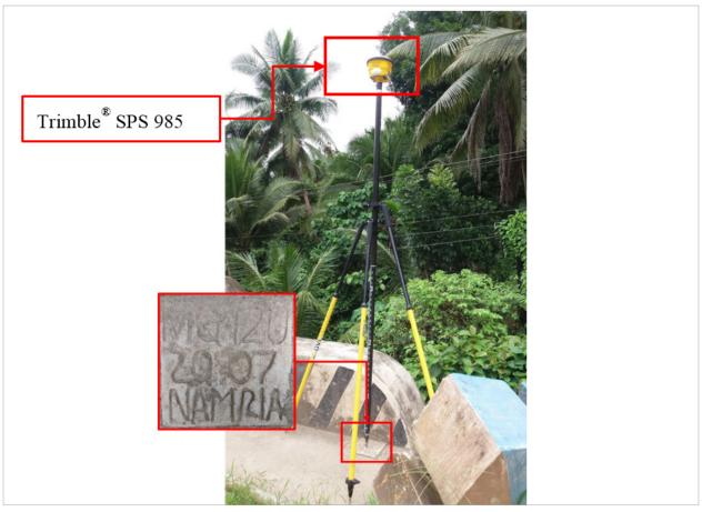
Figure 29. GNSS receiver set-up, Trimble® SPS 985 at MQ-120, located at the approach of the Mangamnan Bridge in Barangay Butansapa, Mogpong, Marinduque
