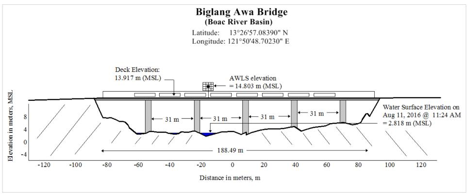
Figure 33. Biglang Awa Bridge cross-section diagram
