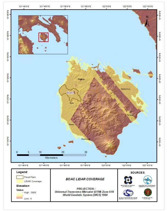
Figure 4. Actual LiDAR survey coverage for Boac Floodplain.
