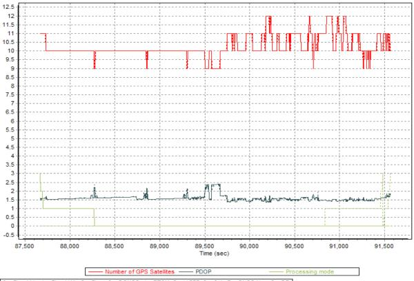
0 = Fixed NL, 1 = Fixed WL, 2 = Float, 3 = DGNSS, 4 = RTCM, 5 = IAPPP, 6 = C/A, 7 = GNSS Nav, 8 = DR
