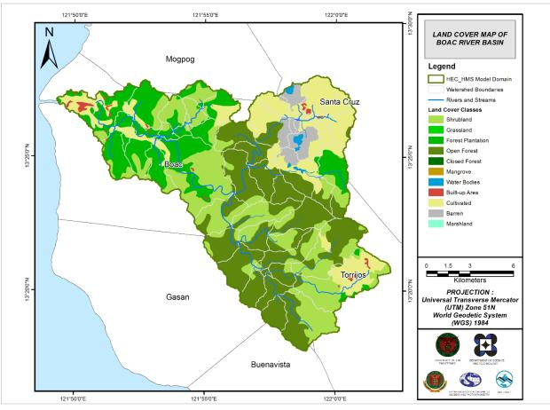
Figure 49. Land cover map of the Boac River Basin, used for the estimation of the CN and watershed lag parameters of the rainfall-runoff model (Source: NAMRIA)
