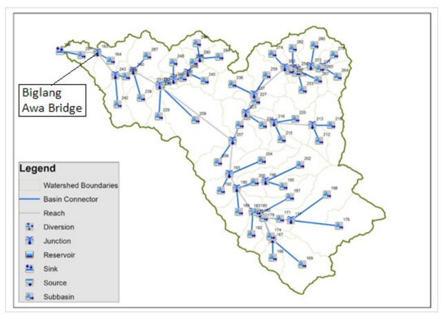
Figure 52. The Boac River Basin model generated using HEC-HMS
