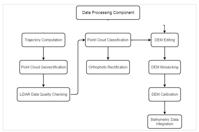
Figure 5. Schematic diagram for the Data Pre-Processing Component
