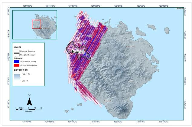
Figure 12. Elevation difference map between flight lines for Boac Floodplain.
