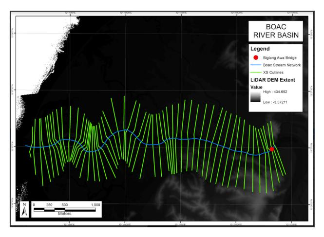
Figure 53. River cross-section of the Boac River, generated through the ArcMap HEC GeoRAS tool
