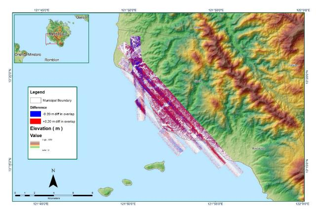
Figure A-8.14 Elevation difference between flight lines
