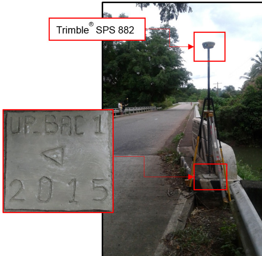
Figure 32. GNSS receiver set up, Trimble® SPS 985, at UP_BAC -1, located at the approach of Bacungan Bridge in Brgy. Bacungan, Quezon, Province of Palawan
