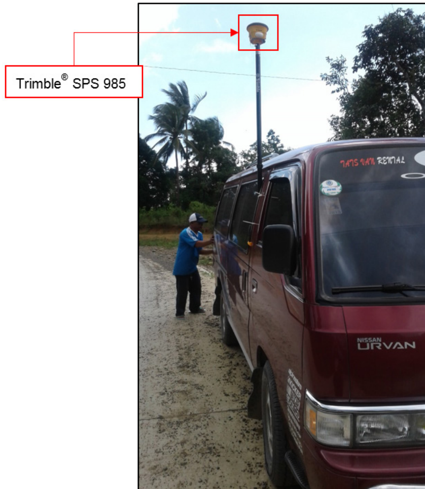
Figure 40. Validation points acquisition survey set-up for Bacungan River
