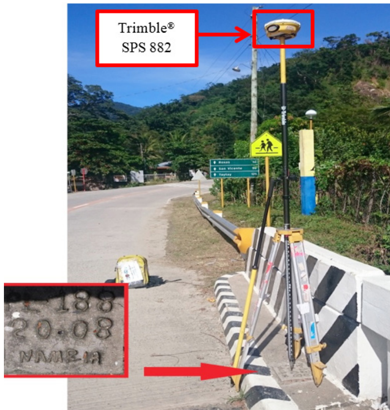
Figure 33. Trimble® SPS 882 GNSS receiver setup at PL-188 located in Langogan Bridge, Brgy. Langogan, Puerto Prinsesa, Palawan
