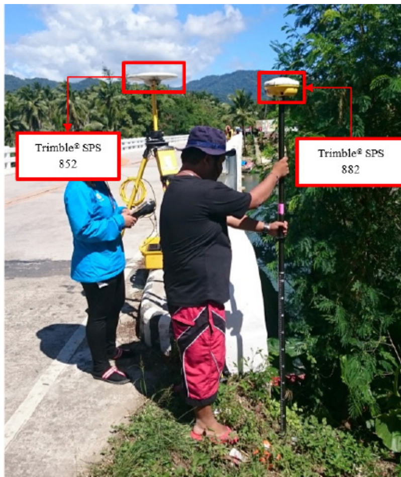
Figure 35. Cross-Section Survey in Babuyan Bridge
