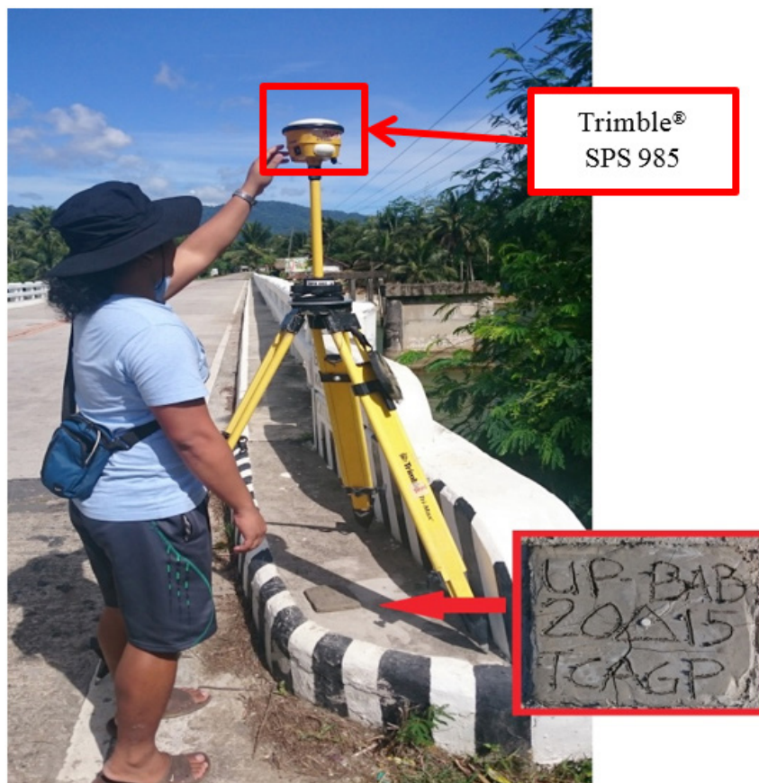
Figure 34. Trimble® SPS 852 GNSS receiver setup at UP-BAB in Babuyan Bridge, Brgy. Maoyon, Puerto Prinsesa, Palawan
