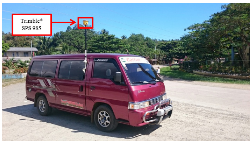
Figure 40. Validation points acquisition survey set-up for Babuyan River
