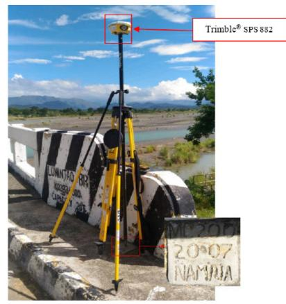
Figure 34. The GNSS (Trimble® SPS 882) receiver occupation, at MC-200 30 located at the approach of Lumintao Bridge in Brgy. Magsikap, Municipality of Rizal, Occidental Mindoro
