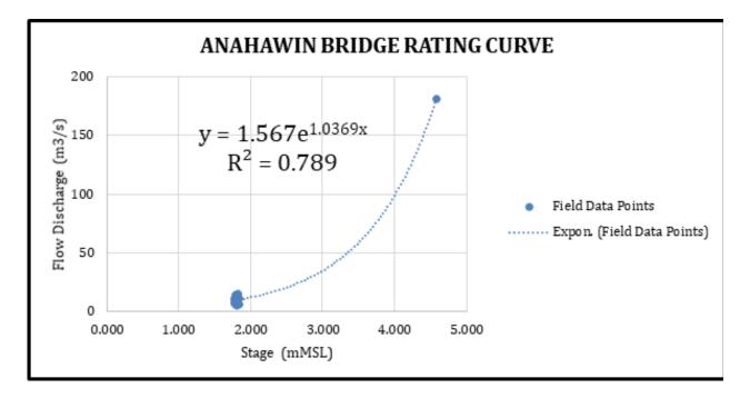
Figure 52. The rating curve of the Anahawin Bridge in Anahawin, Occidental Mindoro.
