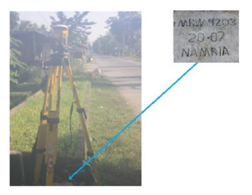
Figure 7. GPS set-up over MRW-4203 in front of the barangay hall of Brgy. Mapaya, municipality of San Jose, Occidental Mindoro (a) and NAMRIA reference point MRW-4203 (b) as recovered by the field team.
