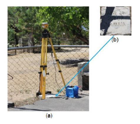
Figure 5. GPS set-up over MRW-24 in the basketball court in Brgy. Iriron, municipality of Calintaan, Occidental Mindoro (a) and NAMRIA reference point MRW-24 (b) as recovered by the field team.
