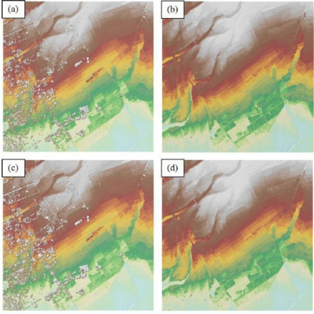
Figure 21. Photo (A) features the production of the last return DSM; (B) depicts the production of the DTM; (C) portrays the production of the first return DSM; and (D) presents the generation of the secondary DTM in some portions of the Anahawin Floodplain.
