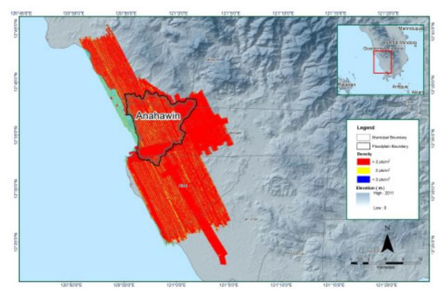
Figure 16. Pulse density map of the merged LiDAR data for the Anahawin Floodplain Survey.
