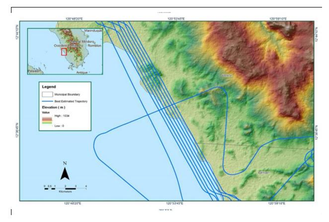
Figure A-8.17. Best estimated trajectory of LiDAR missions conducted over the Anahawin Floodplain.
