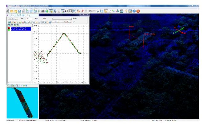
Figure 18. Screen-capture of the quality checking for Anahawin Flight 1156A using the Profile Tool of QT Modeler.
