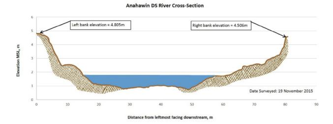
Figure 51. The cross-section plot of the Anahawin Bridge
