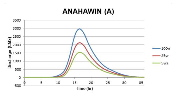
Figure 65. Anahawin river (A) generated discharge using 5-, 25-, and 100-year Romblon rainfall intensity-duration-frequency (RIDF) in HEC-HMS
