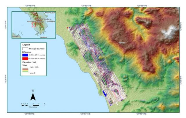
Figure A-8.14. Elevation difference between flight lines
