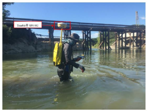
Figure 41. The Cross-section survey conducted at the downstream side of Anahawin Bridge, Brgy.Poblacion, Municipality of Calintaan
