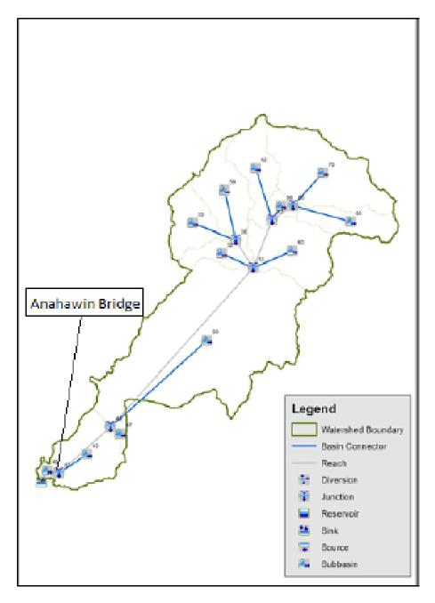
Figure 60. The Anahawin river basin model generated using HEC-HMS
