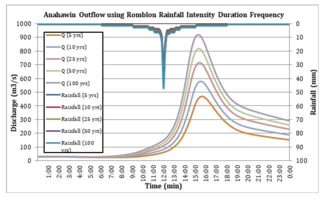
Figure 64. The Outflow hydrograph at the Anahawin Station, generated using the Romblon RIDF simulated in HEC-HMS
