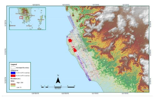
Figure A-8.7. Elevation difference between flight lines
