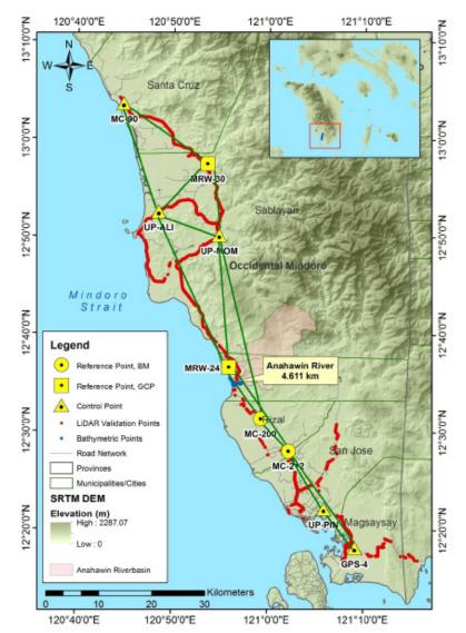
Figure 30. Extent of the bathymetric survey (in blue line) in Anahawin River and the LiDAR data validation survey (red).
