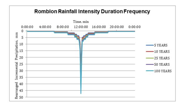
Figure 55. The synthetic storm generated for a 24-hour period rainfall for various return periods
