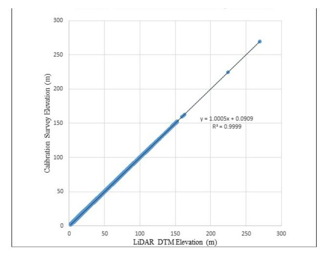
Figure 27. The correlation plot between calibration survey points and LiDAR data.
