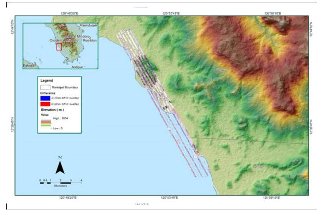
Figure A-8.21. Elevation difference between flight lines
