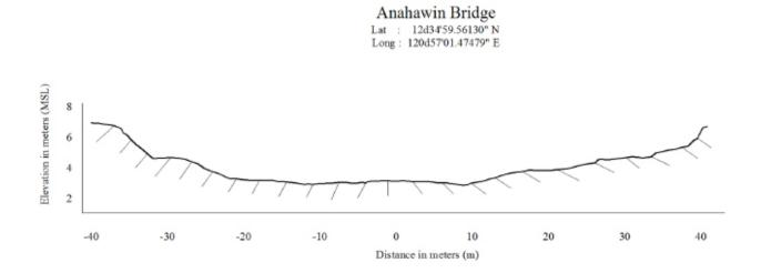
Figure 44. The downstream side of the Anahawin Bridge cross-section survey drawn to scale
