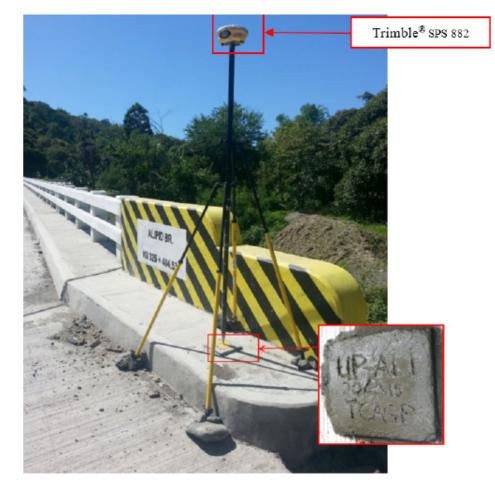
Figure 40. The GNSS receiver occupation, Trimble® SPS 882, at UP-ALI, Alipid Bridge approach in Brgy. Sto. Niño, Municipality of Sablayan, Occidental Mindoro
