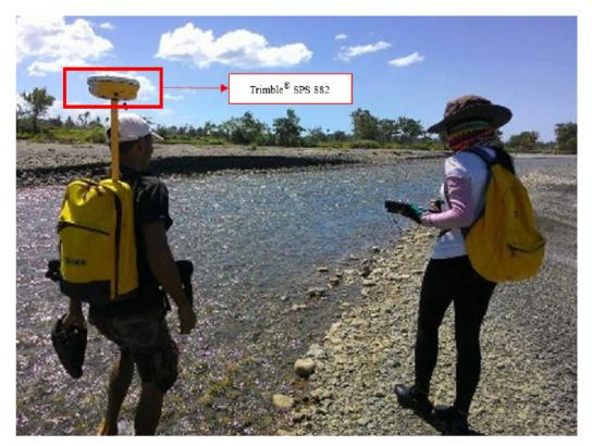
Figure 47. Setup for the manual Bathymetric Survey along Anahawin River
