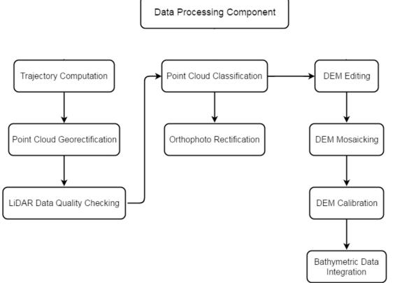
Figure 10. Schematic diagram for Data Pre-processing
