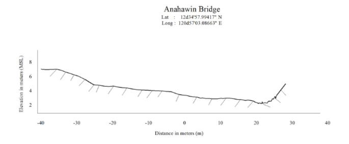
Figure 43. The upstream side of the Anahawin Bridge cross-section survey drawn to scale
