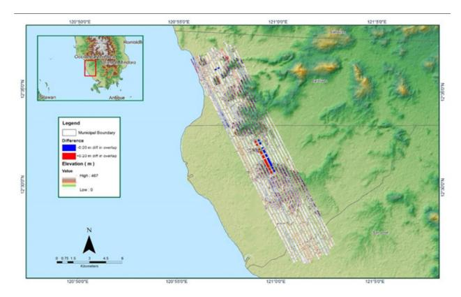
Figure A-8.35. Elevation difference between flight lines
