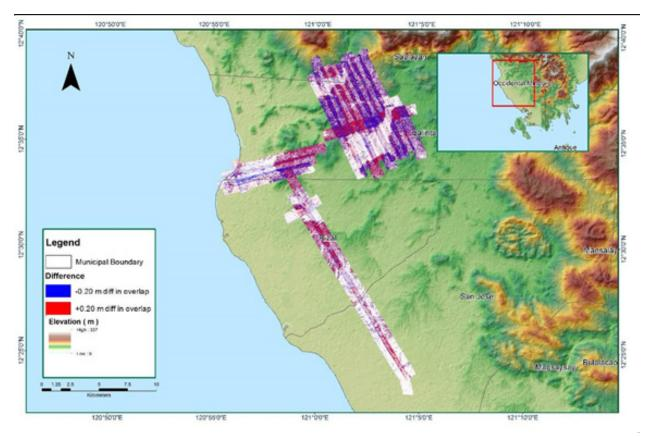
Figure A-8.42. Elevation difference between flight lines
