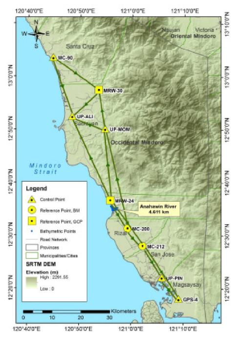
Figure 31. The GNSS Network established in the Anahawin River Survey.
