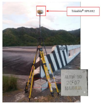
Figure 33. The GNSS (Trimble® SPS 882) receiver setup at MRW- 30 located at the approach of Amnay Bridge in Sitio Kabangkalan, Brgy. Pinagturilan, Municipality of Santa Cruz, Occidental Mindoro
