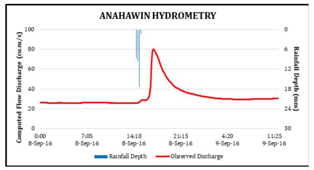
Figure 53. Rainfall and outflow data of the Anahawin River Basin, which was used for modeling.
