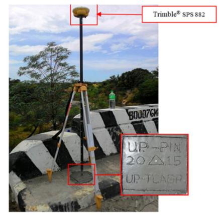
Figure 38. The GNSS receiver occupation, Trimble® SPS 882, at UP-PIN Pinamanaan Bridge approach in Brgy. Mapaya, Municipality of San Jose, Occidental Mindoro
