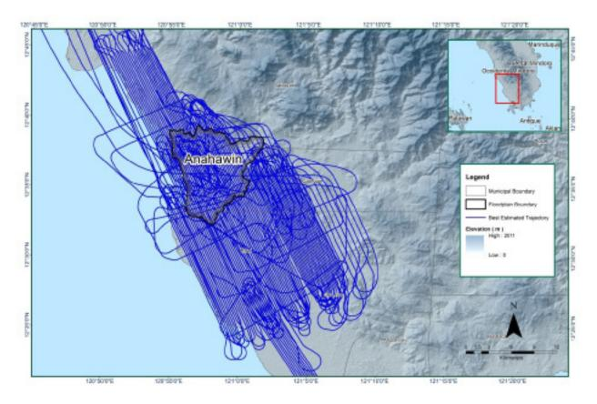
Figure 13. The Best Estimated Trajectory of LiDAR missions conducted over the Anahawin Floodplain.
