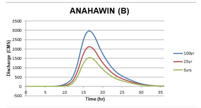
Figure 66. Anahawin river (B) generated discharge using 5-, 25-, and 100-year Romblon rainfall intensity-duration-frequency (RIDF) in HEC-HMS
