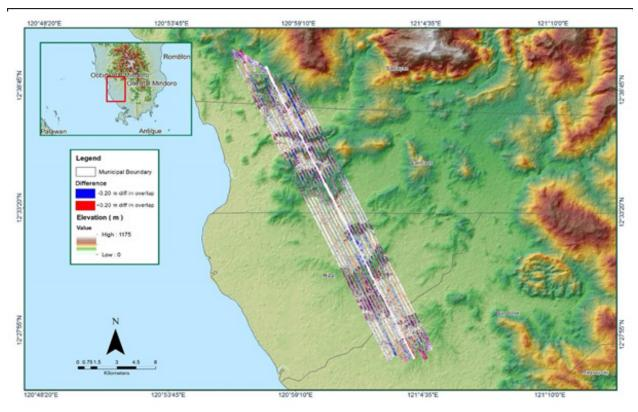
Figure A-8.28. Elevation difference between flight lines
