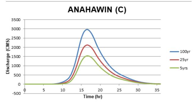
Figure 67. Anahawin river (B) generated discharge using 5-, 25-, and 100-year Romblon rainfall intensity-duration-frequency (RIDF) in HEC-HMS
