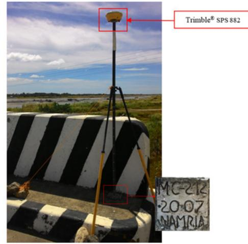
Figure 35. The GNSS (Trimble® SPS 852) base occupation at MC-212, located at the approach of Busuanga Bridge in Bgry. Sto Niño, Municipality of Rizal, Occidental Mindoro
