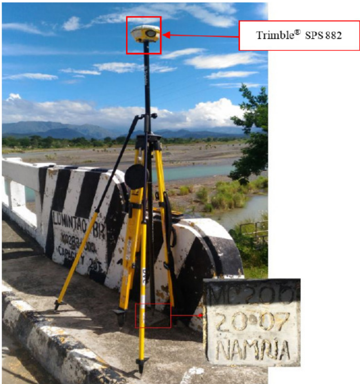
Figure 33. GNSS receiver set-up, Trimble® SPS 882, at MC-200, Lumintao Bridge approach in Brgy. Magsikap, Municipality of Rizal, Occidental Mindoro
