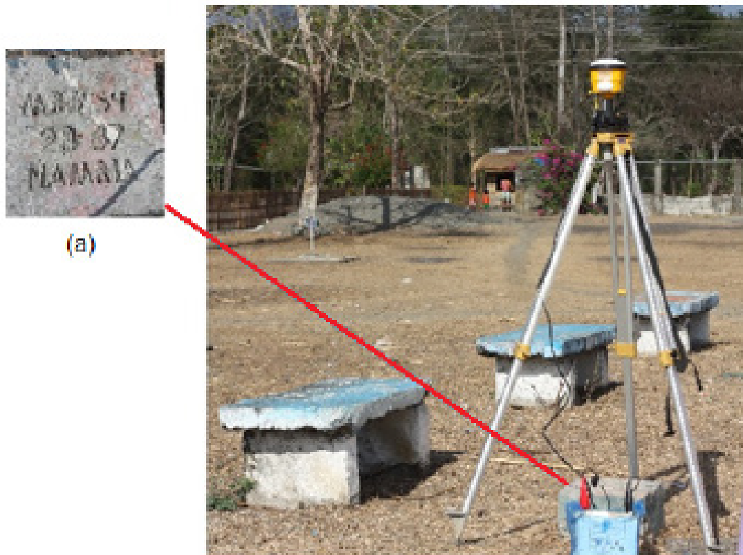
Figure 7. NAMRIA reference point MRW-54 (a) as recovered by the field team and GPS set-up over MRW-54 as recovered in near basketball open court in Brgy. Malisbong, municipality of Sablayan, Occidental Mindoro (b).
