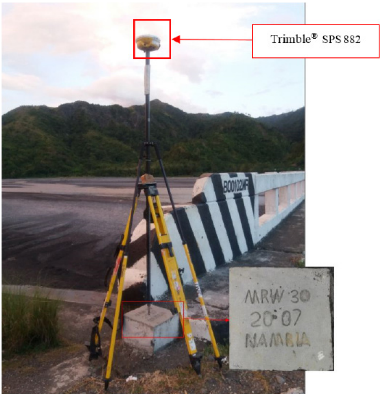
Figure 32. GNSS receiver setup, Trimble® SPS 882, at MRW- 30 Amnay Bridge approach in Sitio Kabangkalan, Brgy. Pinagturilan, Municipality of Santa Cruz, Occidental Mindoro
