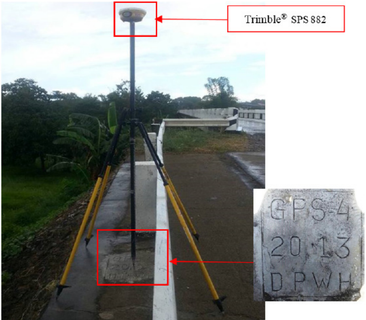
Figure 36. GNSS receiver, Trimble® SPS 882, at GPS-4 on right side of the road abutment after Caguray Bridge going to Bulalacao in Brgy. Poblacion, Municipality of Magsaysay, Occidental Mindoro
