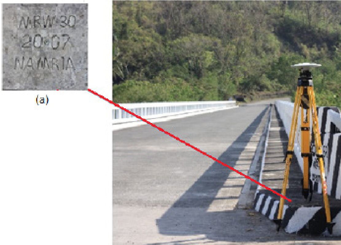
Figure 4. NAMRIA reference point MRW-30 (a) as recovered by the field team and GPS set-up over MRW-30 as recovered in Amnay Bridge in Brgy. Pinagturilan, municipality of Sta. Cruz, Occidental Mindoro (b).
