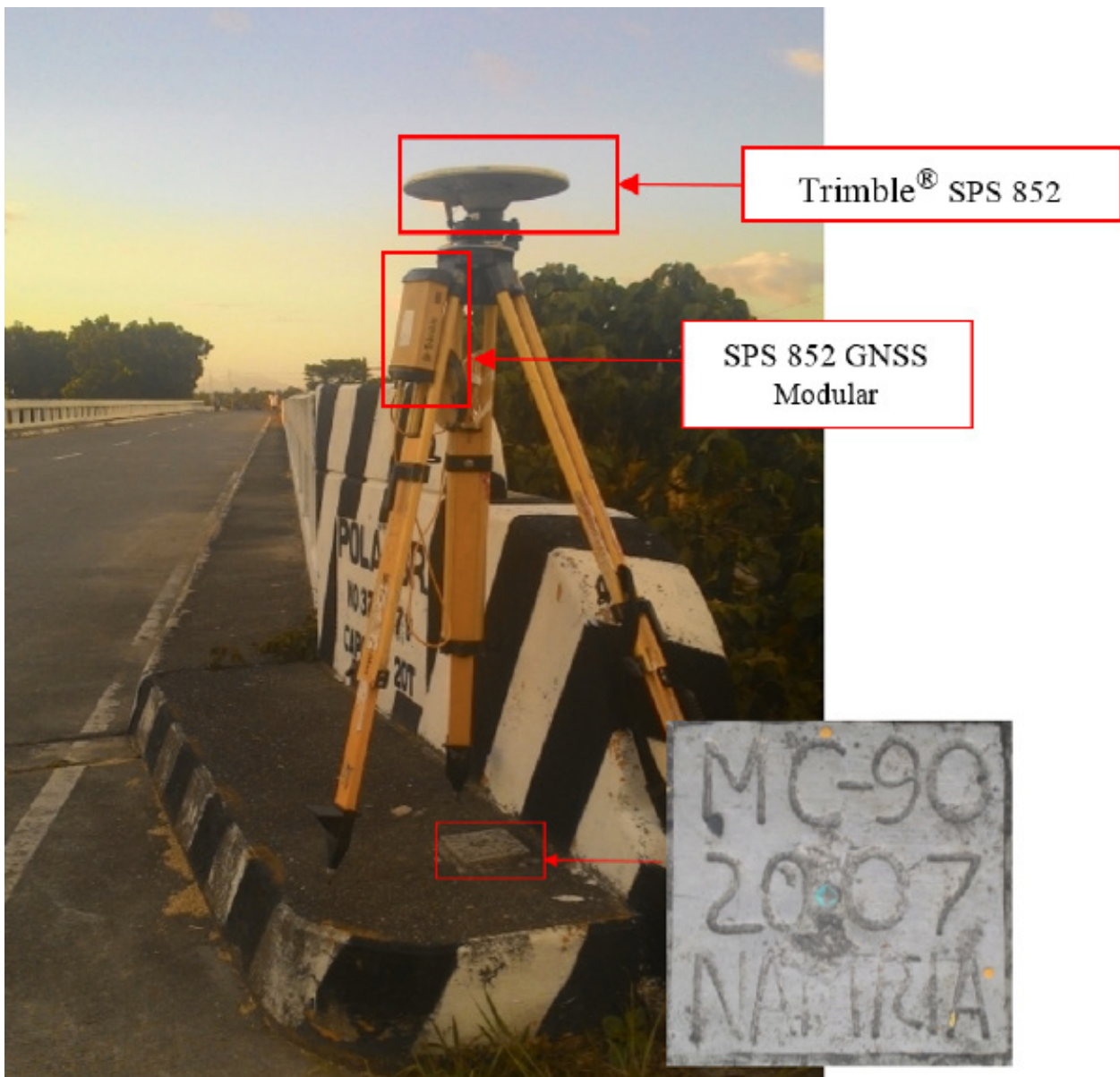
Figure 35. GNSS base, Trimble® SPS 852, at MC-90, used as marker, located at the Pola Bridge approach in Brgy. Barahan, Municipality of Santa Cruz, Occidental Mindoro
