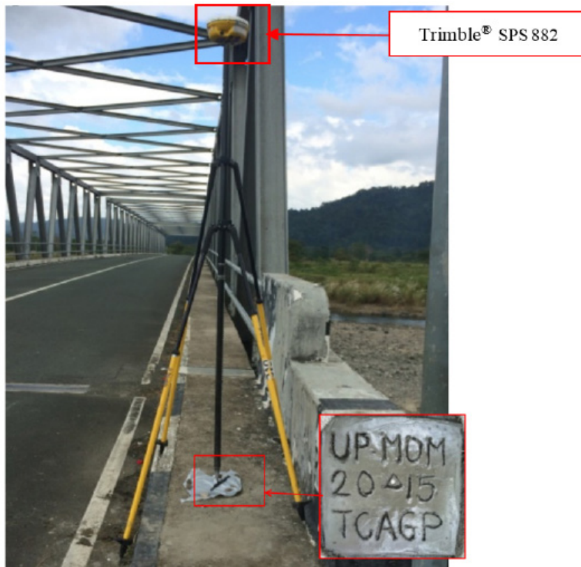
Figure 38. GNSS receiver set-up, Trimble® SPS 882, at UP-MOM, Mompong Bridge approach in Brgy. Lumang Bato, Municipality of Sablayan, Occidental Mindoro
