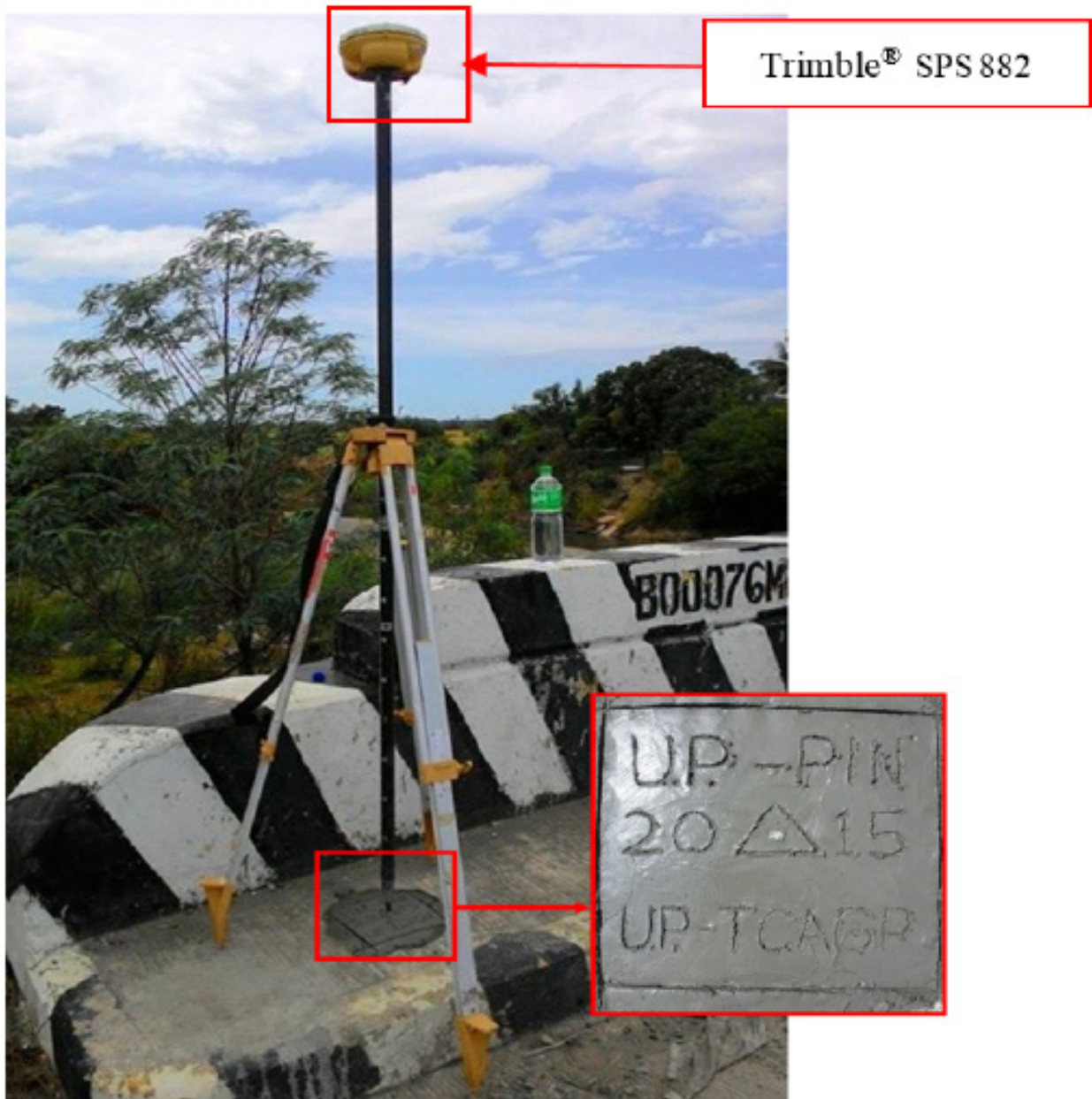
Figure 37. GNSS base receiver set-up, Trimble® SPS 882, at UP-PIN Pinamanaan Bridge approach in Brgy. Mapaya, Municipality of San Jose, Occidental Mindoro
