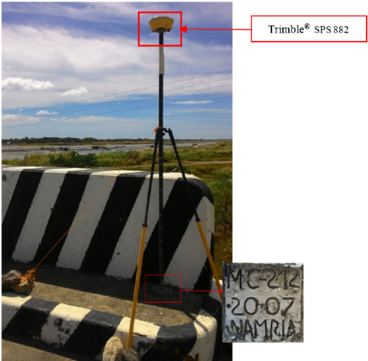
Figure 34. GNSS receiver set-up, Trimble® SPS 882, at MC-212, Busuanga Bridge approach in Bgry. Sto Niño, Municipality of Rizal, Occidental Mindoro
