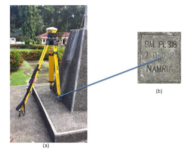
Figure 7. GPS set-up over PL-318 as recovered inside Aborlan Municipal Hall, Aborlan Palawan, (a) NAMRIA reference point PL-318 (b) as recovered by the field team.
