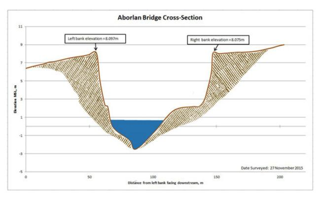
Figure 54. Cross-section plot of Aborlan Bridge.
