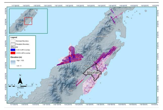
Figure 16. Elevation difference map between flight lines for Aborlan Floodplain.
