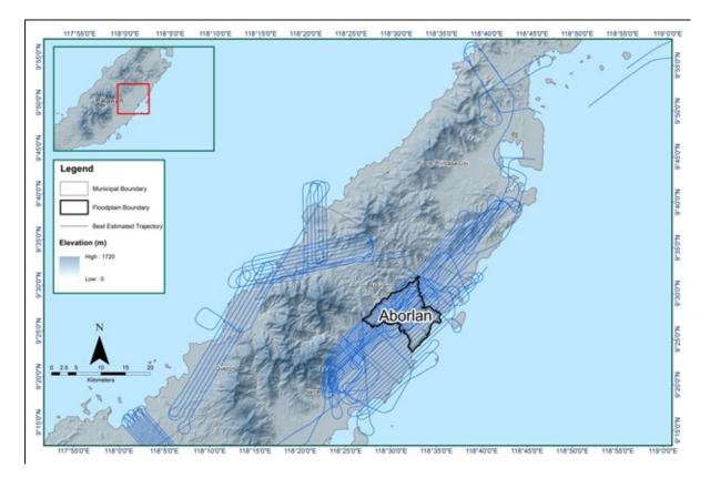
Figure 12. Best estimated trajectory of LiDAR missions conducted over Aborlan Floodplain.
