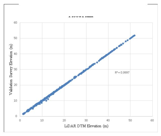
Figure 27. Correlation plot between validation survey points and LiDAR data. Table 20. Validation statistical measures.
