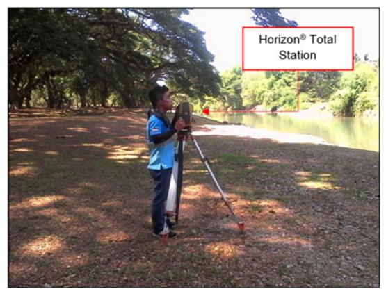
Figure 47. Manual bathymetric survey of ABSD at Aborlan River using Horizon® Total Station.
