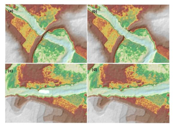
Figure 23. Portions in the DTM of Aborlan Floodplain—a bridge before (a) and after (b) manual editing; and a data gap before (a) and after (b) filling.
