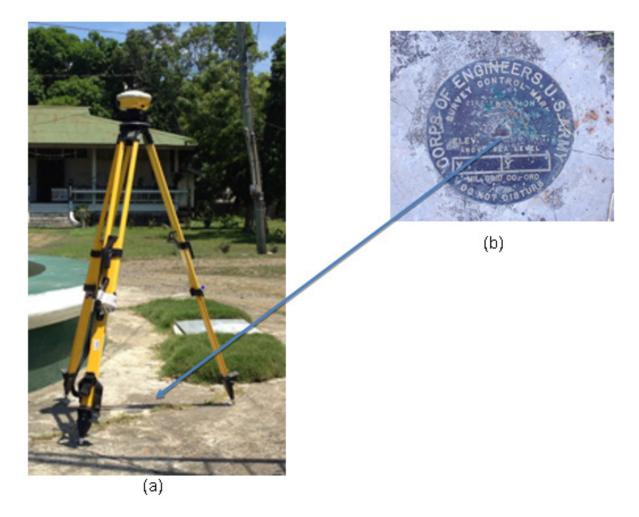
Figure 3. GPS set-up over PLW-50 as recovered at Brgy. Iwahig, Puerto Princesa City (a), NAMRIA reference point PLW-50 (b) as recovered by the field team.
