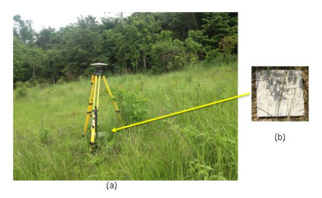
Figure 5. GPS set-up over PLW-113 as recovered in Aborlan Water System in Brgy. Cabigaan, Aborlan, Palawan, (a) NAMRIA reference point PLW-113 (b) as recovered by the field team.
