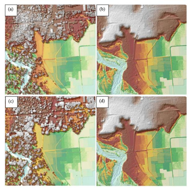
Figure 20. The Production of last return DSM (a) and DTM (b); first return DSM (c) and secondary DTM (d) in some portion of Aborlan Floodplain.
