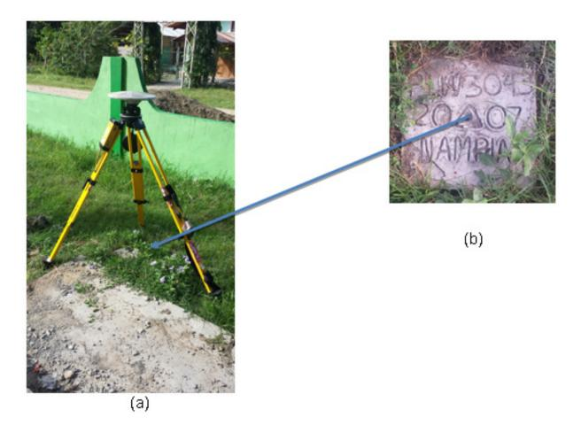
Figure 6. GPS set-up over PLW-3043 as recovered on the ground beside Tigman Barangay Hall, Aborlan, Palawan, (a) NAMRIA reference point PLW-3043 (b) as recovered by the field team.
