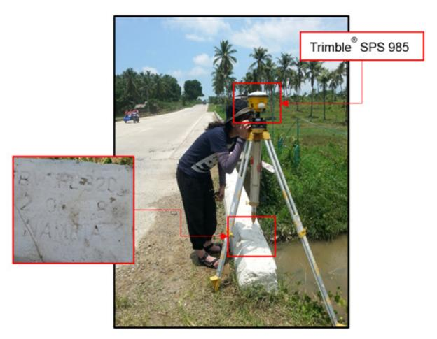
Figure 34. GNSS receiver set=up, Trimble® SPS 985, at PL-320, located on top of a culvert headwall along the National Road in Brgy. Ramon Magsaysay, Aborlan, Province of Palawan.
