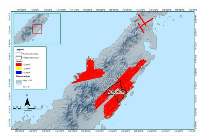
Figure 15. Pulse density map of merged LiDAR data for Aborlan Floodplain.
