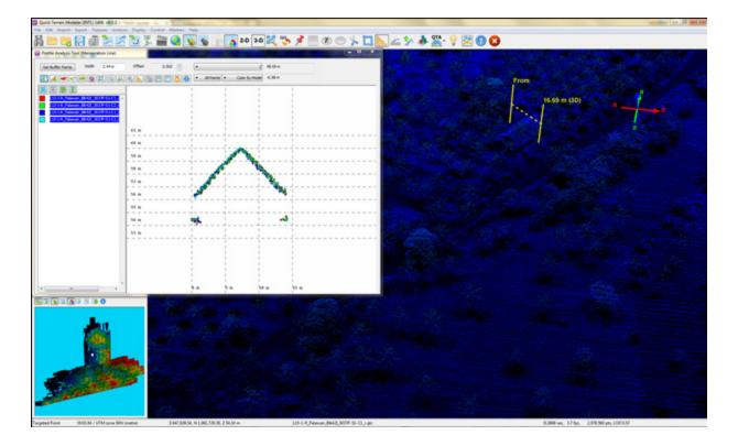
Figure 17. Quality checking for an Aborlan flight 3037P using the Profile Tool of QT Modeler.
