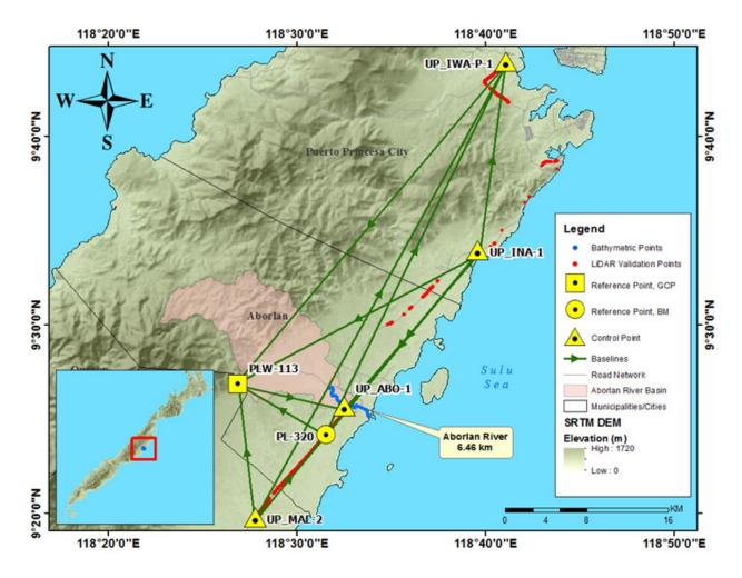
Figure 31. Extent of the bathymetric survey (in blue) in Aborlan River and the LiDAR data validation (in red) .
