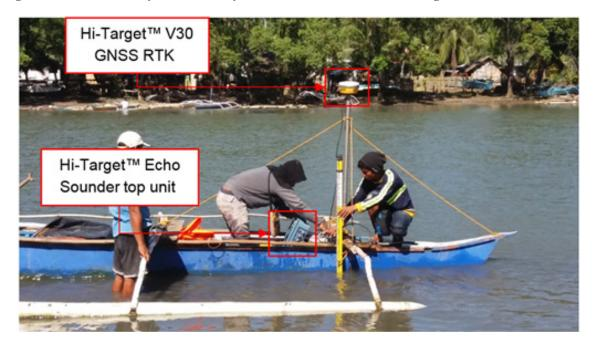
Figure 48. Bathymetric survey of ABSD at Aborlan River using Hi-Target™ Echo Sounder.
