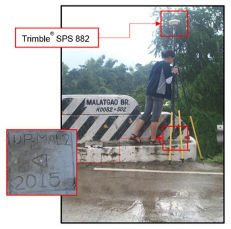
Figure 35. GNSS receiver set-up, Trimble® SPS 882, at UP\_MAL-2, located at the approach of Malatgao Bridge in Brgy. Tinagong Dagat, Narra, Province of Palawan.
