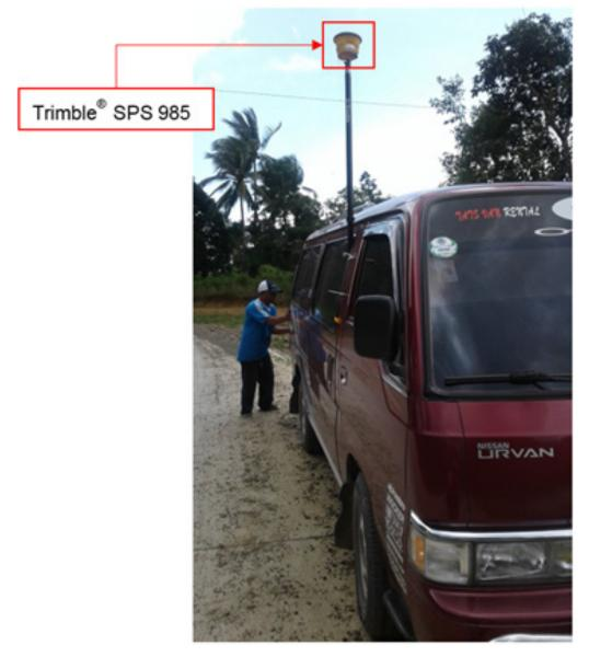
Figure 45. Validation points acquisition survey set-up for Aborlan River.
