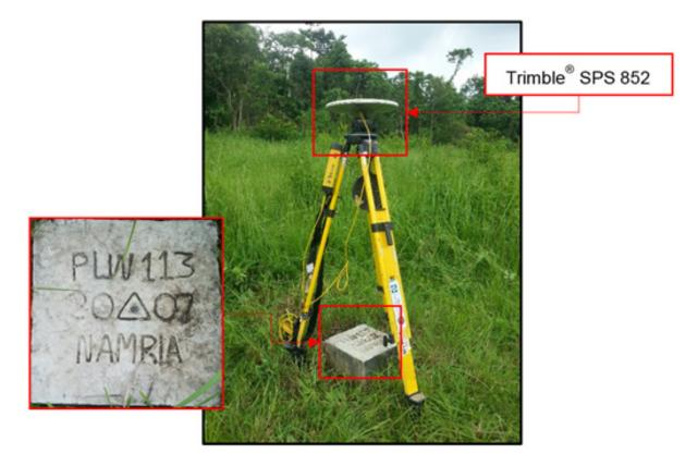
Figure 33. GNSS base set-up, Trimble® SPS 852, at PLW-113, located southwest of Aborlan Water System in Brgy. Dumagueña, Narra, Province of Palawan.
