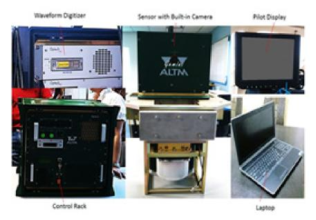
Figure A-1.2. Gemini Sensor Table A-1.2. Parameters and Specifications of Gemini Sensor
