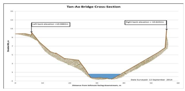
Figure 48. The cross-section plot of the Tanao Bridge
