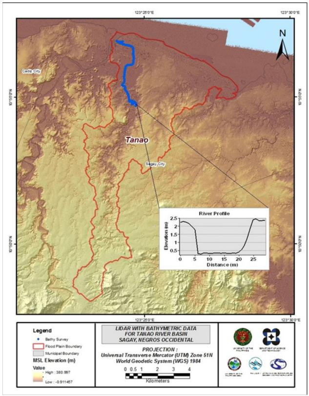
Figure 29. Map of Tanao floodplain with bathymetric survey points shown in blue.
