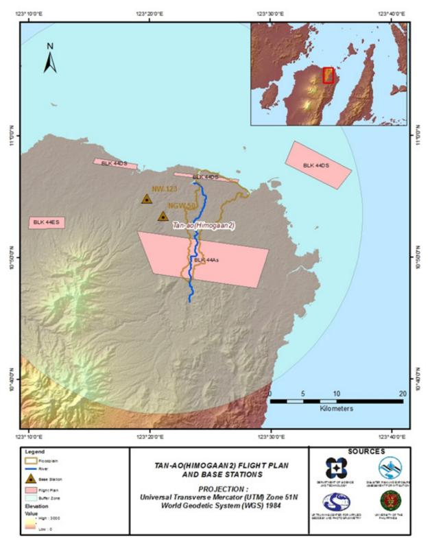
Figure 2. Flight Plan and base stations used for the Tanao Floodplain survey using Aquarius sensor.
