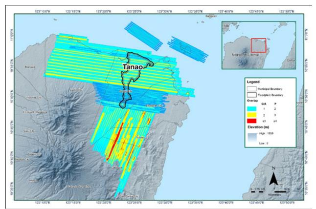
Figure 15. Data overlap between missions and flight lines for the Tanao River Floodplain Survey.
