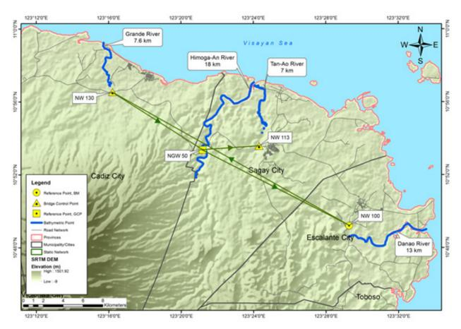
Figure 33. The GNSS Network established in the Tanao River Survey.
