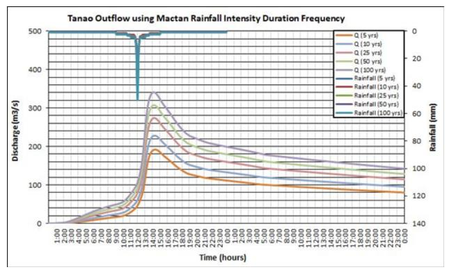
Figure 63. The Outflow hydrograph at the Tanao Station, generated using the Mactan RIDF simulated in HEC-HMS.
