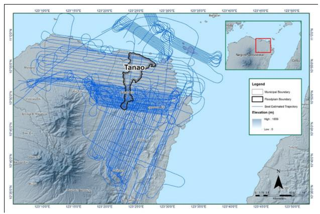
Figure 13. The Best Estimated Trajectory of the LiDAR missions conducted over the Tanao floodplain.
