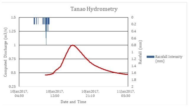
Figure 50. Rainfall and outflow data of the Tanao River Basin, which was used for modeling.
