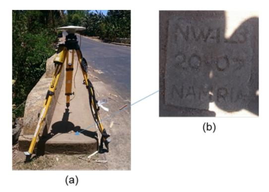
Figure 8. GPS set-up over NW-123 at the right side of the bridge located in Cadiz, Negros Occidental going to San Carlos, along the national road (a) and NAMRIA reference point NW-123 (b) as recovered by the field team.
