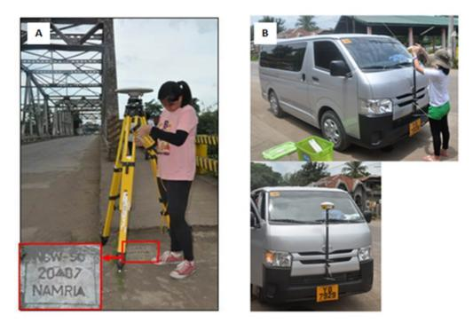
Figure 42. (A) Occupied base station, NGW-50, in Himoga-An Bridge, Sagay City and (B) Installation of GNSS Receiver Trimble® SPS 882 on the van prior the conduct of validation points acquisition survey
