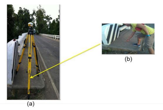
Figure 6. GPS set-up over NGW-58 at the NE sidewalk of Danao Bridge found at Brgy. Jonobjonob, Sitio Labarca, Escalante, Negros Occidental (a) and NAMRIA reference point MGW-58 (b) as recovered by the field team.
