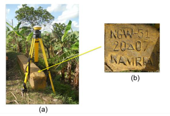
Figure 5. GPS set-up over NGW-51 at the NW tip of a yellow headwall found at the SW of Escalante-Bacolod national road at Brgy. Had Fe, Escalante, Negros Occidental (a) and NAMRIA reference point NGW-51 (b) as recovered by the field team.
