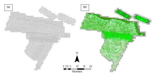
Figure 19. The coverage of the Tanao Floodplain Survey (a) the tile system (b) depicts the classification results in TerraScan.
