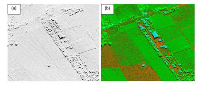
Figure 20. The images before (a) and after (b) undertaking classification.
