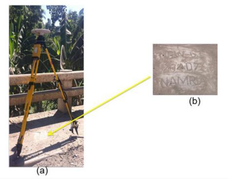
Figure 7. GPS set-up over NGW-63 at the NE end of the sidewalk of Daan-Lunsod Bridge at Brgy. Lemery, Calatrava, Negros Occidental (a) and NAMRIA reference point NGW-63 (b) as recovered by the field team.
