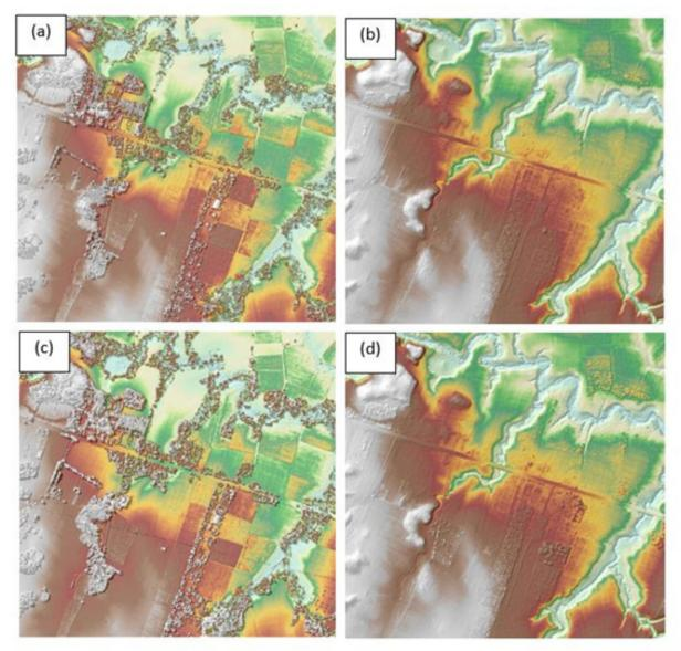
Figure 21. Photo (A) features the production of the last return DSM; (B) depicts the production of the DTM; (C) portrays the production of the first return DSM; and (D) presents the generation of the secondary DTM in some portions of the Tanao Floodplain.
