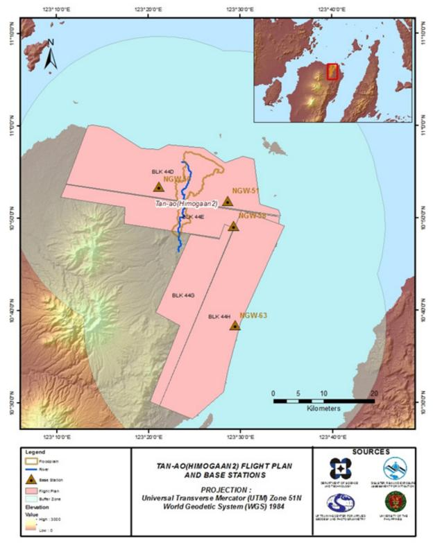
Figure 3. Flight Plan and base stations used for the Tanao Floodplain survey using Pegasus sensor.
