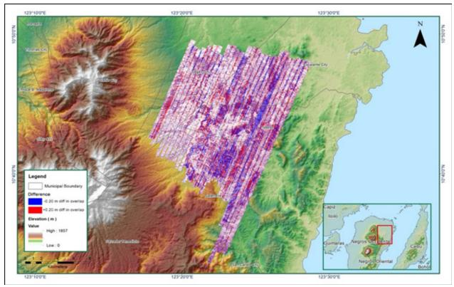
Figure A-8.14 Elevation difference between flight lines
