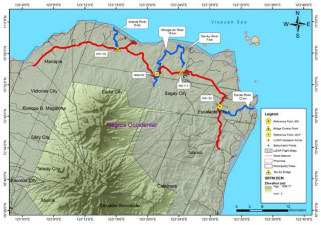
Figure 43. The extent of the LiDAR ground validation survey for Tanao River Basin
