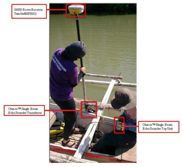
Figure 44. Set up of Ohmex<sup>™</sup> Single Beam Echo Sounder integrated with a roving GNSS receiver on a motor boat for the bathymetric survey in Brgy. Old Sagay, Sagay City, Negros Occidental
