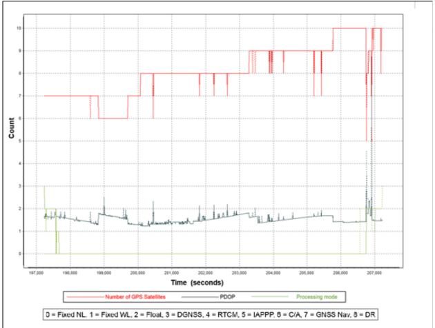
Figure 12. The Solution Status Parameters of Tanao Flight 1433P.
