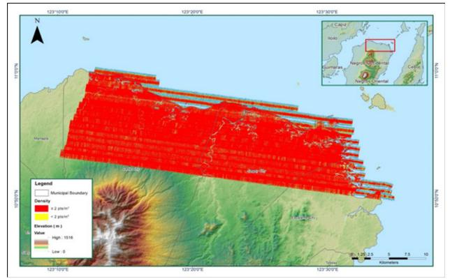
Figure A-8.6 Density map of merged LiDAR data
