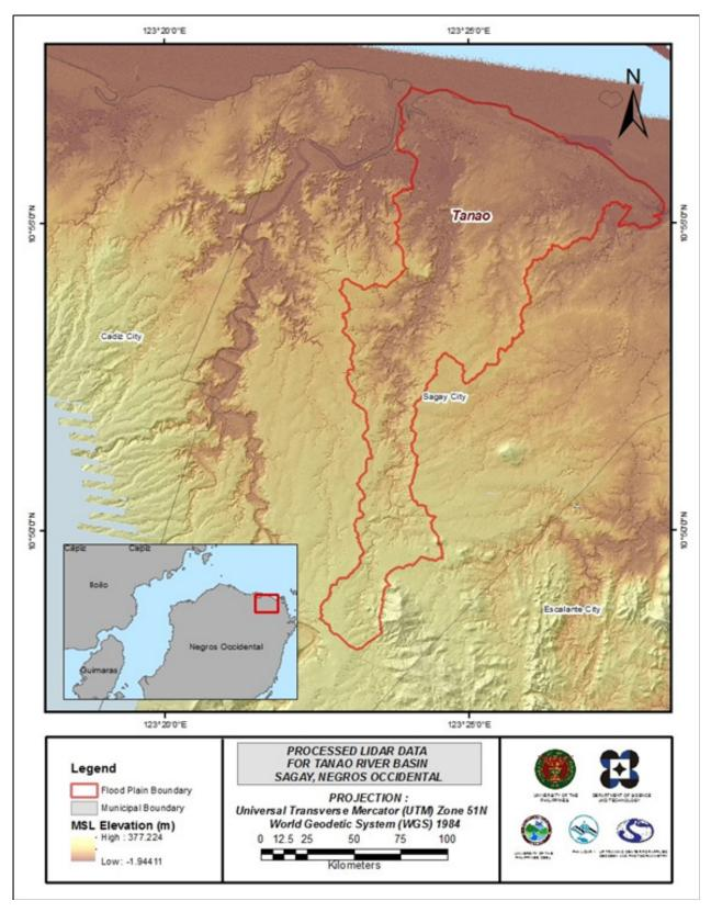
Figure 25. Map of processed LiDAR data for the Tanao Floodplain.
