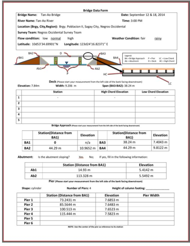
Figure 40. The Tanao Bridge as-built survey data
