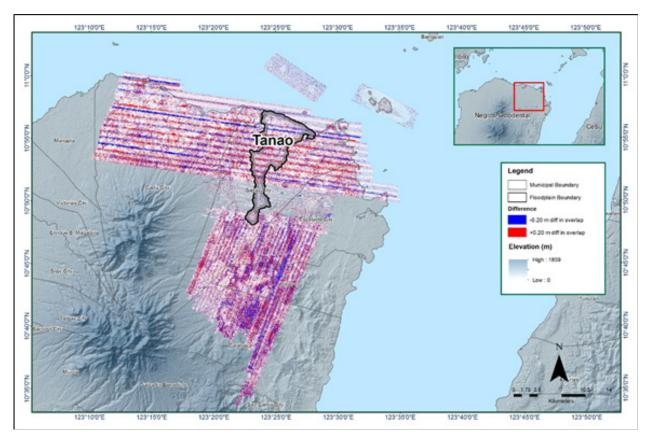
Figure 17. Map of elevation difference Map between flight lines for the Tanao Floodplain Survey.
