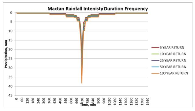
Figure 52. Synthetic storm generated for a 24-hour period rainfall for various return periods
