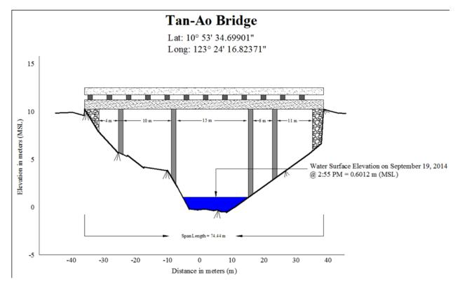
Figure 38. The Tanao Bridge cross-section survey drawn to scale
