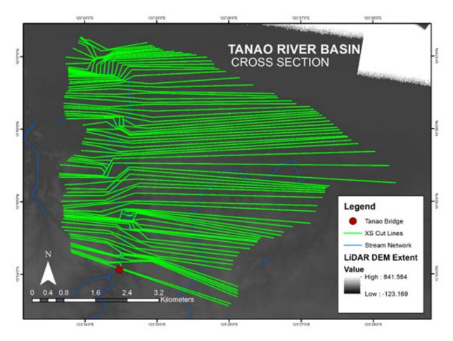
Figure 58. River cross-section of the Tanao River through the ArcMap HEC GeoRas tool
