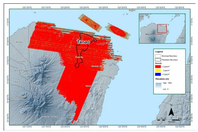
Figure 16. The pulse density map of the merged LiDAR data for the Tanao Floodplain Survey.
