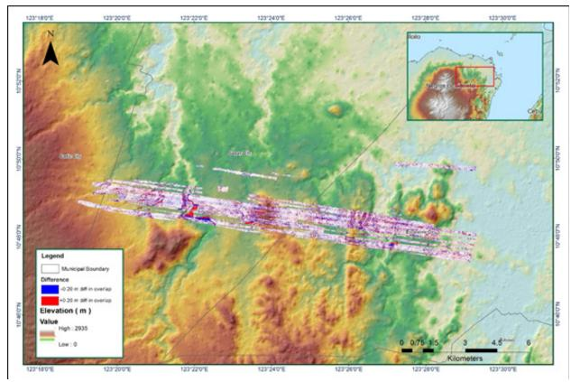
Figure A-8.28 Elevation difference between flight lines
