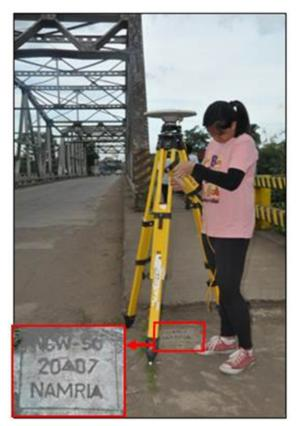
Figure 34. The GNSS base receiver setup, Trimble® SPS 852, at NGW-50 in Himoga-An Bridge, Brgy. Paraiso, Sagay City, Negros Occidental
