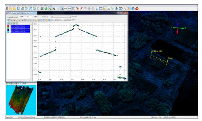
Figure 18. Screen-capture of the quality checking for Tanao Flight 1433P using the Profile Tool of QT Modeler.
