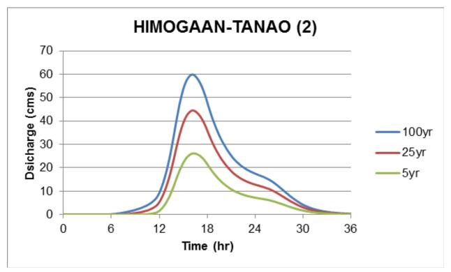
Figure 65. Himogaan and Tanao river (2) generated discharge using 5-, 25-, and 100-year Iloilo and Mactan stations' rainfall intensity-duration-frequency (RIDF) in HEC-HMS
