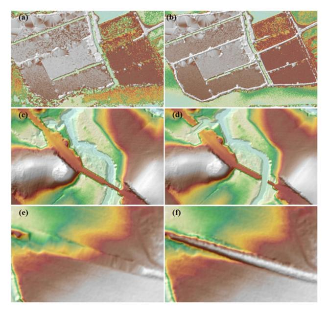
Figure 24. Portions in the DTM of the Tanao Floodplain showing (a) a paddy field before manual editing; (b) paddy after data retrieval; (c) a bridge before undergoing manual editing, while (d) after manual editing; (e) a building before manual editing, while (f) after manual editing.
