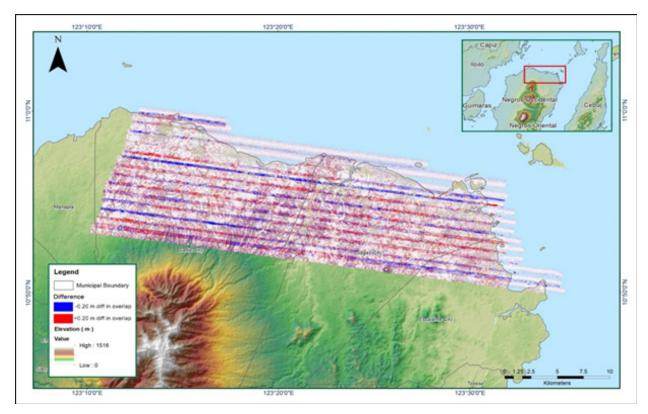
Figure A-8.7 Elevation difference between flight lines
