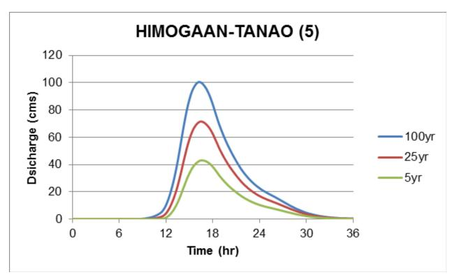
Figure 68. Himogaan and Tanao river (5) generated discharge using 5-, 25-, and 100-year Iloilo and Mactan stations' rainfall intensity-duration-frequency (RIDF) in HEC-HMS
