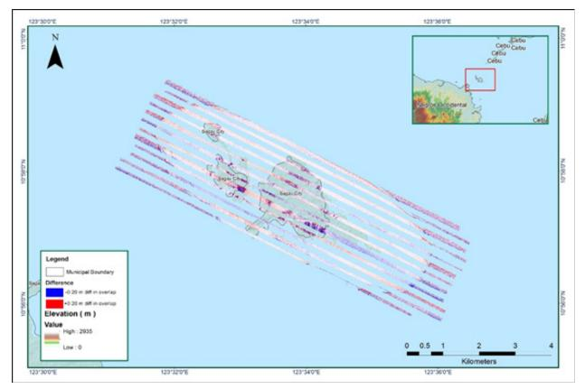
Figure A-8.49 Elevation difference between flight lines
