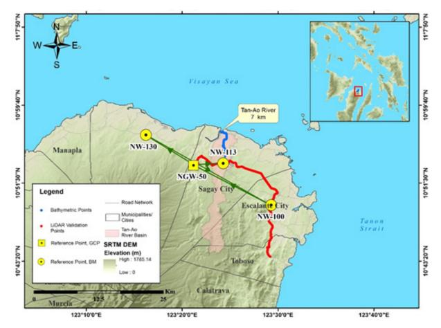
Figure 32. Extent of the bathymetric survey (in blue line) in Tanao River.
