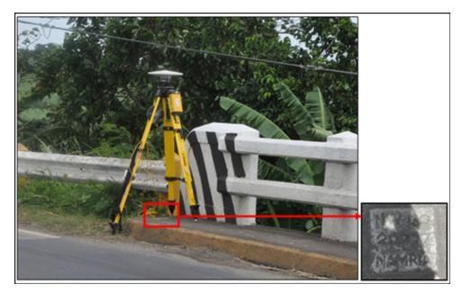
Figure 36. The GNSS (Trimble® SPS 852) receiver occupation, at NW-130 in Troso Bridge, Brgy. Daga, Cadiz City, Negros Occidental
