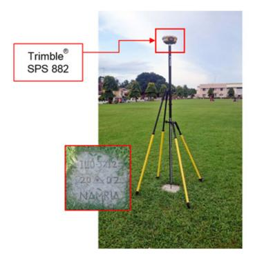
Figure 41. GNSS receiver set-up, Trimble® SPS 882 at ILO-3212, located in Pototan Town Plaza in Barangay San Jose Ward, Municipality of Pototan, Iloilo
