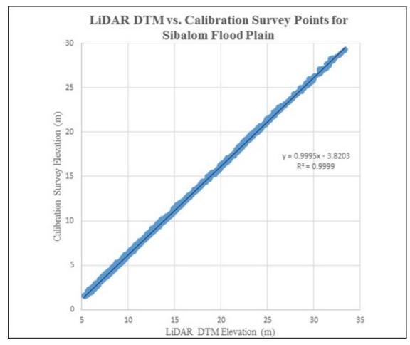
Figure 29. Correlation plot between the calibration survey points and the LiDAR data
