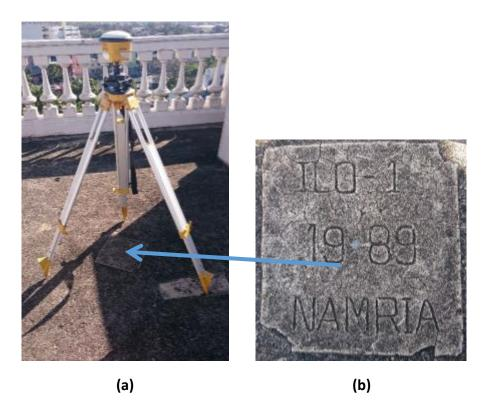
Figure 5. (a) GPS set-up over ILO-1, on top of St. Clements Church bell tower, across the Western Institute of Technology; and (b) NAMRIA reference point ILO-1, as recovered by field team
