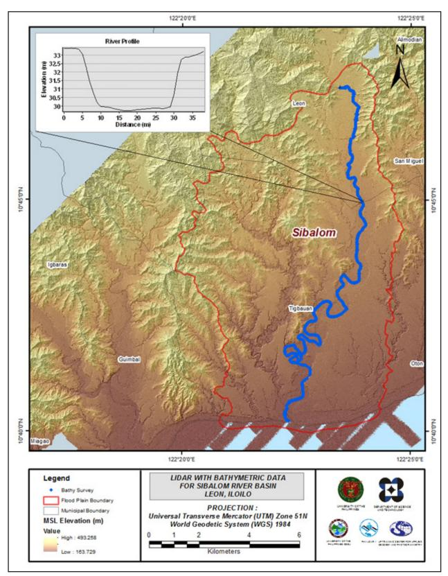
Figure 31. Map of the Sibalom floodplain, with bathymetric survey points shown in blue
