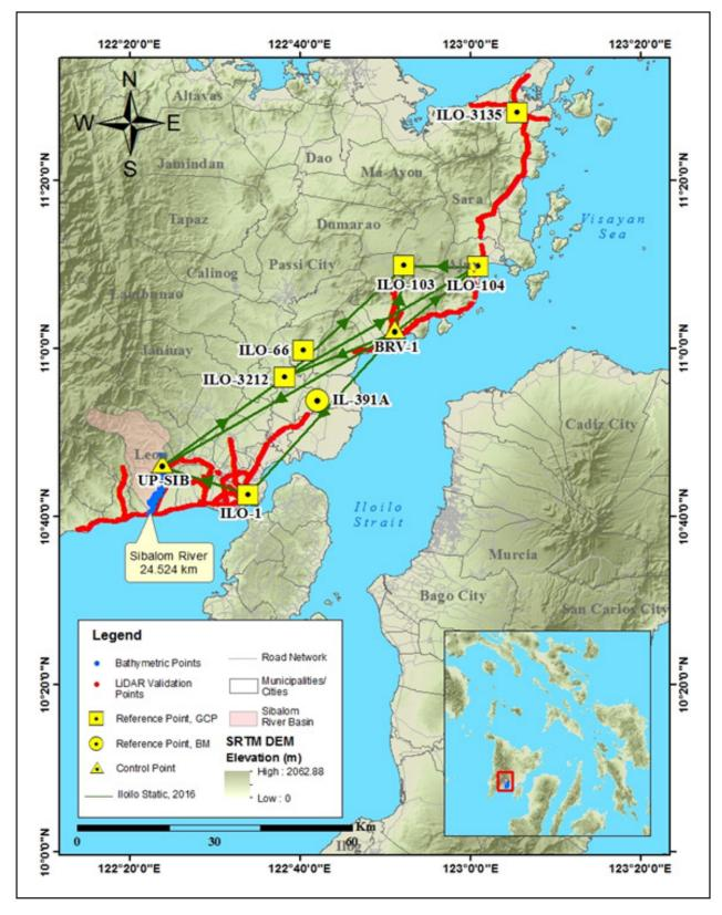
Figure 34. Extent of the bathymetric survey (in blue line) in the Sibalom River and the LiDAR data validation survey (in red)
