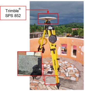
Figure 37. GNSS base set-up, Trimble® SPS 852 at BRV-1, situated on top of Hollywood Star Inn in Barangay Poblacion, Municipality of Barotac Viejo, Iloilo
