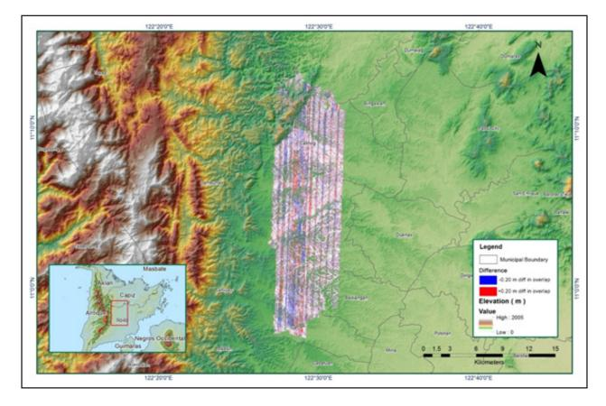
Figure A-8.62. Elevation difference between flight lines
