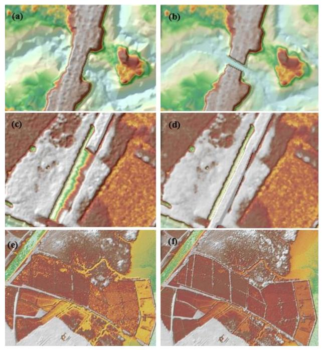
Figure 26. Portions in the DTM of the Sibalom floodplain – a bridge (a) before and (b) after manual editing; a road (c) before and (d) after data retrieval; and a paddy field (e) before and (f) after data retrieval
