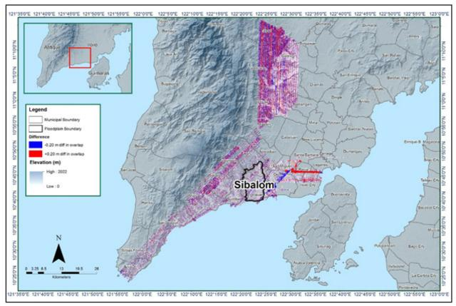
Figure 19. Elevation difference map between flight lines for the Sibalom floodplain
