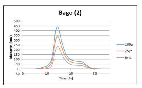
Figure 72. Sibalom River (2) generated discharge using 5-, 25-, and 100-year Iloilo City RIDF in HEC-HMS
