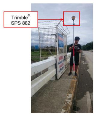
Figure 43. As-built survey of the Baltazar Bridge
