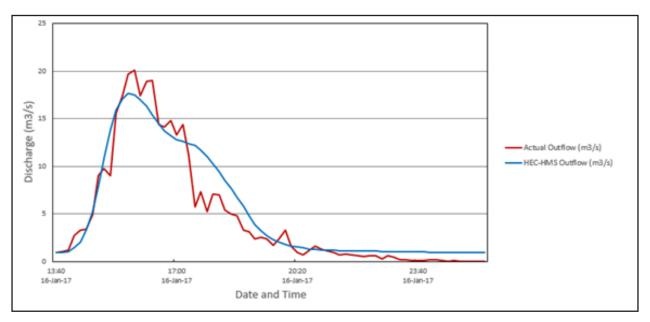
Figure 69. Outflow hydrograph of Sibalom produced by the HEC-HMS model, compared with observed outflow
