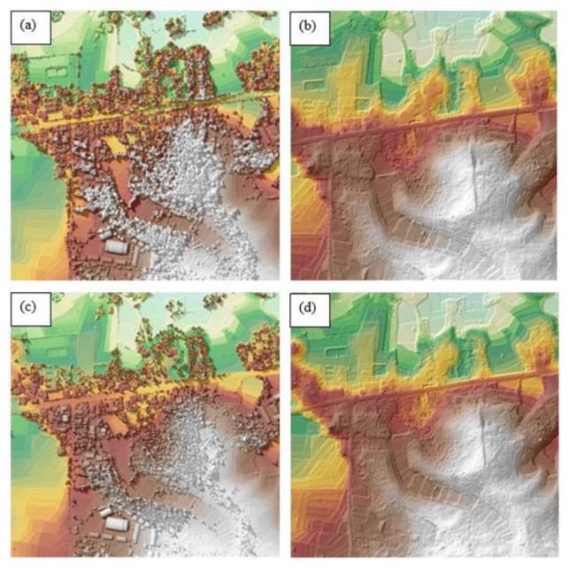
Figure 23. (a) The production of last return DSM and (b) DTM, (c) first return DSM and (d) secondary DTM in some portion of the Sibalom floodplain
