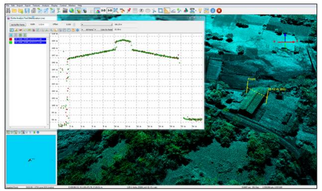
Figure 20. Quality checking for Sibalom Flight 2528G, using the Profile Tool of QT Modeler
