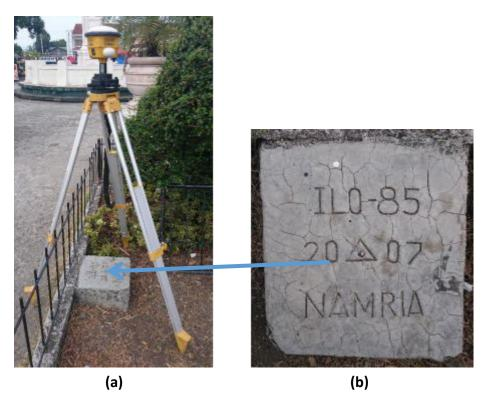
Figure 6. (a) GPS set-up over ILO-85, at the corner of a planting strip and sidewalk at the town plaza of Barangay Poblacion, Miagao, Iloilo, about 14 m fronting the Rizal monument; and (b) NAMRIA reference point ILO-85, as recovered by the field team
