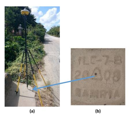
Figure 10. (a) GPS set-up over ILC-7B; and (b) NAMRIA reference point ILC-7B, as recovered by the field team
