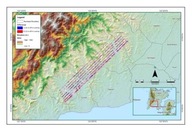
Figure A-8.7. Elevation difference between flight lines
