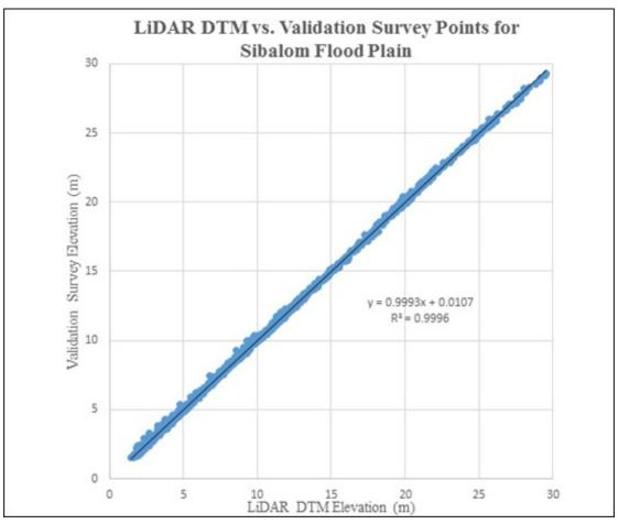
Figure 30. Correlation plot between the validation survey points and the LiDAR data
