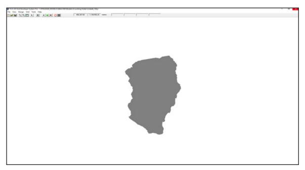
Figure 66. Screenshot of a sub-catchment with the computational area to be modeled in the FLO-2D Grid Developer System Pro (FLO-2D GDS Pro)
