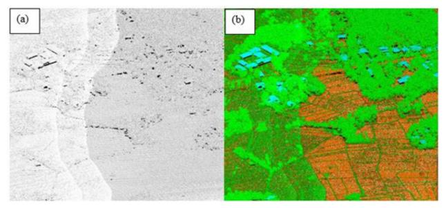
Figure 22. Point cloud (a) before and (b) after classification
