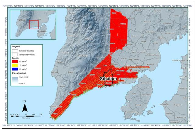
Figure 18. Pulse density map of merged LiDAR data for the Sibalom floodplain
