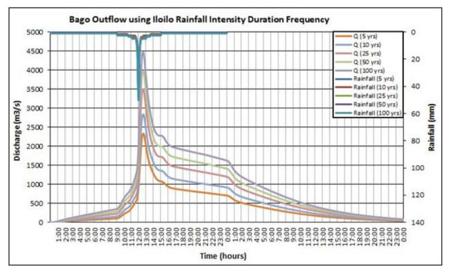
Figure 70. Outflow hydrograph at the Sibalom Station generated using the Iloilo RIDF, simulated in HEC-HMS
