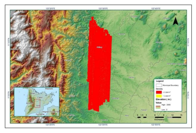
Figure A-8.61. Density map of merged LiDAR data
