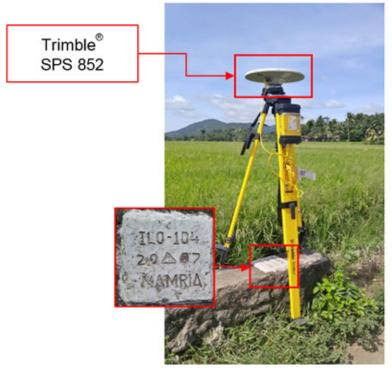
Figure 40. GNSS receiver set-up, Trimble® SPS 852 at ILO-104, located along the National Highway in Barangay San Antonio, Municipality of Ajuy, Iloilo
