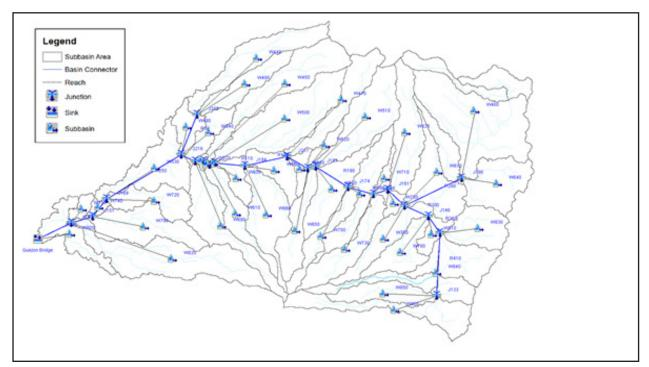
Figure 64. The Sibalom River Basin model, generated using HEC-HMS
