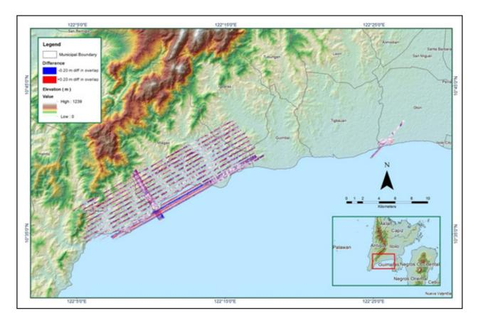
Figure A-8.34. Elevation difference between flight lines
