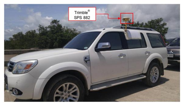
Figure 48. Validation points acquisition survey set-up along the Sibalom River Basin
