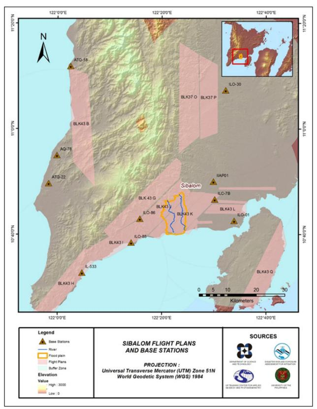
Figure 2. Flight plans and base stations used to cover the Sibalom floodplain survey
