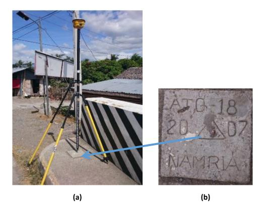
Figure 3. (a) GPS set-up over ATQ-18 on the NE approach of the Binangbang Bridge, about 600 meters NE of Barbaza Town Hall, 4 meters from the road centerline, 50 meters SE of Barbaza Multi-Purpose Coop; and, (b) NAMRIA reference point ATQ-18, as recovered by the field team
