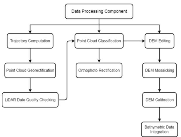
Figure 12. Schematic diagram for the Data Pre-Processing Component
