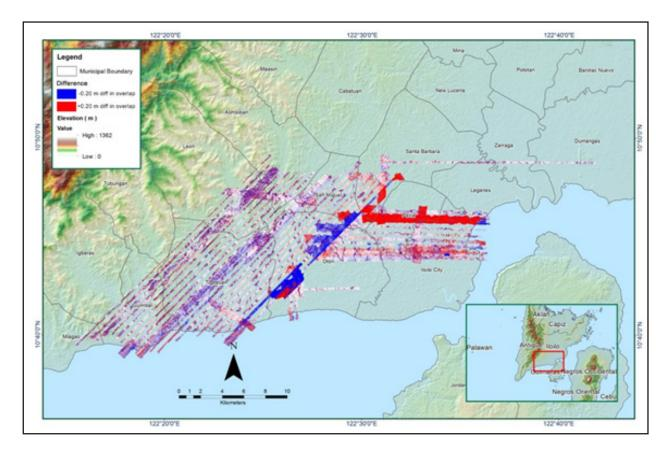
Figure A-8.14. Elevation difference between flight lines
