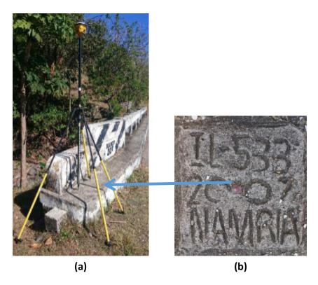
Figure 9. (a) GPS set-up over IL-533, located 3 meters from the edge of the sidewalk of the Amboyu-an Bridge at Barangay Amboyu-an, San Joaquin, Iloilo; and (ii.) NAMRIA reference point IL-533, as recovered by the field team
