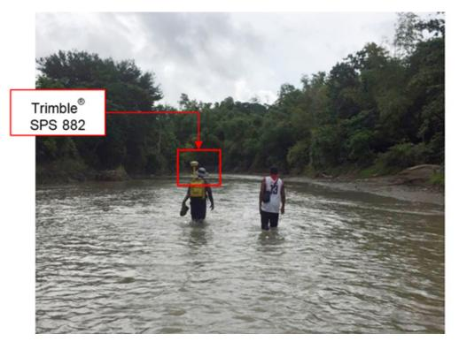
Figure 50. Manual bathymetric survey using a Trimble® SPS 882 in GNSS PPK survey technique in continuous topo mode in the Sibalom River
