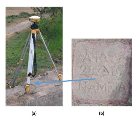
Figure 4. (a) GPS set-up over ATQ-22 on top of the N edge of the NW draft on an irrigation canal, 60 meters NE of the national highway centerline, 120 meters N of the road going to the barangay proper, and about 300 meters E of KM Post 110; and (b) NAMRIA reference point ATQ-22, as recovered by the field team
