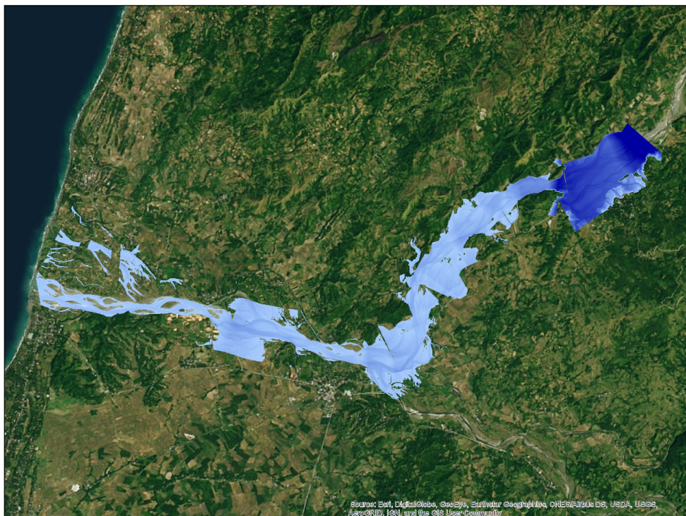
Figure 68. The sample output map of the Sibalom 2RAS Model.
