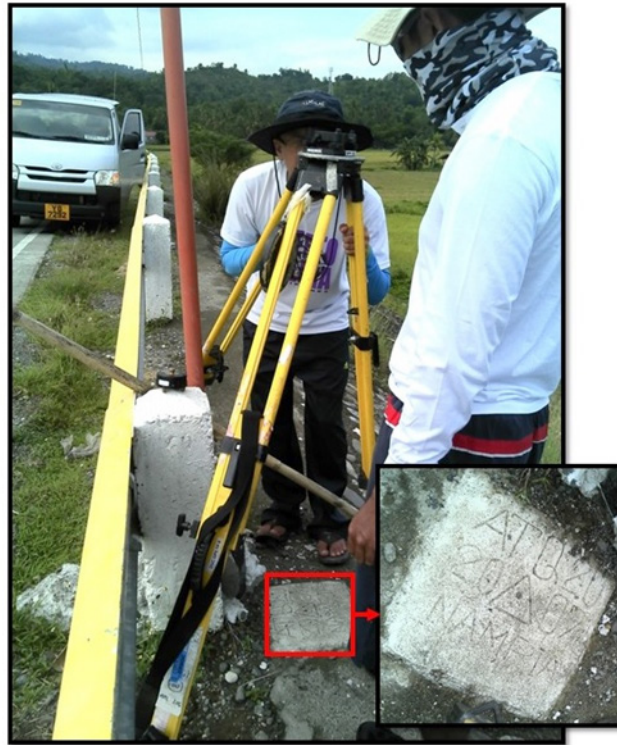
Figure 38. GNSS base receiver setup, Trimble® SPS 852 at ATQ-20 in Brgy. Zaragoza, Municipality of Bugasong, Antique.
