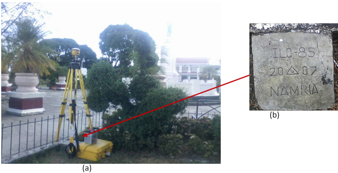
Figure 10. GPS set-up over ILO-85 as recovered at the Town Plaza in Miag-ao, Iloilo (a) NAMRIA reference point ILO-85 (b) as recovered by the field team.
