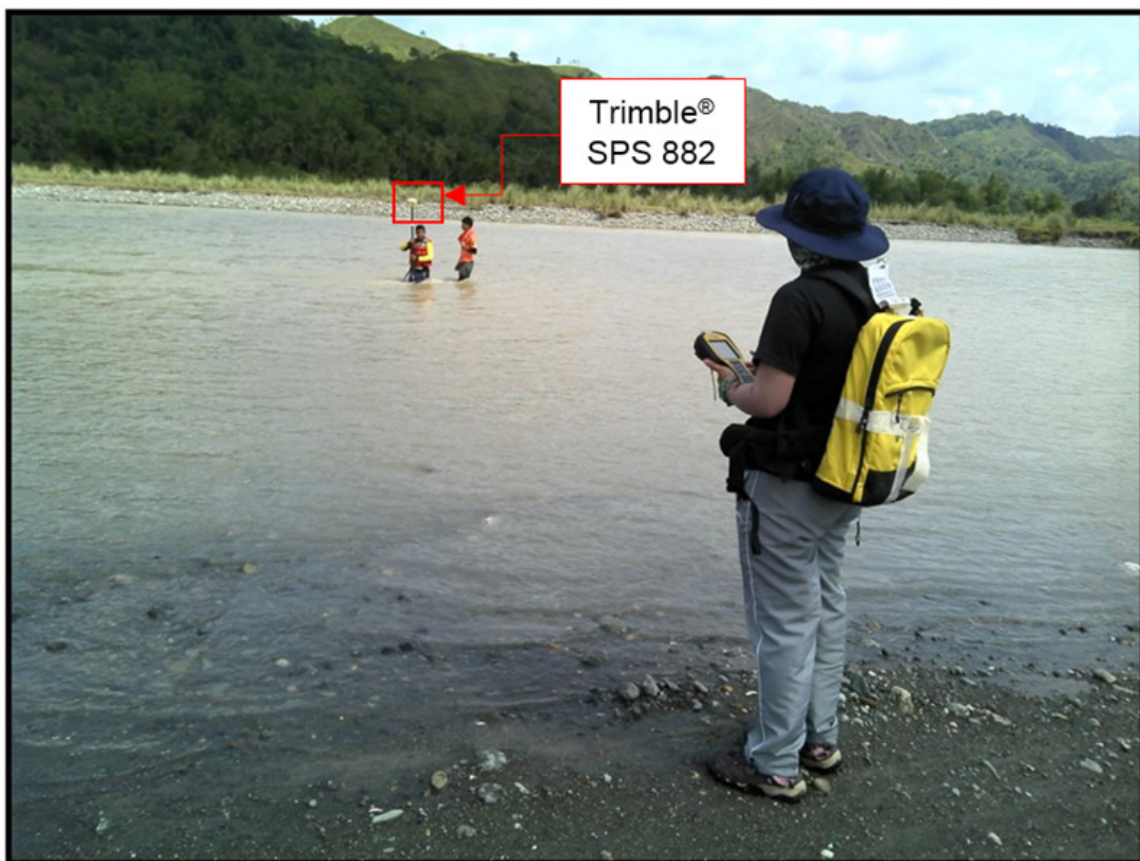
Figure 50. The setup for the manual Bathymetric Survey in Sibalom 2River
