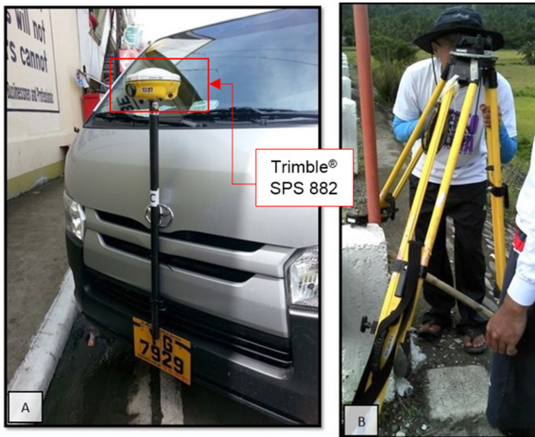
Figure 48. (A) Trimble™ SPS 882 attached to a vehicle and (B) Setting up of GNSS base station at ATQ-20
