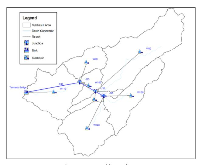
Figure 55. The Ipayo River Basin model generated using HEC-HMS  $\,$
