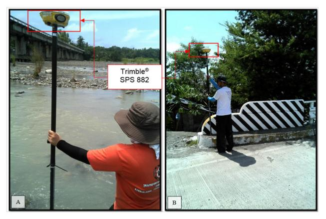
Figure 36. a) Cross-section survey, and b) Bridge-as-built survey of Ipayo Bridge in the Municipality of Patnongon
