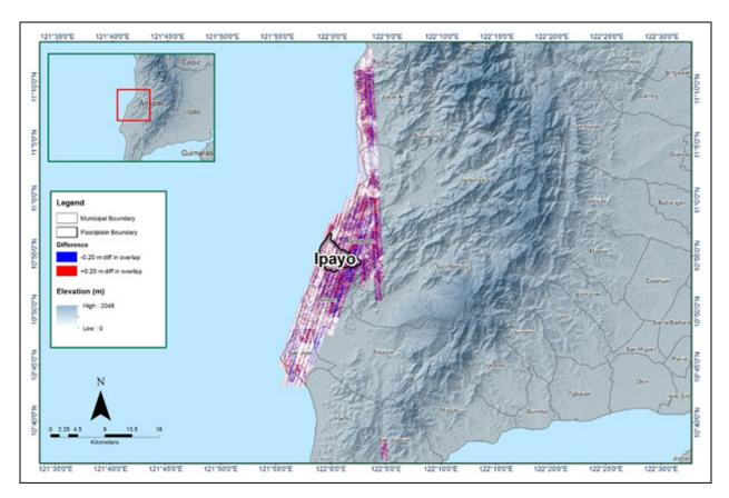
Figure 16. Elevation difference map between flight lines for Ipayo Floodplain.
