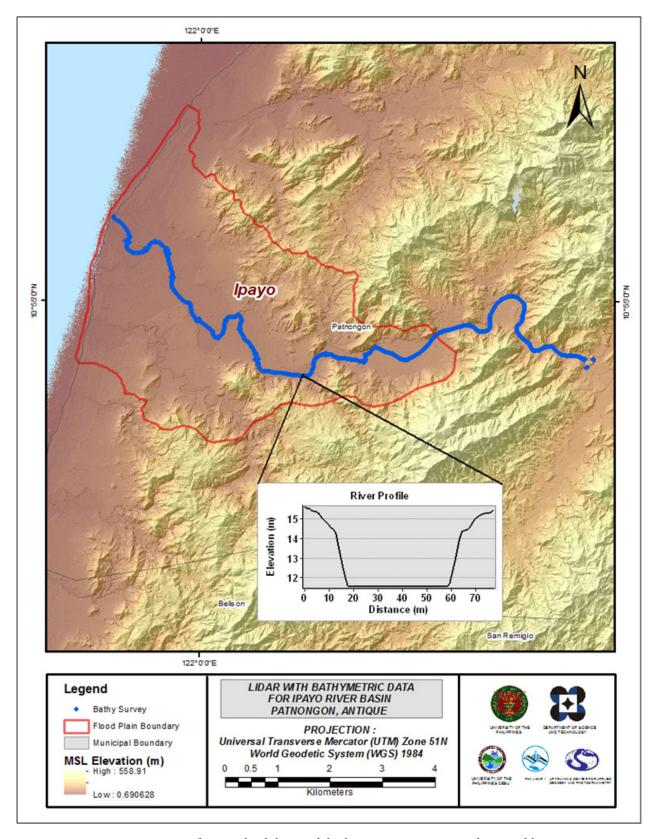
Figure 28. Map of Ipayo Floodplain with bathymetric survey points shown in blue.
