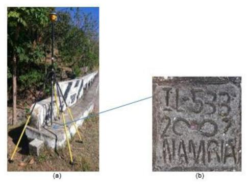
Figure 7. a) GPS set-up over IL-533, located 3 meters from the edge of the sidewalk of Amboyu-an Bridge at Brgy. Amboyu-an, San Joaquin, Iloilo, and b) NAMRIA reference point IL-533, as recovered by the field team.
