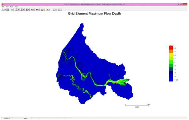
Figure 59. Generated 100-year rain return flow depth map from FLO-2D Mapper
