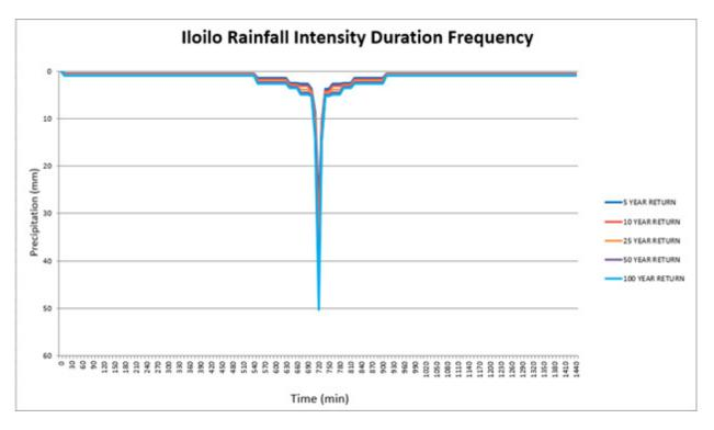
Figure 50. The synthetic storm generated for a 24-hour period for various return periods
