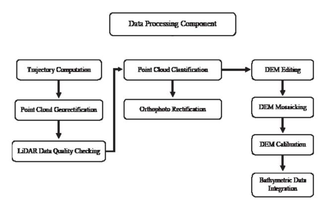
Figure 9. Schematic Diagram for Data Pre-Processing Component
