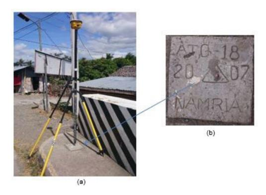
Figure 3. a) GPS set-up over ATQ-18 on the NE approach of Binangbang Bridge, about 600 meters NE of Barbaza Town Hall, 4 meters from the road centerline, 50 meters SE of Barbaza Multi-Purpose Coop, and b) NAMRIA reference point ATQ-18, as recovered by the field team.
