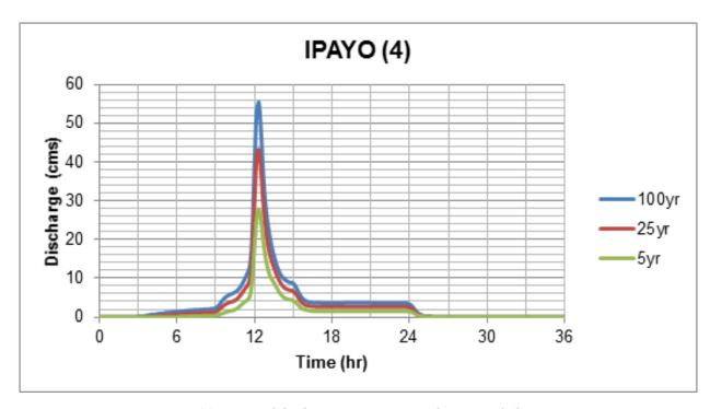
Figure 65. Ipayo river (3) generated discharge using 5-, 25-, and 100-year Iloilo RIDF in HEC-HMS
