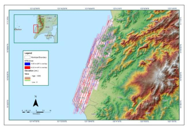
Figure A-8.14. Elevation difference between flight lines
