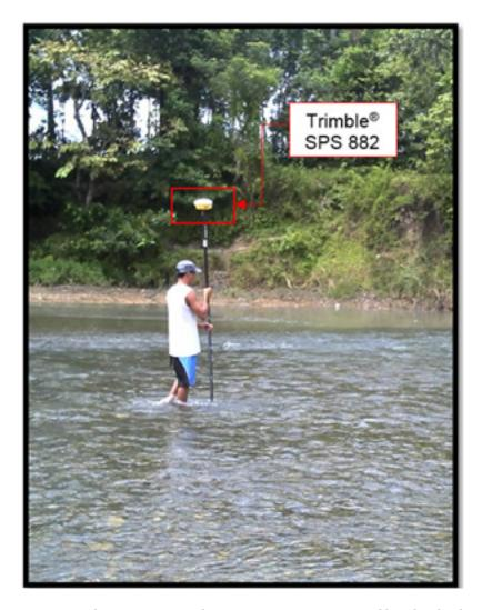
Figure 42. Bathymetric Survey along Ipayo River accompanied by a local aide
