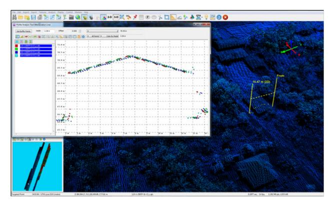
Figure 17. Quality checking for a Ipayo Flight 2587P using the Profile Tool of QT Modeler.
