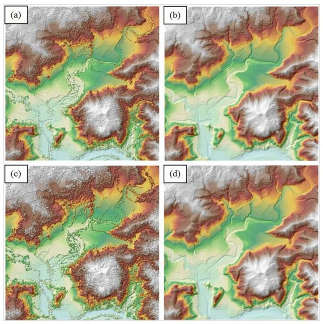
Figure 20. The Production of last return DSM (a) and DTM (b), first return DSM (c) and secondary DTM (d) in some portion of IpayoFloodplain.
