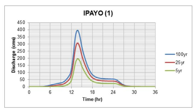
Figure 62. Ipayo river (1) generated discharge using 5-, 25-, and 100-year Iloilo RIDF in HEC-HMS
