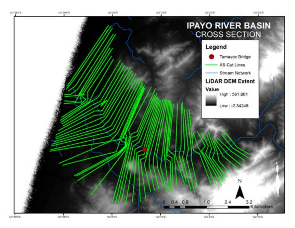
Figure 56. River cross-section of Ipayo River generated through Arcmap HEC GeoRAS tool
