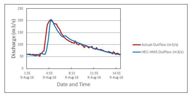
Figure 60. Outflow Hydrograph of Ipayo River Basin produced by the HEC-HMS model compared with observed outflow
