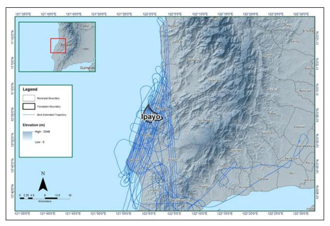
Figure 12. Best estimated trajectory of the LiDAR missions conducted over the Ipayo Floodplain.
