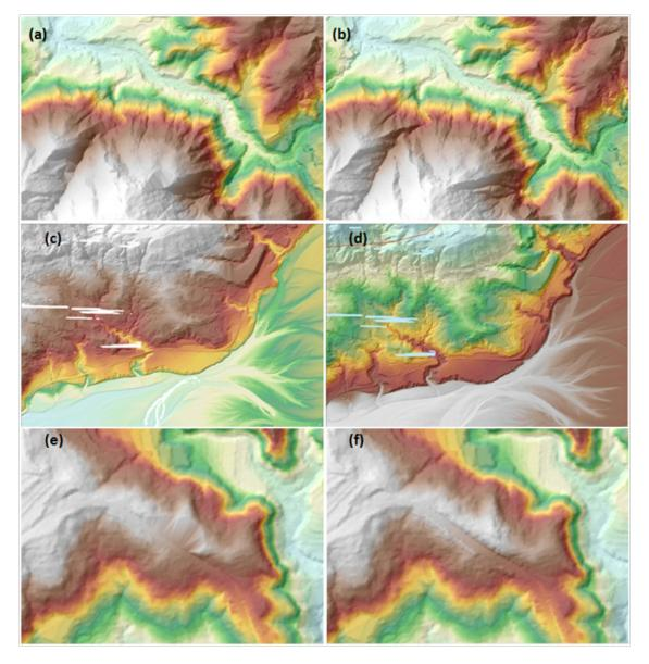
Figure 23. Portions in the DTM of Ipayo Floodplain – a mountain before (a) and after (b) data retrieval; bridges before (c) and after (d) manual editing; and an area before (e) and after (f) data retrieval.
