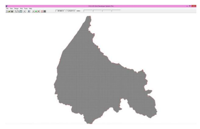
Figure 57. A screenshot of the river subcatchment with the computational area to be modeled in FLO-2D GDS Pro
