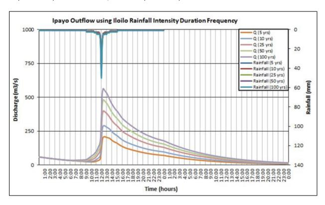
Figure 61. The Outflow hydrograph at Ipayo Station, generated using Iloilo RIDF simulated in HEC-HMS
