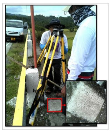
Figure 33. GNSS base receiver set-up, Trimble® SPS 852 at ATQ-20 in Brgy. Zaragoza, Municipality of Bugasong, Antique
