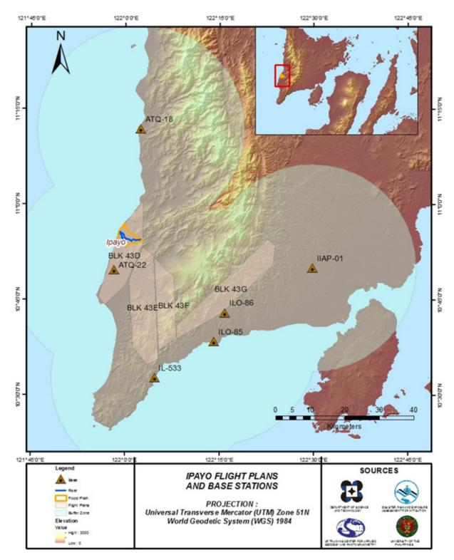
Figure 2. Flight plans and base stations used to cover Ipayo Floodplain
