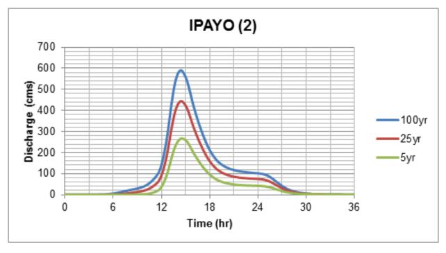
Figure 63. Ipayo river (2) generated discharge using 5-, 25-, and 100-year Iloilo RIDF in HEC-HMS
