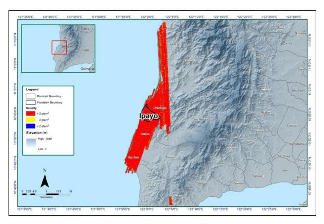
Figure 15. Pulse density map of merged LiDAR data for Ipayo Floodplain.
