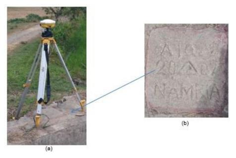
Figure 4. a) GPS set-up over ATQ-22 on top of the N edge of the NW draft on an irrigation canal, 60 meters NE to the national highway centerline, 120 meters N of the road going to the barangay proper and about 300 meters E of KM Post 110, and b) NAMRIA reference point ATQ-22, as recovered by field team.
