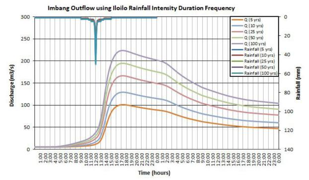
Figure 63. Outflow hydrograph at Imbang Station generated using Iloilo RIDF simulated in HEC-HMS
