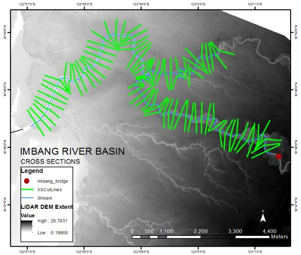
Figure 58. River cross-section of Imbang River generated through Arcmap HEC GeoRAS tool
