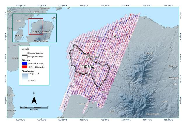
Figure 15. Elevation difference map between flight lines for Imbang floodplain.
