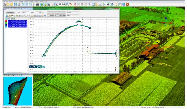
Figure 16. Quality checking for Imbang flight 1393P using the Profile Tool of QT Modeler.
