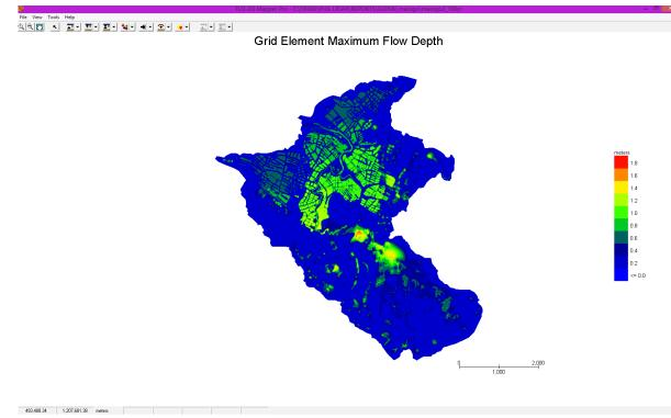
Figure 61. Generated 100-year rain return flow depth map from FLO-2D Mapper
