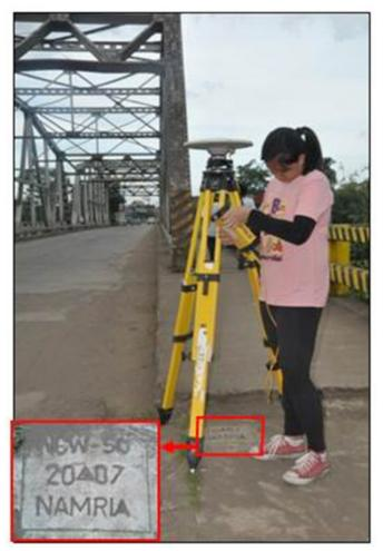
Figure 32. GNSS base receiver setup, Trimble<sup>®</sup> SPS 852, at NGW-50 in Himoga-An Bridge, Brgy. Paraiso, Sagay City, Negros Occidental
