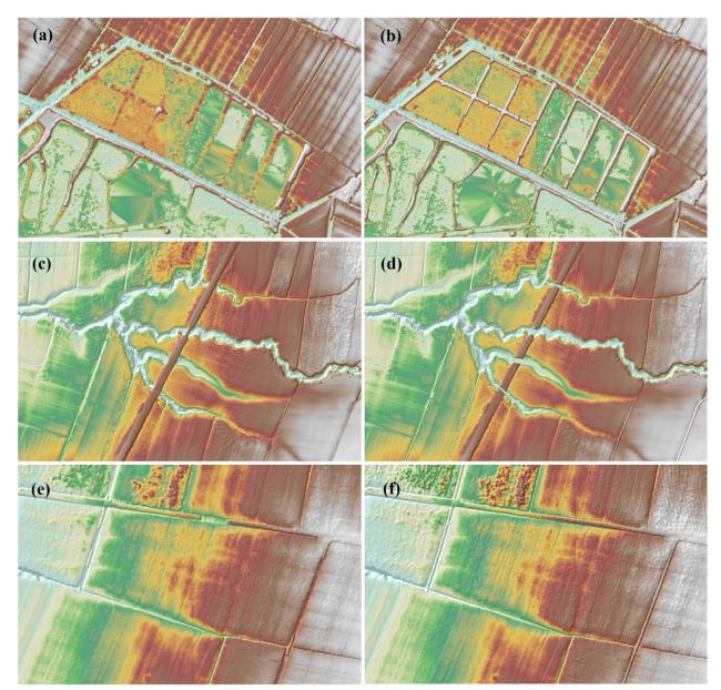
Figure 22. Portions in the DTM of Imbang floodplain – a paddy field before (a) and after (b) data retrieval; bridges before (c) and after (d) manual editing; and a road before (e) and after (f) data retrieval.
