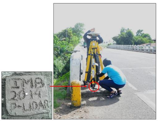
Figure 35. GNSS base receiver setup, Trimble<sup>®</sup> SPS 852, at IMB in Imbang Bridge, Brgy. Lantad, Silay City, Negros Occidental
