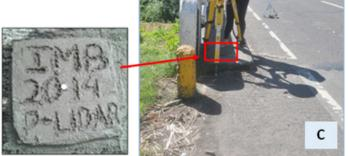
Figure 41. (A) GNSS Receiver Trimble<sup>®</sup> SPS 882 installation (B) Final set up of GNSS Receiver and (C) Base setup at IMB in Imbang Bridge, Silay City
