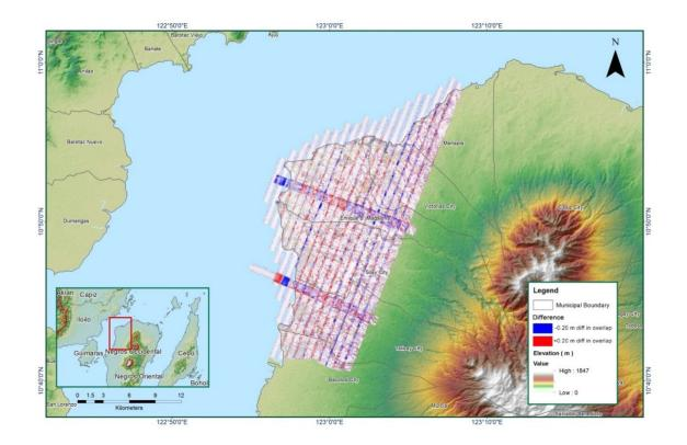
Figure 1.1.7 Elevation difference between flight lines
