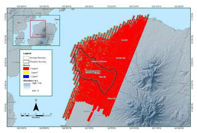
Figure 14. Pulse Density map of merged LiDAR data for Imbang floodplain.
