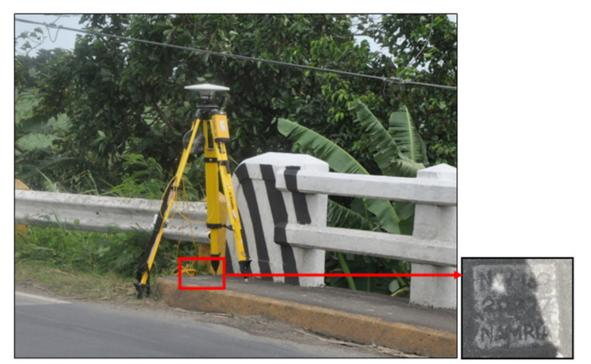
Figure 34. GNSS base receiver setup, Trimble<sup>®</sup> SPS 852, over NW-130 in Troso Bridge, Brgy. Daga, Cadiz City, Negros Occidental
