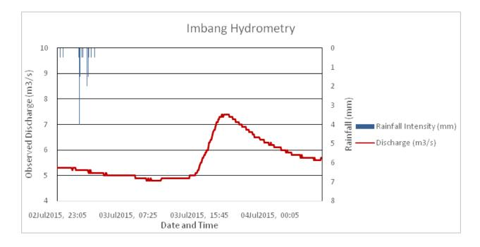
Figure 50. Rainfall and outflow data at Imbang used for modeling
