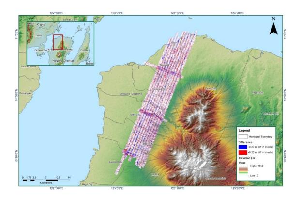
Figure 1.2.7 Elevation difference between flight lines
