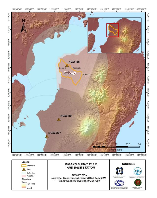
Figure 3. Flight plans and base station for Imbang floodplain
