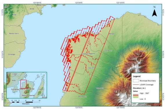
Figure 1.1.4 Coverage of LIDAR data
