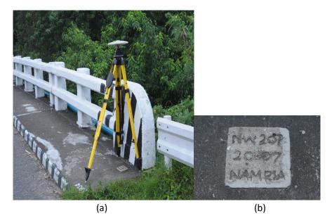
Figure 6. GPS set-up (a) over NW-207, positioned on concrete sidewalk at Ponteverda Bridge, located in Brgy. San Juan, Ponteverda, Negros Occidental, and NAMRIA benchmark NW-207 (b) as recovered by the field team.
