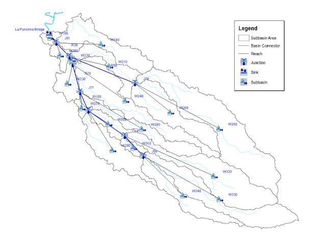
Figure 57. The Imbang river basin model generated using HEC-HMS
