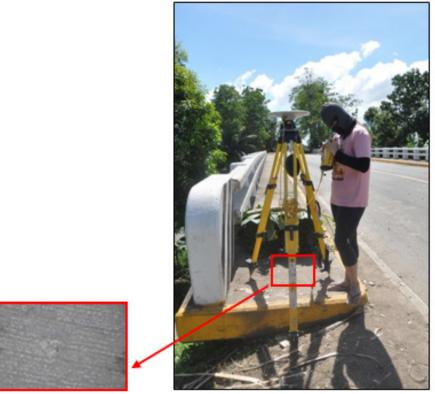
Figure 33. GNSS base receiver setup, Trimble<sup>®</sup> SPS 852, at NW-100 in Danao Bridge,Brgy. Jonobjonob, Escalante City, Negros Occidental
