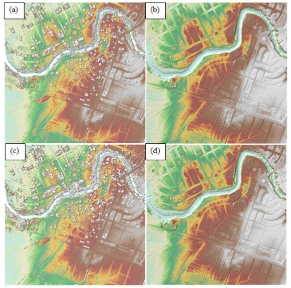
Figure 19. The production of last return DSM (a) and DTM (b), first return DSM (c) and secondary DTM (d) in some portion of Imbang floodplain.
