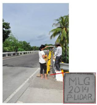
Figure 36. GNSS base receiver setup, Trimble<sup>®</sup> SPS 852, at MLG in Malogo Bridge,Brgy. Alicante, Victorias City, Negros Occidental
