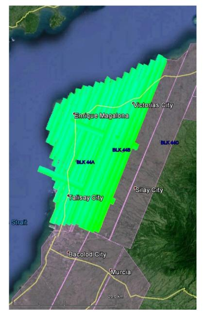
Flight No.:10007PArea:BLK 44AMission Name:1BLK44LMSCALIB275AParameters:Altitude: 1000; Scan Frequency: 30; Scan Angle: 25; Overlap: 30%
