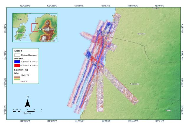
Figure 1.3.7. Elevation difference between flight lines
