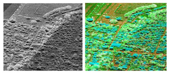
Figure 18. Point cloud before (a) and after (b) classification.
