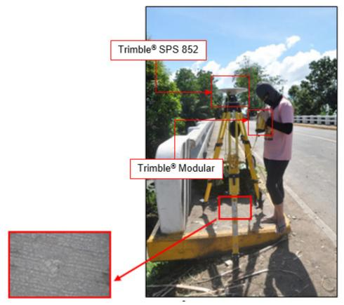
Figure 4. GPS set-up over NGW-58 in Brgy. Jonobjonob, Sitio Labarca, Escalante, Negros Occidental. It is on top of embedded benchmark NW-100.
