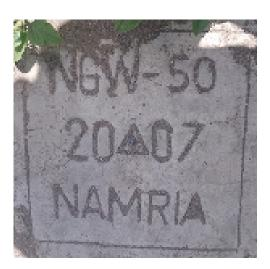
Figure 3. GPS set-up over NGW-50 in Sagay, Negros Occidental (a) NAMRIA reference point NGW-50 (b) as recovered by the field team.
