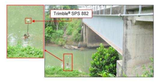
Figure 34. Cross-section survey at Troso Bridge in Cadiz City
