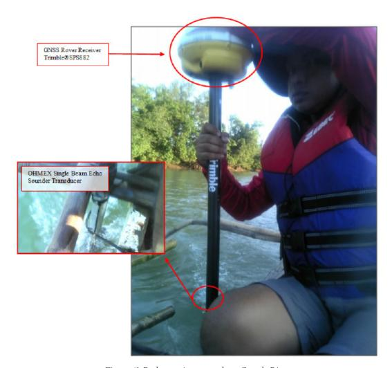
Figure 41. Bathymetric survey along Grande River
