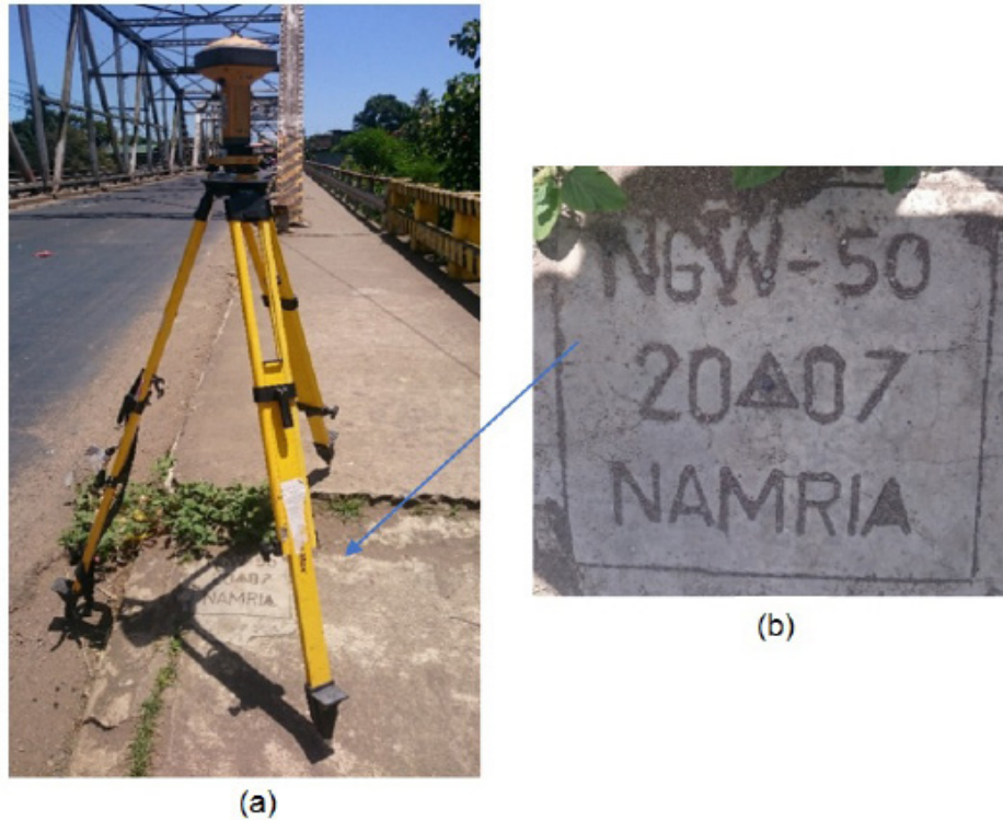
Figure 3. GPS set-up over NGW-50 in Sagay, Negros Occidental (a) NAMRIA reference point NGW-50 (b) as recovered by the field team.
