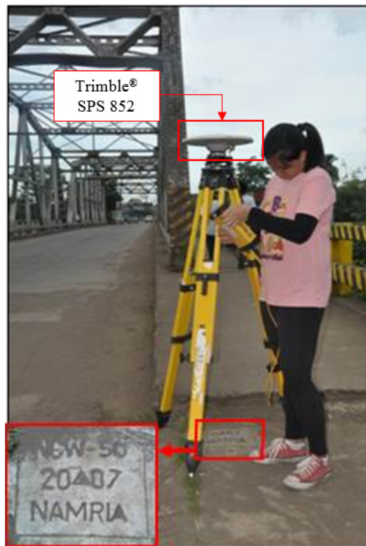
Figure 32. GNSS base receiver setup, Trimble® SPS 852, at NGW-50 in Himoga-An Bridge, Brgy. Paraiso, Sagay City, Negros Occidental
