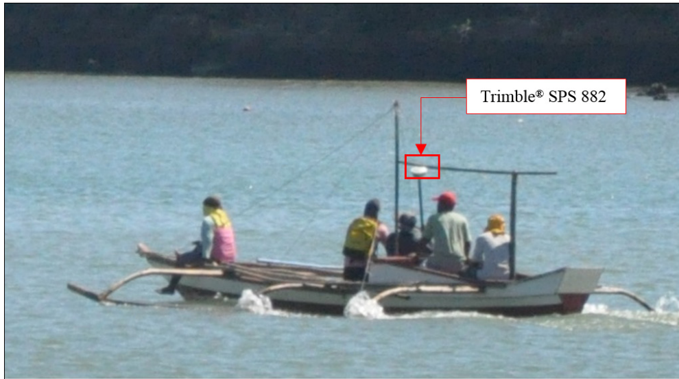
Figure 42. Execution of bathymetric survey using Ohmex™ Single Beam Echo Sounder along Danao River
