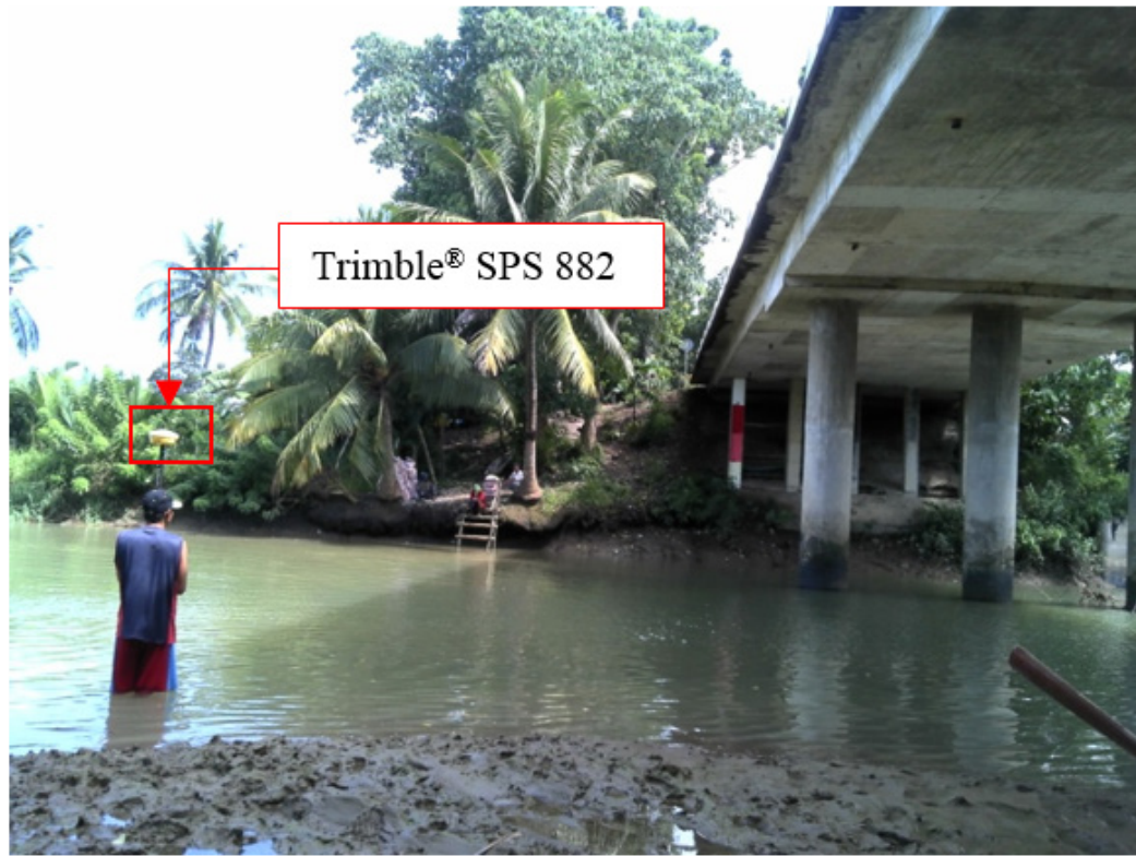
Figure 35. Cross-section survey at Danao Bridge in Escalante City
