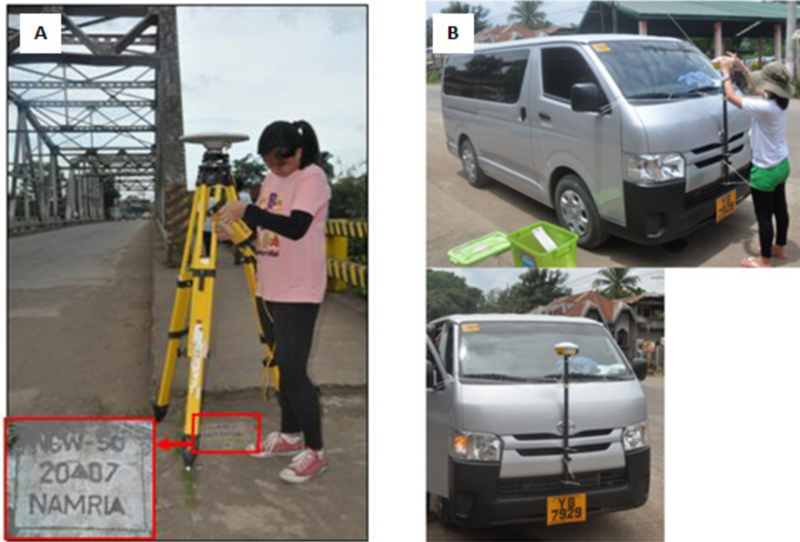
Figure 40. (A) Occupied base station, NGW-50 in Himoga-An Bridge, Sagay City and (B) Installation of GNSS Receiver Trimble® SPS882 on the van prior the conduct of ground validation points
