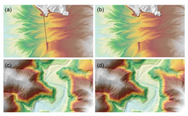
Figure 20. Portions in the DTM of Dalanas Floodplain – bridge before (a) and after (b) manual editing; and a river bank before (c) and after (d) data retrieval
