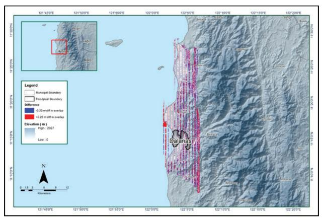
Figure 13. Elevation difference map between flight lines for Dalanas Floodplain
