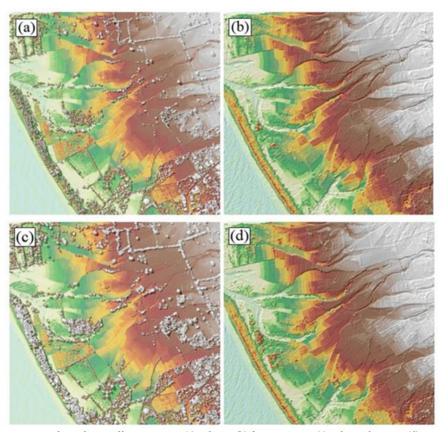
Figure 17. The production of last return DSM (a) and DTM (b), first return DSM (c) and secondary DTM (d) in some portion of Dalanas Floodplain
