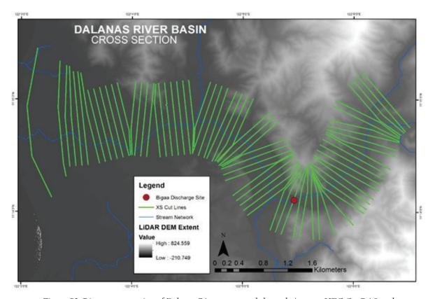
Figure 52. River cross-section of Dalanas River generated through Arcmap HEC GeoRAS tool
