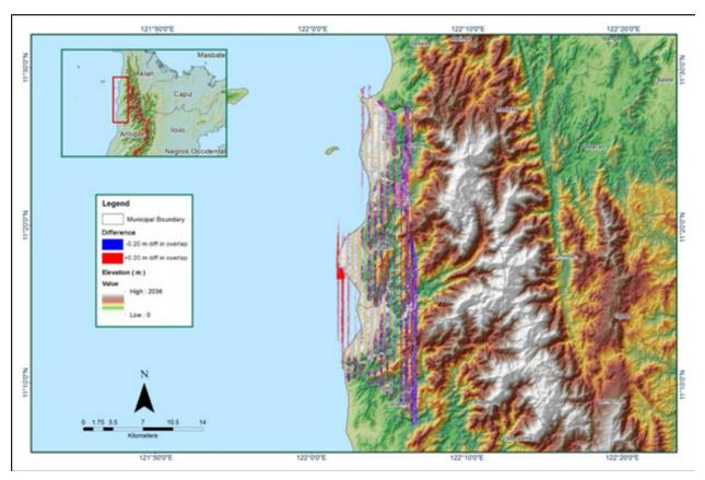
Figure-A.8.7. Elevation difference between flight lines
