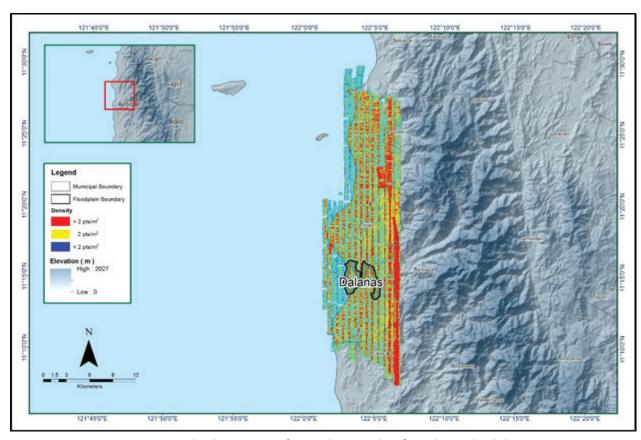
Figure 12. Pulse density map of merged LiDAR data for Dalanas Floodplain
