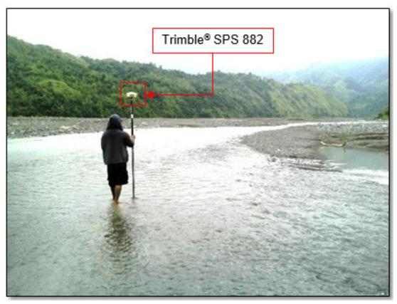
Figure 38. Bathymetric Survey along Dalanas River
