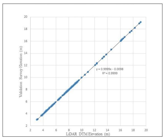
Figure 24. Correlation plot between validation survey points and LiDAR data
