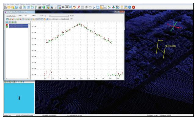
Figure 14. Quality checking for a Dalanas flight 2586G using the Profile Tool of QT Modeler
