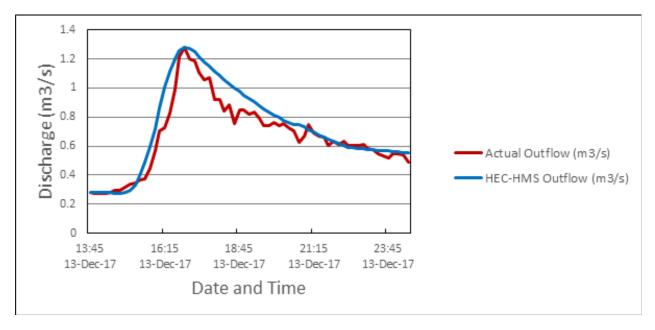
Figure 56. Outflow Hydrograph of Dalanas produced by the HEC-HMS model compared with observed outflow
