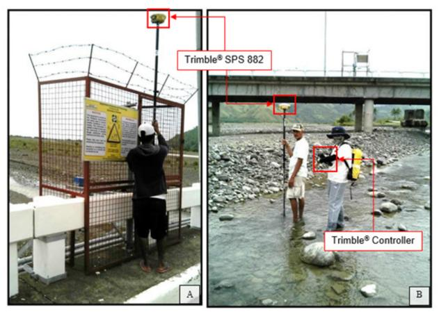
Figure 32. (A) As built survey and (B) Cross section survey in Dalanas Bridge in the Municipality of Barbaza
