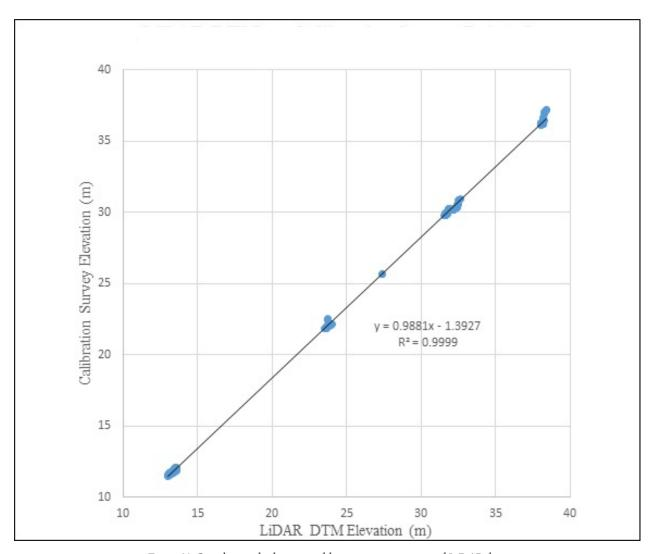
Figure 23. Correlation plot between calibration survey points and LiDAR data
