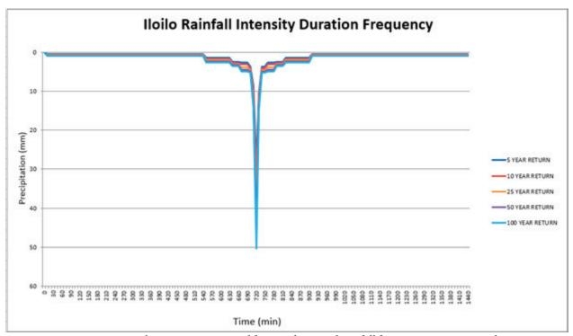
Figure 46. Synthetic storm generated for a 24-hr period rainfall for various return periods
