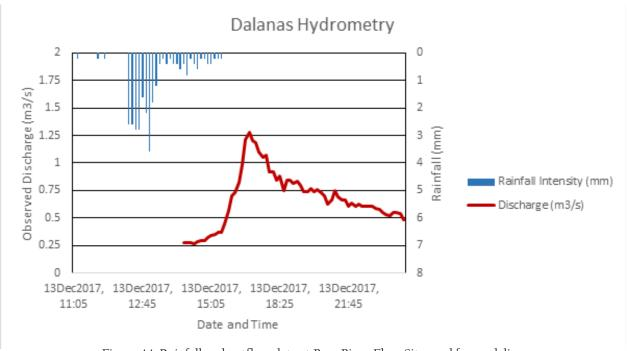
Figure 44. Rainfall and outflow data at Brgy Bigaa Flow Site used for modeling
