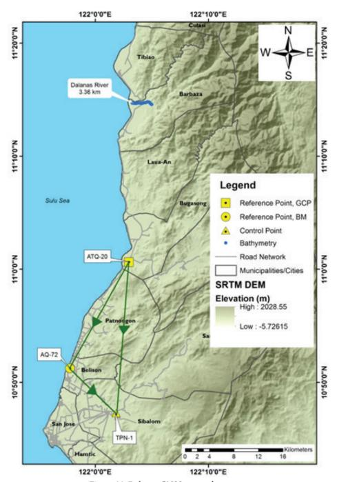
Figure 28. Dalanas GNSS network survey
