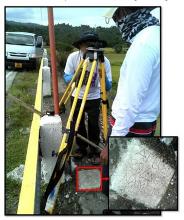
Figure 29. GNSS base receiver setup, Trimble® SPS 852 at ATQ-20 in Brgy. Zaragoza, Municipality of Bugasong, Antique
