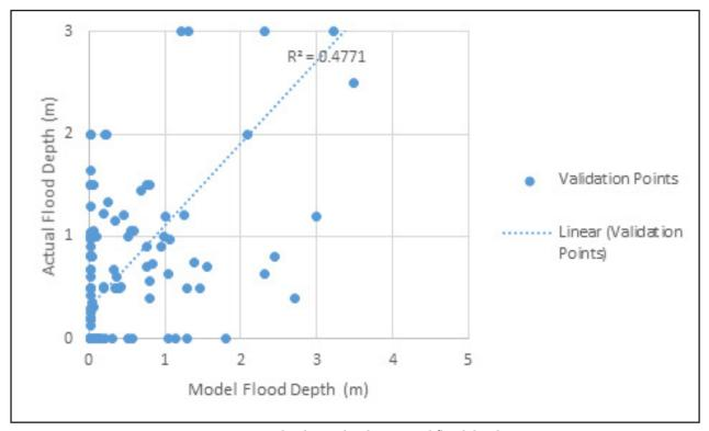
Figure 102. Flood map depth vs. actual flood depth
