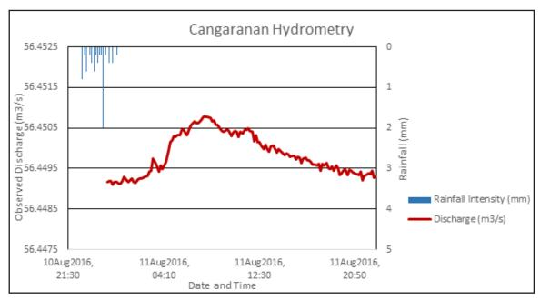
Figure 53. Rainfall and outflow data of the Cangaranan River Basin, which was used for modeling
