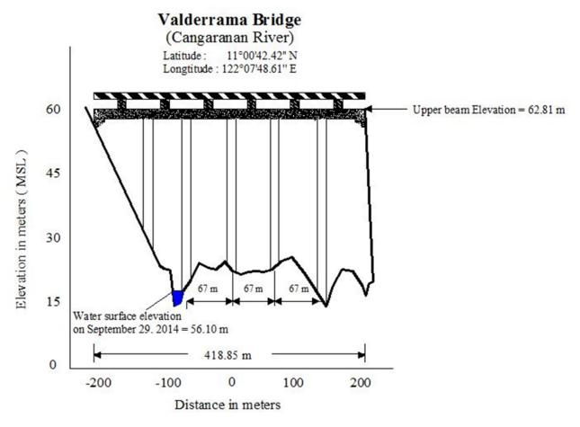
Figure 41. Valderrama Bridge cross section diagram
