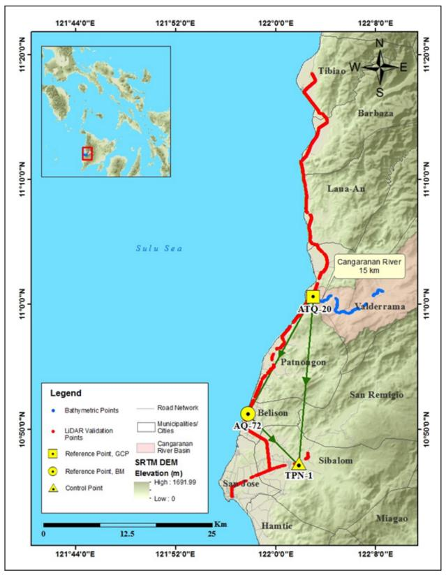
Figure 32. Extent of the bathymetric survey (in blue line) in the Cangaranan River and the LiDAR data validation survey (in red)
