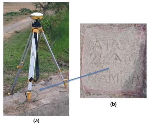
Figure 6 . (a) GPS set-up over ATQ-22 in Barangay Concepcion, Belison, Province of Antique; and (b) NAMRIA reference point ATQ-22, as recovered by the field team
