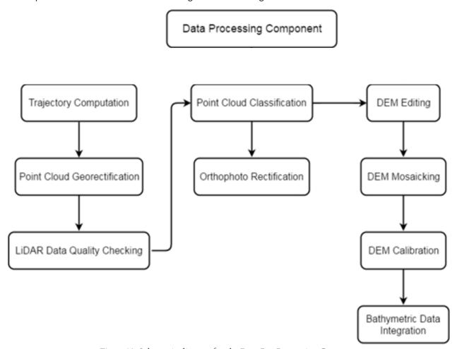
Figure 10. Schematic diagram for the Data Pre-Processing Component
