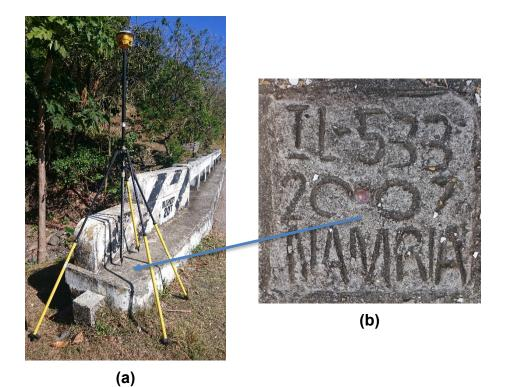
Figure 7. (a) GPS set-up over IL-533 in Barangay Amboyu-an, San Joaquin, Province of Iloilo; and (b) NAMRIA reference point IL-533, as recovered by the field team
