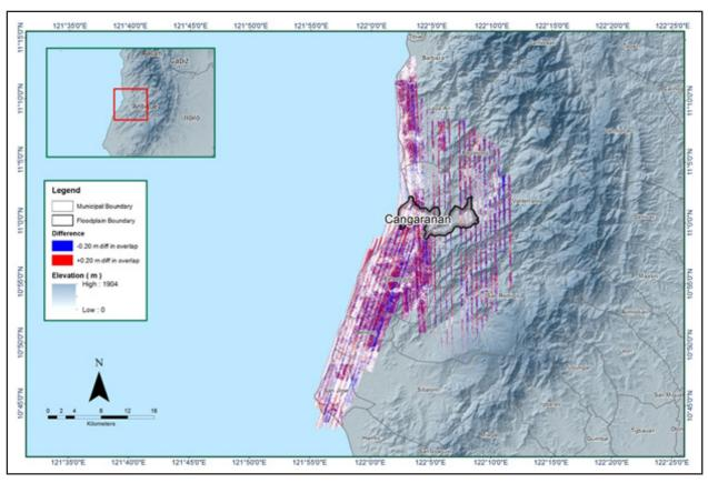
Figure 17. Elevation difference map between flight lines for the Cangaranan Floodplain
