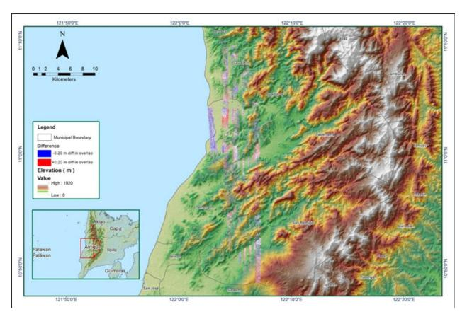
Figure A-8.14. Elevation difference between flight lines
