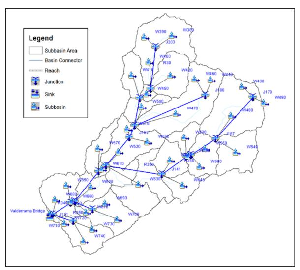
Figure 60. The Cangaranan River Basin model, generated using HEC-HMS
