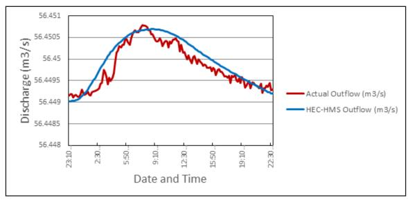
Figure 65. Outflow Hydrograph of Cangaranan produced by the HEC-HMS model, compared with observed outflow
