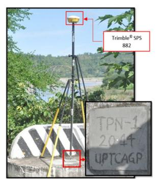
Figure 36. UP-TCAGP-established control point, TPN-1, with Trimble® SPS 882, on the Tipuluan Bridge in Barangay Pasong, Municipality of Sibalom, Antique
