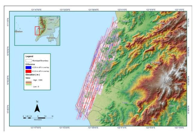
Figure A-8.28. Elevation difference between flight lines
