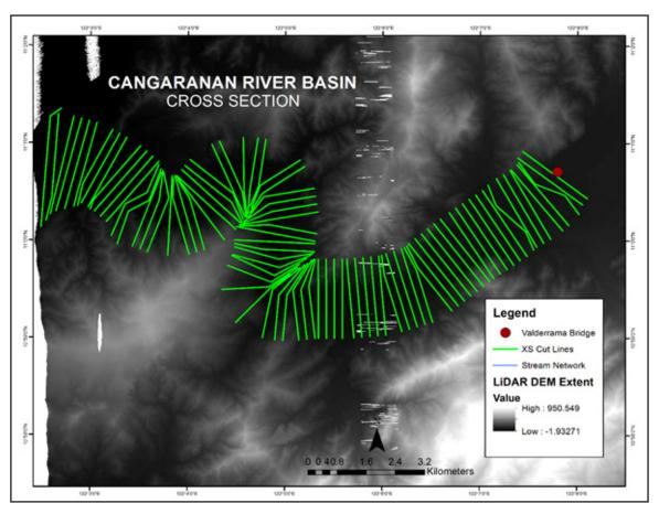
Figure 61. River cross-section of the Cangaranan River, generated through ArcMap HEC GeoRAS tool
