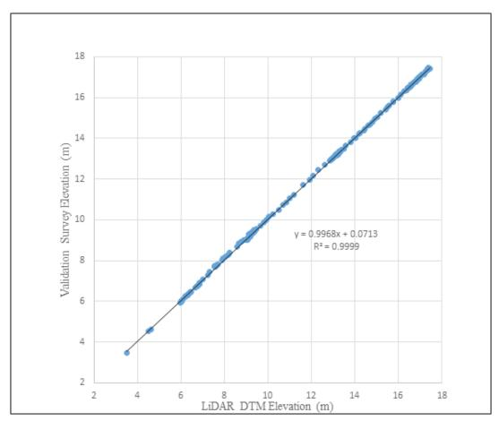
Figure 28. Correlation plot between the validation survey points and the LiDAR data
