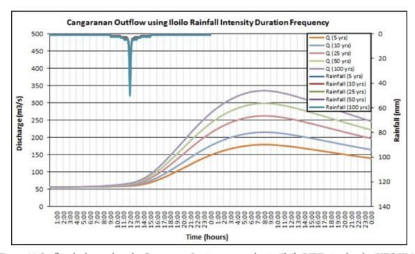
Figure 66. Outflow hydrograph at the Cangaranan Station generated using Iloilo RIDF, simulated in HEC-HMS
