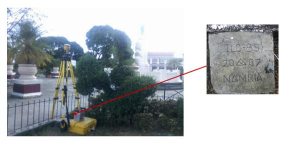
Figure 3. (a) GCP set-up over ILO-85, located at the Town Plaza in Miag-ao, Iloilo; and (b) NAMRIA reference point ILO-85, as recovered by the field team
