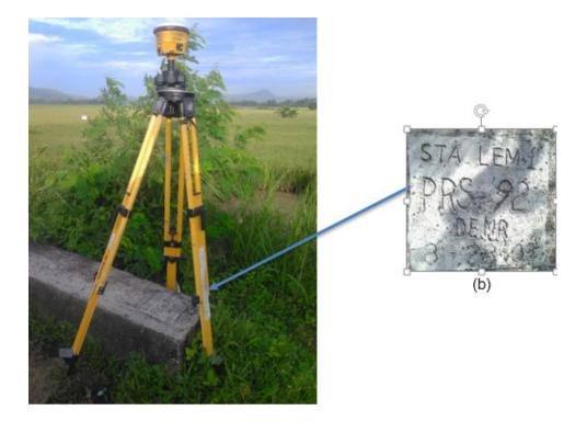
Figure 6. GCP set-up over ILO-97 as located in Brgy. Tabunan, Municipality of Lemery situated in an irrigation canal near the national road (a) and NAMRIA reference point ILO-97 (b) as recovered by the field team
