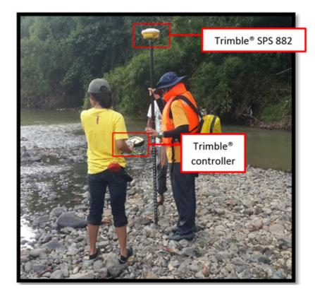
Figure 48. Manual Bathymetry using PPK Survey
