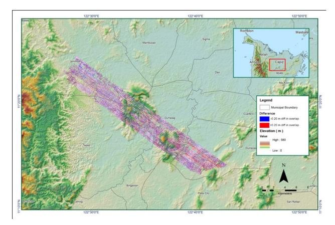
Figure A-8.70. Elevation difference between flight lines
