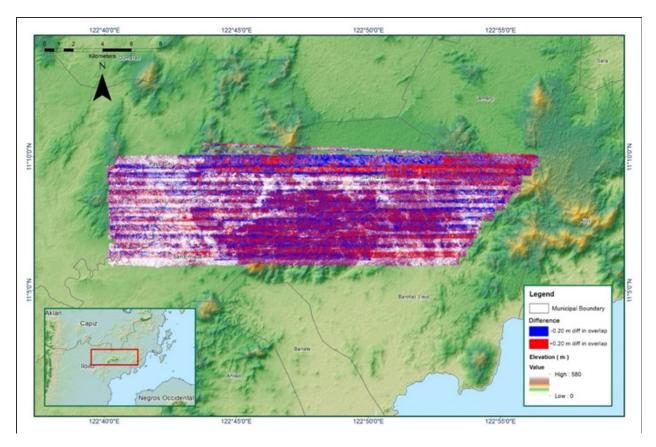
Figure A-8.7. Elevation difference between flight lines
