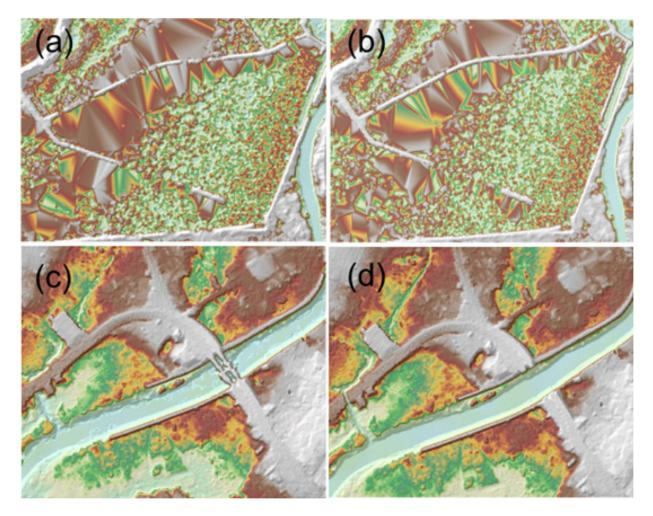
Figure 23. Portions in the DTM of Barotac floodplain – a paddy field before (a) and after (b) data retrieval; bridges before (c) and after (d) manual editing
