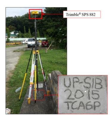
Figure 35. Trimble® SPS 882 setup at UP-SIB located at Sibalom Bridge, Brgy. Anonang, Leon, Iloilo
