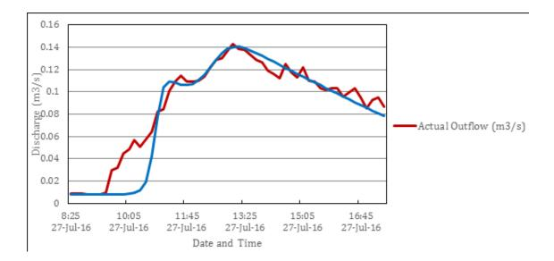
Figure 66. Outflow Hydrograph of Barotac produced by the HEC-HMS model compared with observed outflow
