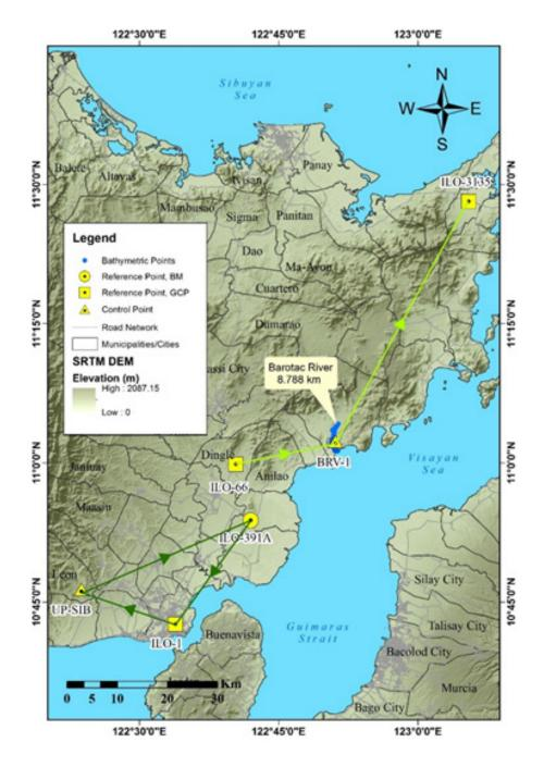
Figure 32. GNSS Network of Barotac River Field Survey.
