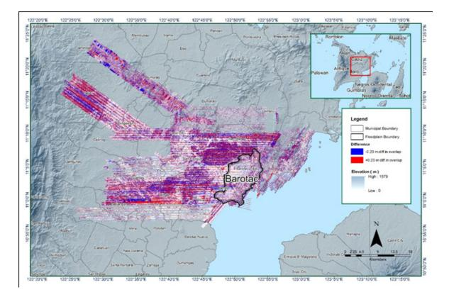
Figure 16. Elevation difference map between flight lines for Barotac floodplain
