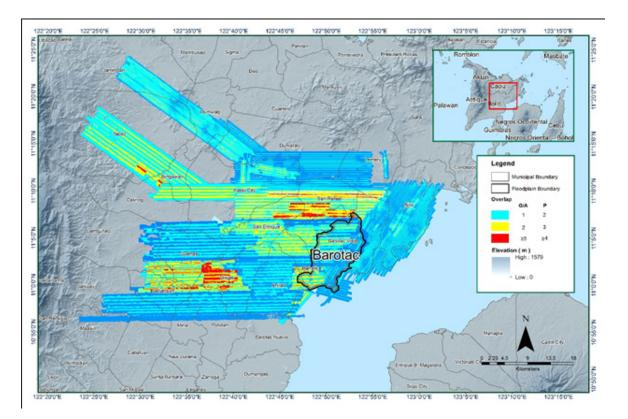
Figure 14. Image of data overlap for Barotac Floodplain
