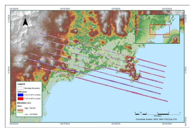
Figure A-8.77. Elevation difference between flight lines
