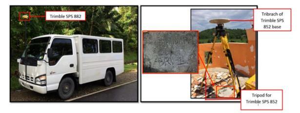
Figure 45. (A) Set-up of Trimble® SPS 882 attached to a vehicle and (B) Setting up of GNSS base station at BRV-1
