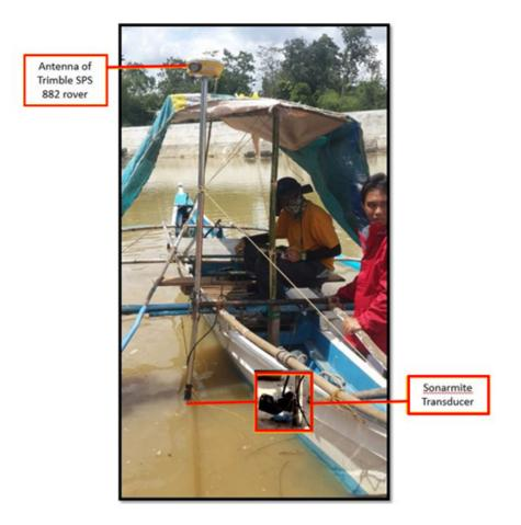
Figure 47. Bathymetric survey using OHMEXTM echo sounder
