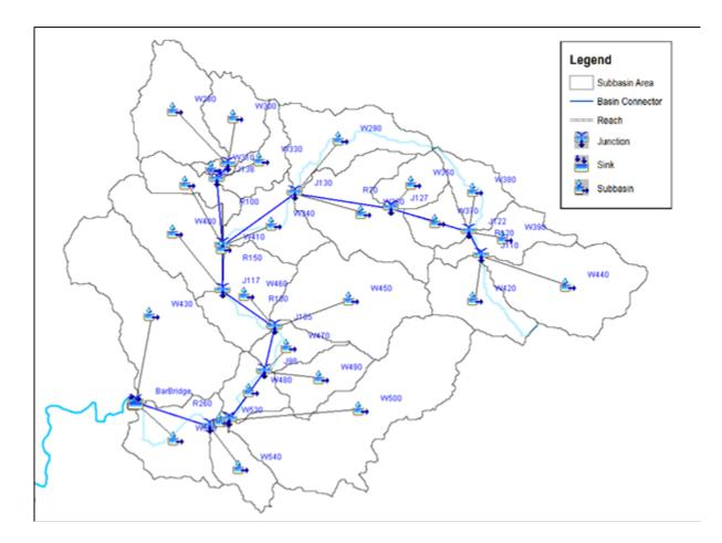
Figure 61. The Barotac river basin model generated using HEC-HMS
