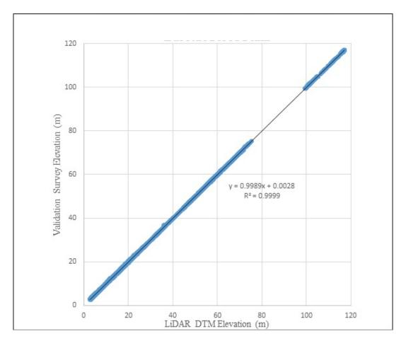
Figure 27. Correlation plot between validation survey points and LiDAR data
