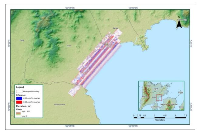
Figure A-8.21. Elevation difference between flight lines
