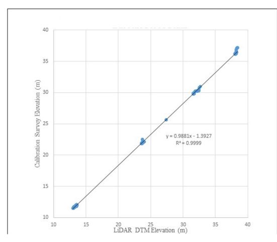
Figure 26. Correlation plot between calibration survey points and LiDAR data
