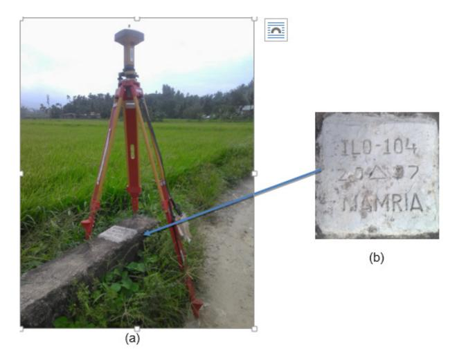
Figure 7. GCP set-up over ILO-104 in Brgy. Poblacion, Municipality of Ajuy situated in an irrigation canal near Ajuy High School (a) and NAMRIA reference point ILO-104 (b) as recovered by the field team
