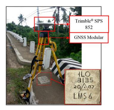
Figure 37. Trimble® SPS 852 setup at ILO-3135 located in Balasan Bridge, Brgy. Poblacion Sur, Municipality of Balasan, Iloilo
