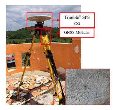
Figure 36. Trimble® SPS 852 setup at BRV-1 located in the rooftop of Hollywood Star Inn, Brgy. Poblacion, Municipality of Barotac Viejo, Iloilo
