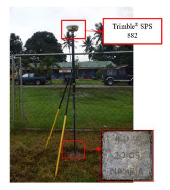
Figure 38. Trimble® SPS 882 setup at ILO-66, located inside Dingle Elementary School, Brgy. Camambugan, Municipality of Dingle, Iloilo
