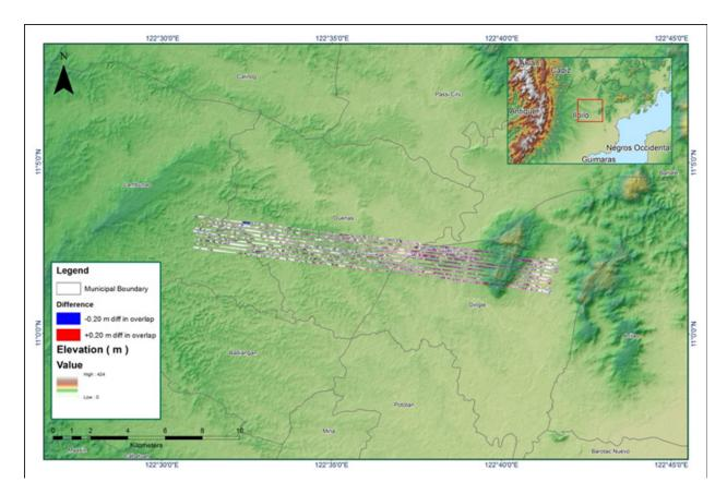
Figure A-8.91. Elevation difference between flight lines
