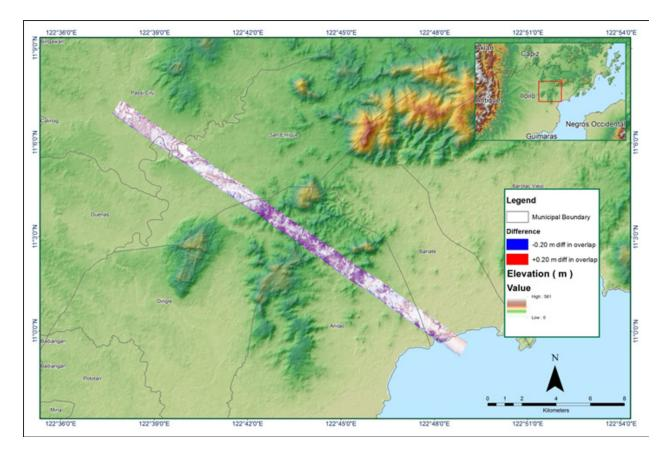
Figure A-8.14. Elevation difference between flight lines
