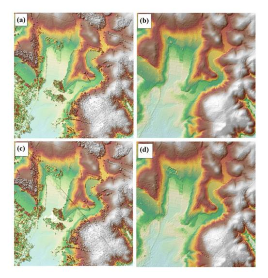
Figure 20. The production of last return DSM (a) and DTM (b), first return DSM (c) and secondary DTM (d) in some portion of Barotac Floodplain
