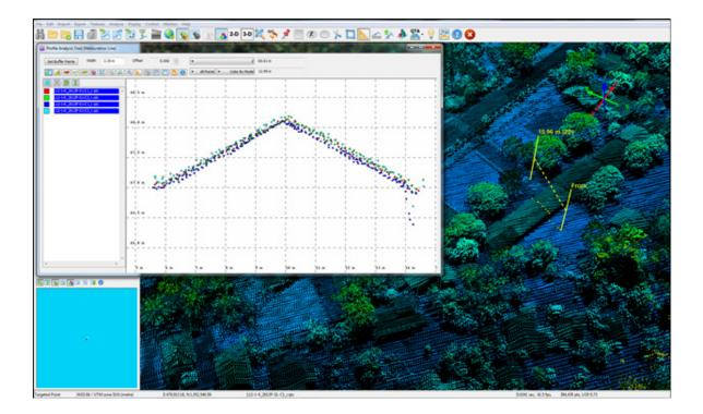
Figure 17. Quality checking for a Barotac flight 2613P using the Profile Tool of QT Modeler.
