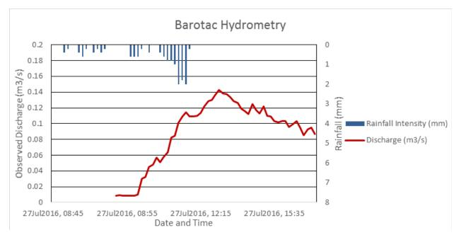
Figure 54. Rainfall and outflow data at Barotac used for modeling
