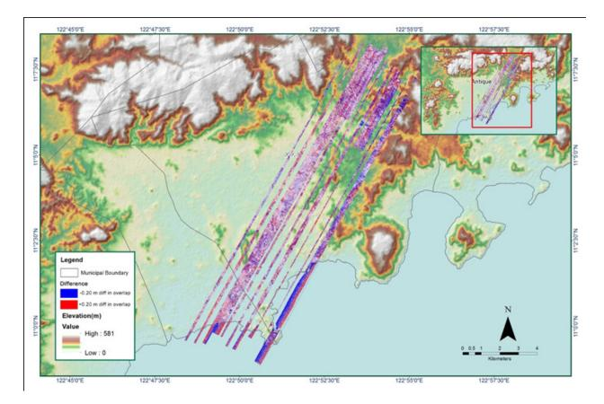
Figure A-8.84. Elevation difference between flight lines
