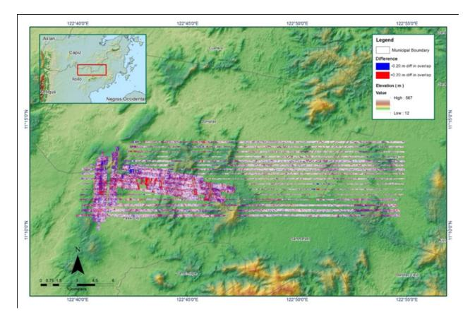
Figure A-8.28. Elevation difference between flight lines
