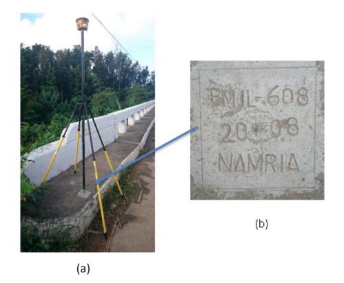
Figure 4. GPS set-up overIL-608 in San Rafael, Province of Iloilo (a) and NAMRIA reference point IL-608 (b) as recovered by the field team
