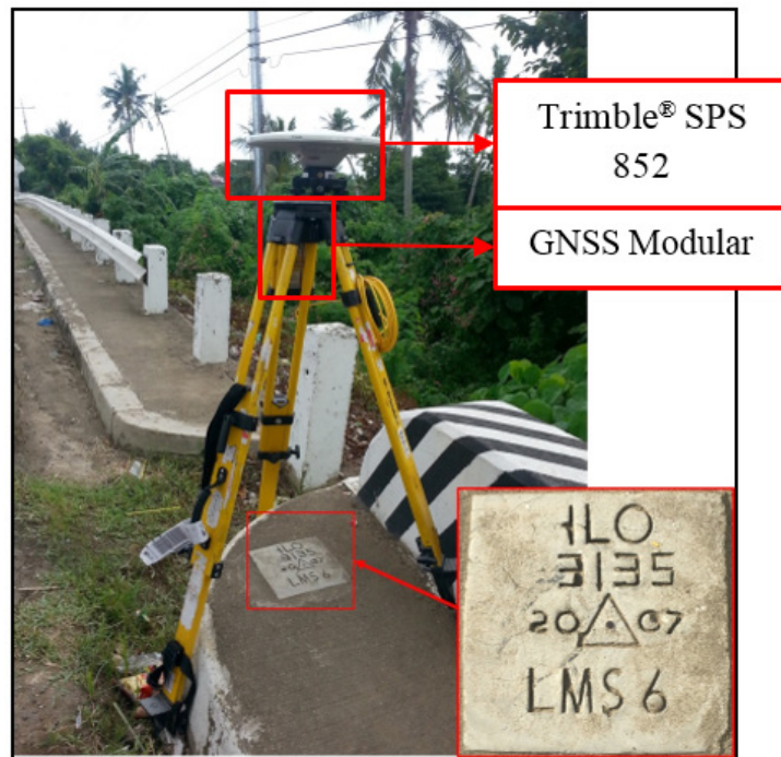
Figure 36. Trimble® SPS 852 set-up at ILO-3135, located at the Balasan Bridge in Barangay Poblacion Sur, Municipality of Balasan, Iloilo
