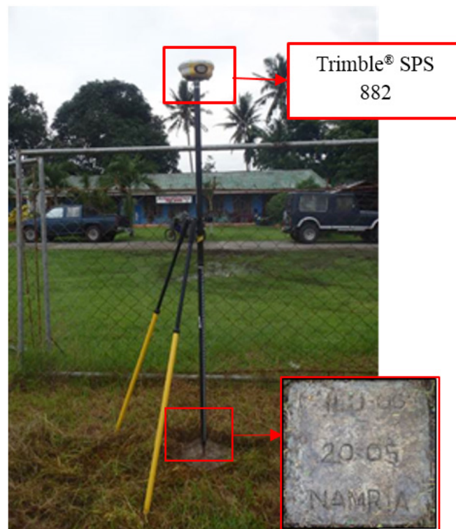
Figure 37. Trimble® SPS 882 set-up at ILO-66, located inside Dingle Elementary School, Barangay Camambugan, Municipality of Dingle, Iloilo
