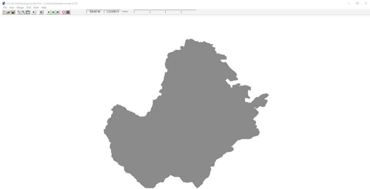
Figure 60. Screenshot of a sub-catchment with the computational area to be modeled in FLO-2D Grid Developer System Pro (FLO-2D GDS Pro)
