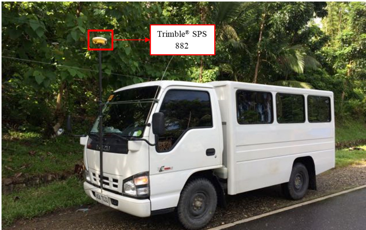
Figure 43. Validation points acquisition set-up for the Balantian River Basin
