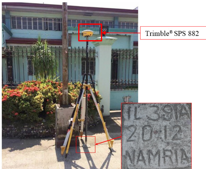
Figure 33. Trimble® SPS 882 set-up at IL-39A, located in Barangay JT Bretaña, Municipality of Barotac Nuevo, Iloilo
