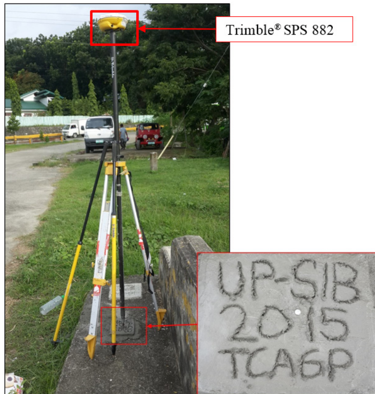
Figure 34. Trimble® SPS 882 set-up at UP-SIB located at the Sibalom Bridge in Barangay Anonang, Leon, Iloilo
