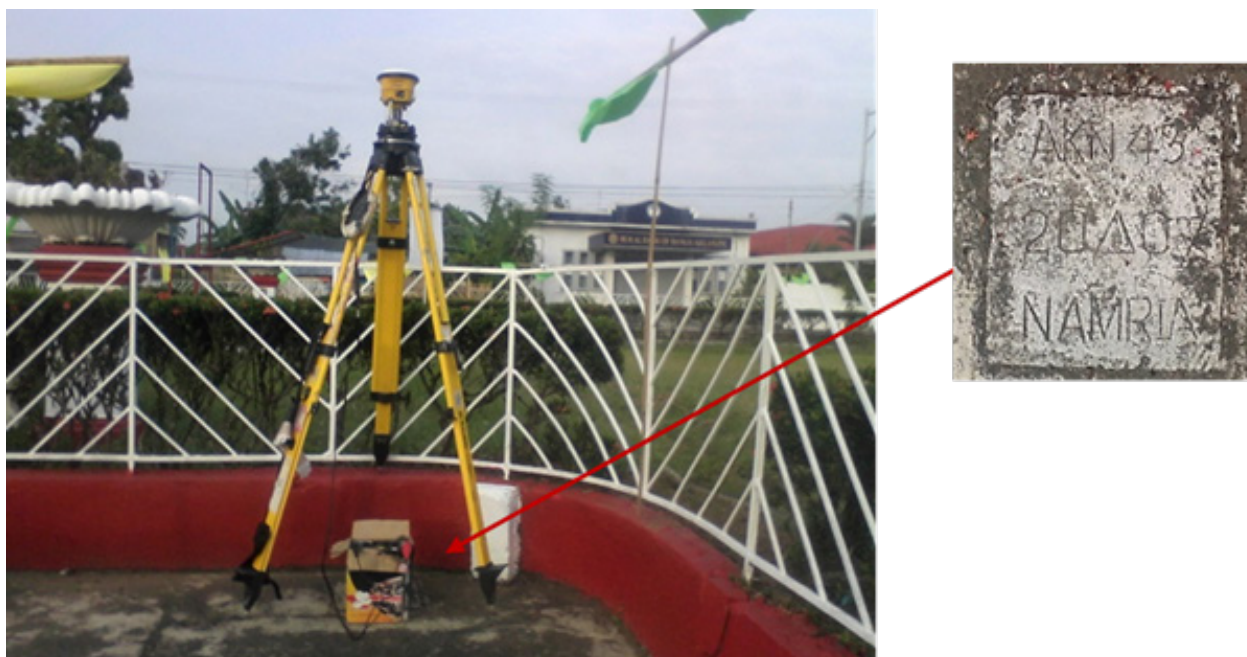
Figure 4. GPS set-up over AKN-43 located on the concrete sidewalk in front of the municipal hall of Banga, Aklan, and NAMRIA reference point AKN-43 (b) as recovered by the field team.
