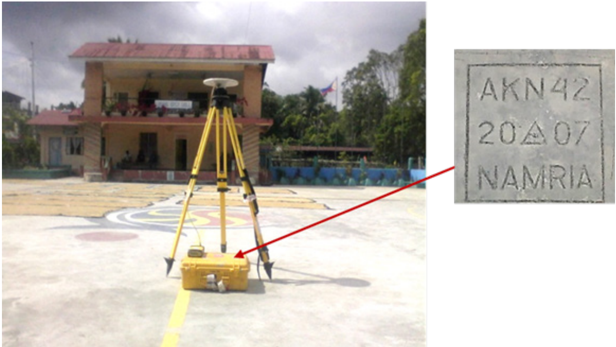
Figure 5. GPS set up over AKN-42 at the open court in Barangay Libang, Makato, Aklan (a) and NAMRIA reference point AKN-42 (b) as recovered by the field team.
