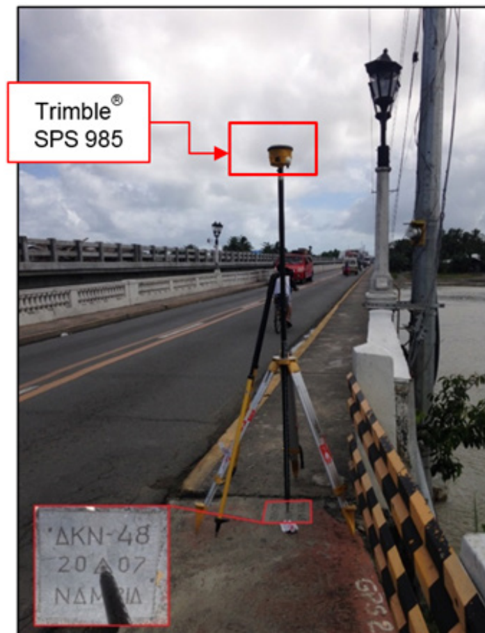
Figure 37. Trimble® SPS 985 GNSS receiver occupation at AKN-48 in Kalibo Bridge, Brgy. Poblacion, Municipality of Kalibo
