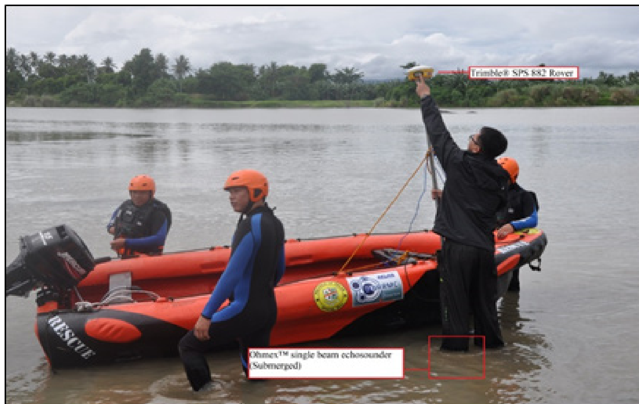
Figure 45. OHMEX™ single beam echosounder set up on a boat for Aklan River bathymetric survey
