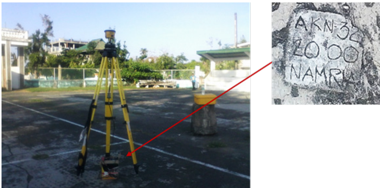
Figure 6. GPS set up over AKN-32 located at the centerpoint of Batan Multi-purpose Sports Center, (a) and NAMRIA reference point AKN-32 (b) as recovered by the field team.
