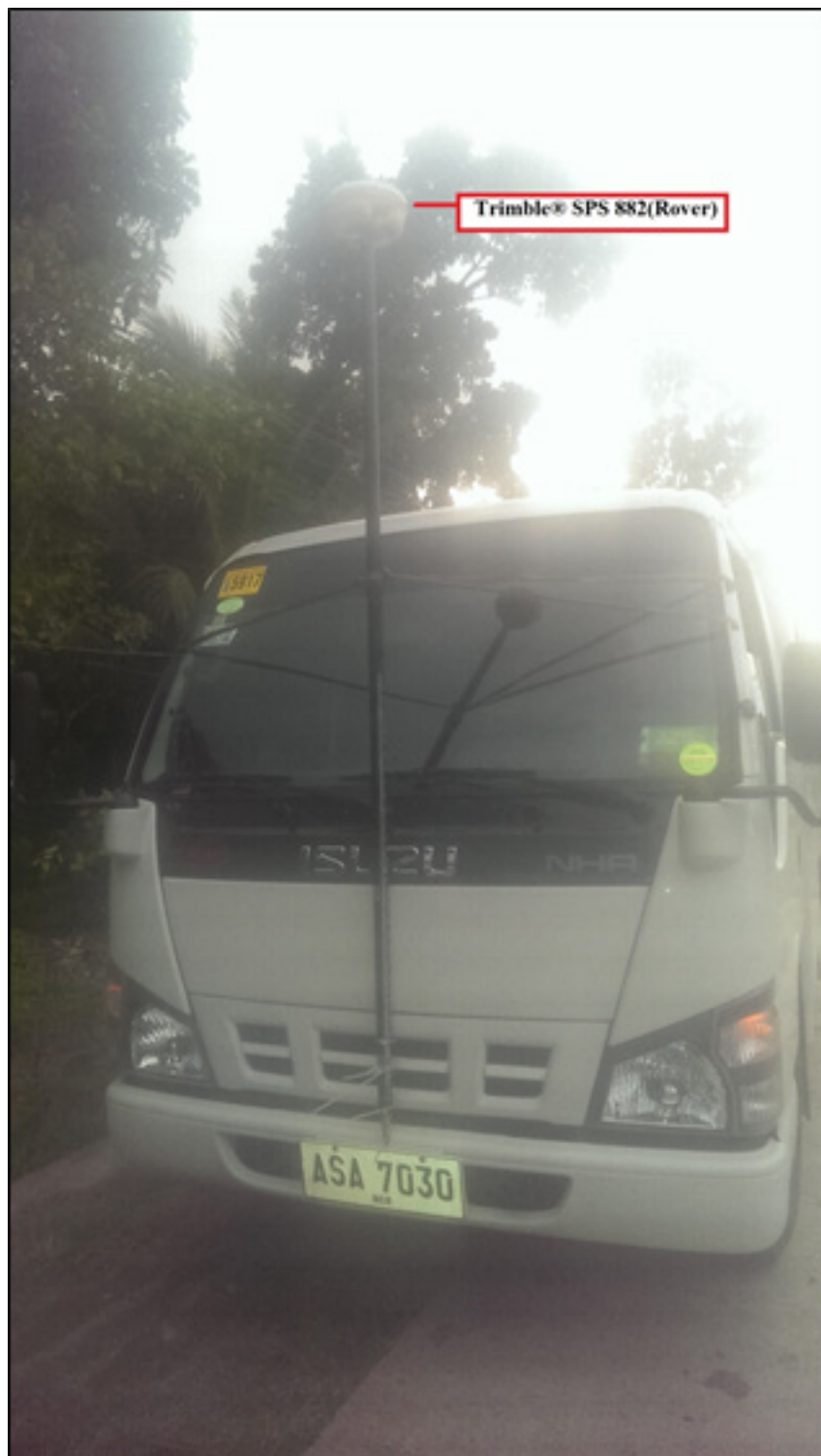
Figure 43. Validation points acquisition survey set-up
