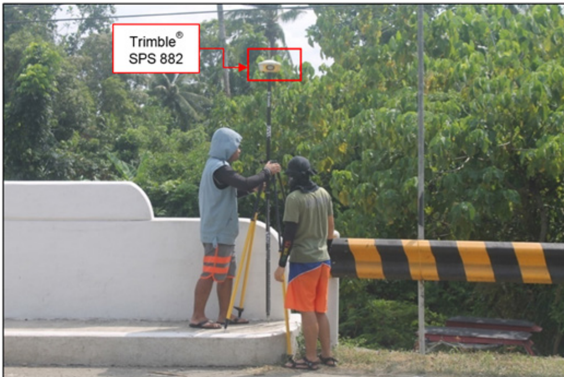
Figure 35. Trimble® SPS 882 GNSS receiver setup at AK-173, Dumga Bridge, Brgy. Dumga, Municipality of Makato
