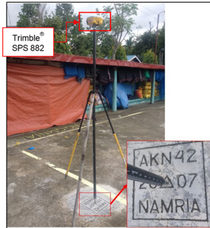
Figure 36. Trimble® SPS 882 GNSS receiver setup at AKN-42 inside a basketball court in Brgy. Libang, Municipality of Makato
