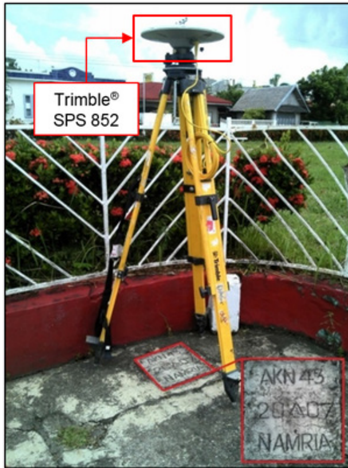
Figure 34. Trimble® SPS 852 GNSS receiver base station at AKN-43 in front of Banga Municipal Hall, Brgy. Poblacoin, Municipality of Banga
