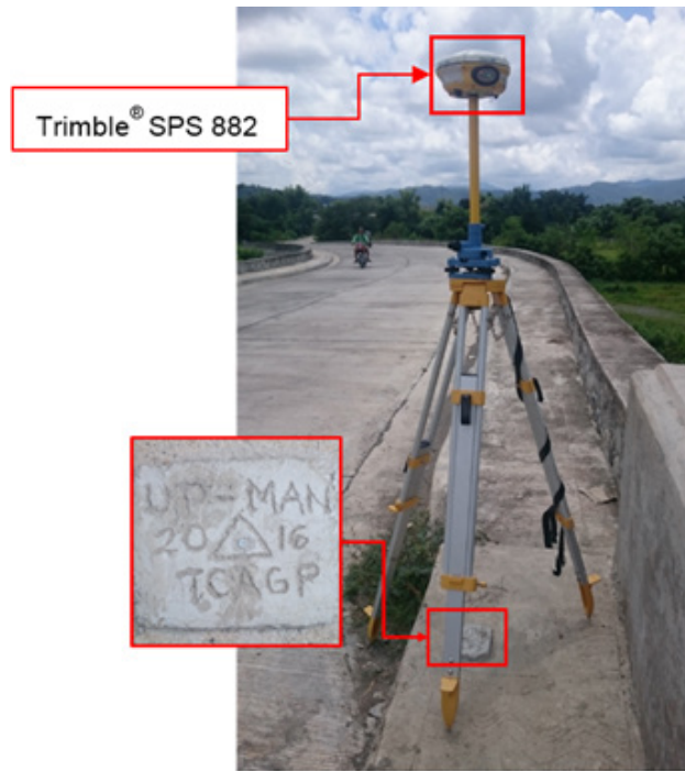
Figure 35. GNSS receiver setup, Trimble® SPS 882, at UP-MAN located at the approach of Manabo Bridge in Brgy. San Juan Norte, Municipality of Manabo, Abra.
