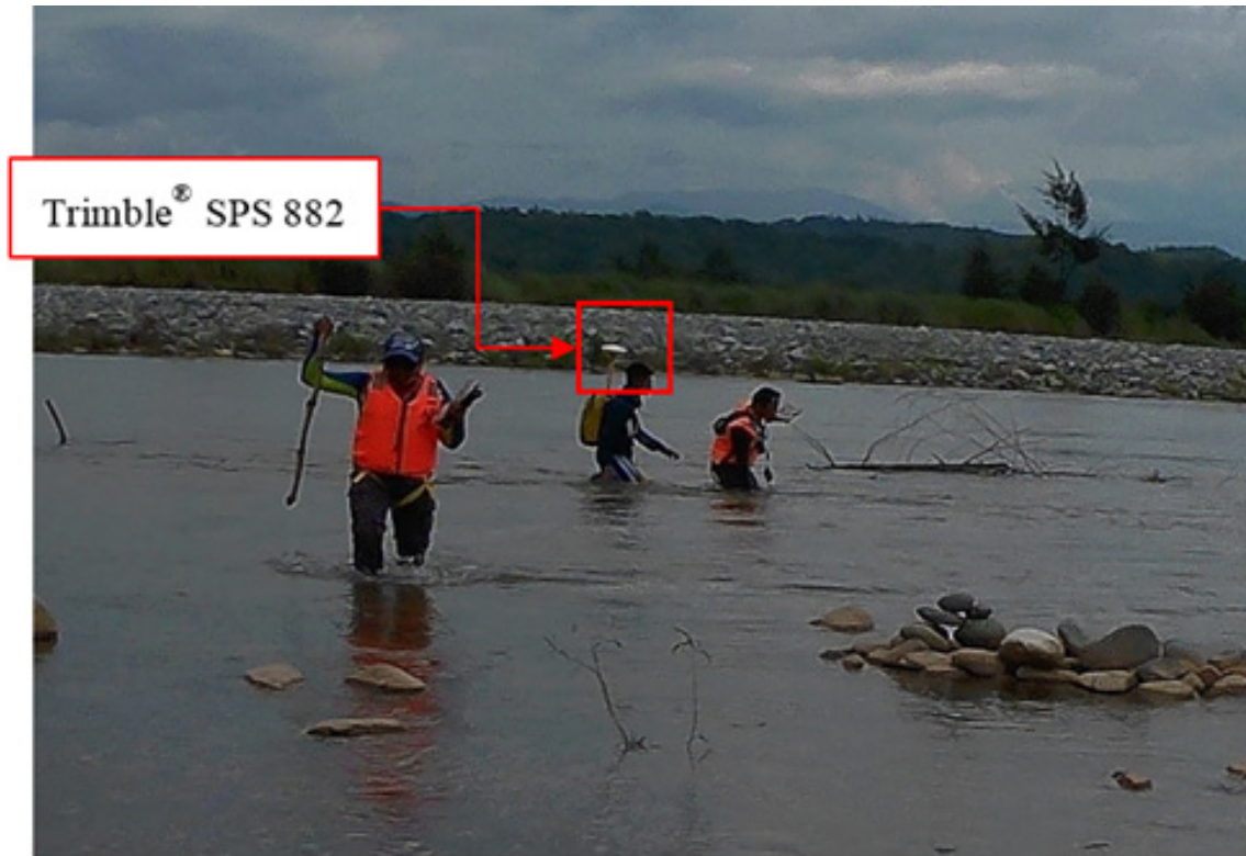
Figure 45. Set-up for the manual bathymetric survey.
