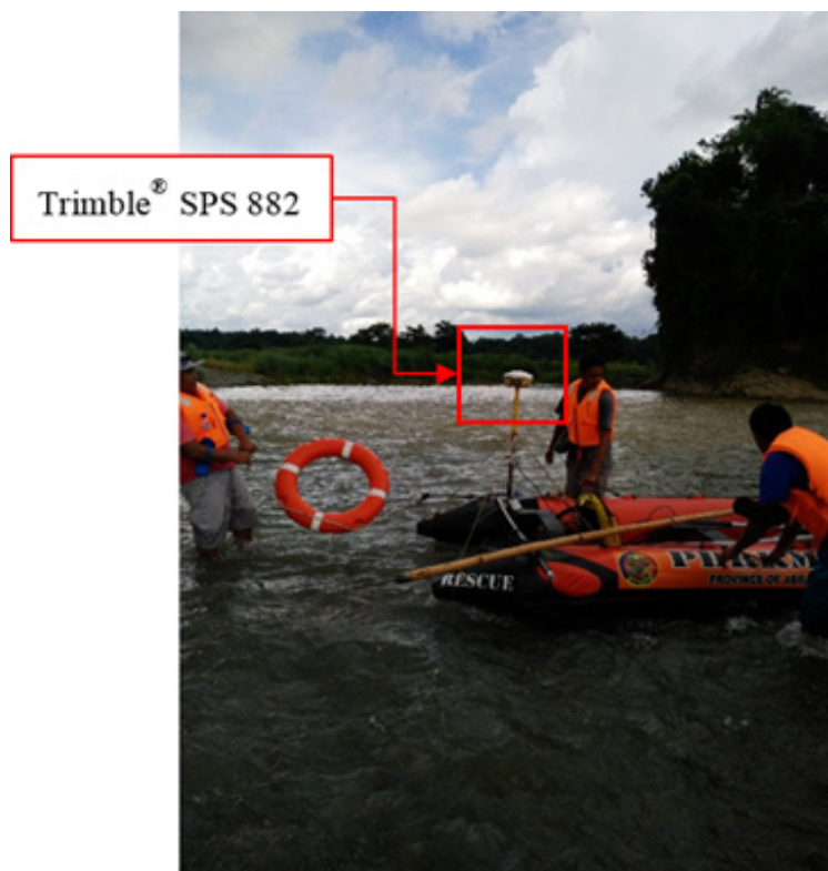
Figure 44. Set up of the bathymetric survey at Tineg River using Ohmex™ single beam echo sounder.
