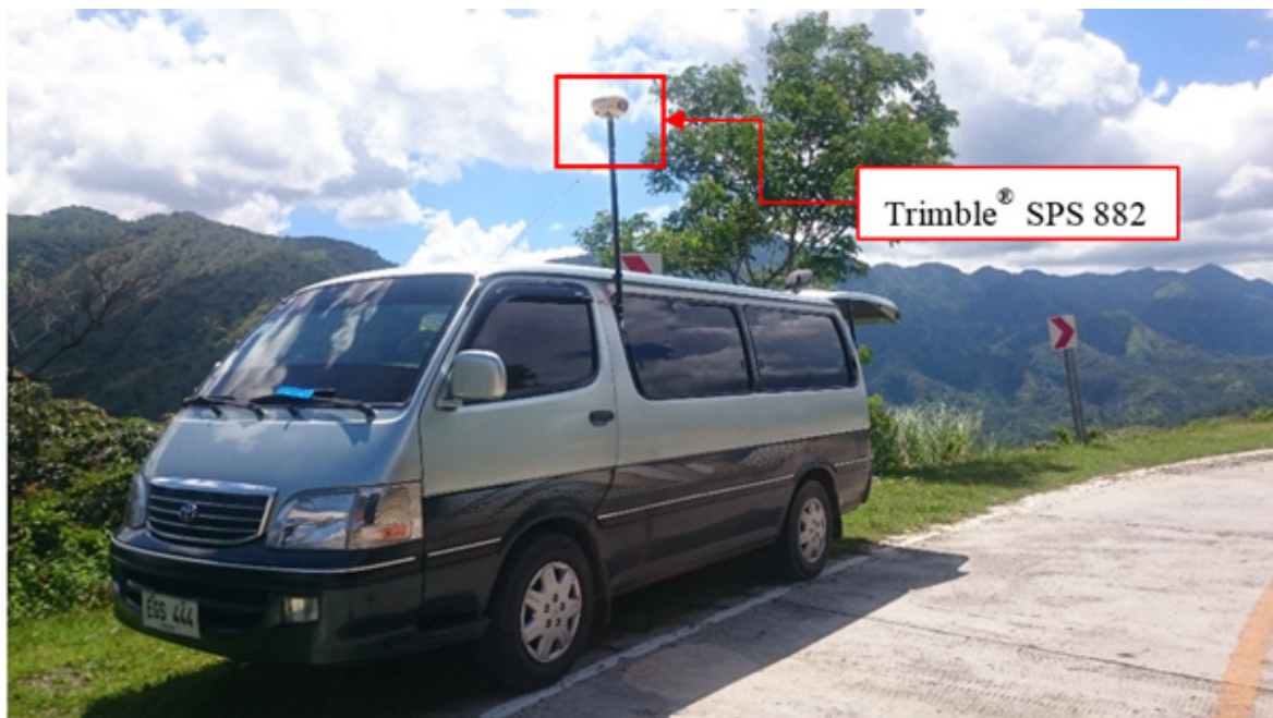
Figure 42. GNSS Receiver Trimble® SPS 882 installed on a vehicle for Ground Validation Survey.
