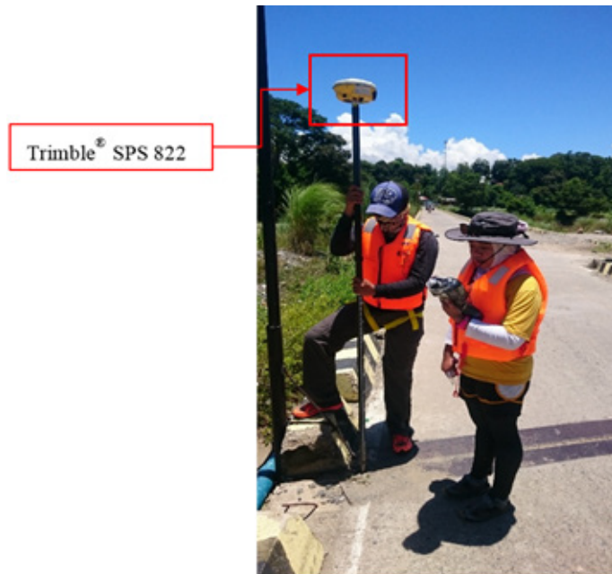
Figure 37. Bridge As-Built Survey using PPK Technique.
