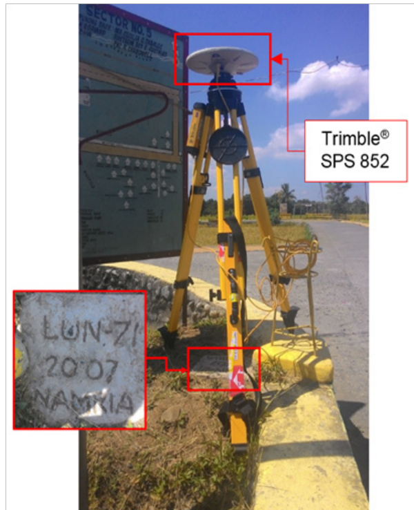
Figure 33. GNSS base set up, Trimble® SPS 852, at LUN-71, situated beside the irrigation canal at the right intersection of barangay roads, in Brgy. General Prim West, Municipality of Sudipen, La Union
