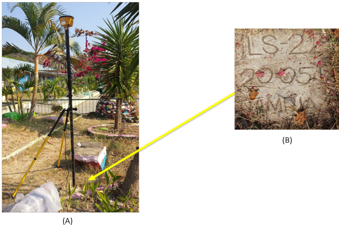
Figure 7. GPS set-up over ILS-22 as recovered inside Lidlidda North Central School in Lidlidda, Ilocos Sur (a) and NAMRIA reference point ILS-22 (b) as recovered by the field team.
