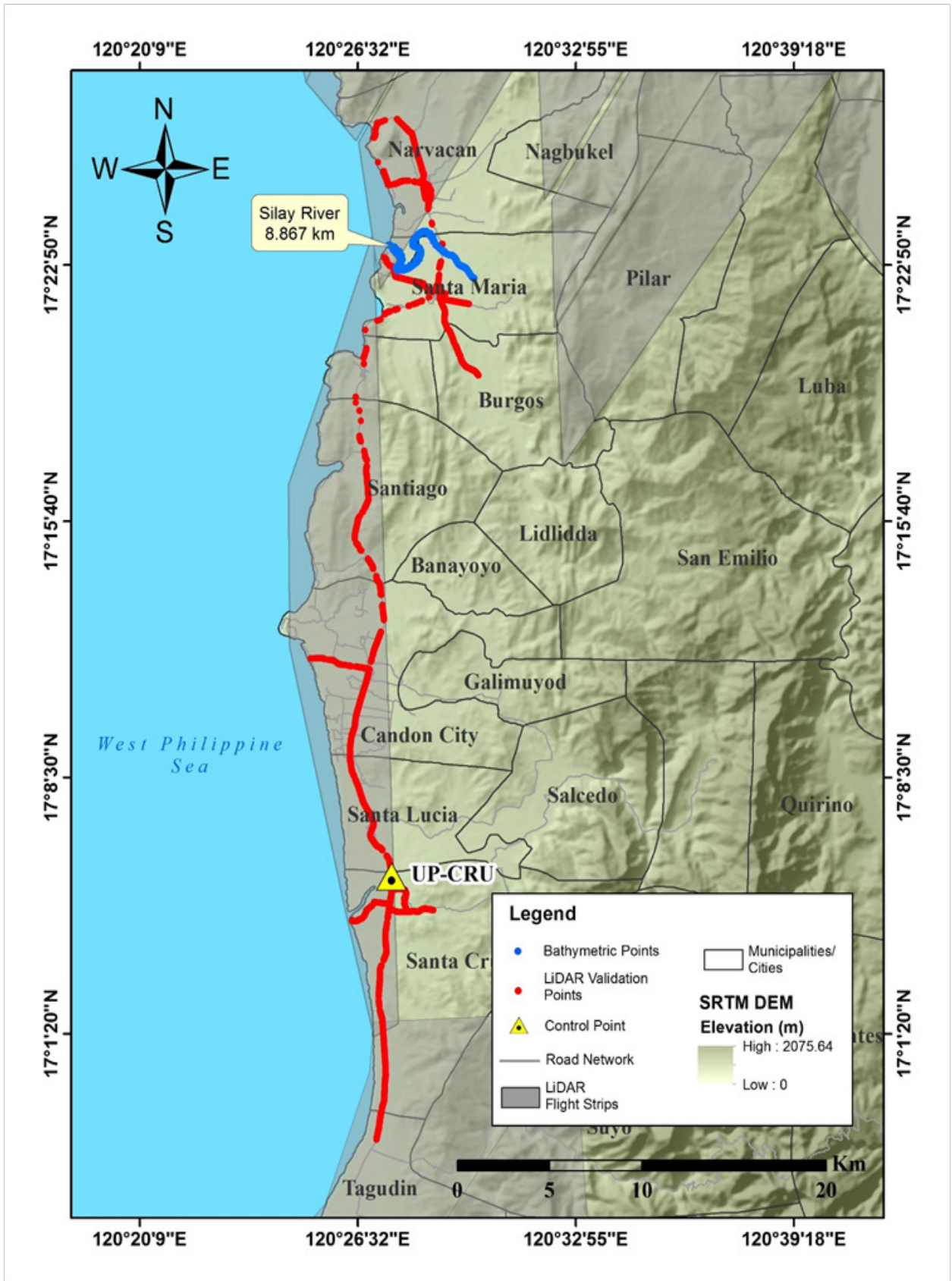
Figure 49. Validation point acquisition survey of Silay River basin
