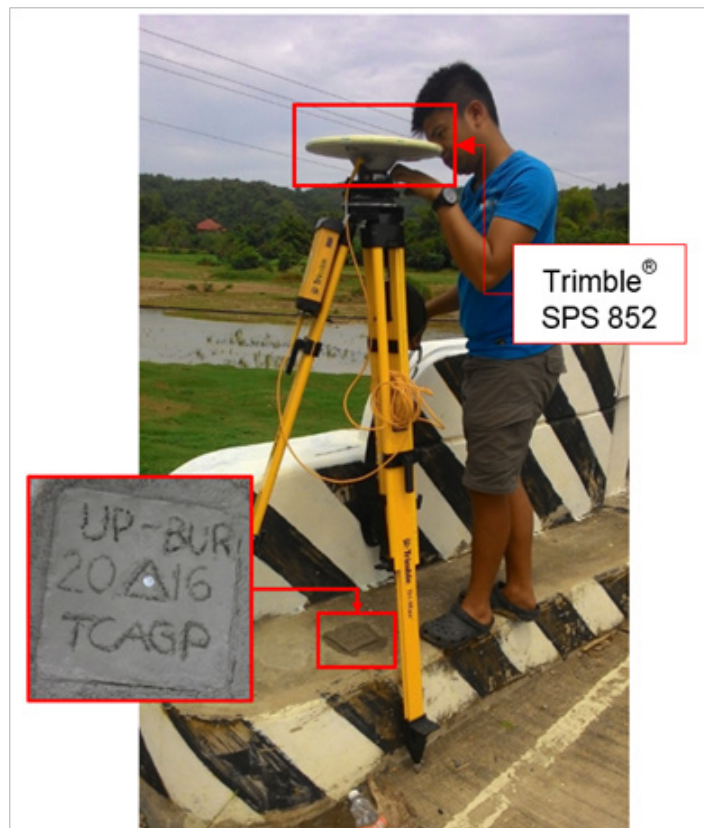
Figure 35. GNSS receiver setup, Trimble® SPS 852, at UP-BUR, located at the approach of Burgos Bridge, in Brgy. Poblacion Norte, Municipality of Burgos, Ilocos Sur
