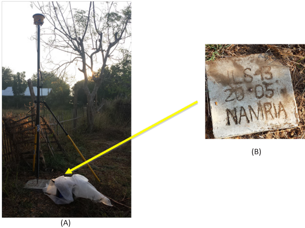
Figure 6. GPS set-up over ILS-13 located beside the school oval of Cabugao South Central School in Barangay Bonifacio, Cabugao Ilocos Sur (a) and NAMRIA reference point ILS-13 (b) as recovered by the field team.
