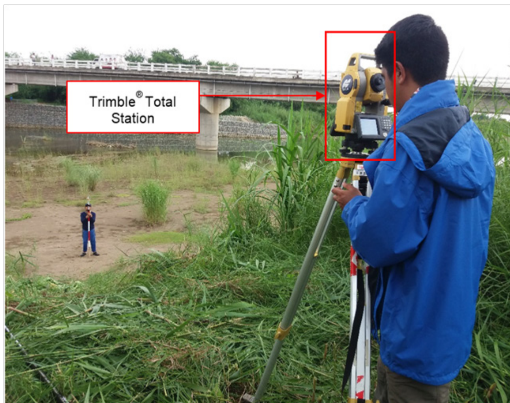
Figure 40. Cross section Survey of Santa Maria Bridge using Total Station
