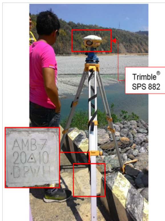
Figure 34. GNSS receiver setup, Trimble® SPS 882, at AMB-7, located at the approach of Alilem Bridge, in Brgy. Kiat, Municipality of Alilem, Ilocos Sur
