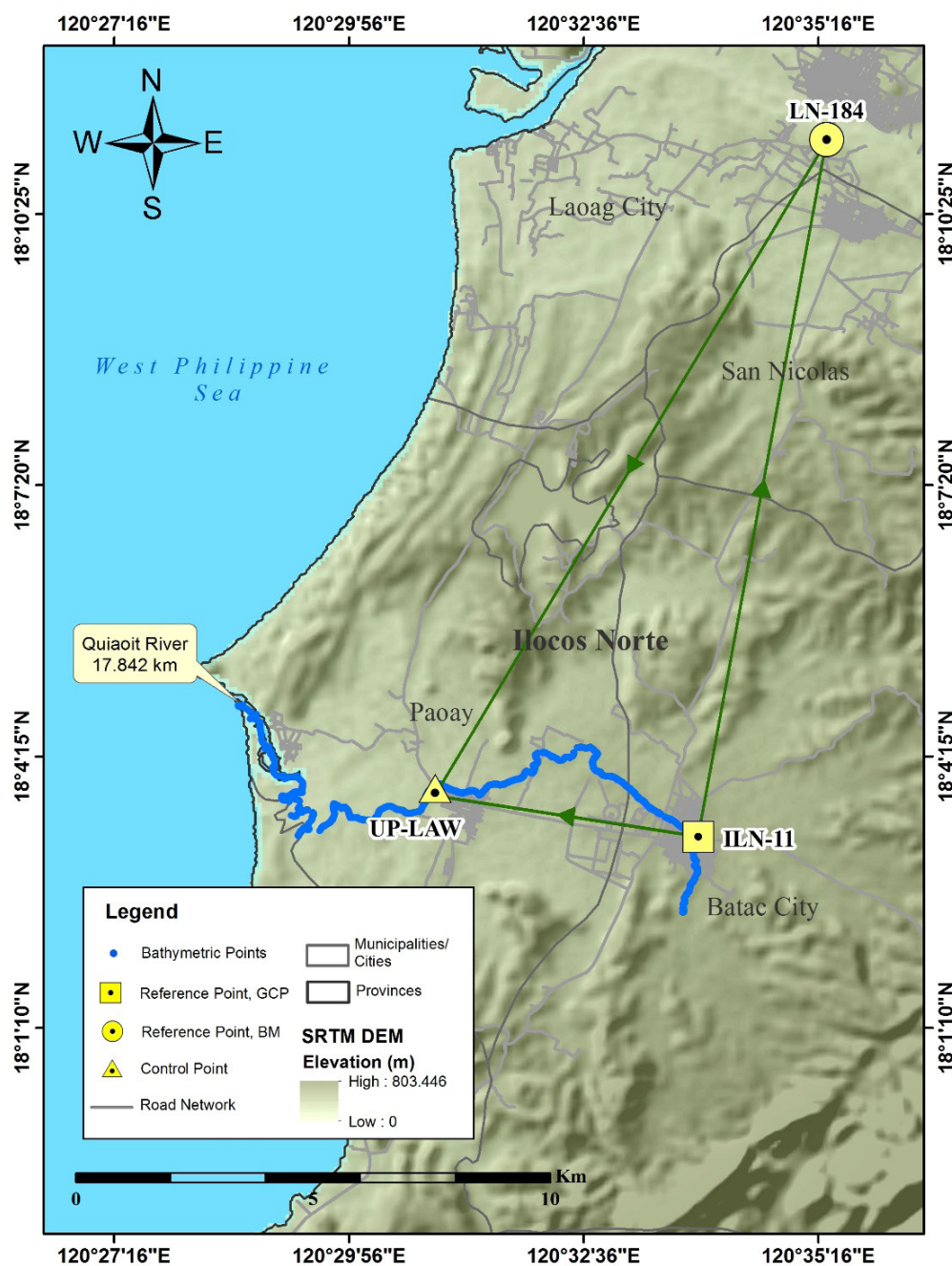
Figure 27. GNSS network covering Quiaoit River
