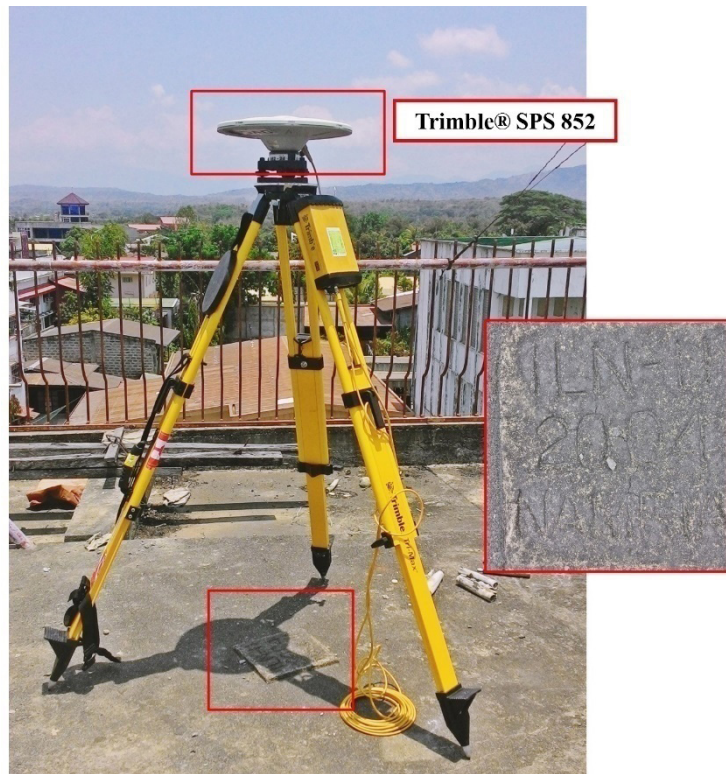
Figure 28. GNSS base set-up, Trimble® SPS 852, at ILN-11, located on the roof top of Batac City Hall in Brgy. San Roque, Batac City, Ilocos Sur
