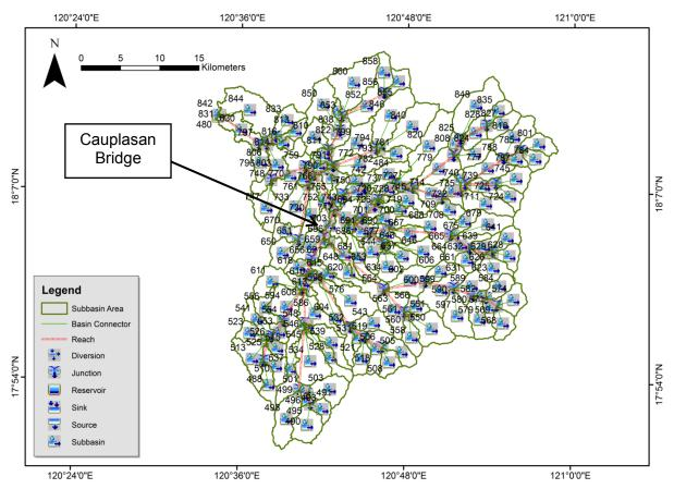
Figure 55. The Laoag river basin model generated using HEC-HMS.
