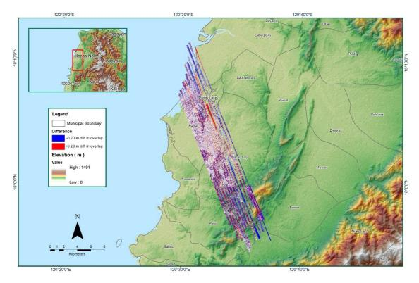
Figure 1.11.7. Elevation difference between flight lines
