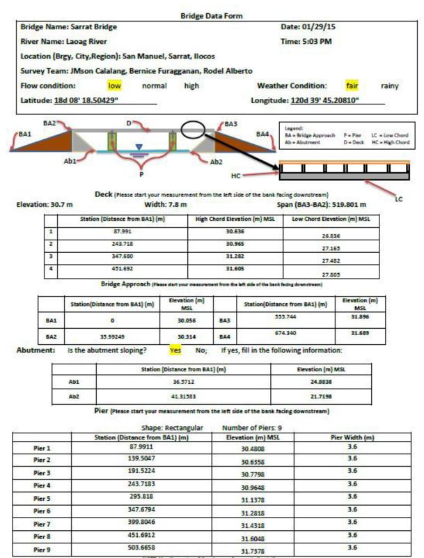
NOTE: Use the center of the pier as reference to its station
