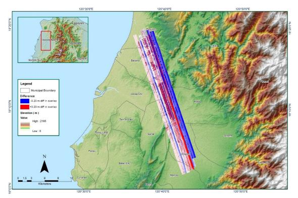
Figure 1.5.4. Elevation difference between flight lines
