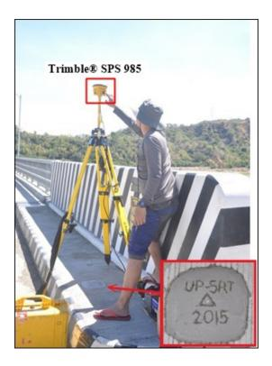
Figure 33.GNSS receiver setup, Trimble<sup>®</sup> SPS 985 at UP-SRT at Sarrat Bridge inBrgy. San Marcos, Municipality of Sarrat, Ilocos Norte.
