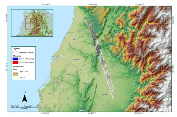
Figure 1.4.7. Elevation difference between flight lines
