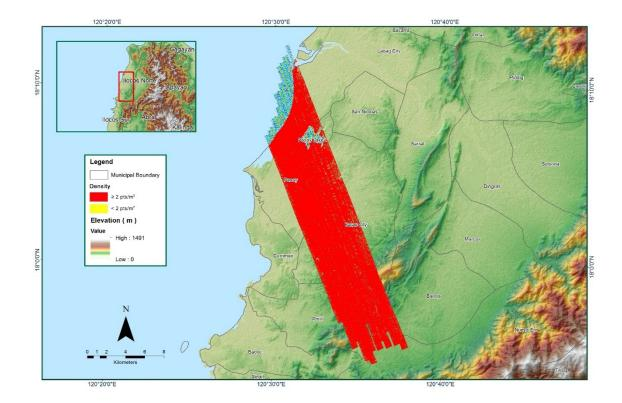
Figure 1.11.6. Density map of merged LiDAR data
