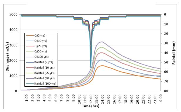
Figure 59. Outflow hydrograph at Laoag Station generated using the Laoag RIDF simulated in HEC-HMS.
