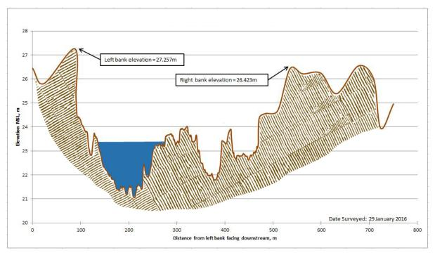
Figure 46. Cross-Section Plot of Cauplasan Bridge
