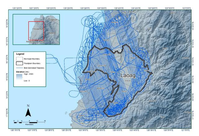
Figure 12. The best estimated trajectory of the LiDar missions conducted over the Laoag floodplain.
