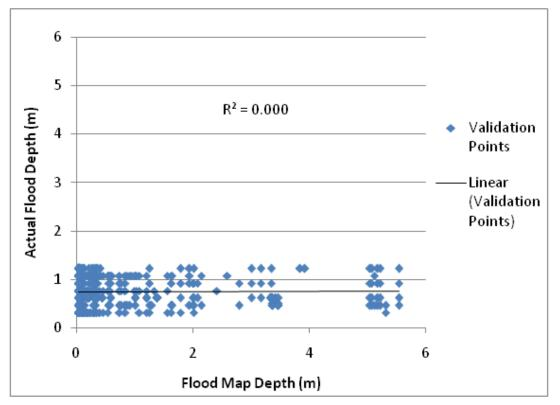
Figure 161. Flood Map Depth vs Actual Flood Depth for Laoag
