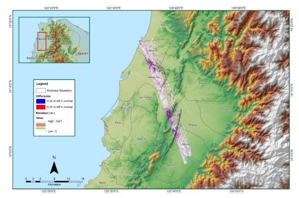
Figure 1.6.7. Elevation difference between flight lines
