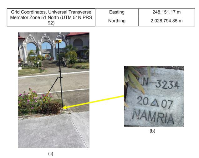
Figure 6.GPS set-up over ILN-3234 located in front of the Administration Building of Mariano Marcos Memorial University in Batac Ilocos Norte (a) and NAMRIA reference point ILN-3234 (b) as recovered by the field team.
