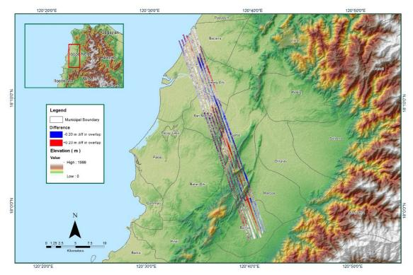
Figure 1.7.7. Elevation difference between flight lines
