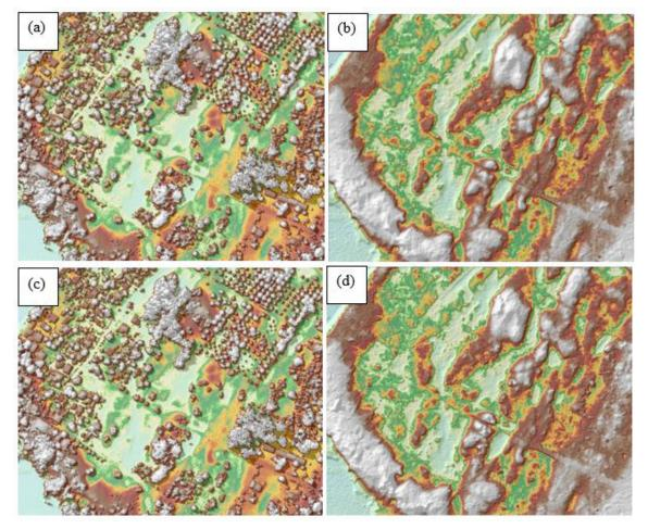
Figure 20. The production of last return DSM (a) and DTM (b), first return DSM (c) and secondary DTM (d) in some portion of Laoag floodplain.
