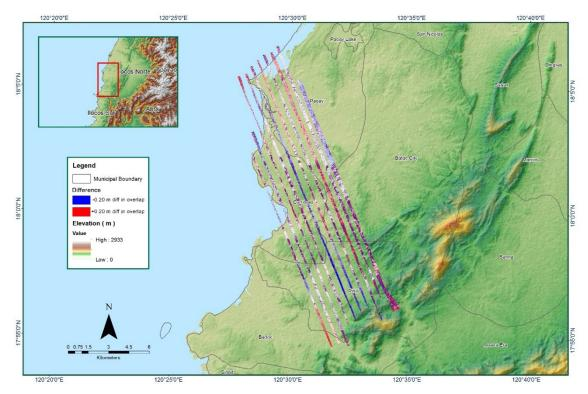
Figure 1.12.7. Elevation difference between flight lines
