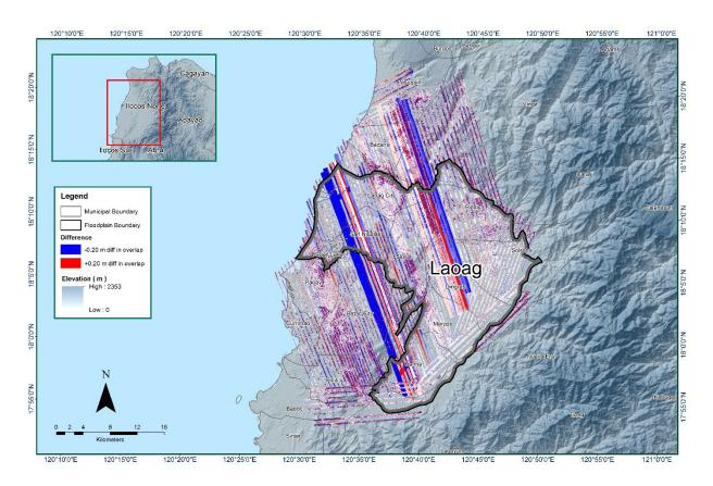
Figure 16. Elevation difference map between flight lines for Laoag floodplain.
