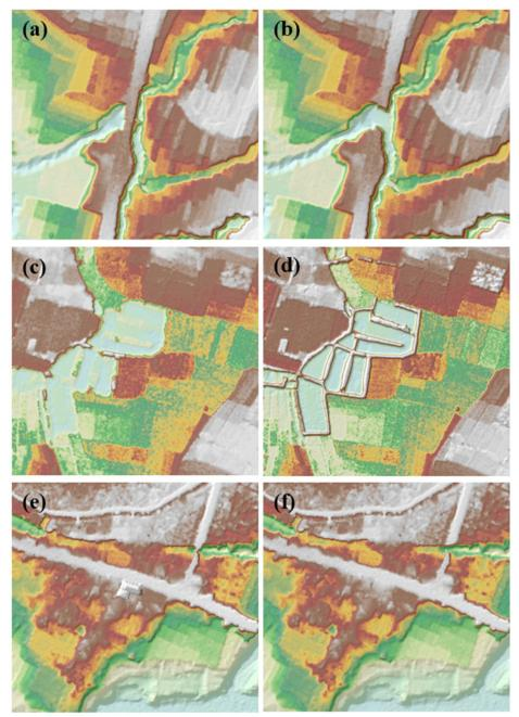
Figure 21. Portions in the DTM of Laoag floodplain – a bridge before (a) and after (b) manual editing; a paddy field before (c) and after (d) data retrieval; and a building before (e) and after (f) manual editing.
