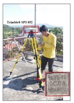
Figure 31.Base setup, Trimble<sup>®</sup> SPS 852, at ILN-11 located on the rooftop of the Batac City Hall inBrgy. Ricarte Poblacion, Batac City, Ilocos Norte
