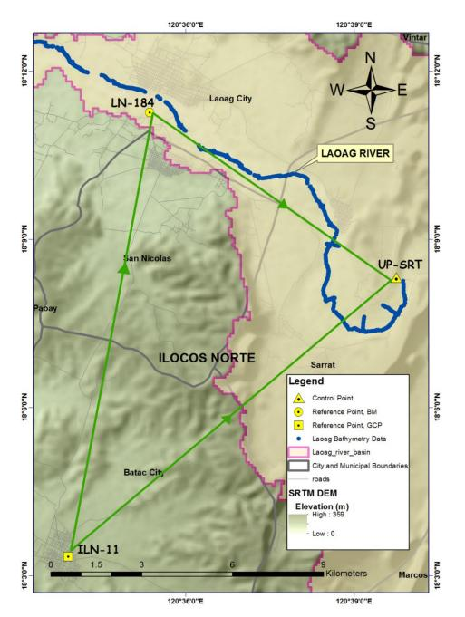
Figure 30.GNSS Network of Laoag River field Survey
