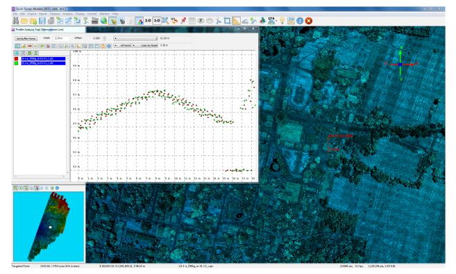
Figure 17. Quality checking for a Laoag flight 7096G using the Profile Tool of QT Modeler.
