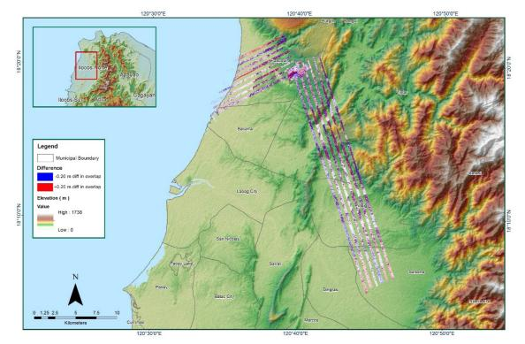
Figure 1.3.7. Elevation difference between flight lines
