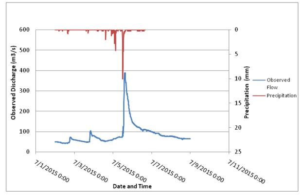
Figure 48. Rainfall and outflow data at Cauplasan Bridge used for modeling
