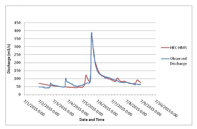
Figure 58.Outflow Hydrograph of Laoag produced by the HEC-HMS model compared with observed outflow
