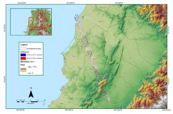
Figure 1.9.7. Elevation difference between flight lines
