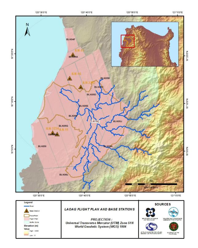
Figure 2. Flight plan and base stations used for Laoag floodplain.
