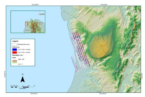
Figure 1.2.7 Elevation difference between flight lines
