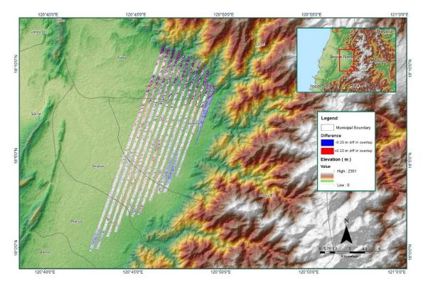
Figure 1.13.7. Elevation difference between flight lines
