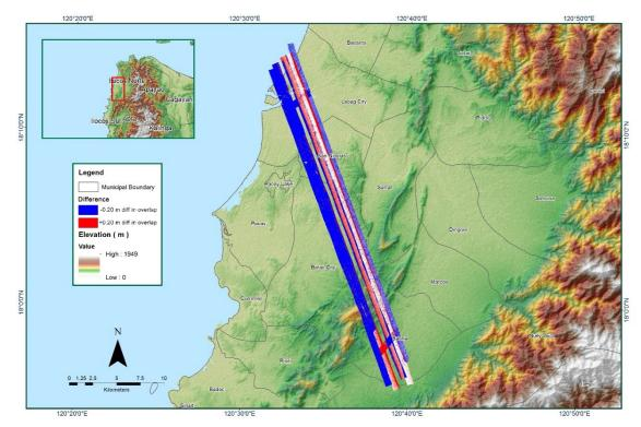
Figure 1.10.7. Elevation difference between flight lines
