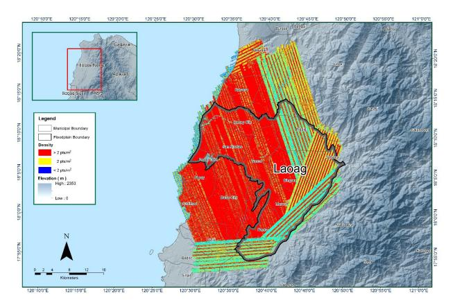
Figure 15. Density map of merged LiDAR data for Laoag floodplain.
