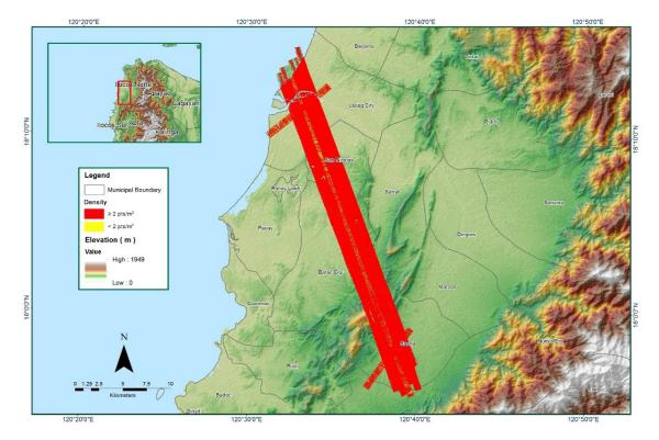
Figure 1.10.6. Density map of merged LiDAR data
