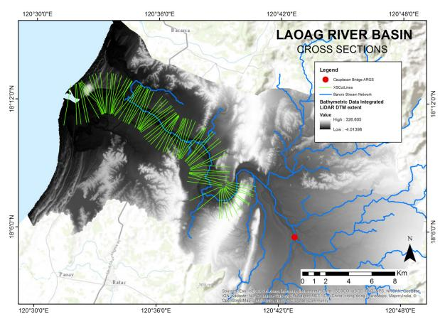
Figure 56. River cross-section of Laoag River generated through Arcmap HEC GeoRAS tool
