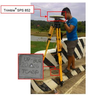
Figure 34. GNSS receiver setup, Trimble® SPS 852, at UP-BUR, located at the approach of Cabicungan Bridge in Brgy. Dibalio, Municipality of Claveria, Cagayan
