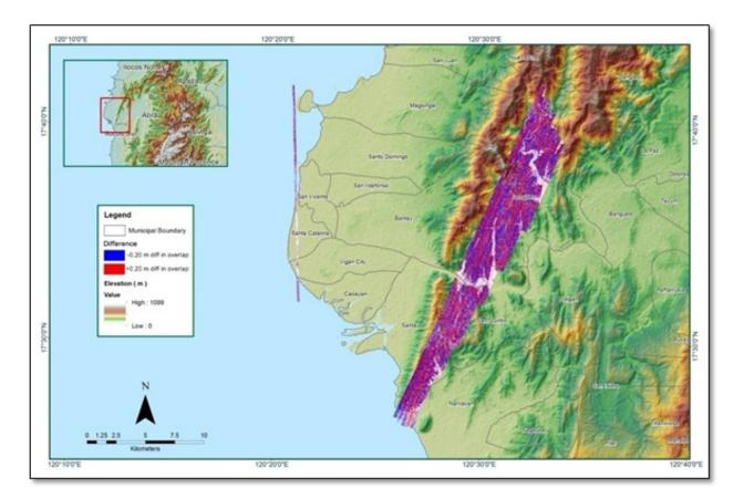
Figure A-8.42. Elevation difference between flight lines
