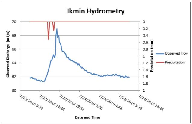
Figure 67. Rainfall and outflow data at Ikmin Bridge used for modeling
