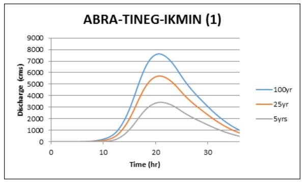
Figure 79. Abra-Tineg-Ikminriver (1) generated discharge using 5-, 25-, and 100-year Laoag rainfall intensity-duration-frequency (RIDF) in HEC-HMS
