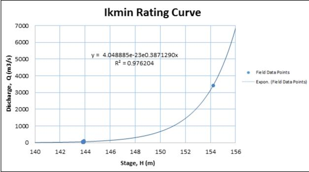
Figure 66. Rating Curve at Ikmin Bridge, Batac, Ilocos Norte
