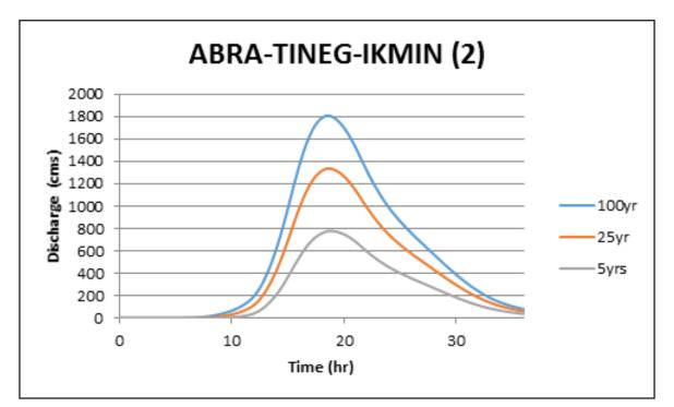
Figure 80. Abra-Tineg-Ikminriver (2) generated discharge using 5-, 25-, and 100-year Laoag rainfall intensity-duration-frequency (RIDF) in HEC-HMS
