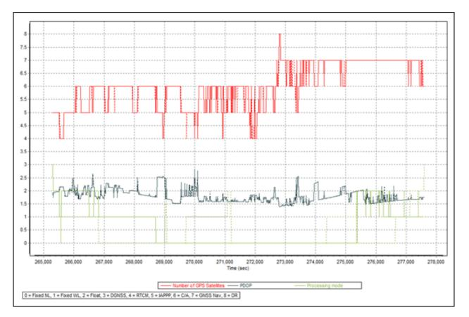
Figure A-8.8. Solution Status Parameters
