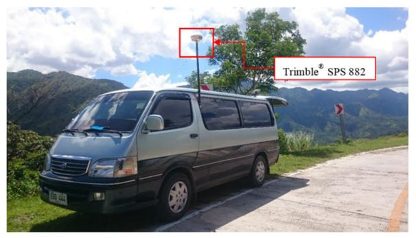
Figure 61. Validation points acquisition survey set up along Ikmin River Basin
