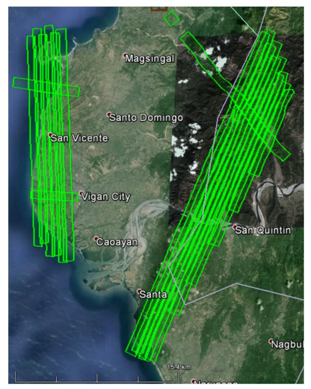
Flight No. : Area: Total Area: Mission Name: Altitude: PRF: Lidar FOV: 7114 G BLK07CS& BLK06G sq km 2BLK07CS067A & 2BLK06G067A 1800m / 1200m 50 kHz SCF: 50 Hz 18 deg Sidelap: 55% / 40%
