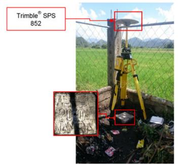
Figure 31. GNSS base set up, Trimble® SPS 852, at ABR-32, located behind basketball court in Brgy. Lagben, Municipality of Lagangilang, Abra
