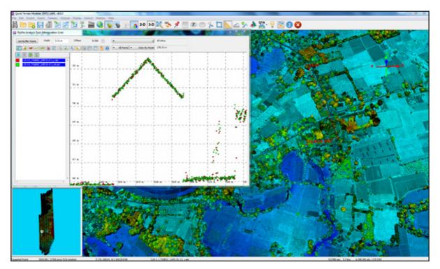
Figure 18. Quality checking for a Ikmin flight 7108GC using the Profile Tool of QT Modeler.
