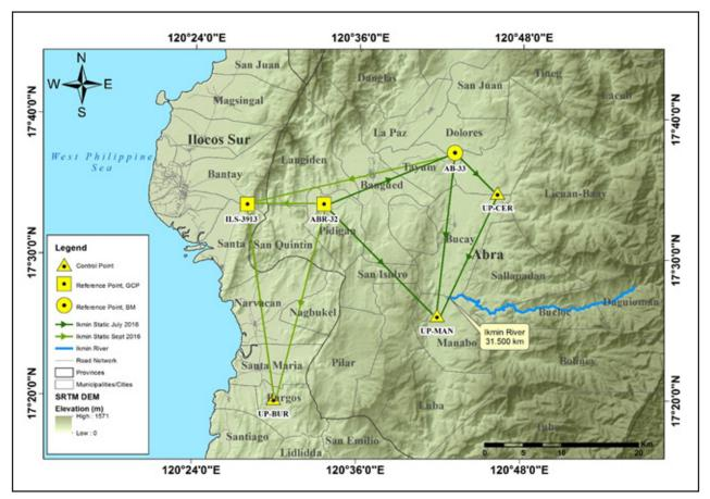
Figure 30. GNSS Network covering Ikmin River
