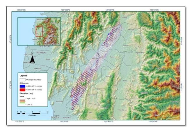
Figure A-8.70. Elevation difference between flight lines
