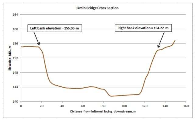
Figure 65. Cross-Section Plot of Ikmin Bridge
