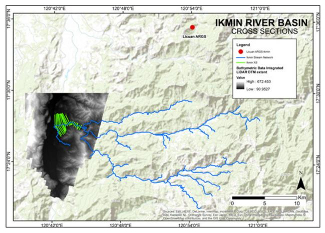
Figure 75. River cross-section of Ikmin River generated through Arcmap HEC GeoRAS tool
