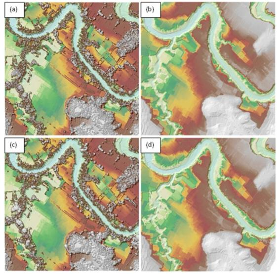
Figure 21. The production of last return DSM (a) and DTM (b), first return DSM (c) and secondary DTM (d) in some portion of Ikmin Floodplain.
