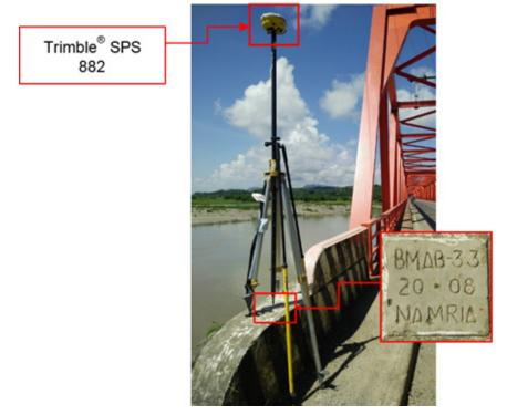
Figure 32. GNSS receiver setup, Trimble® SPS 882, atAB-33, located at the approach ofDon Mariano Marco Bridge, Brgy. Pamutic, Municipality of Pidigan, Abra
