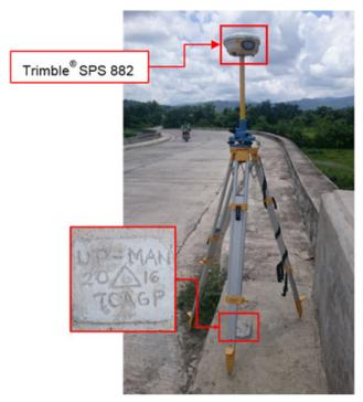
Figure 36. GNSS receiver setup, Trimble® SPS 882, at UP-MAN, located at the approach of Manabo Bridge, Brgy. San Juan Norte,Municipality of Manabo, Abra
