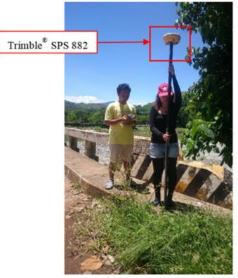
Figure 41. As-Built Survey of Cervantes Bridge
