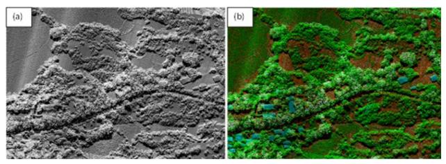
Figure 20. Point cloud before (a) and after (b) classification.
