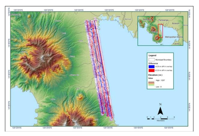
Figure A-8.63. Elevation difference between flight lines
