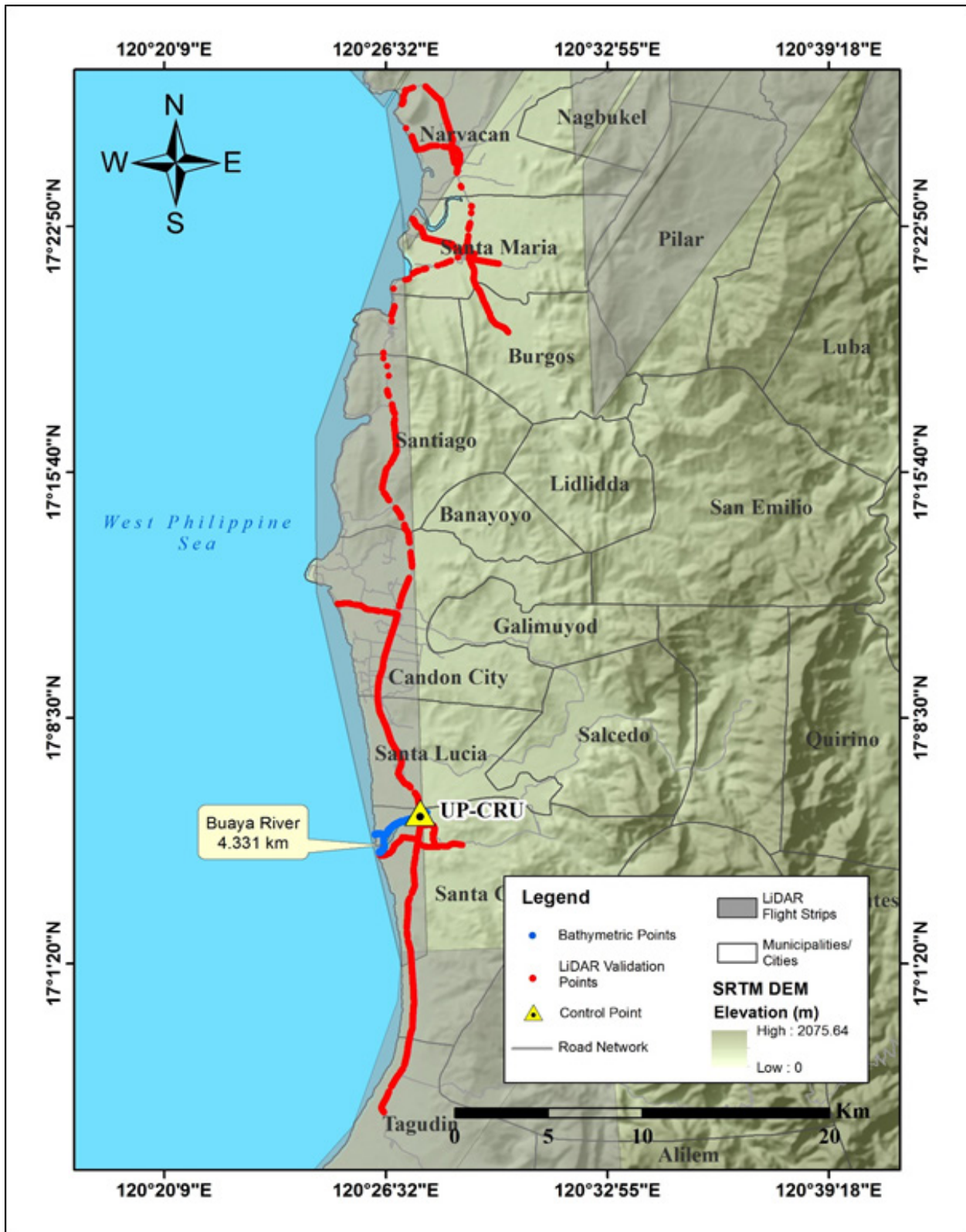
Figure 42. Validation point acquisition survey of Buaya River basin
