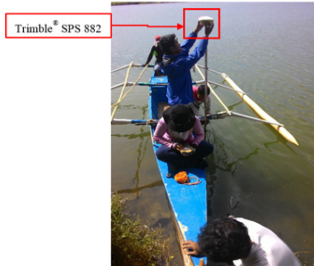
Figure 43. Bathymetric survey using Ohmex™ single beam echo sounder in Buaya River
