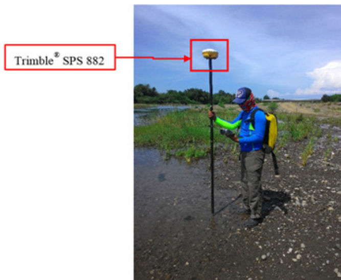
Figure 44. Manual bathymetric survey in Buaya River
