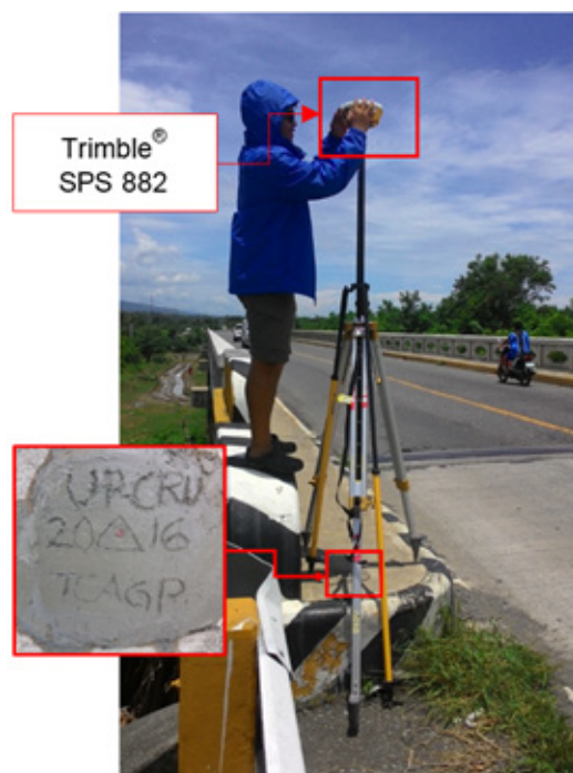
Figure 34. GNSS receiver setup, Trimble® SPS 882, at UP-CRU, located at the approach of Santa Cruz Bridge, in Brgy. Quinsoriano, Municipality of Santa Cruz, Ilocos Sur
