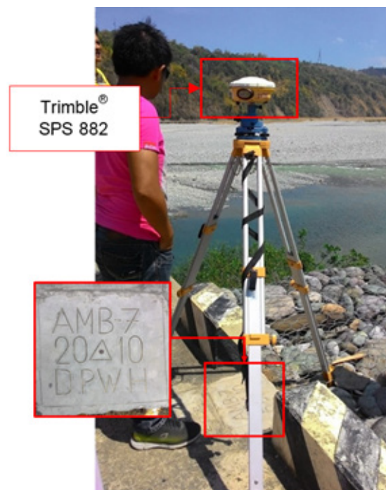
Figure 32. GNSS receiver setup, Trimble® SPS 882, at AMB-7, located at the approach of Alilem Bridge, in Brgy. Kiat, Municipality of Alilem, Ilocos Sur
