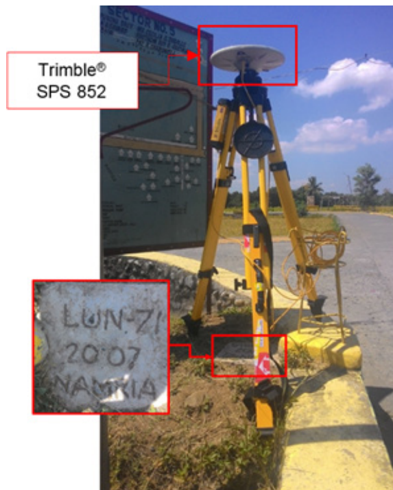
Figure 31. GNSS base set up, Trimble® SPS 852, at LUN-71, situated beside the irrigation canal at the right intersection of barangay roads, in Brgy. General Prim West, Municipality of Sudipen, La Union
