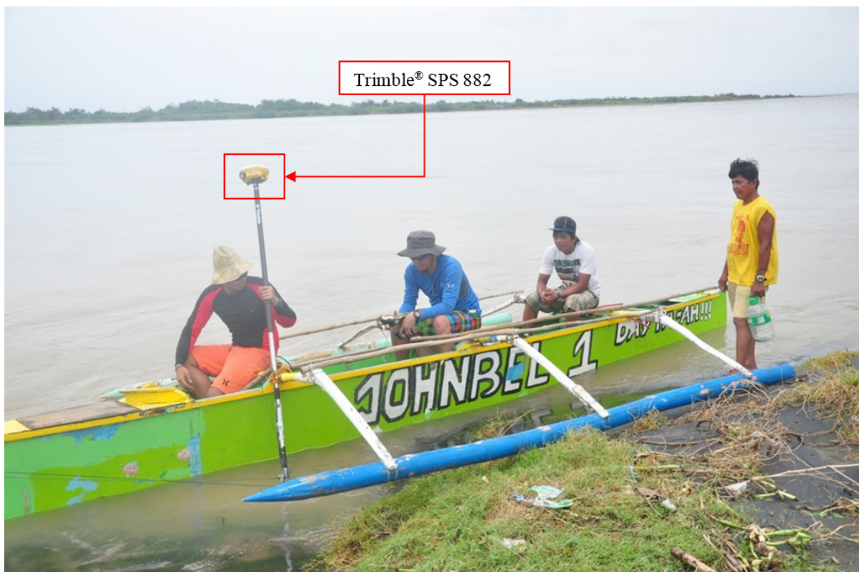
Figure 50. Bathymetry survey set-up for Bauang River
