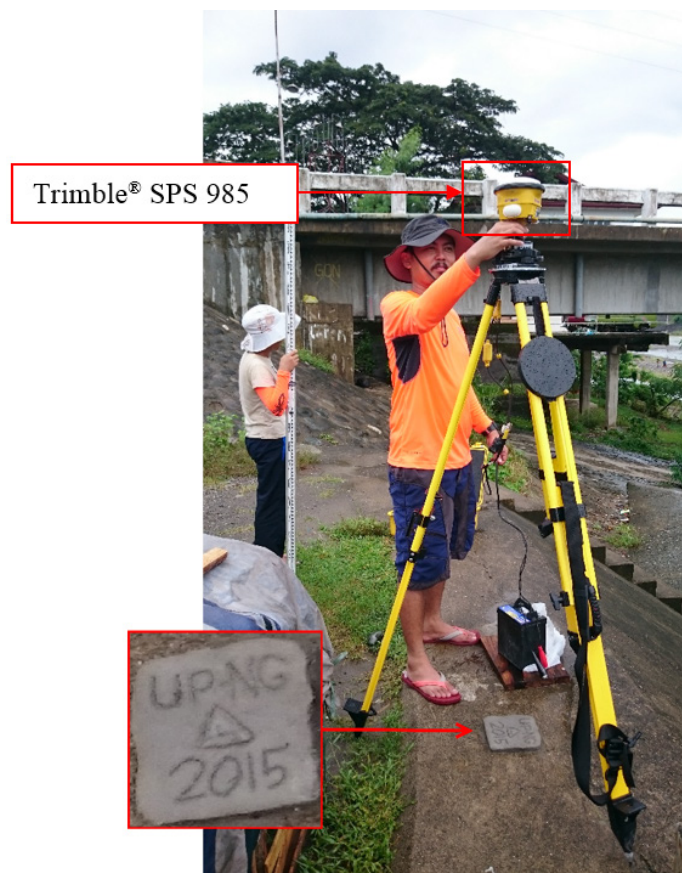
Figure 39. GNSS receiver Trimble® SPS 985 at UP-NG, located at the Naguilian Bridge approach in Barangay Cabaritan, Municipality of Naguilian, La Union
