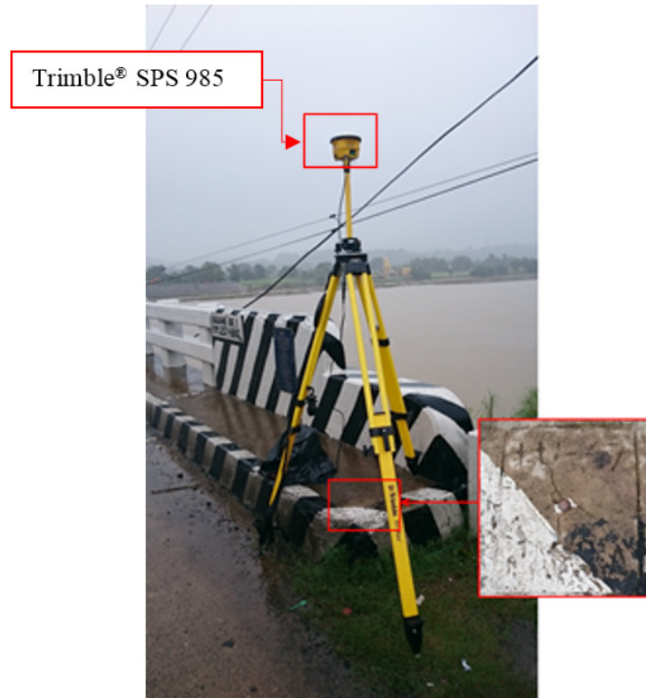
Figure 34. GNSS receiver Trimble® SPS 985 at LU-67, located at the Bauang Bridge approach in Barangay Nagrebcan, Municipality of Bauang, La Union
