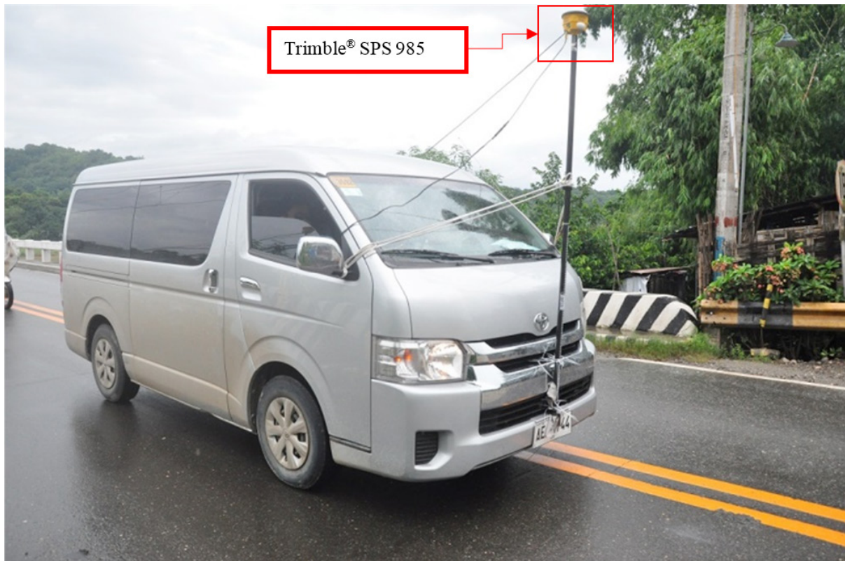
Figure 48. Set-up for the validation points acquisition in the Bauang River Basin
