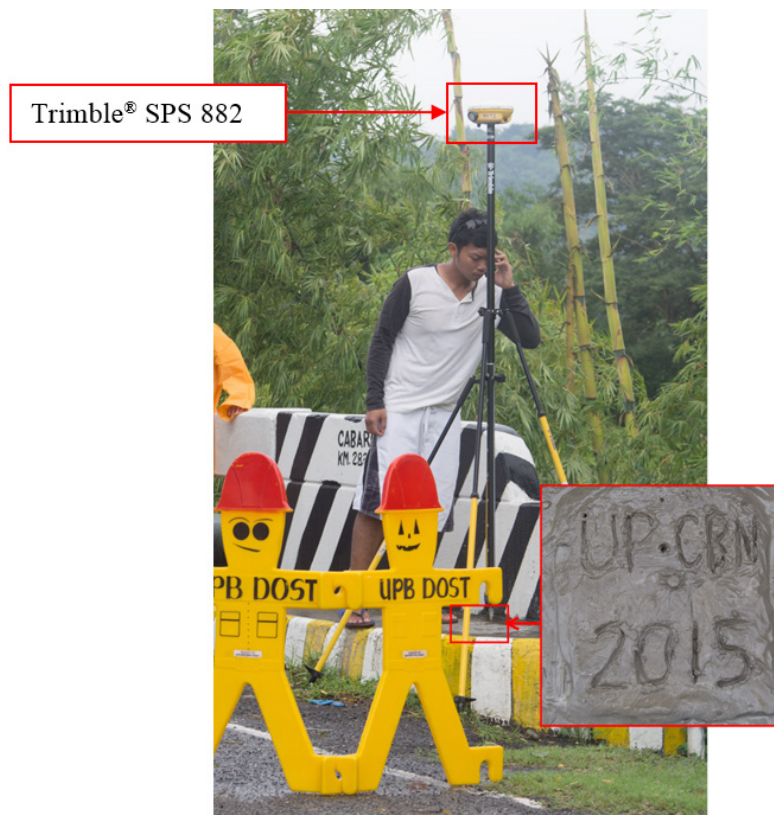
Figure 37. GNSS receiver Trimble® SPS 882 at UP-CBN, located at the Cabaroan Bridge approach in Barangay Cabaroan, Municipality of San Juan, La Union
