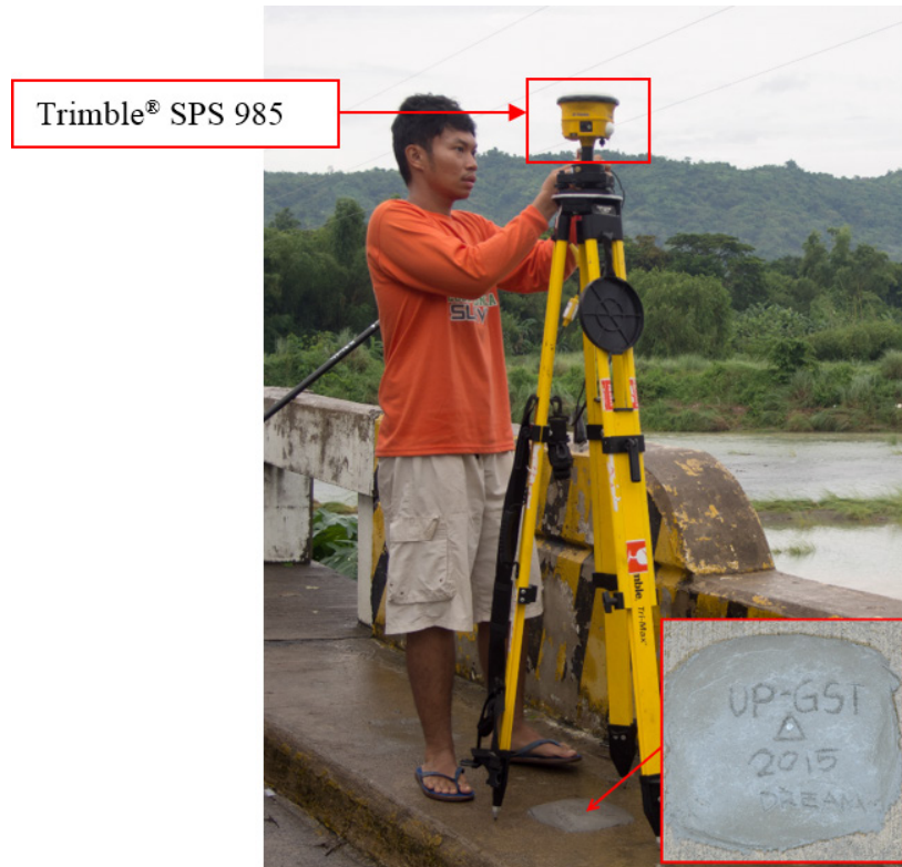
Figure 38. GNSS receiver Trimble® SPS 985 at UP-GST, located at the Guesset Bridge approach in Barangay Ambaracao, Municipality of Naguilian, La Union
