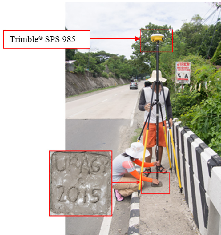
Figure 36. GNSS receiver Trimble® SPS 882 at UP-AGY, located at the Aringay Bridge approach in Barangay Poblacion, Municipality of Aringay, La Union
