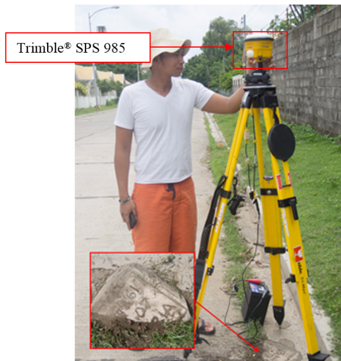
Figure 35. GNSS receiver Trimble® SPS 985 at LUN-61, located near the BPPC Housing in Barangay Guerrero, Municipality of Bauang, La Union
