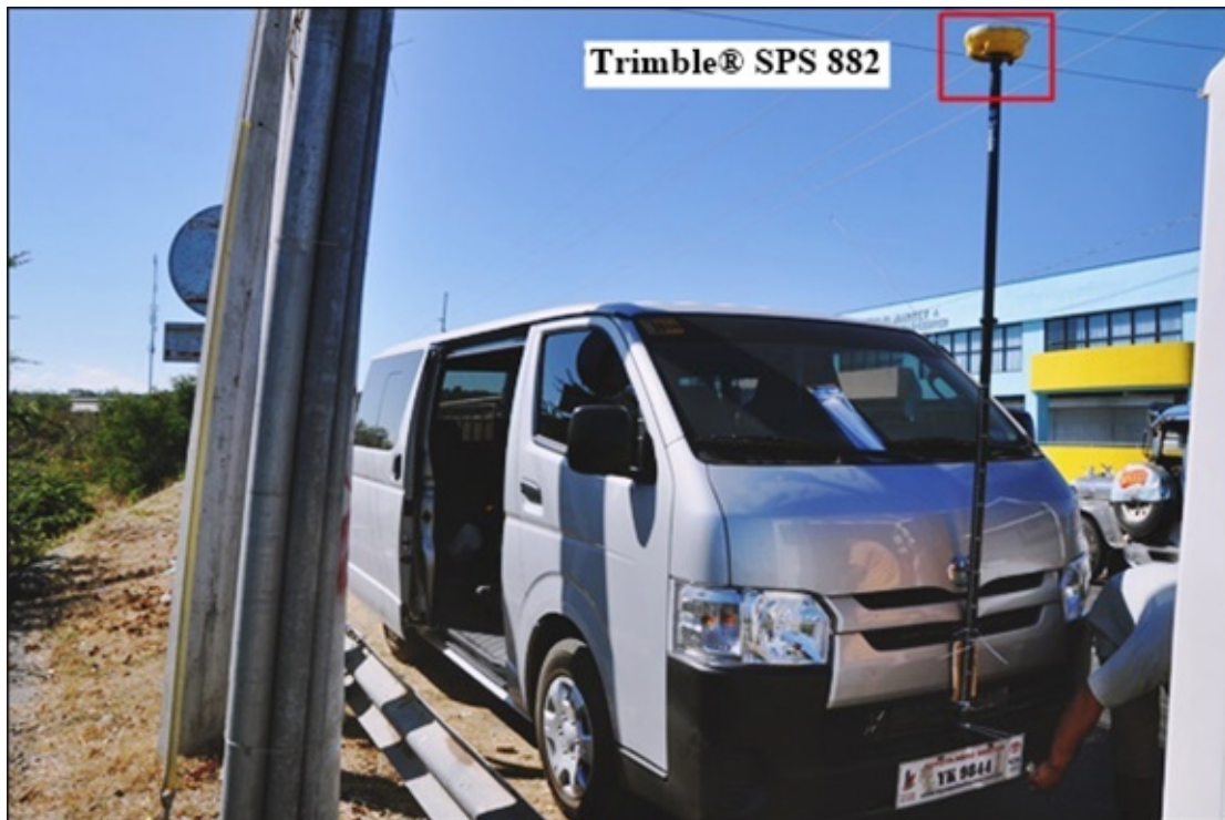
Figure 41. GNSS Receiver Trimble® SPS 882 installed on a vehicle for Ground Validation Survey.
