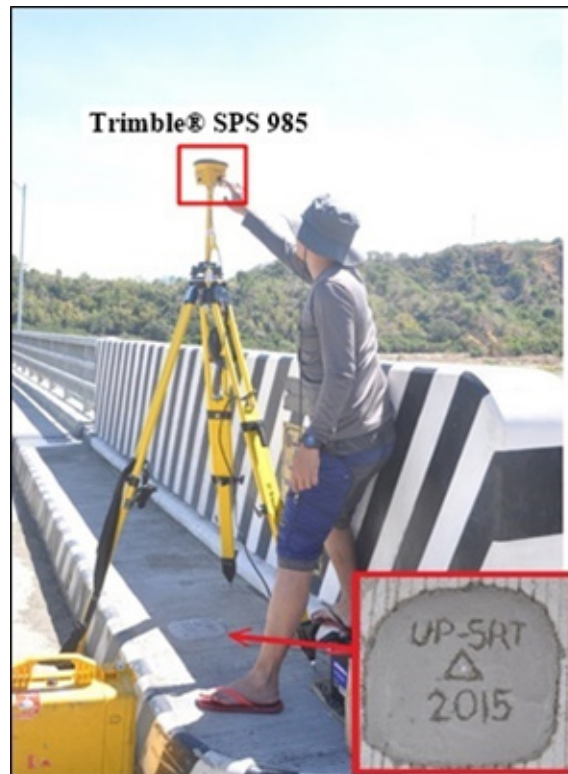
Figure 33. GNSS receiver setup, Trimble® SPS 985 at UP-SRT at Sarrat Bridge in Brgy. San Marcos, Municipality of Sarrat, Ilocos Norte.
