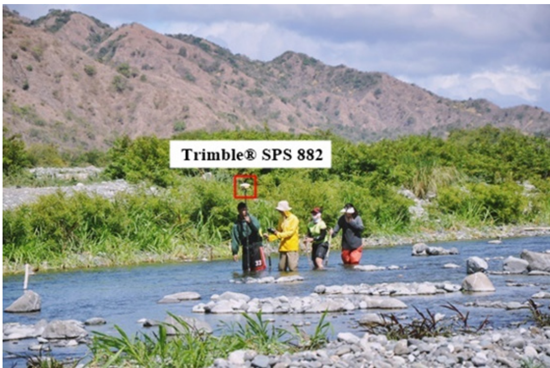
Figure 43. Set up of the bathymetric survey at Bacarra River using Trimble® SPS 852 in GNSS PPK survey technique.
