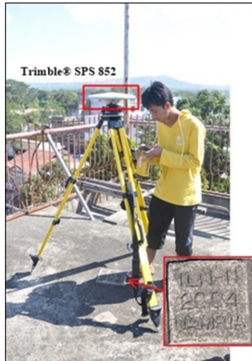
Figure 31. Base setup, Trimble® SPS 852, at ILN-11 located on the rooftop of the Batac City Hall in Brgy. Ricarte Poblacion, Batac City, Ilocos Norte.
