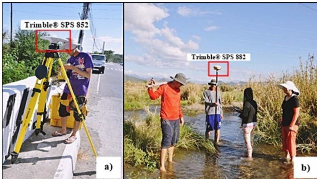
Figure 36. As-built survey conducted at Bacarra Bridge.
