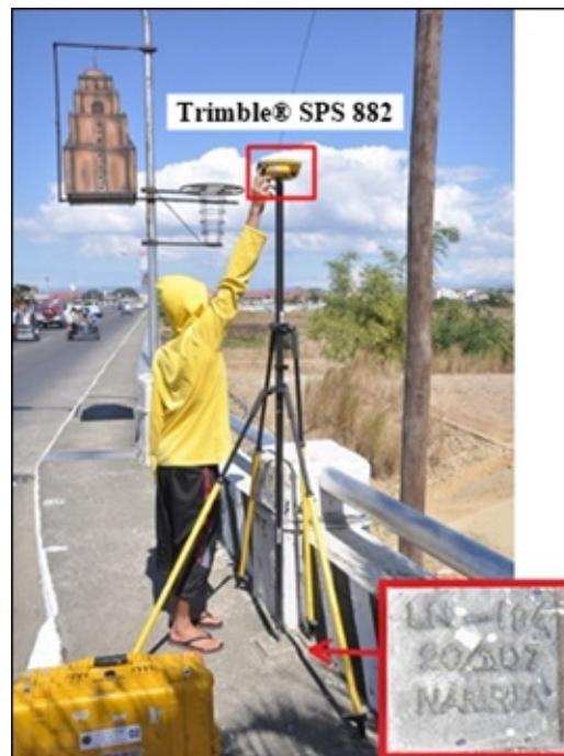
Figure 32. GNSS receiver setup, Trimble® SPS 882 at BM LN-184 on the approach of Gilbert Bridge in Brgy. No. 51-A, Nangalisan East, Laog City, Ilocos Norte.
