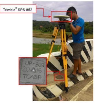
Figure 37. GNSS receiver setup, Trimble® SPS 852, at UP-BUR located at the approach of Burgos Bridge in Brgy. Poblacion Norte, Municipality of Burgos, Abra.
