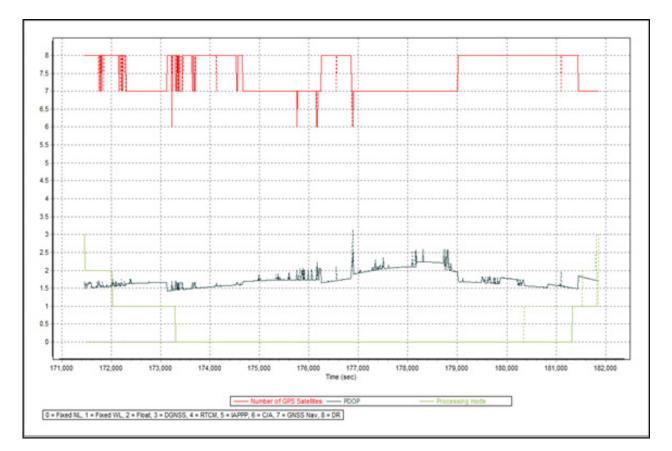
Figure A-8.29. Solution Status Parameters
