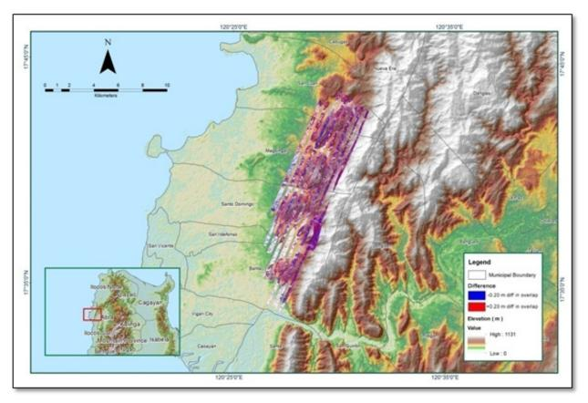
Figure A-8.35. Elevation difference between flight lines
