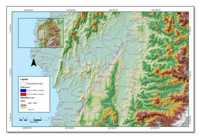
Figure A-8.77. Elevation difference between flight lines
