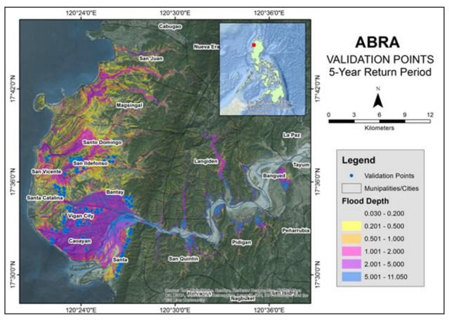
Figure 168. Validation Points for a 5-year Flood Depth Map of the Abra Floodplain.
