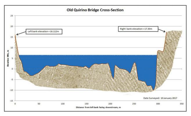
Figure 48. Cross-Section Plot of Banaong Bridge or Old Quirino Bridge.
