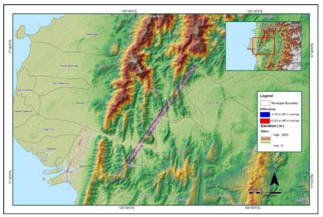
Figure A-8.105 Elevation difference between flight lines
