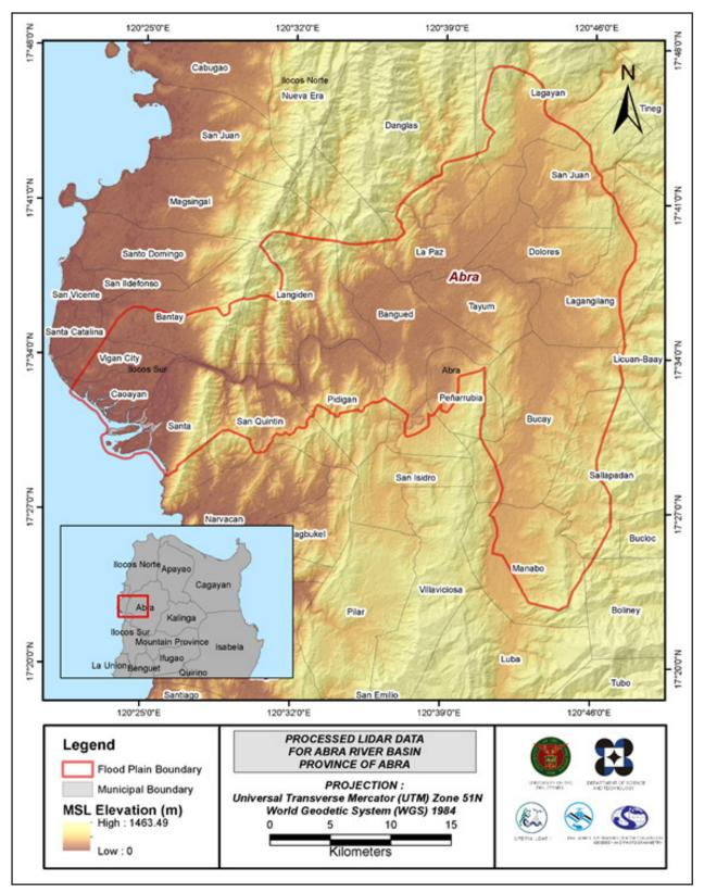
Figure 23. Map of processed LiDAR data for the Abra Floodplain.
