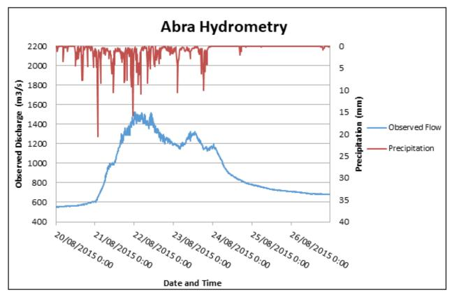
Figure 50. Rainfall and outflow data at Banaoang Bridge, which was used for modeling.
