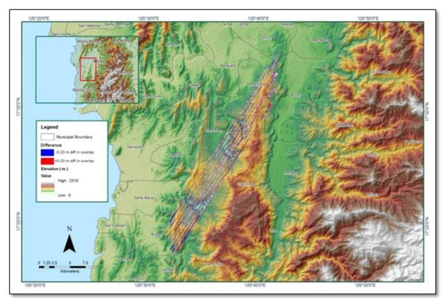
Figure A-8.98 Elevation difference between flight lines
