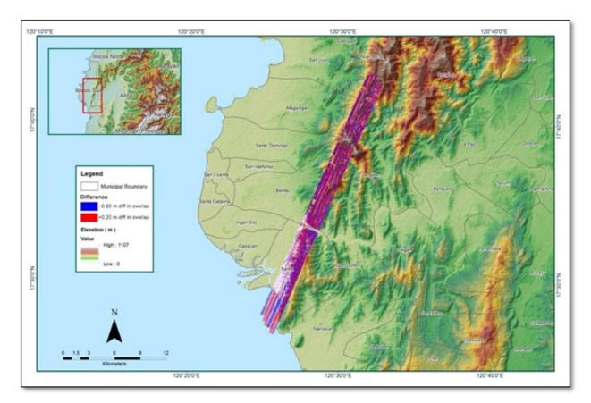
Figure A-8.49. Elevation difference between flight lines
