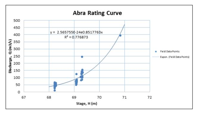
Figure 49. The rating curve at Banaoang Bridge, Santa, Ilocos Sur.
