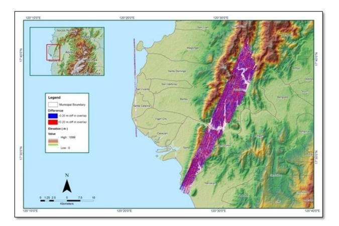
Figure A-8.42. Elevation difference between flight lines
