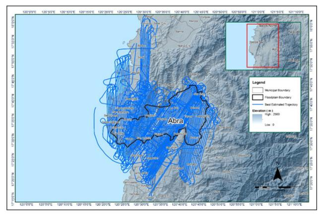
Figure 13. Best Estimated Trajectory of the LiDAR missions conducted over the Abra Floodplain.
