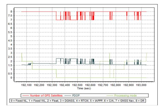
Figure A-8.57. Solution Status Parameters
