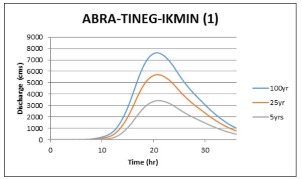
Figure 62. Abra-Tineg-Ikmin river (1) generated discharge using 5-, 25-, and 100-year Laoag rainfall intensityduration-frequency (RIDF) in HEC-HMS.
