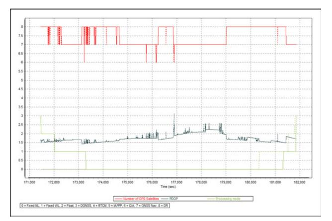
Figure A-8.50. Solution Status Parameters
