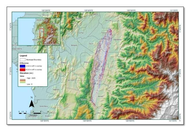
Figure A-8.84. Elevation difference between flight lines
