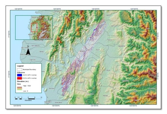
Figure A-8.70. Elevation difference between flight lines
