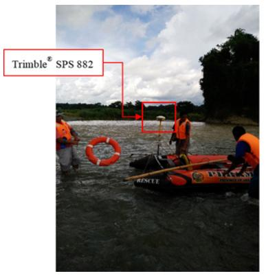
Figure 44. Set up of the bathymetric survey at Abra River using Ohmex<sup>™</sup> single beam echo sounder.
