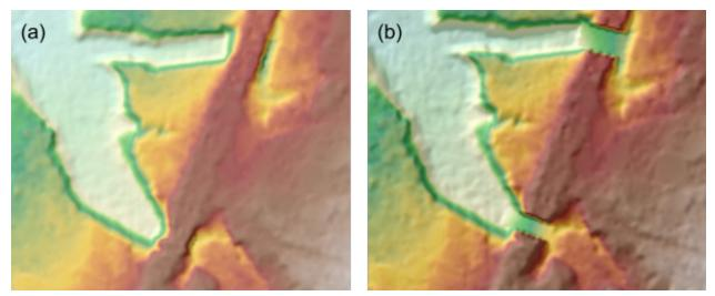
Figure 22. Portions in the DTM of the Abra Floodplain – a bridge before (a) and after (b) manual editing.
