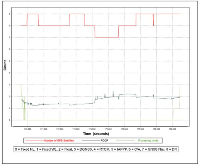
Figure 12. Solution Status Parameters of Abra Flight 7108GC.
