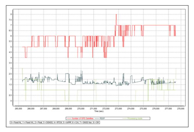
Figure A-8.15. Solution Status Parameters
