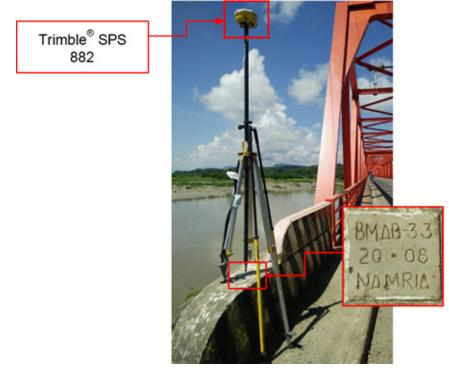
Figure 33. GNSS receiver setup, Trimble® SPS 882, at AB-33 located at the approach of Don Mariano Marcos Bridge, Municipality of Dolores, Abra.
