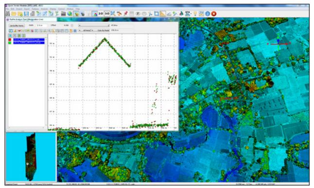
Figure 18. Quality checking for aAbra flight 7108GC using the Profile Tool of QT Modeler
