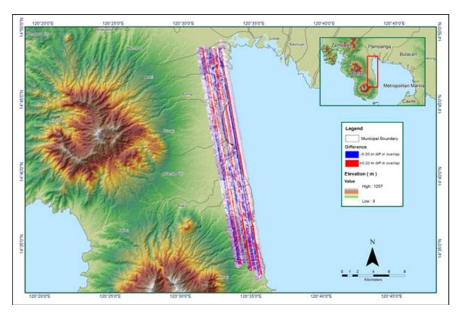
Figure A-8.63. Elevation difference between flight lines
