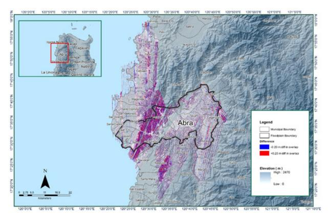
Figure 17. Elevation difference Map between flight lines for the Abra Floodplain Survey
