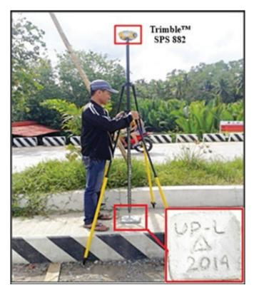
Figure 39. GNSS receiver setup, Trimble<sup>®</sup> SPS 882, at UP-L, located at the approach of Liangan Bridge, in Brgy.
