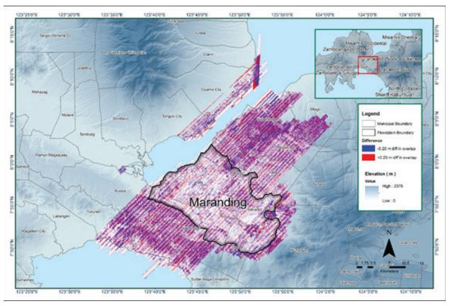
Figure 20. Map of elevation difference Map between flight lines for the Maranding Floodplain Survey.
