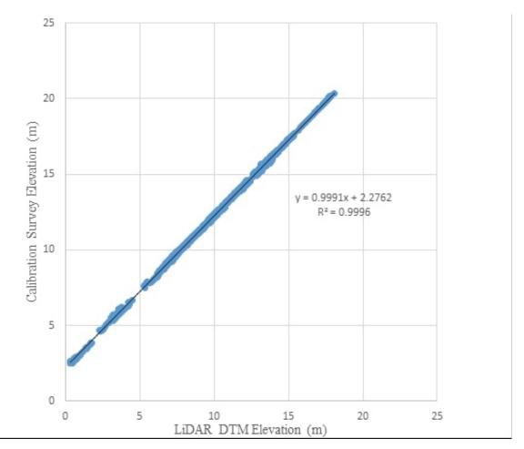
Figure 30. Correlation plot between calibration survey points and LiDAR data.
