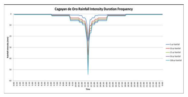
Figure 55. The synthetic storm generated for a 24-hour period rainfall for various return periods.
