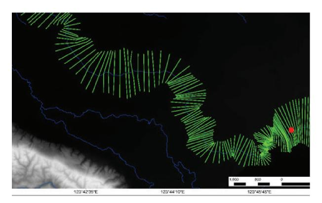
Figure 60. River cross-section of the Maranding River through the ArcMap HEC GeoRas tool.
