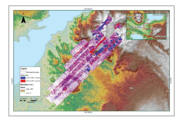
Figure A-8.7 Elevation difference between flight lines
