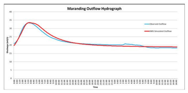
Figure 62. Outflow Hydrograph of Maranding produced by the HEC-HMS model compared with observed outflow.
