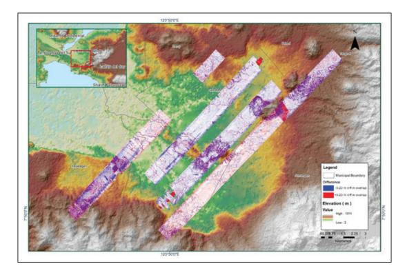
Figure A-8.14 Elevation difference between flight lines
