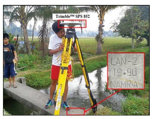
Figure 37. GNSS base set up, Trimble<sup>®</sup> SPS 852, at LAN-2, situated on top of a concrete irrigation canal gate in Brgy. Maranding, Municipality of Kapatagan, Lanao Del Norte.
