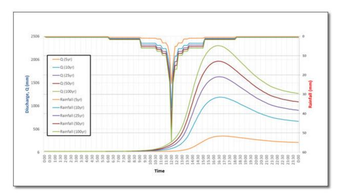
Figure 63. The Outflow hydrograph at the Maranding Station, generated using the Cagayan de Oro RIDF simulated in HEC-HMS.
