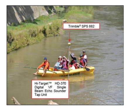
Figure 46. Set up of Hi-Target<sup>™</sup> Single Beam Echo Sounder integrated with a roving GNSS receiver on a motor boat for the bathymetric survey in Maranding River.
