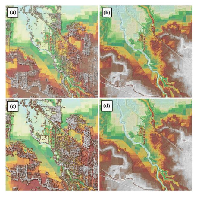
Figure 24. Photo (A) features the production of the last return DSM; (B) depicts the production of the DTM; (C) portrays the production of the first return DSM; and (D) presents the generation of the secondary DTM in some portions of the Maranding Floodplain.
