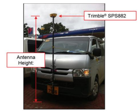
Figure 44. Trimble<sup>®</sup> SPS882 set-up on a vehicle for validation points acquisition along the major roads near Maranding River.
