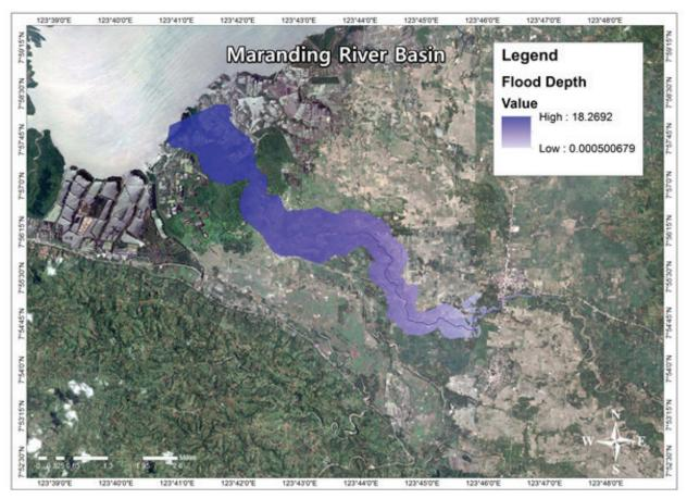
Figure 64. The sample output map of the Maranding RAS Model.
