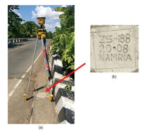
Figure 4. GPS set-up over ZS-188 (a) at Brgy. Licomo, Zamboanga City, Zamboanga del Sur and NAMRIA reference point ZS-188 (b) as recovered by the field team
