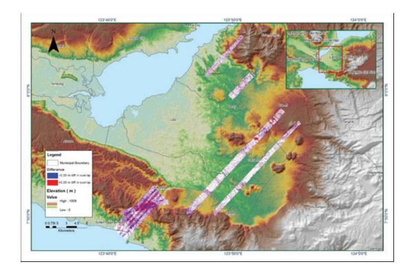
Figure A-8.28 Elevation difference between flight lines
