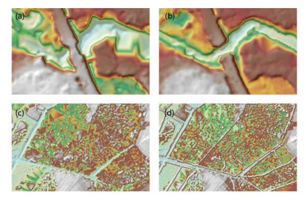
Figure 27. Portions in the DTM of the Maranding Floodplain showing (a) a bridge before undergoing manual; (b) bridge after manual editing; (c) a paddy field before undergoing manual editing; while (d) after data retrieval.
