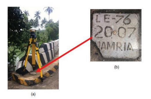
Figure 9. GPS set-up over LE-76 at Bulod Bridge footwalk of Brgy. Bulod, Tubud, Lanao del Norte (a) and NAMRIA reference point LE-76 (b) as recovered by the field team.
