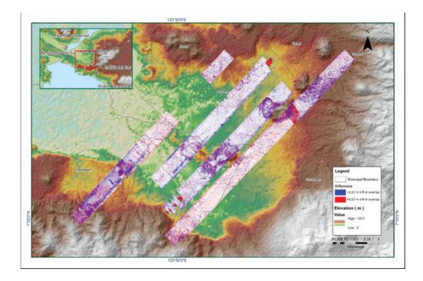
Figure A-8.42 Elevation difference between flight lines
