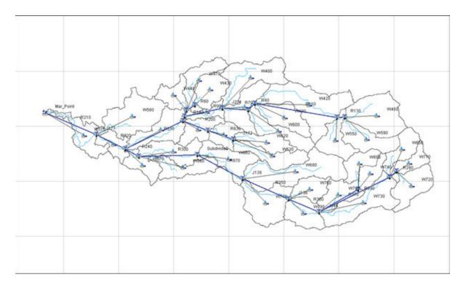
Figure 59. The Maranding river basin model generated using HEC-HMS.
