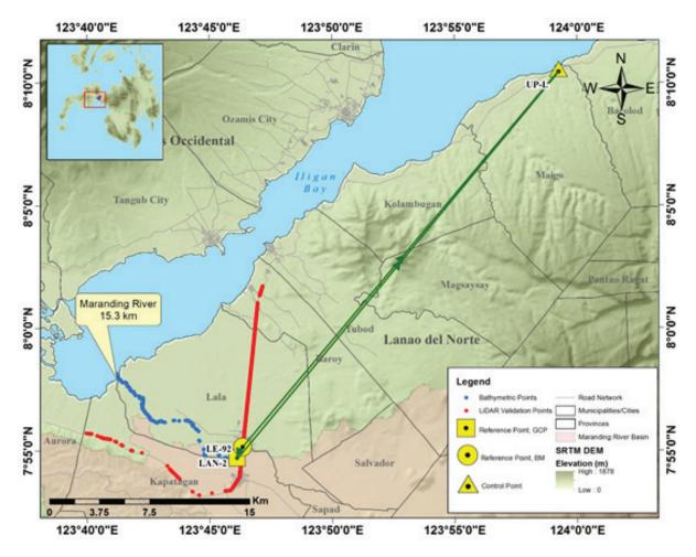
Figure 35. .Extent of the bathymetric survey (in blue line) in Maranding River.
