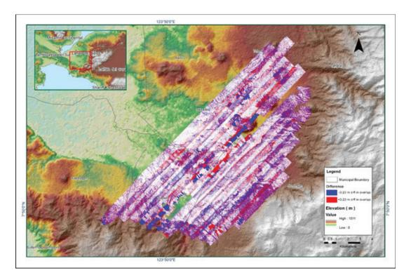
Figure A-8.35 Elevation difference between flight lines
