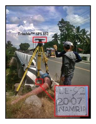
Figure 38. GNSS base set up, Trimble<sup>®</sup> SPS 852, at LE-92, located at the approach of Maranding Bridge, in Brgy.
