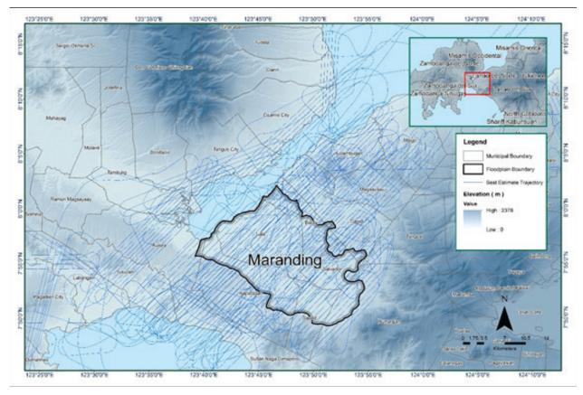
Figure 16. Best Estimated Trajectory of the LiDAR missions conducted over the Maranding Floodplain
