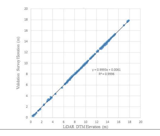
Figure 31. Correlation plot between the validation survey points and the LiDAR data.
