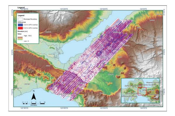
Figure A-8.70 Elevation difference between flight lines
