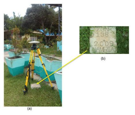
Figure 10. GPS set-up over ZGN-138 (a) in Katipinan Zamboanga del Norte and NAMRIA reference point ZGN-138 (b) as recovered by the field team.
