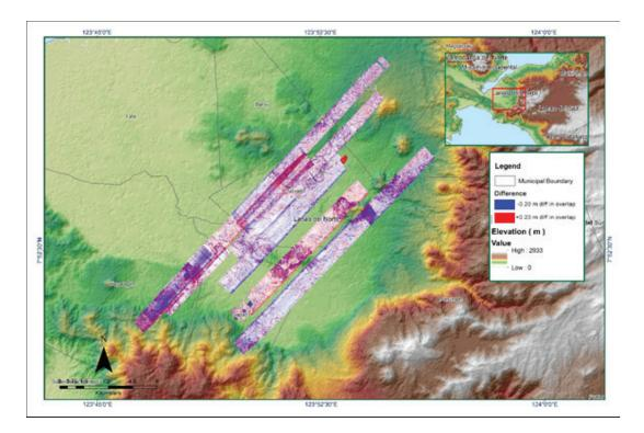
Figure A-8.49 Elevation difference between flight lines
