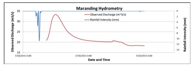
Figure 53. Rainfall and outflow data of the Maranding River Basin, which was used for modeling.
