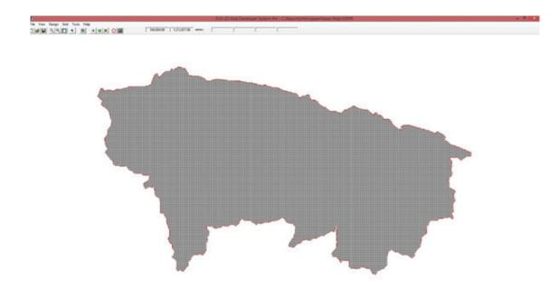
Figure 61. . A screenshot of the river sub-catchment with the computational area to be modeled in FLO-2D Grid Developer System Pro (FLO-2D GDS Pro)
