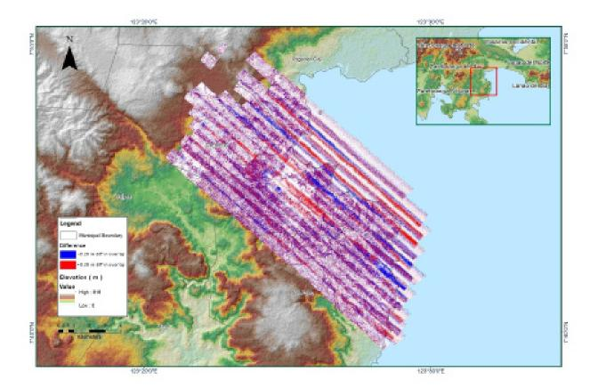
Figure A-8.84. Elevation difference between flight lines
