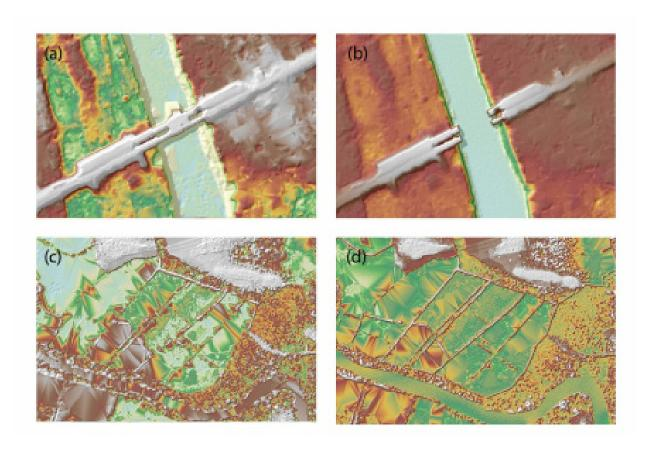
Figure 25. Portions in the DTM of Labangan floodplain – a bridge before (a) and after (b) manual editing; a paddy field before (c) and after (d) data retrieval
