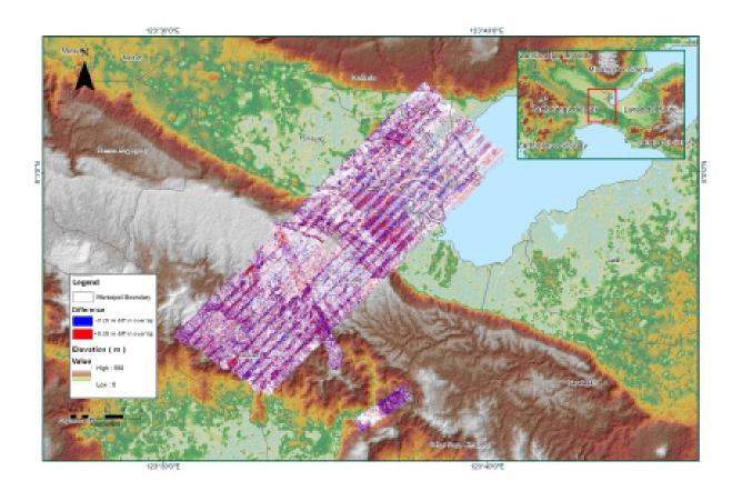
Figure A-8.56. Elevation difference between flight lines
