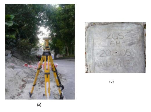
Figure 6. GPS set-up over ZGS-68 at CENRO, Brgy. Poblacion, Municipality of Guipos, Zamboanga del Sur (a) and NAMRIA reference point ZGS-68 (b) as recovered by the field team.
