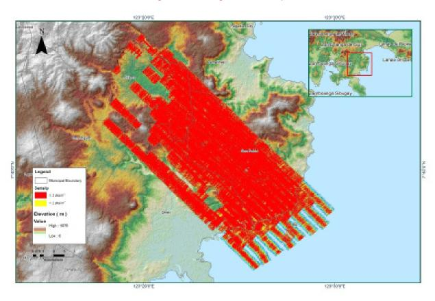
Figure A-8.76. Density map of merged LiDAR data
