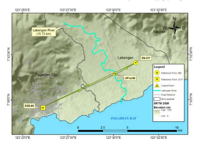
Figure 34. GNSS Network of Labangan Field Survey
