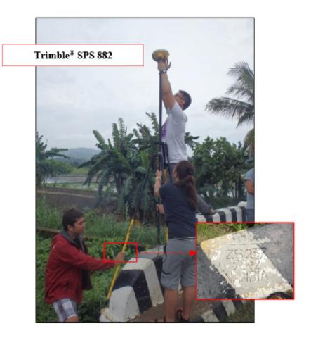
Figure 35. GNSS receiver occupation, Trimble® SPS 882, at ZS-237, Lantian Bridge, in Brgy. Upper Campo Islam, Labangan City, Zamboanga del Sur
