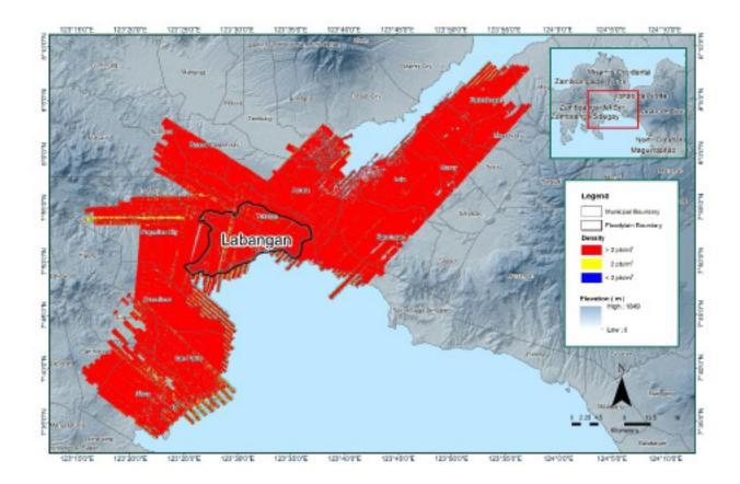
Figure 17. Pulse density map of merged LiDAR data for Labangan floodplain.
