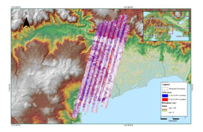
Figure A-8.14. Elevation difference between flight lines
