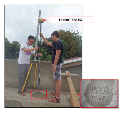
Figure 37. GNSS base occupation, Trimble® SPS 852, at control point UP-LAB, Labangan Bridge in Brgy. New Labangan, Labangan City, Zamboanga del Sur
