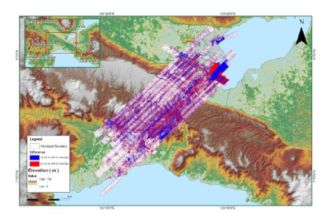
Figure A-8.49. Elevation difference between flight lines
