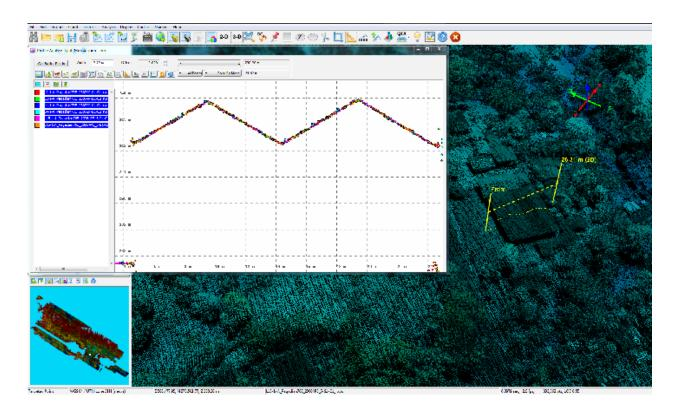
Figure 19. Quality checking for a Labangan flight 23064P using the Profile Tool of QT Modeler.
