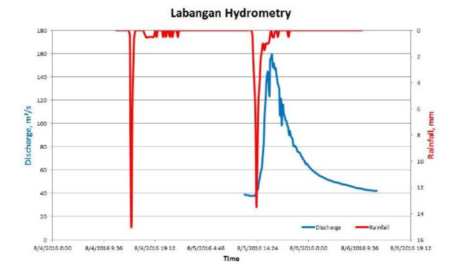
Figure 56. Rainfall and outflow data at Isidro Rey LL. Real III Hanging Bridge used for modeling
