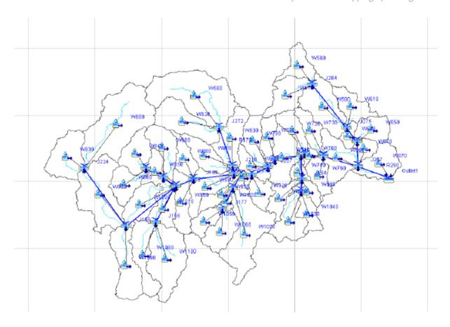
Figure 63. The Labangan Hydrologic Model generated in HEC-GeoHMS
