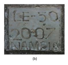
Figure 7. GPS set-up over LE-50 at Barogohan Bridge and at the NE of the Covenant Baptist Church, Maigo, Lanao del Norte (a) and NAMRIA reference point LE-50 (b) as recovered by the field team.
