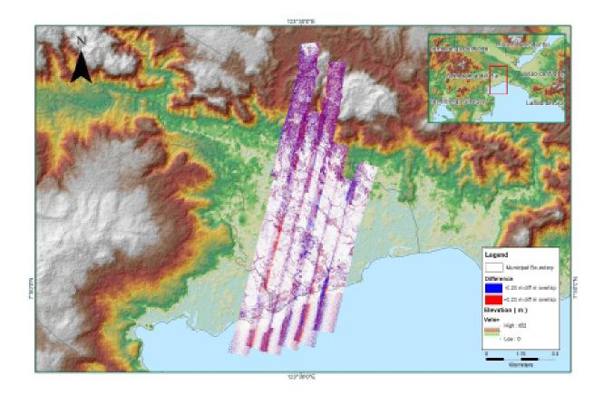
Figure A-8.28. Elevation difference between flight lines
