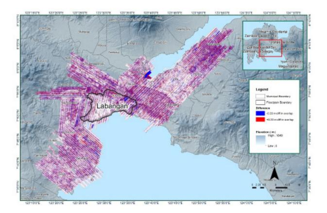
Figure 18. Elevation difference map between flight lines for Labangan floodplain.
