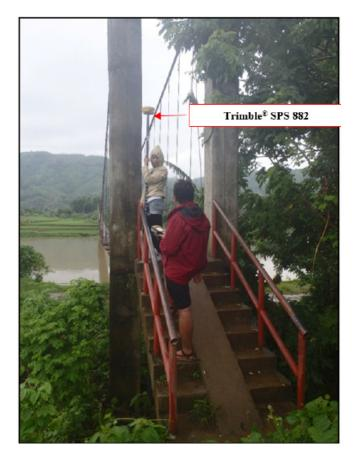
Figure 40. Cross-section survey at the Hanging Bridge in Brgy.Bokong, Labangan, Zamboanga del Sur
