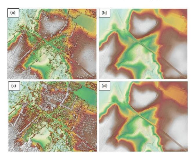
Figure 22. The production of last return DSM (a) and DTM (b), first return DSM (c) and secondary DTM (d) in some portion of Labangan floodplain.
