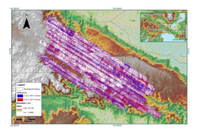
Figure A-8.35. Elevation difference between flight lines
