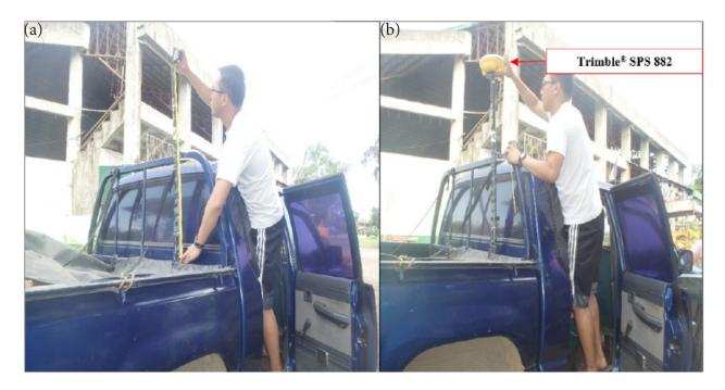
Figure 48. Validation points acquisition survey set-up
