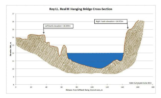
Figure 54. Cross-Section Plot of Isidro Rey LL. Real III Hanging Bridge
