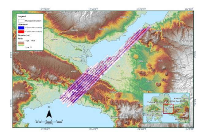
Figure A-8.105. Elevation difference between flight lines
