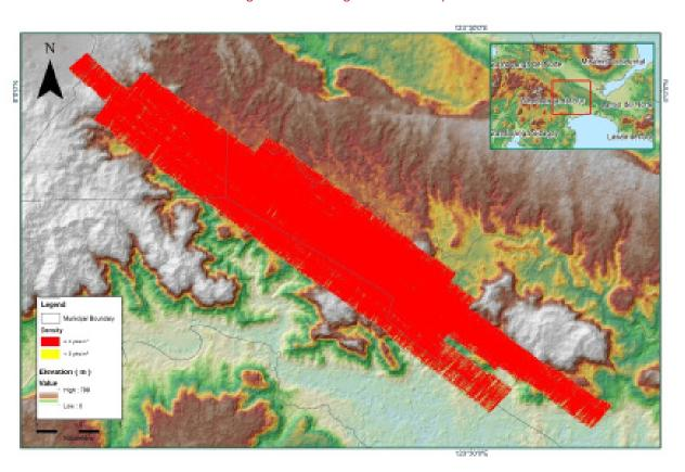
Figure A-8.41. Density map of merged LiDAR data
