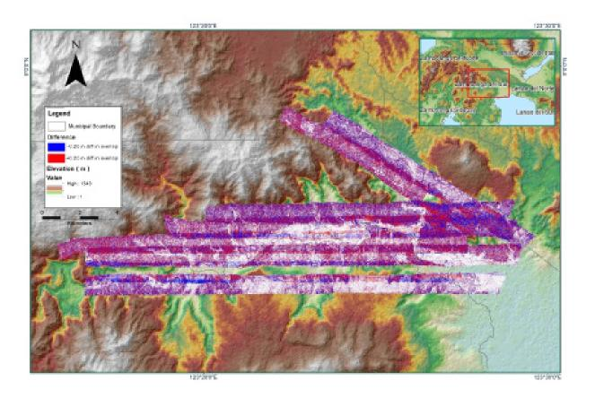
Figure A-8.7. Elevation difference between flight lines
