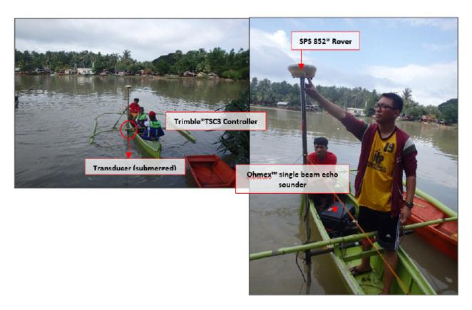
Figure 50. OHMEX™ single beam echo sounder set up on a boat for Labangan River bathymetric survey
