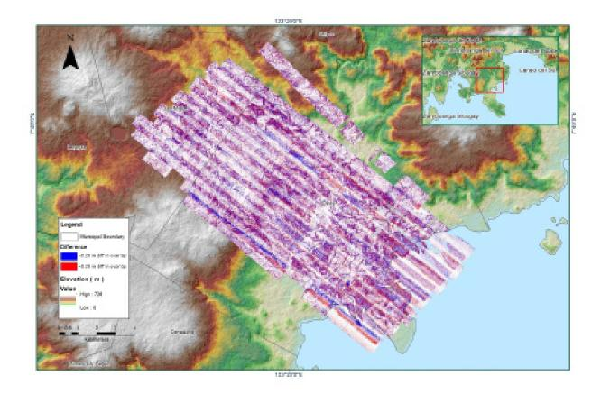
Figure A-8.70. Elevation difference between flight lines
