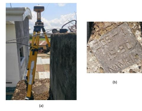
Figure 4. GPS set-up of ZGS-1 at National Irrigation Administration (NIA) compound, Brgy. Dipolo, Molave, Zamboanga del Sur (a) and NAMRIA reference point ZGS-1 (b) as recovered by the field team.
