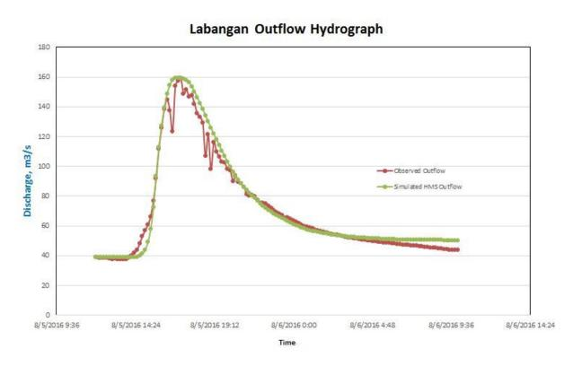
Figure 66. Outflow Hydrograph of Isidro Rey LL. Real III Bridge generated in HEC-HMS model compared with observed outflow
