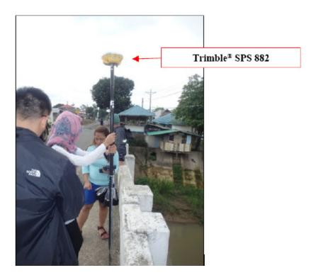
Figure 38. Cross-section survey at Labangan Bridge in Brgy. New Labangan, Labangan, Zamboanga del Sur
