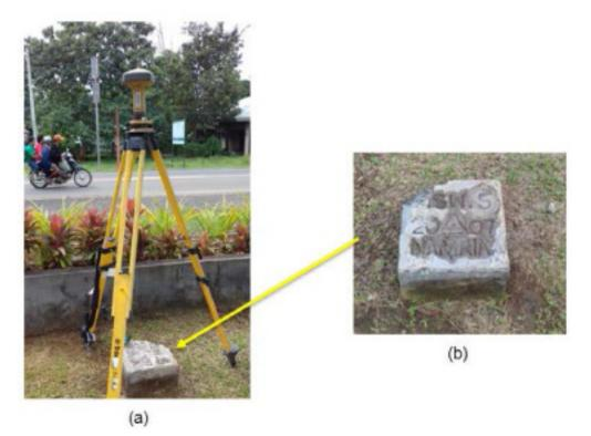
Figure 7. GPS set-up over MSW-05 (a) in Sapang Dalaga, Misamis Occidental and NAMRIA reference point MSW-05 (b) as recovered by the field team.
