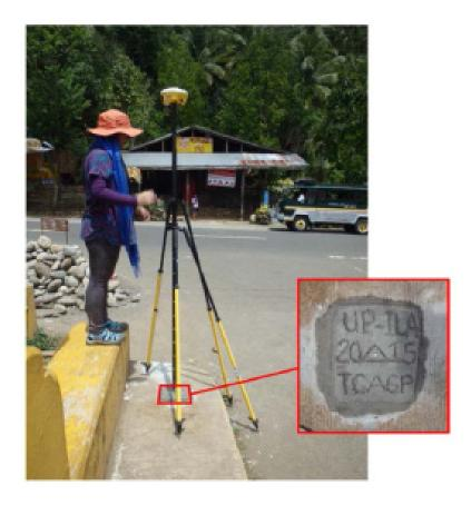
Figure 37. GNSS base receiver, Trimble® SPS 882, setup at UP-ILA in Ilaya Bridge, Brgy. Ilaya, Dapitan City
