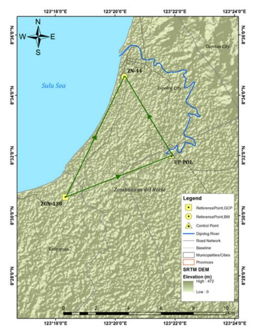
Figure 34. GNSS Network of Dipolog Field Survey
