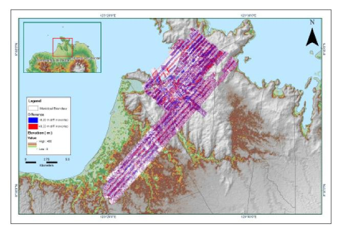
Figure A-8.7. Elevation difference between flight lines
