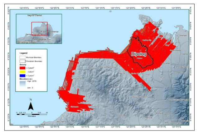
Figure 17. Pulse density map of merged LiDAR data for Dipolog Floodplain.
