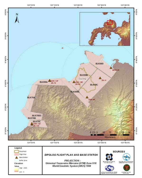
Figure 3. Flight plans and base stations for Dipolog Floodplain.
