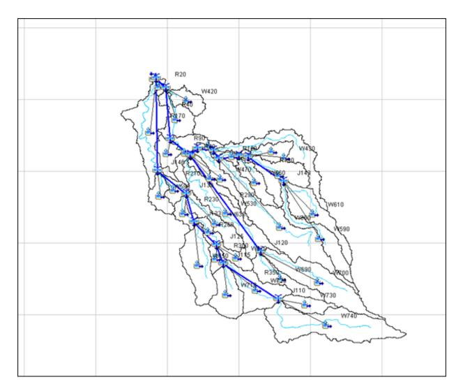
Figure 59. The Dipolog Hydrologic Model generated in HEC-GeoHMS
