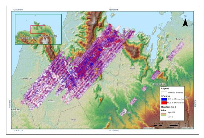
Figure A-8.56. Elevation difference between flight lines
