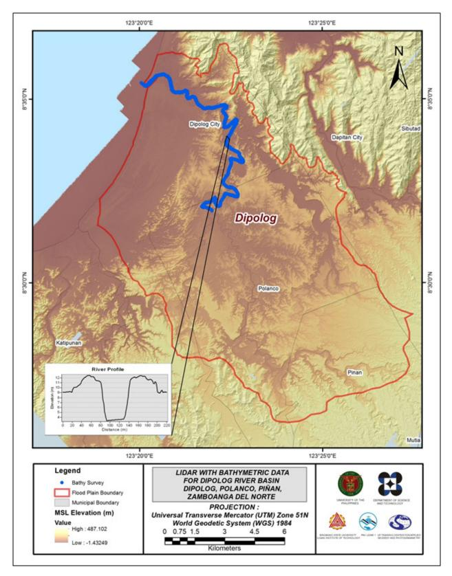
Figure 30. Map of Dipolog Floodplain with bathymetric survey points shown in blue.
