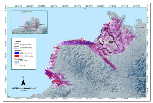
Figure 18. Elevation difference map between flight lines for Dipolog Floodplain.
