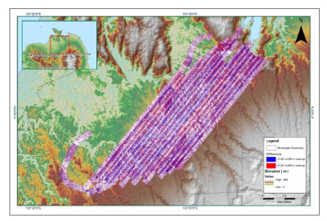
Figure A-8.14. Elevation difference between flight lines
