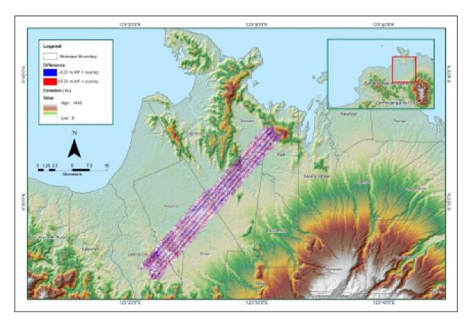
Figure A-8.42. Elevation difference between flight lines
