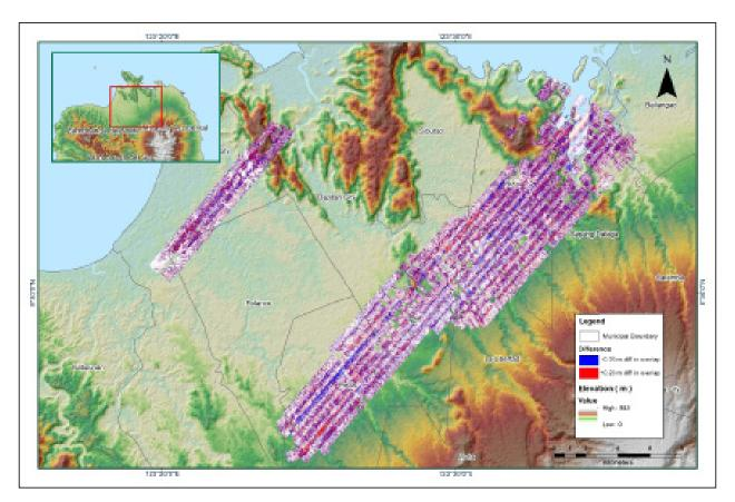
Figure A-8.63. Elevation difference between flight lines
