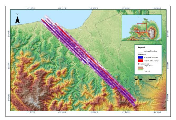
Figure A-8.21. Elevation difference between flight lines
