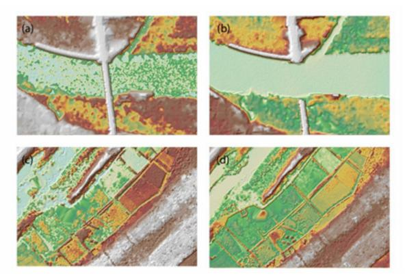
Figure 25. Portions in the DTM of Dipolog Floodplain – a bridge before (a) and after (b) manual editing; a paddy field before (c) and after (d) data retrieval.
