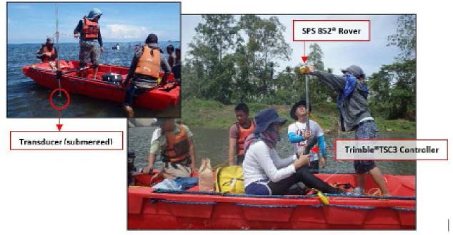
Figure 45. OHMEX™ Single Beam Echo Sounder set up on a rubber boat for the Dipolog River bathymetric survey
