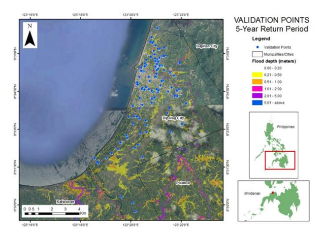
Figure 99. Validation points for 5-year Flood Depth Map of Dipolog Floodplain
