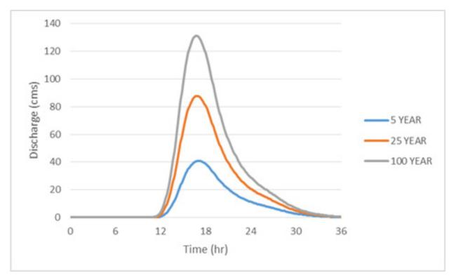
Figure 69. Dipolog river (6) generated discharge
