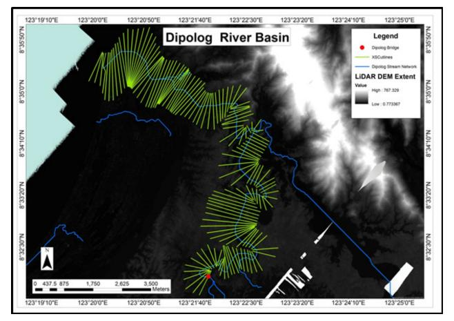
Figure 60. River cross-section of Dipolog River generated through Arcmap HEC GeoRAS tool
