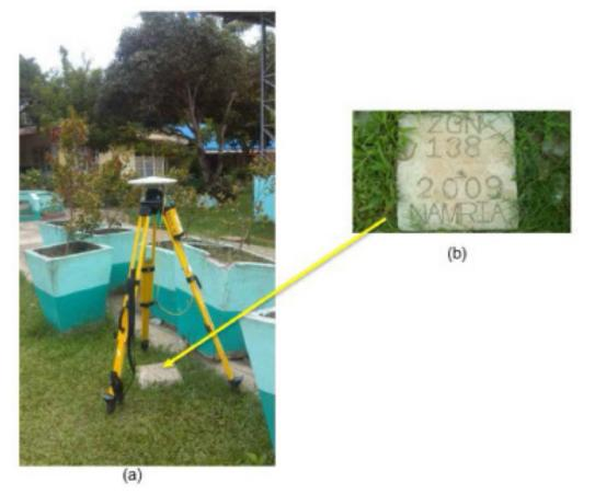
Figure 4. GPS set-up over ZGN-138 (a) in Katipunan Zamboanga del Norte and NAMRIA reference point ZGN-138 (b) as recovered by the field team.
