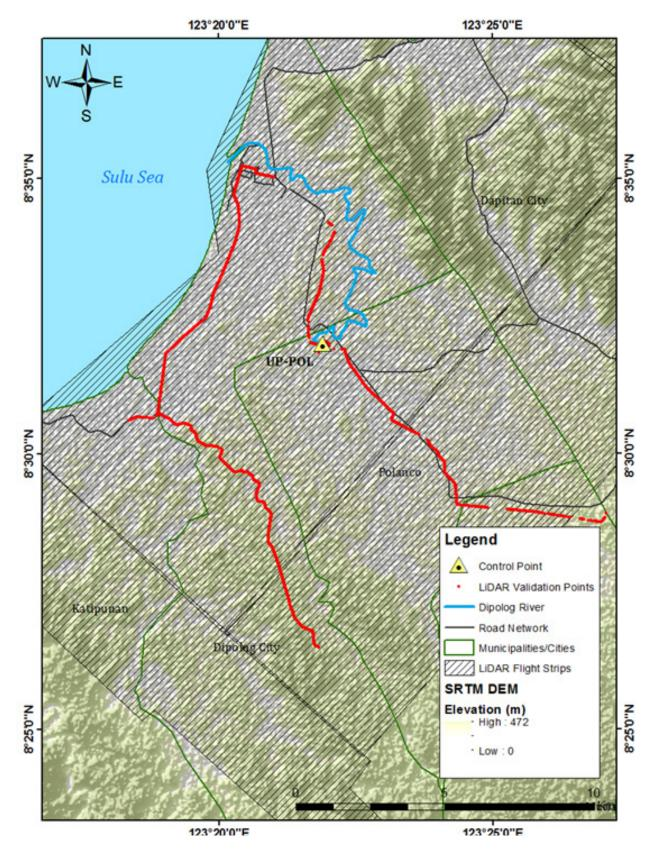
Figure 44. LiDAR Ground Validation Survey along Dipolog City
