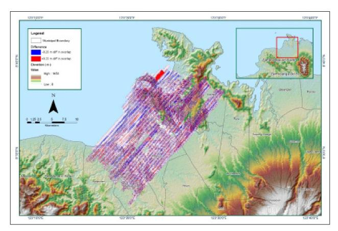
Figure A-8.35. Elevation difference between flight lines
