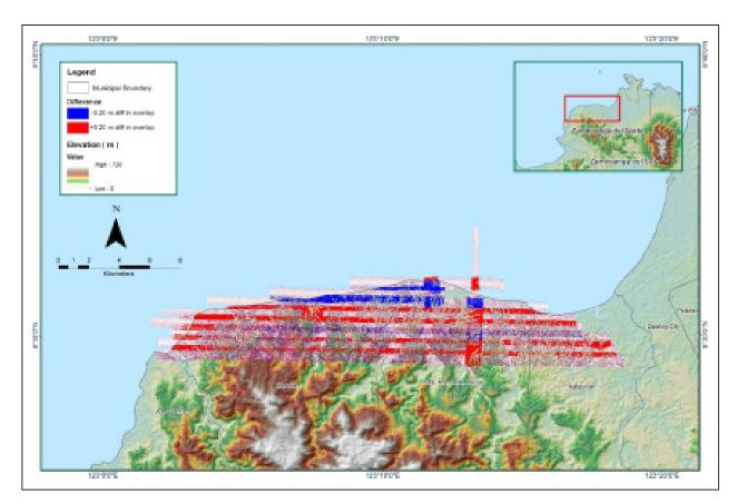
Figure A-8.28. Elevation difference between flight lines
