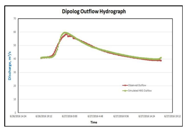
Figure 62. Outflow Hydrograph of Dipolog Bridge generated in HEC-HMS model compared with observed outflow
