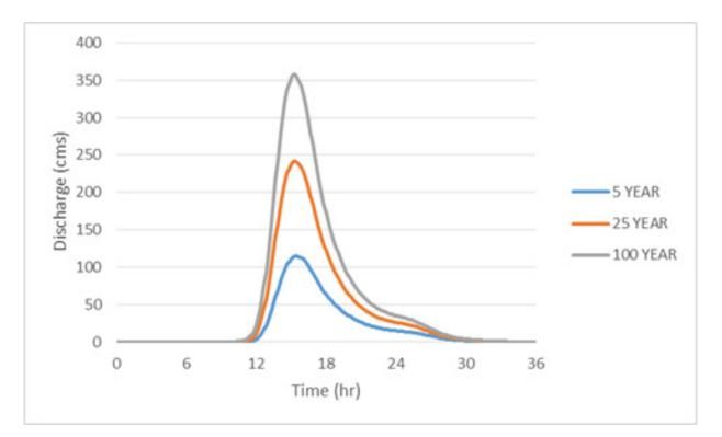
Figure 65. Dipolog river (2) generated discharge
