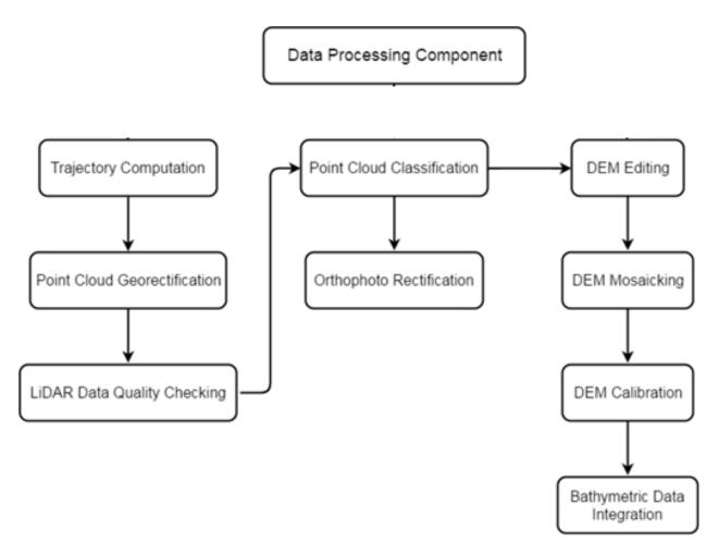
Figure 11. Schematic Diagram for Data Pre-Processing Component
