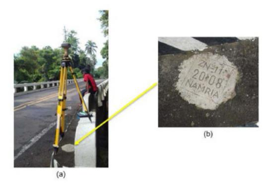
Figure 8. GPS set-up over ZN-11 at Potungan Bridge, Dapitan, Zamboanga del Norte (a) reference point ZN-11 (b) as established by the field team.
