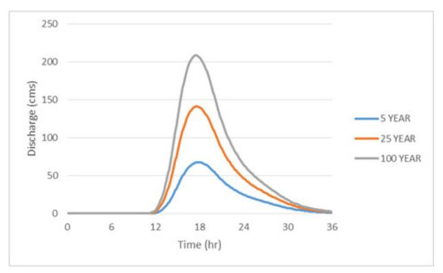
Figure 68. Dipolog river (5) generated discharge
