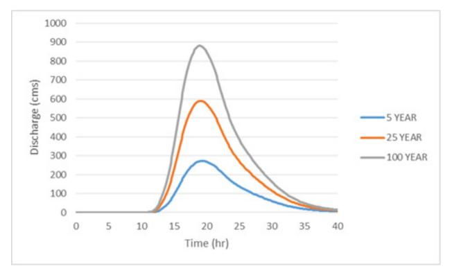
Figure 64. Dipolog river (1) generated discharge
