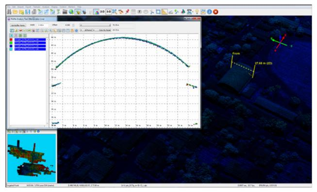
Figure 19. Quality checking for a Dipolog flight 2177P using the Profile Tool of QT Modeler.
