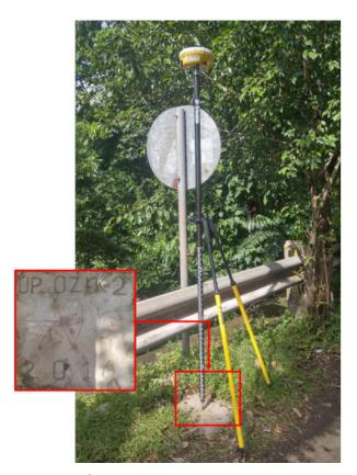
Figure 37. GNSSS setup of Trimble® SPS 852 at UP-OZA2, located near the Ozamiz Steel Bridge approach in Brgy. Mentering, Ozamiz City, Misamis Occidental
