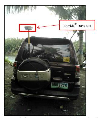
Figure 46. The validation point acquisition survey setup using a GNSS receiver fixed in a vehicle along the Clarin River Basin
