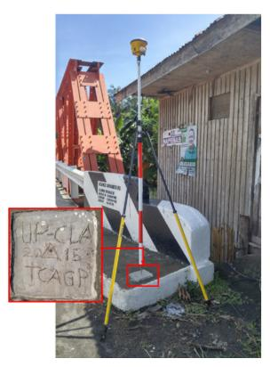
Figure 35. GNSSS setup of Trimble $^{\otimes}$  SPS 985 at CLA, Clarin Bridge approach in Brgy. Poblacion IV, Municipality of Clarin, Misamis Occidental
