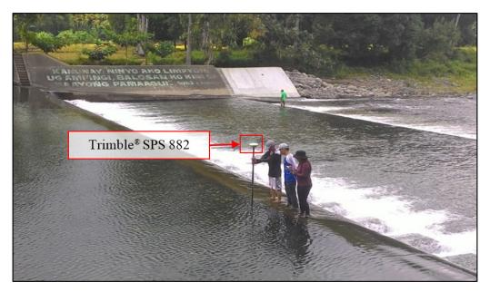
Figure 49. Manual bathymetric survey along Clarin River
