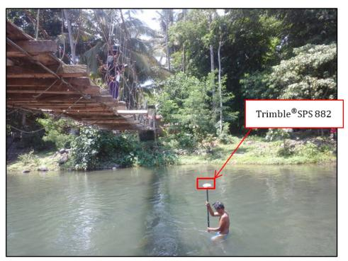
Figure 38. Cross-section survey on the downstream side of Masabud-Pan-ay Hanging Bridge Municipality of Clarin, Misamis Occidental
