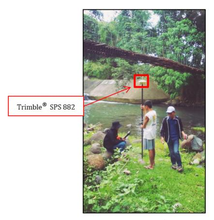
Figure 39. Cross-section survey on the downstream side of Masabud-Canicapan Hanging Bridge, Municipality of Clarin, Misamis Occidental
