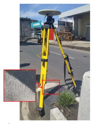
Figure 36. GNSSS setup of Trimble® SPS 852 at MW-42, located at the end of a center island near Citi Hardware in Brgy. Carmen Annex, Ozamiz City, Misamis Occidental
