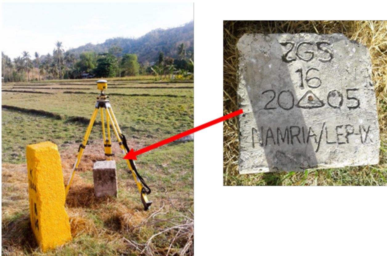
Figure 6. GPS set-up over ZGS-16 at Purok Nangka, Brgy. Baclay, Municipality of Tukuran, Zamboanga del Sur (a) and NAMRIA reference point ZGS-16 (b) as recovered by the field team.
