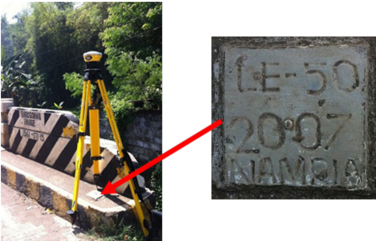
Figure 4. GPS set-up over LE-50 at Barogohan Bridge and at the NE of the Covenant Baptist Church, Maigo, Lanao del Norte (a) and NAMRIA reference point LE-50 (b) as recovered by the field team.
