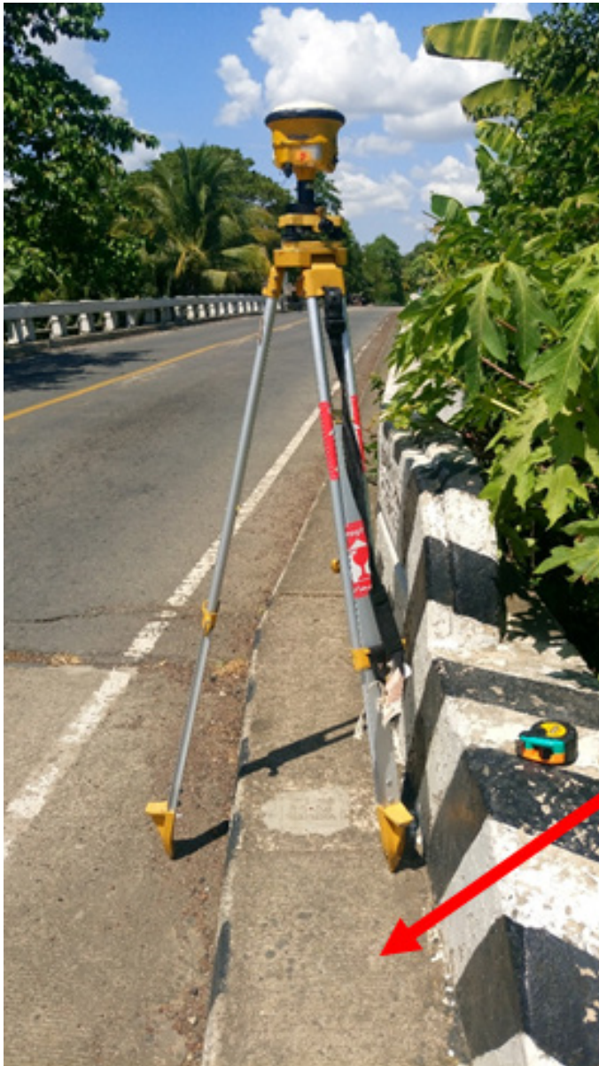
Figure 7. GPS set-up over ZS-188 at Brgy. Licomo, Zamboanga City, Zamboanga del Sur (a) and NAMRIA reference point ZS-188 (b) as recovered by the field team.
