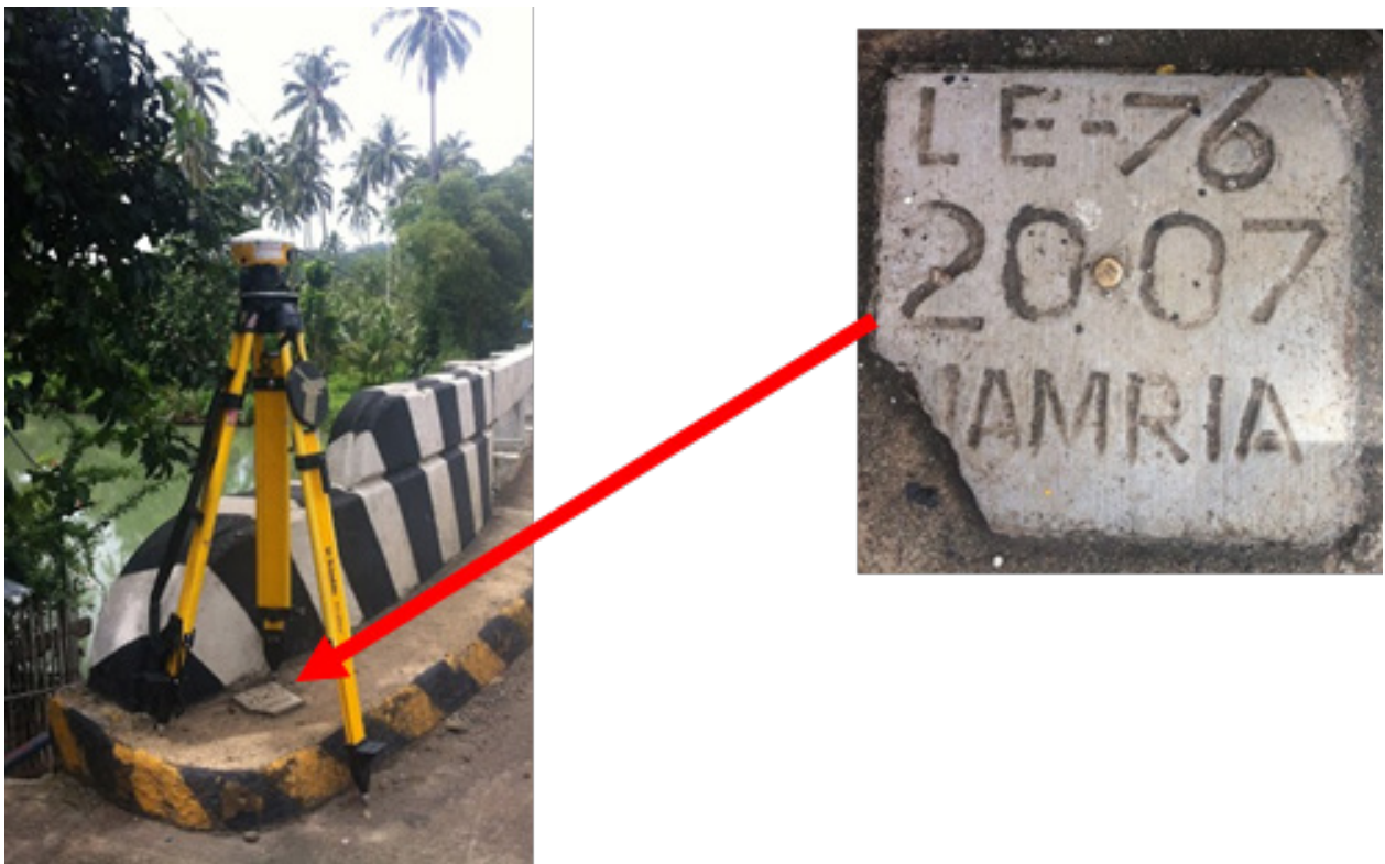
Figure 5. GPS set-up over LE-76 at Bulod Bridge footwalk of Brgy. Bulod, Tubud, Lanao del Norte (a) and NAMRIA reference point LE-76 (b) as recovered by the field team.
