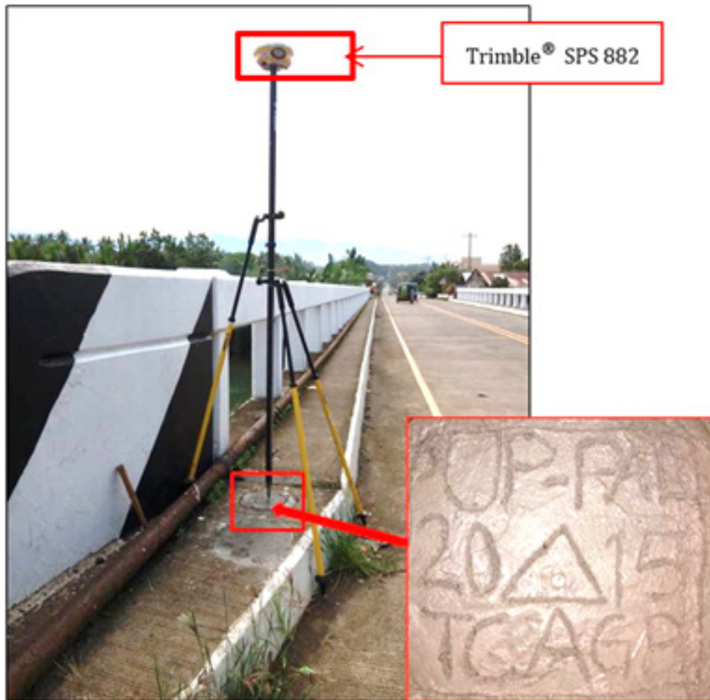
Figure 38. Trimble® SPS 882 setup at UP-PAL, Palilan Bridge approach in Brgy. Rizal, Jimenez, Misamis Occidental
