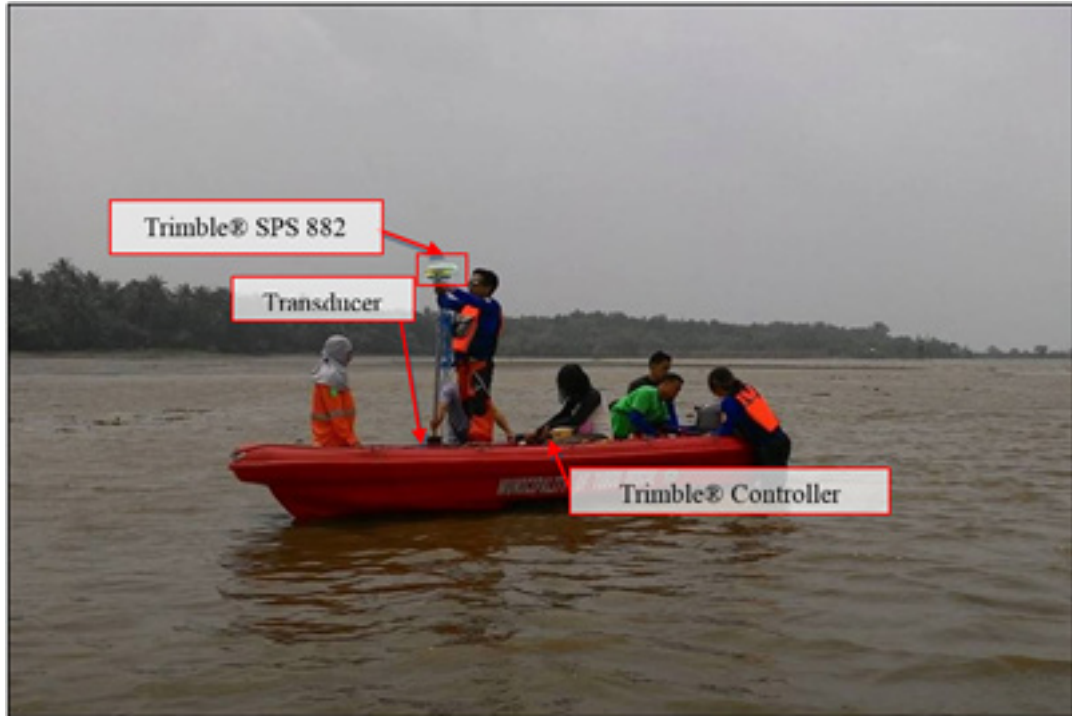
Figure 46. Bathymetric survey using an Ohmex™ single beam echo sounder along Bulod River
