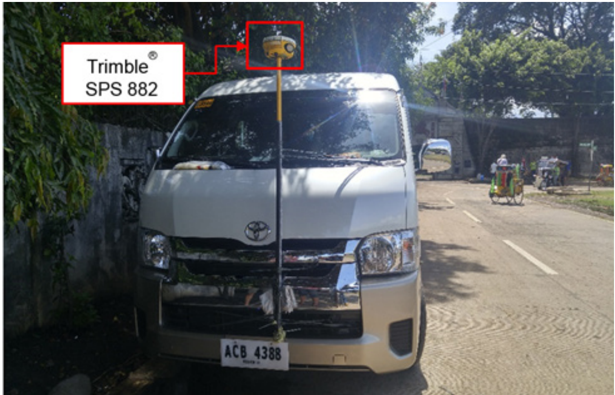
Figure 44. Validation points acquisition survey set up along Bulod River Basin
