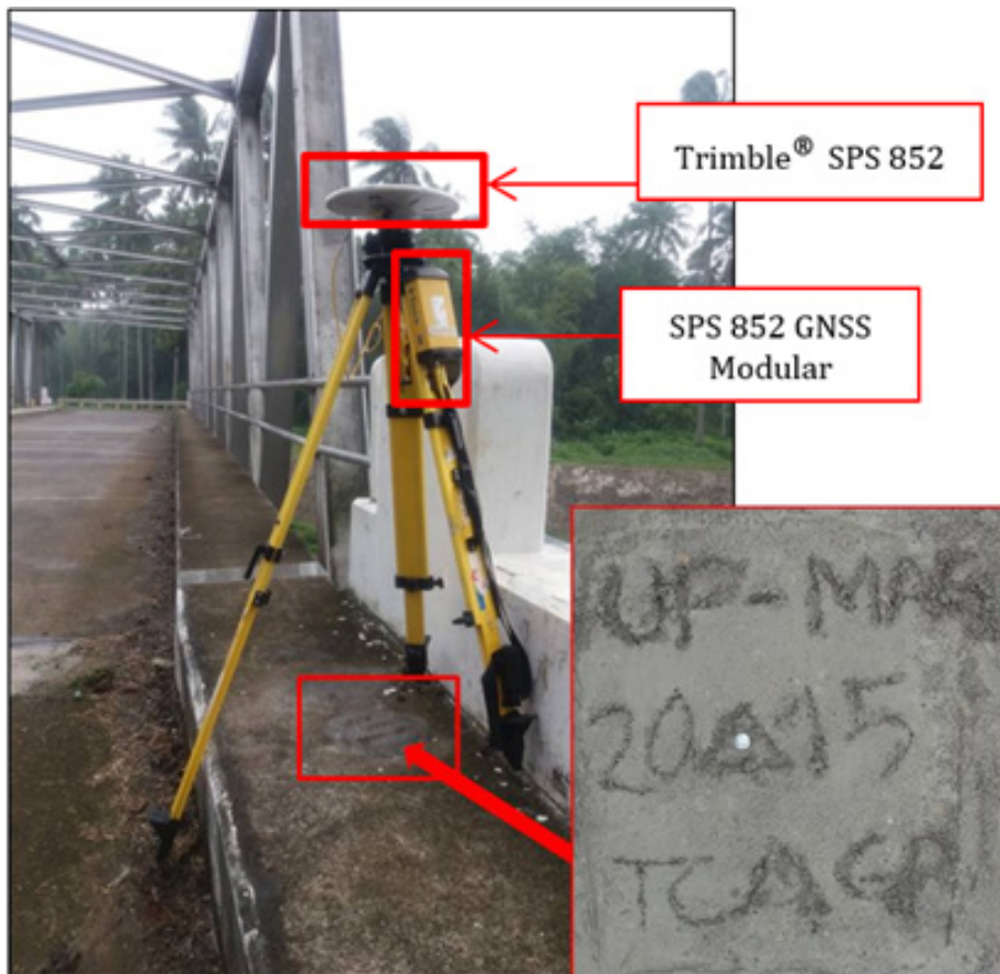
Figure 37. Trimble® SPS 852 setup at UP-MAG, Magsaysay Bridge approach in Brgy. Baguiguicon, Mun. of Magsaysay, Lanao del Norte
