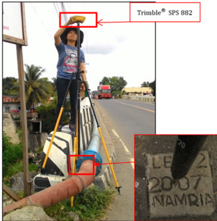
Figure 34. Trimble® SPS 882 setup at LE-92 on the southwest end of Maranding Bridge foot walk in Brgy. Maranding, Mun. of Lala, Lanao del Norte
