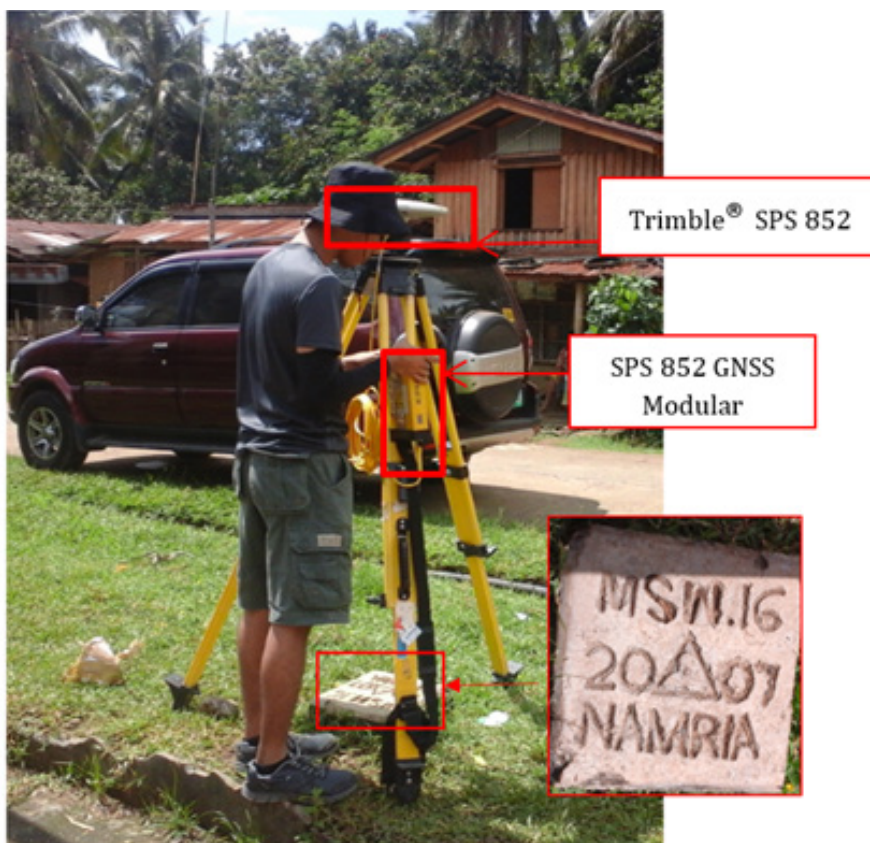
Figure 33. Trimble® SPS 852 setup at MSW-16 beside the fence of the basketball court in Brgy. Stimson Abordo, Ozamiz City, Misamis Occidental
