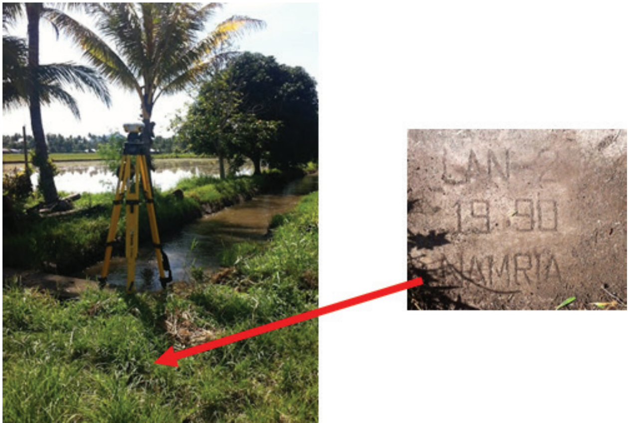
Figure 3. GPS set-up over LAN-2 at Brgy. Pinoyak, Lala Lanao del Norte (a) and NAMRIA reference point LAN-2 (b) as recovered by the field team.
