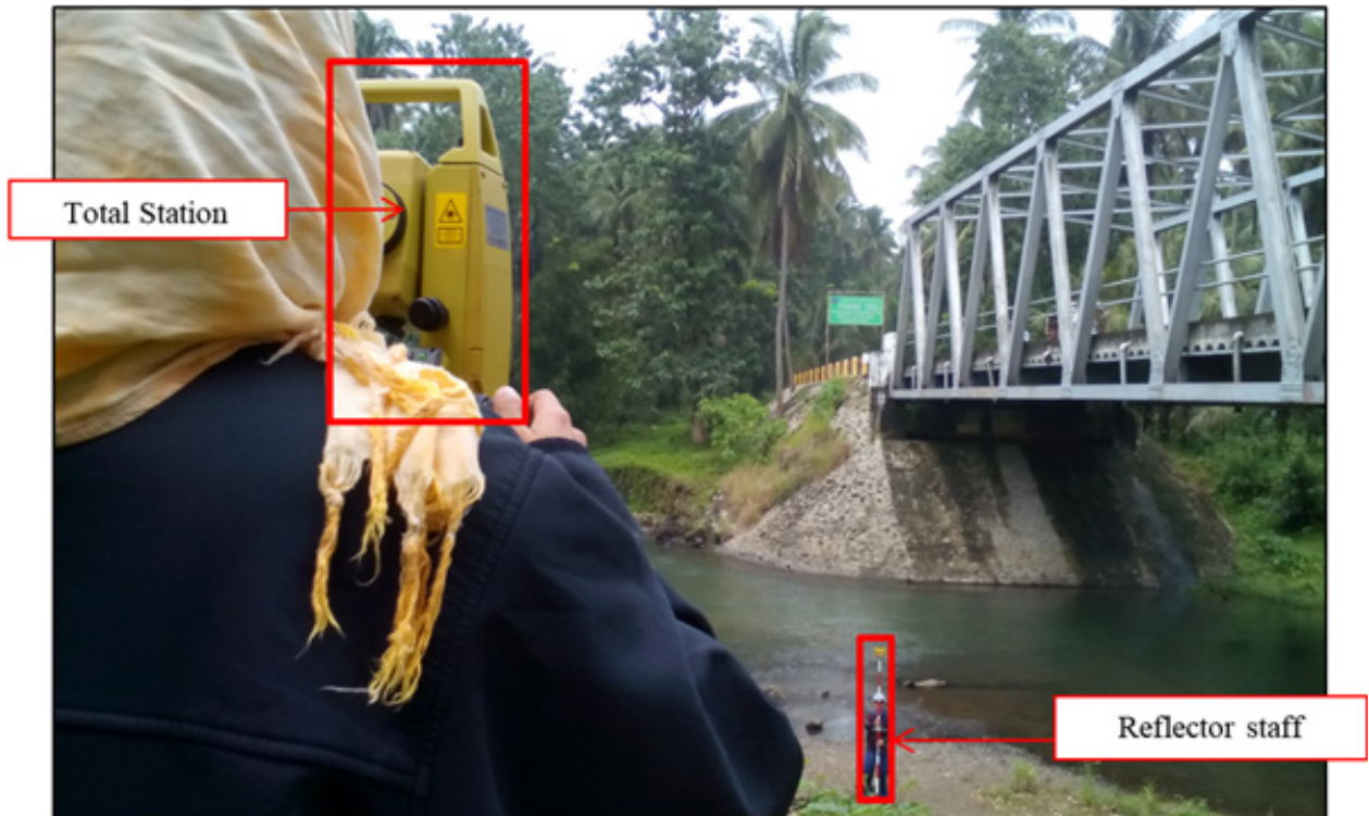
Figure 39. Cross-section for Bulod River along the upstream side of Magsaysay Bridge, Brgy. Sto. Nino, Tubod, Lanao del Norte.
