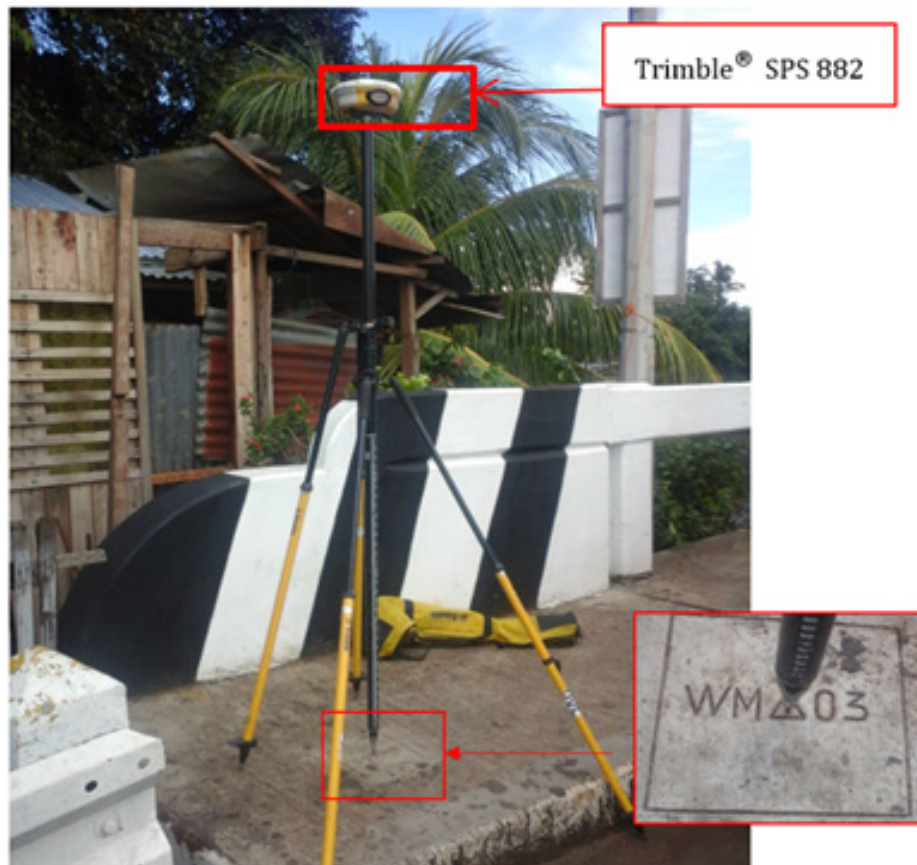
Figure 35. Trimble® SPS 882 setup at WM-03, G. Pelaez Bridge approach in Brgy. Langcangan Lower, Oroquieta City, Misamis Occidental
