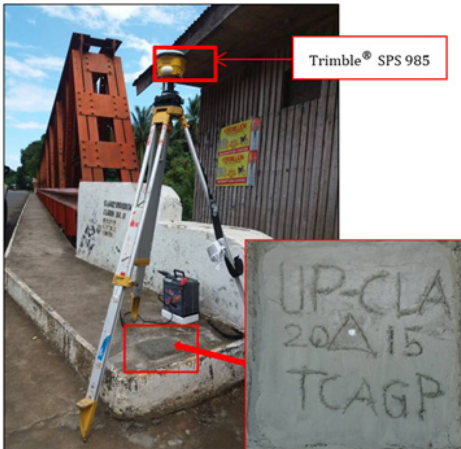
Figure 36. Trimble® SPS 985 setup at UP-CLA, Clarin Bridge approach in Brgy. Poblacion IV, Mun. of Clarin, Misamis Occidental
