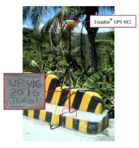
Figure 36. GNSS base set up, Trimble® SPS 882, at UP-VIG, located at the approach of Vigo Bridge in Brgy. Vigo Central, Municipality of San Francisco, Quezon
