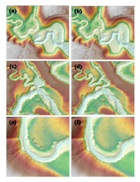
Figure 18. Portions in the DTM of Yabaan Floodplain – a bridge before (a) and after (b) manual editing; an embankment bar before (c) and after (d) data retrieval; and a pit before (e) and after (f) manual editing.
