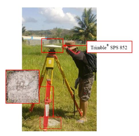
Figure 30. GNSS base set up, Trimble® SPS 852, at QZN-47, located at the back of the Principal's Office of Mulanay Elementary School in Barangay II, Municipality of Mulanay, Quezon.
