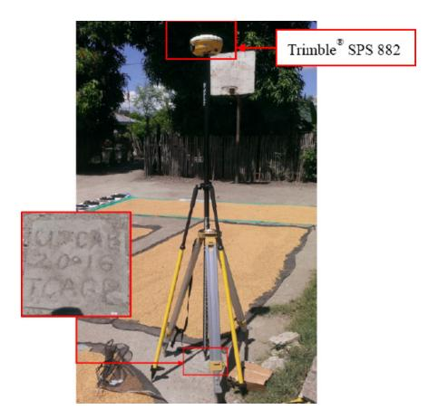
Figure 33. GNSS base set up, Trimble® SPS 882, at UP-CAB, located inside a basketball court in Brgy. Aloneros, Municipality of Guinayangan, Quezon
