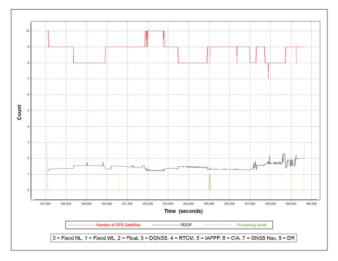
Figure 8. Solution Status Parameters of Yabaan Flight 23342P.
