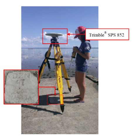
Figure 32. GNSS base set up, Trimble® SPS 852, at QZN-41, located in front of Brgy. Sabang basketball court found in Calauag Port, Barangay I, Municipality of Calauag, Quezon
