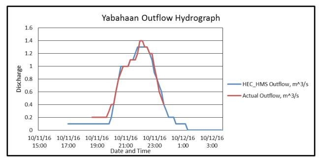
Figure 62. Outflow Hydrograph of Yabaan produced by the HEC-HMS model compared with observed outflow.
