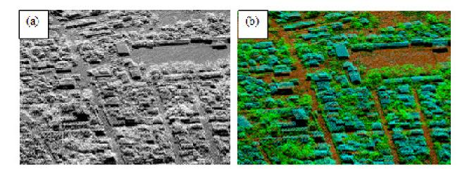
Figure 16. Point cloud before (a) and after (b) classification.
