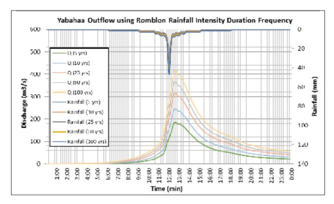
Figure 63. Outflow hydrograph at Yabaan Station generated using Romblon RIDF simulated in HEC-HMS
