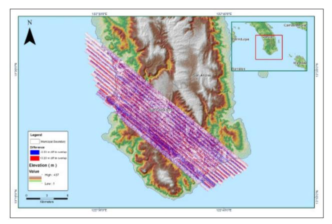
Figure A-8.7. Elevation difference between flight lines
