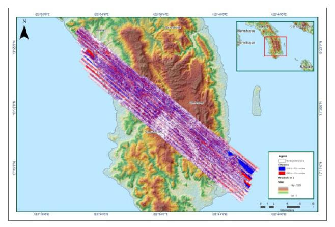
Figure A-8.14. Elevation difference between flight lines
