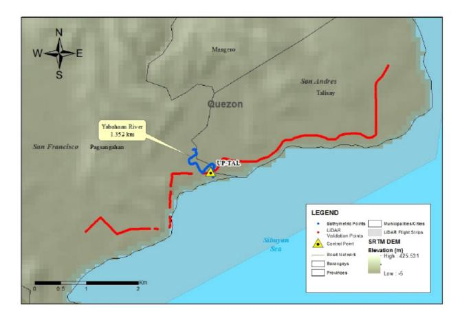
Figure 43. LiDAR validation points acquisition survey for Yabaan River Basin
