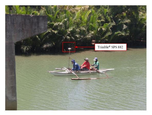
Figure 44. Bathymetry by boat set up for Yabaan River survey
