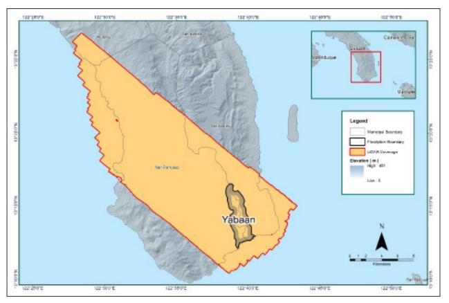
Figure 10. Boundary of the processed LiDAR data on top of a SAR Elevation Data over Yabaan Floodplain.
