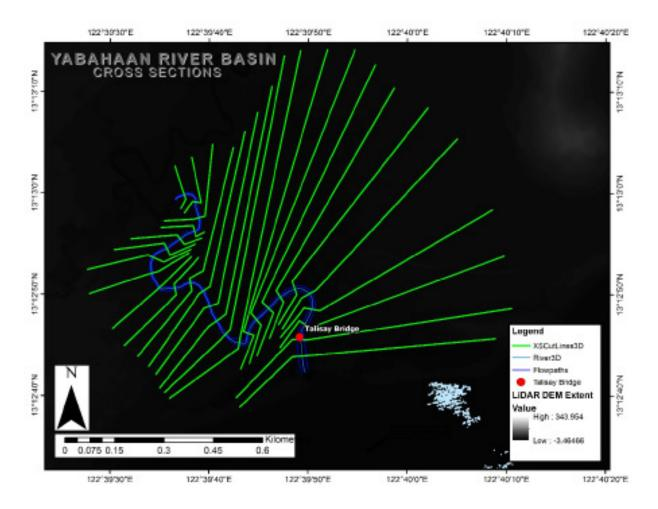
Figure 58. Figure 58. River cross-section of Yabaan (also known as Yabahaan) River generated through Arcmap HEC GeoRAS tool
