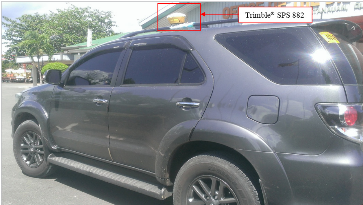
Figure 46. GNSS Receiver Trimble® SPS 882 installed on a vehicle for Ground Validation Survey.
