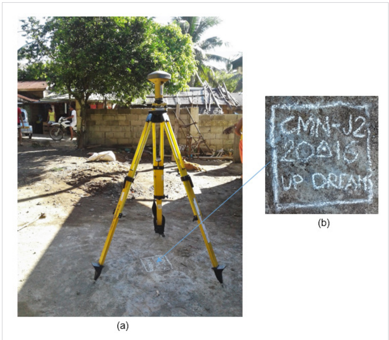
Figure 6. GPS set-up over CMN-J2 as established in at Barangay Maibago, Labo, Camarines Norte (a) and reference point CMN-J2 (b) as established by the field team.
