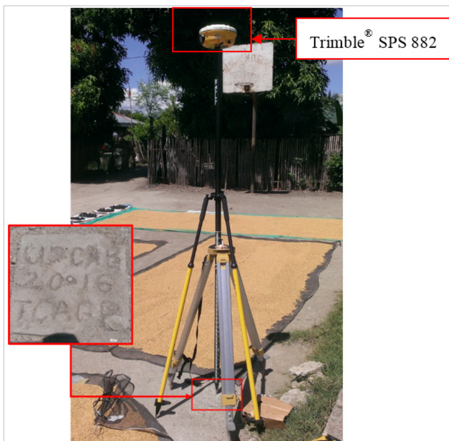
Figure 37. GNSS base set up, Trimble® SPS 882, at UP-CAB, located inside a basketball court in Brgy. Aloneros, Municipality of Guinayangan, Quezon.
