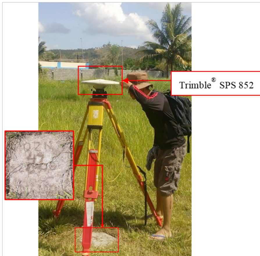
Figure 34. GNSS base set up, Trimble® SPS 852, at QZN-47, located at the back of the Principal's Office of Mulanay Elementary School in Barangay II, Municipality of Mulanay, Quezon.
