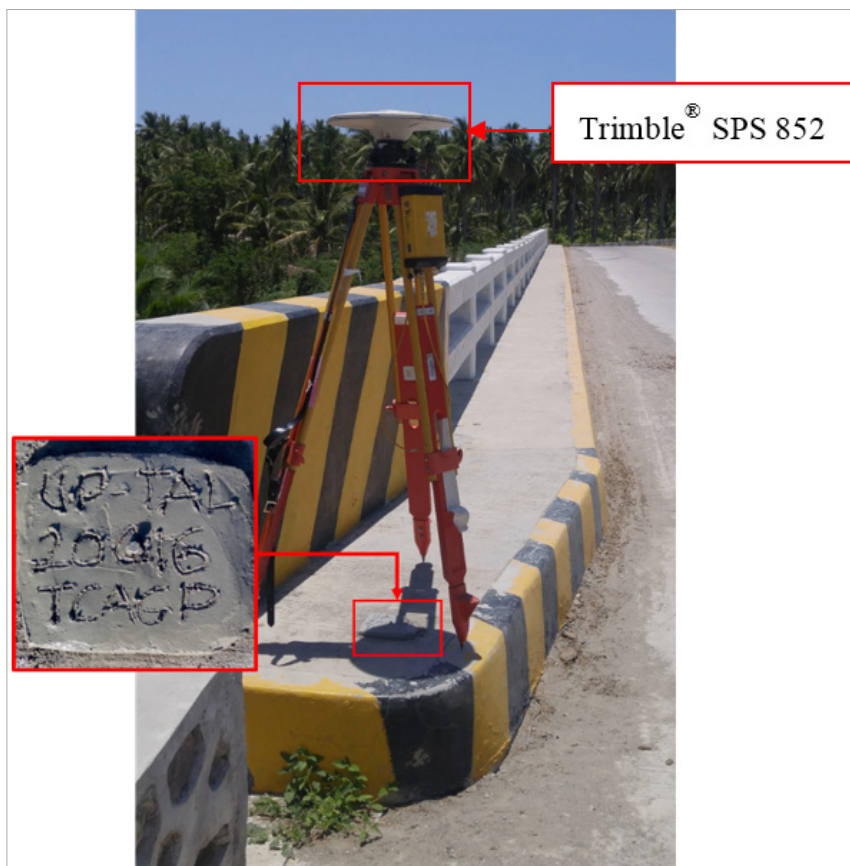
Figure 39. GNSS base set up, Trimble® SPS 852, at UP-TAL, located at the approach of Talisay Bridge in Brgy. Pagsangahan, Municipality of San Francisco, Quezon.
