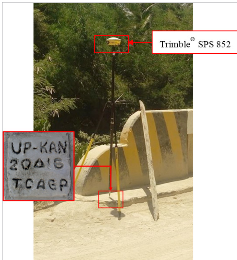
Figure 38. GNSS base set up, Trimble® SPS 852, at UP-KAN, located at the approach of Kanguinsa in Brgy. Silongin, Municipality of San Francisco, Quezon.
