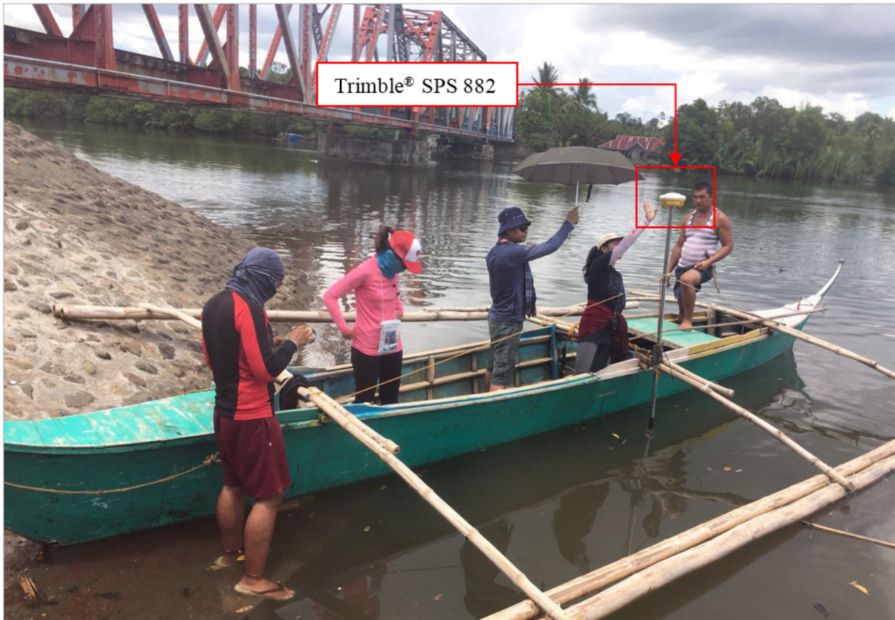
Figure 48. Set up of the bathymetric survey at Cabibihan River.
