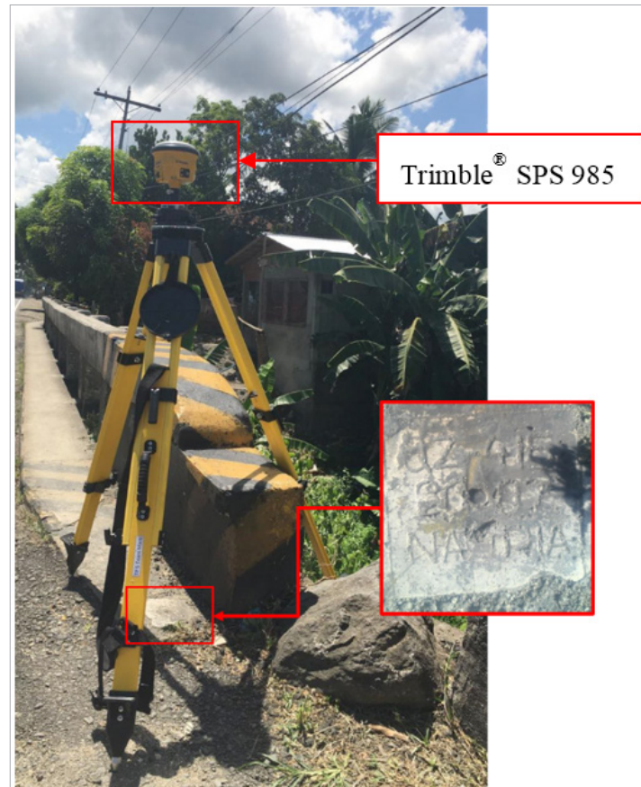
Figure 35. GNSS base set up, Trimble® SPS 985, at QZ-415, located at the approach of Pansol Bridge in Brgy. Pansol, Municipality of Lopez, Quezon.
