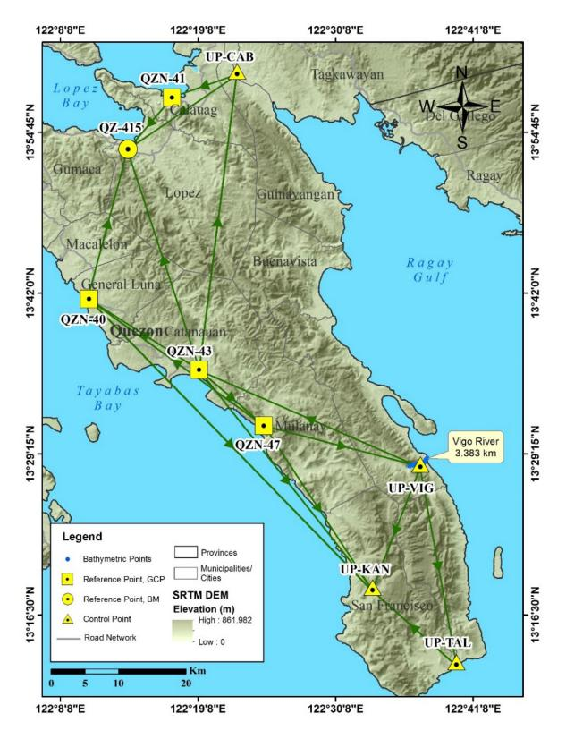
Figure 31. The GNSS Network established in the Vigo River field Survey.
