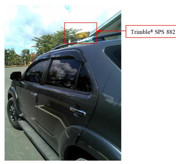
Figure 46. Validation points acquisition survey set up along Vigo River Basin
