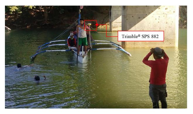
Figure 48. Bathymetric survey using Ohmex™ single beam echo sounder in Vigo River
