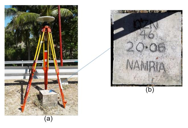
Figure 3. GPS set-up over QZN-46 near the pier in Brgy. Pagdamayan, San Narciso, Quezon (a) and NAMRIA reference point CVT-199 (b) as recovered by the field team.
