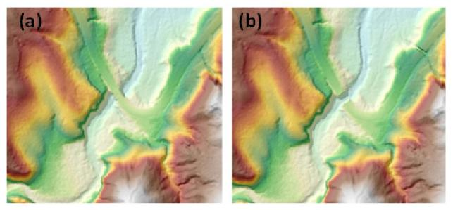
Figure 22. Portions in the DTM of Vigo Floodplain – a bridge before (a) and after (b) manual editing.
