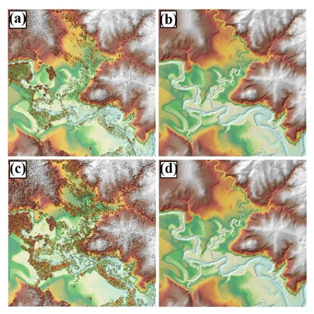
Figure 19. The production of last return DSM (a) and DTM (b), first return DSM (c) and secondary DTM (d) in some portion of Vigo Floodplain.
