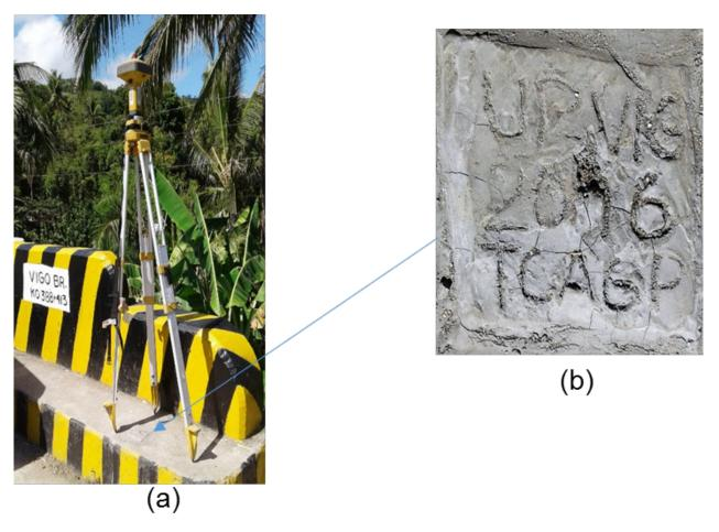
Figure 4. GPS set-up over UP-VIG established in Vigo Bridge along San Narciso-San Andres road in Brgy. Binay, San Narciso, Quezon (a) and established reference point UP-VIG (b) as recovered by the field team.
