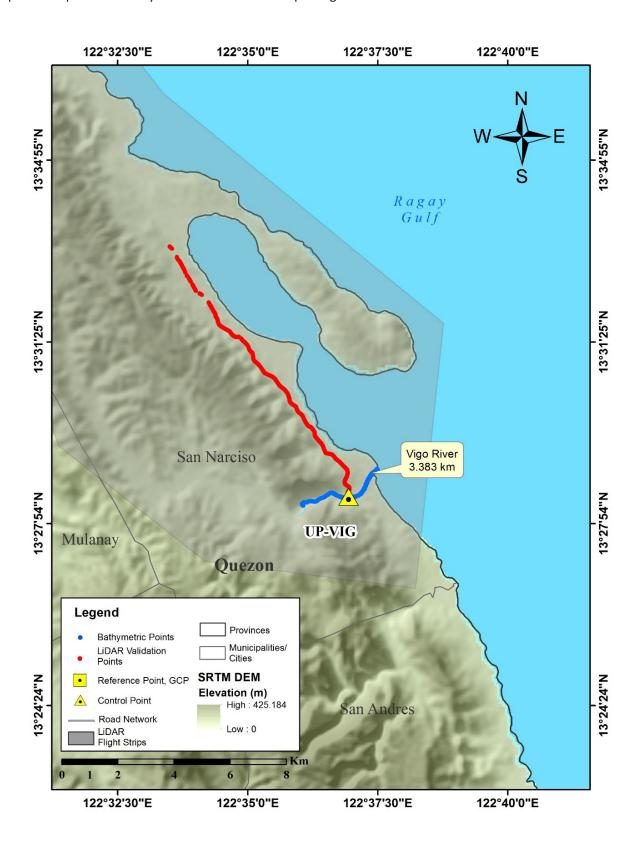
Figure 47. LiDAR validation point acquisition survey for Vigo River basin
