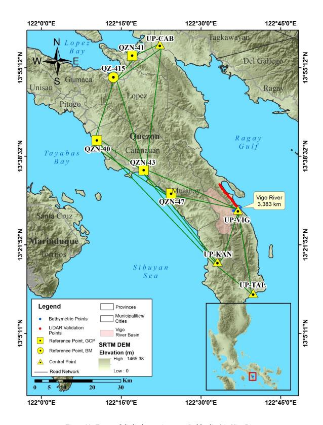
Figure 30. Extent of the bathymetric survey (in blue line) in Vigo River and the LiDAR data validation survey (in red).
