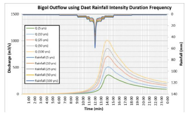
Figure 67. Outflow hydrograph at Vigo (also known as Bigol) Station generated using Daet RIDF simulated in HEC-HMS
