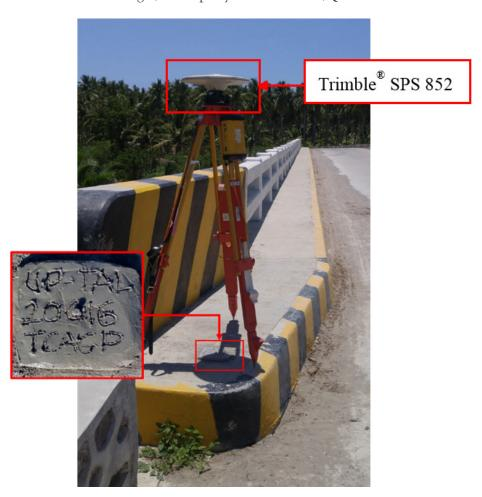
Figure 39. GNSS base set up, Trimble® SPS 852, at UP-TAL, located at the approach of Talisay Bridge in Brgy. Pagsangahan, Municipality of San Francisco, Quezon
