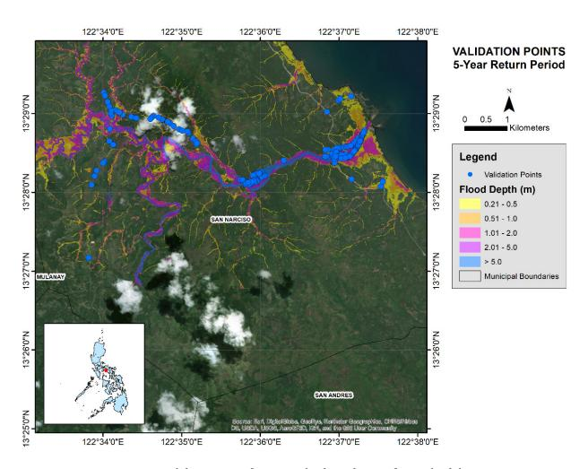
Figure 81. Validation points for 5-year Flood Depth Map of Vigo Floodplain
