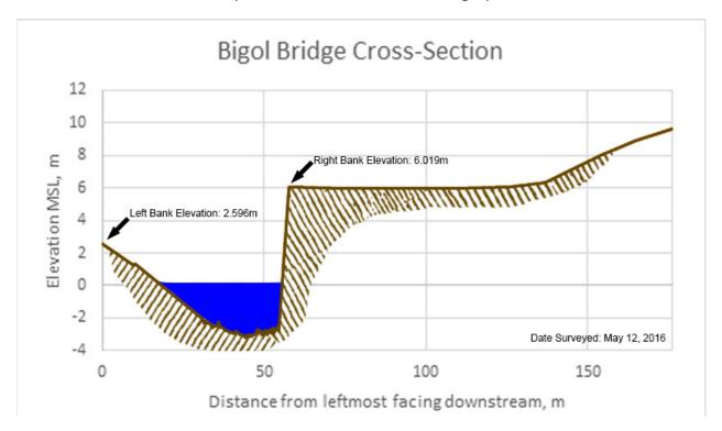
Figure 52. Cross-Section Plot of Vigo (also known as Bigol) Bridge
