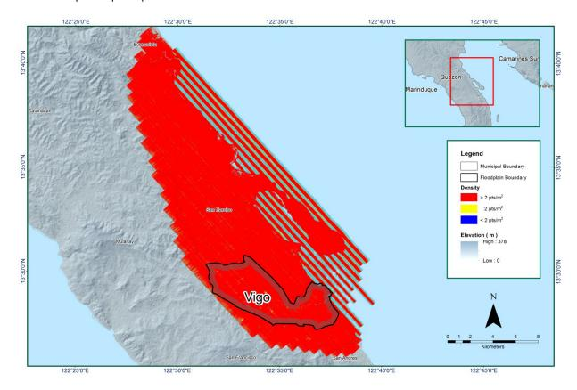
Figure 14. Pulse density map of merged LiDAR data for Vigo Floodplain.
