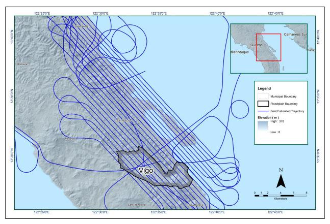
Figure 11. Best estimated trajectory of the LiDAR missions conducted over the Vigo Floodplain.
