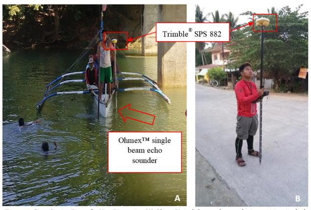
Figure 41. Cross-Section Survey for Vigo River using (A) Ohmex™ single beam echo sounder in acquiring riverbed elevation for the cross sectional points and (B) Trimble® SPS 882 in PPK survey technique for the acquiring cros section and as-built points
