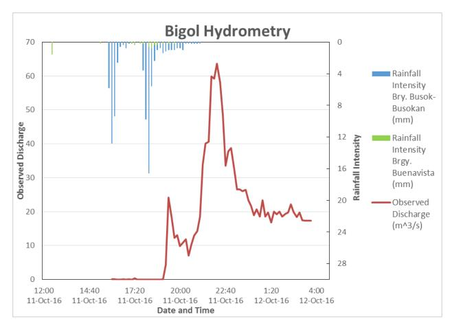
Figure 54. Rainflow and outflow data at Vigo (also known as Bigol) River used for modeling
