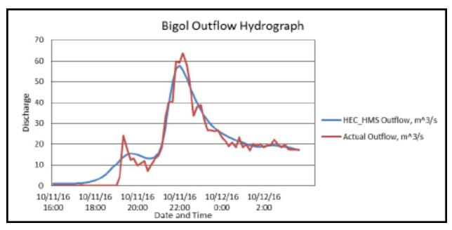
Figure 66. Outflow Hydrograph of Vigo (also known as Bigol) River produced by the HEC-HMS model compared with observed outflow.
