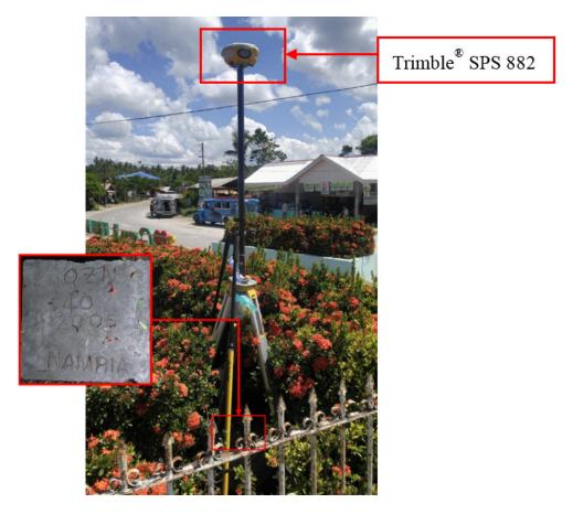
Figure 32. GNSS base set up, Trimble® SPS 882, at QZN-40, located inside a triangular plant area found at the center of a triangular island in Brgy. San Jose, Municipality of Gen. San Narciso, Quezon
