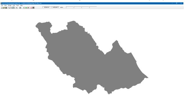
Figure 63. A screenshot of the river sub-catchment with the computational area to be modeled in FLO-2D Grid Developer System Pro (FLO-2D GDS Pro)
