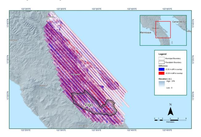
Figure 15. Elevation Difference Map between flight lines for Vigo Floodplain Survey.
