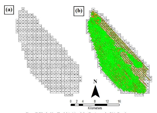
Figure 17. Tiles for Vigo Floodplain (a) and classification results (b) in TerraScan.
